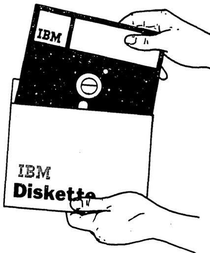
Return the diskette to its protective envelope whenever it is removed from the diskette drive and whenever you are writing on a label on the diskette.
