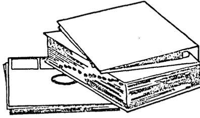
Do not erase labels attached to the diskette, or make any erasures on or near the diskette. Erasure residue could get in the diskette, and this should be avoided. To discourage erasures, IBM recommends that you use a fiber-tip or ball-point pen when marking on the diskette labels. Mark temporary labels before attaching them to the diskette. Alter temporary labels with the diskette in the envelope.
