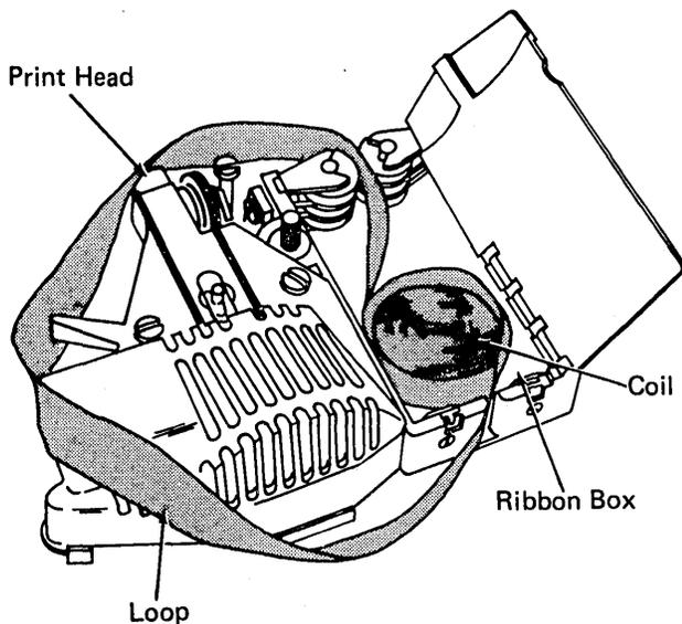
10. Eject the new ribbon from its holder into the ribbon box by pressing on the disk.
