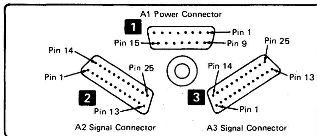
**B** I/O Cable Assembly Connector
