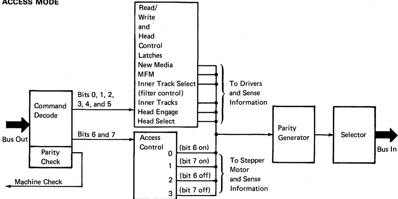
In access mode, the system can check the status of the drive and diskette, move the heads, select the correct side and current, and load or unload the heads. The adapter is in access mode when no read, write, or diagnostic operation is in progress, and a diskette drive has been selected.
