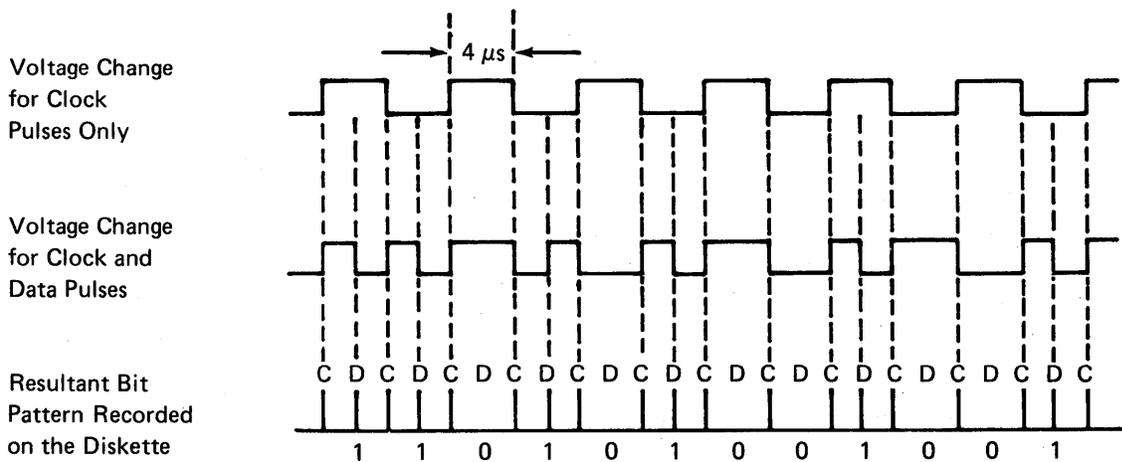
The C and D above the line show the clock and data bit times.
