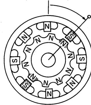
*Note:* Current flows only in one-half of the winding at a time. Polarity of the stator poles is determined by which half of the winding has the current flow.
