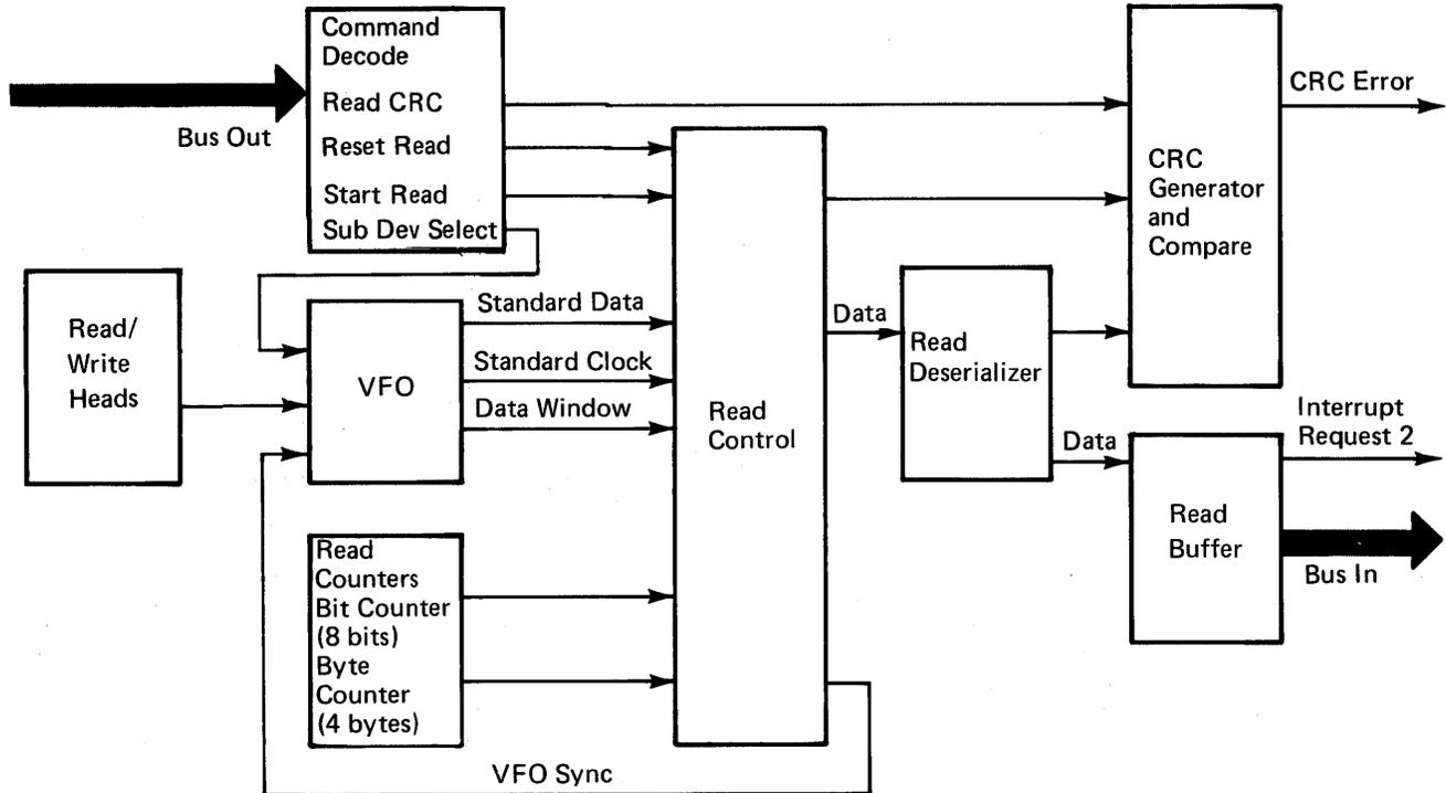
The correct drive, head, and track for a read operation is selected during access mode. A read operation senses data that has been recorded on a diskette and sends this data to the system. The data rate for read operation is 48k bytes/seconds.
