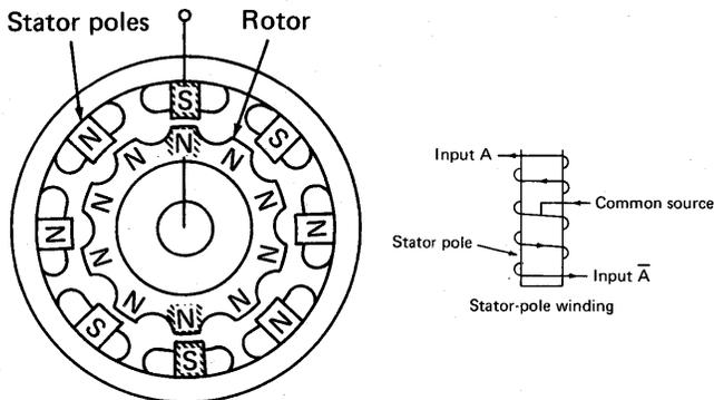
If you could rotate the stator in either direction, the rotor would maintain its detented position and follow the stator as shown. Both the stator poles and the rotor are shown rotated  $45^\circ$  clockwise.
