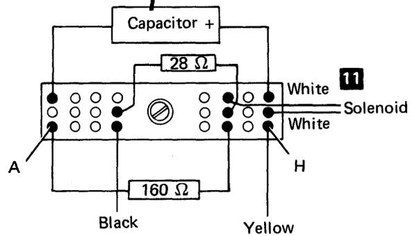
This illustrates machines without EC 836576. Machines with EC 836576 will not have this terminal block or associated components.
