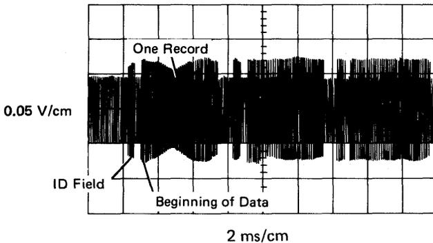
*Note:* Use Tektronix 453, 454, or similar oscilloscope with x10 probes.
