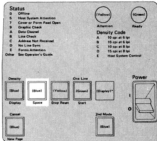
Pressing the Space key advances the forms one line if the Ready light is off and the display shows a 0, C, D, or blank.
