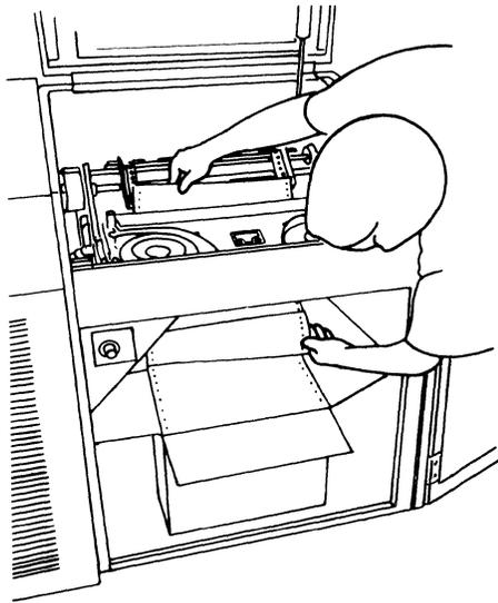
5. Place the form's left margin holes over the left tractor pins, close the tractor cover, and tighten the tractor knob.
