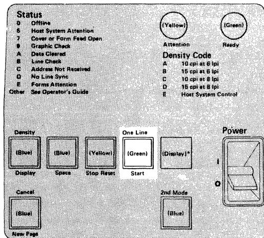
Pressing the Start key causes the Ready light to come on and begins the function selected by the Mode Switch. The display must show 0, C, D, or blank for this to occur.
