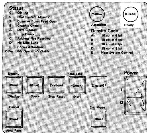
When the green Ready light is on and the printer is online (the Mode Switch is set to Online or Buffer Print), the printer is ready to print data it receives from the host.
