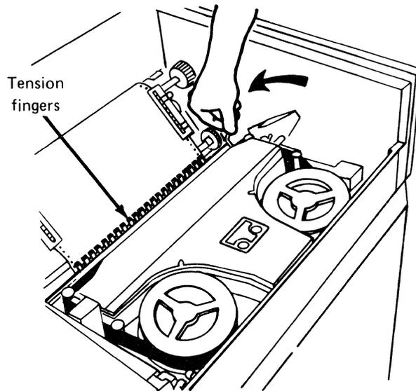
3. Close the forms feed by pulling it toward the front of the printer until it is locked in place.
