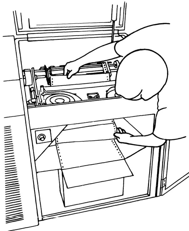
8. Close the forms feed by pulling it toward the front of the printer until it is locked in place.
