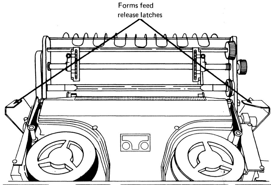
Pushing both forms feed release latches downward opens the forms feed for loading or unloading forms, and for changing the ribbon and ribbon shield.
