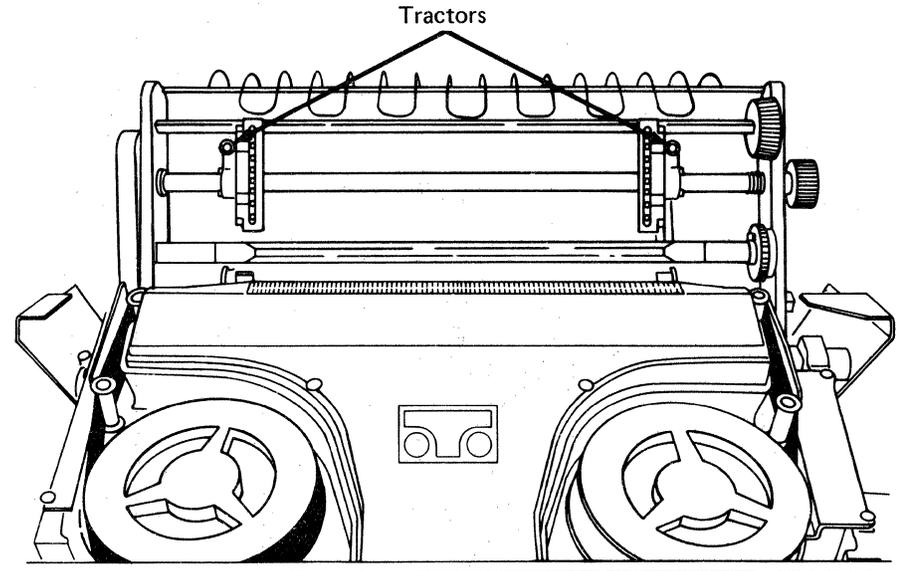
Loosening the tractor locking knobs allows the tractors to be moved so that forms of different widths can be used.
