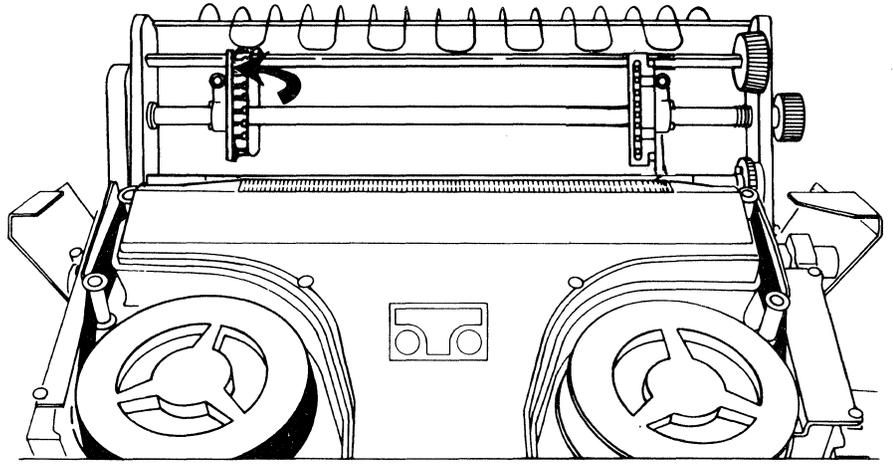
5. Release the forms feed by pushing down on the release latches **B**.
