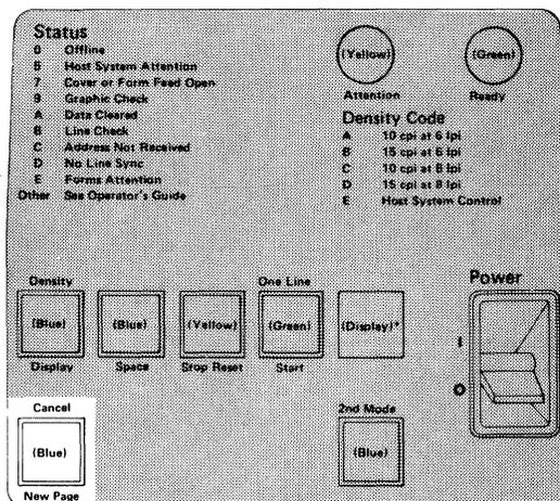
Pressing the New Page key advances the forms to the first print line of the next form. The Ready light must be off and the display must be 0, C, D, or blank for this to occur. In addition, the printer must have received a command from the host defining the page length according to the physical forms length. If this command is not received, or if the printer is offline, the forms advance only one line.
