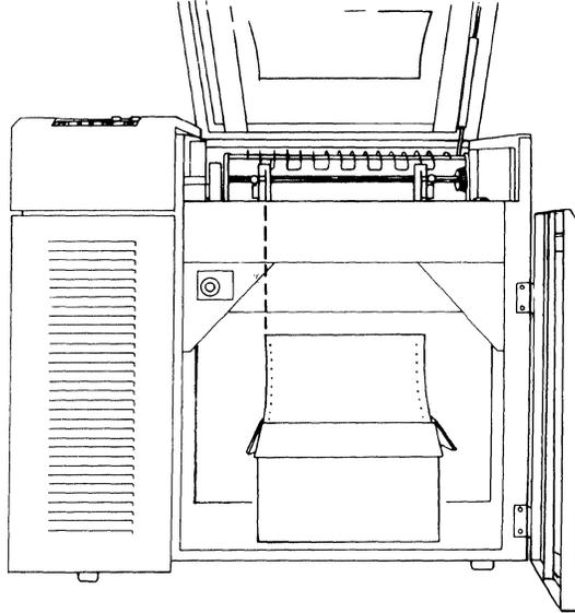
4. Feed the forms up between the forms feed and tension fingers.
