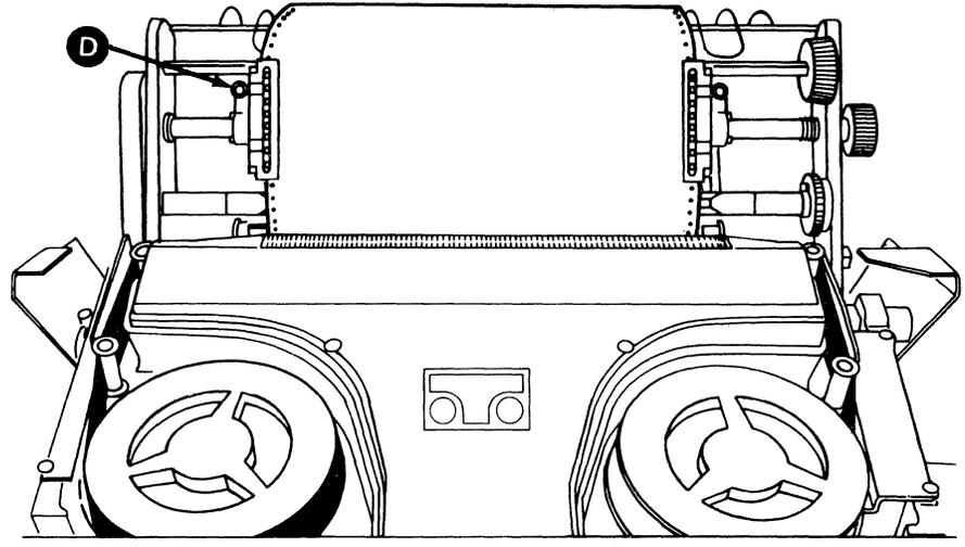
**Note:** If you are using multipart forms, ensure that the tractor pins fit completely through all the margin holes.
