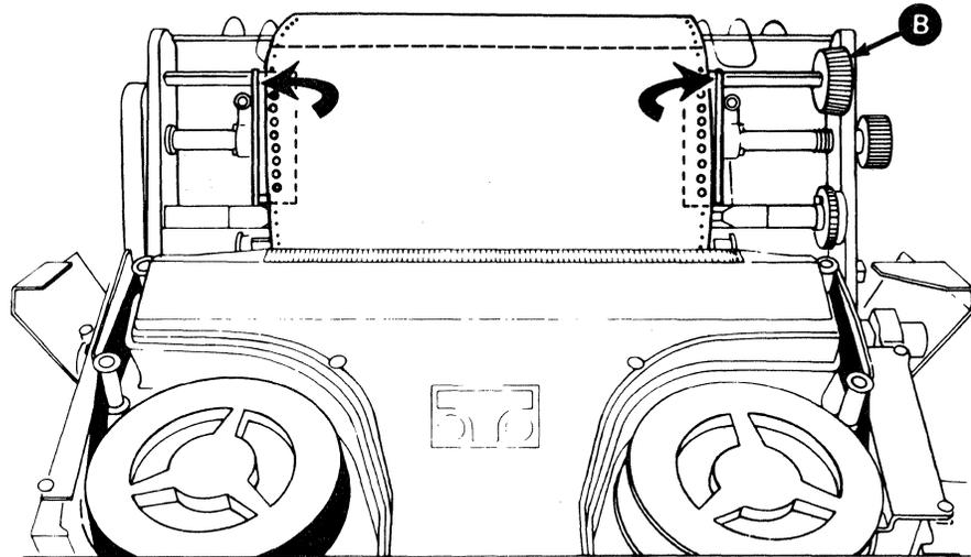
7. Unload the forms by pulling them off of the tractor pins and downward out of the printer.
