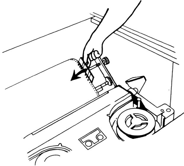
**Note:** If forms are wider than 375 millimeters (14.8 inches), you may have to readjust the left tractor.
