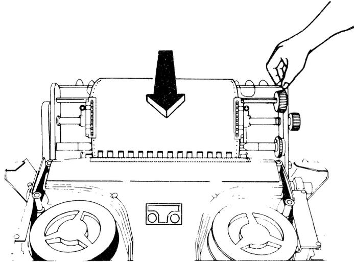
4. Turn the horizontal adjustment control to align the first print position with the forms alignment scale.
