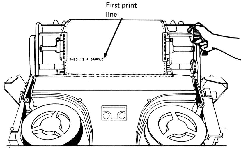
2. Push the tension fingers to the rear of the printer.
