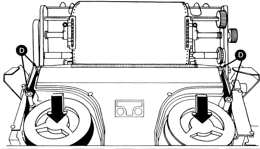
5. Close the forms feed by pulling it toward the front of the printer until it is locked in place.
