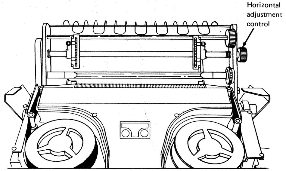
Turning the horizontal adjustment control moves both tractors in the same direction for fine horizontal alignment of the forms when aligning the print positions. The total span of movement is approximately 15 millimeters (0.6 inch). The horizontal adjustment control is used with the alignment scale.
