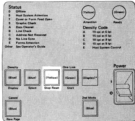
The Stop Reset key has two purposes. Pressing the Stop Reset key stops the printer after completion of the line being printed or at the end of forms movement. The Ready light goes off and the Attention light goes on.
