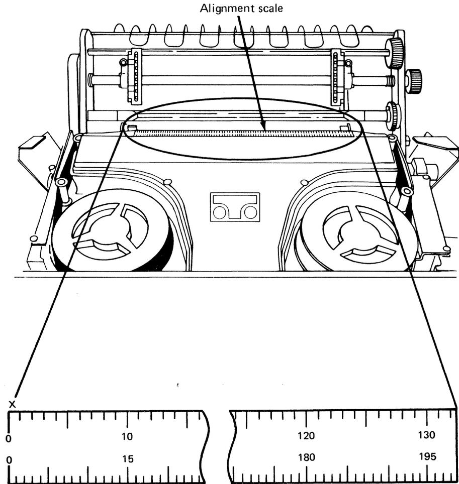
The first possible print position (X) is between the 0 and the 1 mark on the alignment scale.
