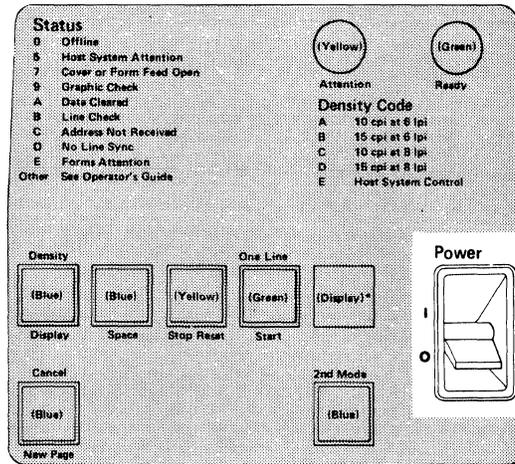
Placing the Power switch in the | (on) position switches on the printer power; placing the Power switch in the O (off) position switches off the printer power.
