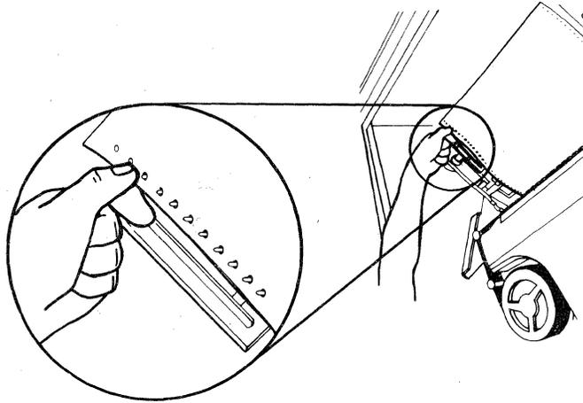
6. Loosen the right tractor locking knob **C**, open the tractor cover, and align the tractor pins with the right margin holes of the forms.
