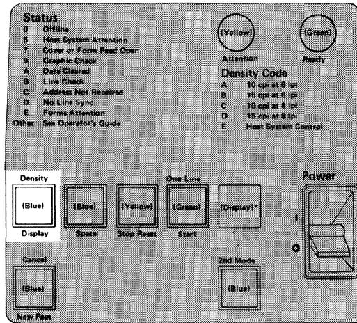
Pressing the Display key displays the current density code. The Ready light must be off and the display must be 0, C, D, or blank for this to occur.
