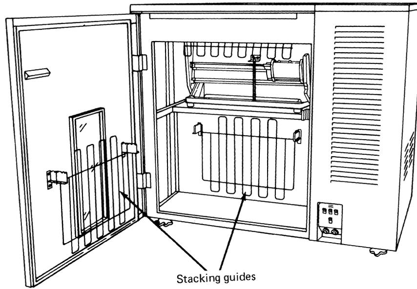
The two stacking guides inside the rear door are adjustable to accommodate forms of various lengths (between folds).
