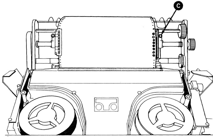
7. Place the form's right margin holes over the right tractor pins. Close the tractor cover and tighten the tractor locking knob.
