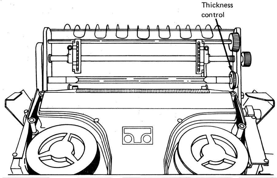
Turning the thickness control adjusts the print impressions on the forms. The correct thickness control setting depends on the forms thickness, type, quality, size, and number of copies. (See "C. Adjusting the Thickness Control" in Chapter 3.)
