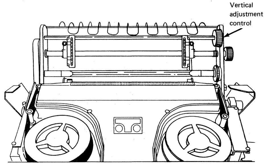
Turning the vertical adjustment control moves the forms vertically.
