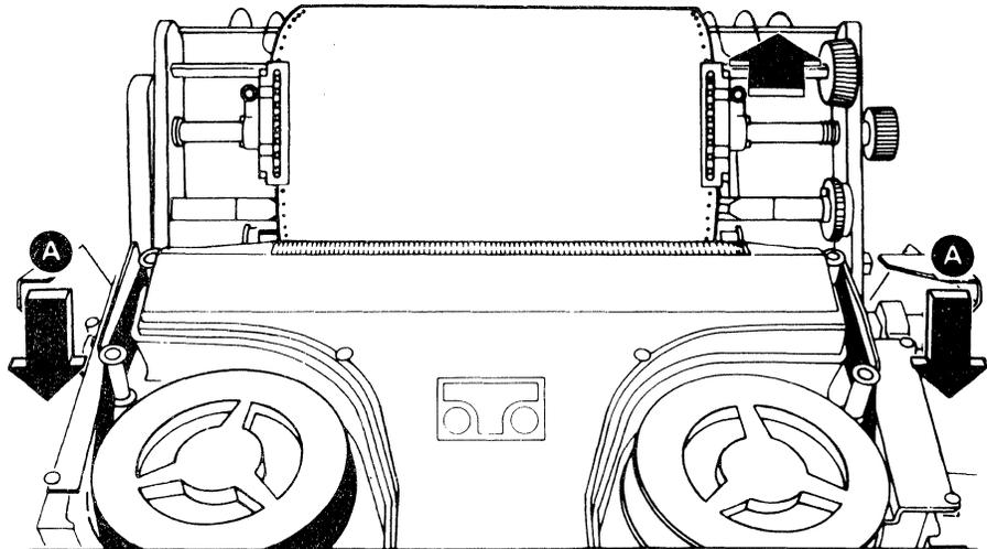
4. Pull the tension fingers toward the front of the printer.
