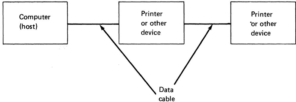
If your printer is one of several devices attached to the host, it must have its own identity (address) which the host uses when communicating with your printer. This address is set with address switches (on the customer access panel) when the printer is set up.
