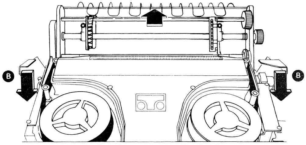
6. Pull the tension fingers toward the front of the printer.
