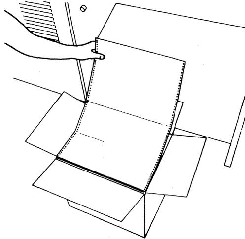
3. Place the forms into the forms compartment, and roughly align the left edge of the forms with the left tractor pins.
