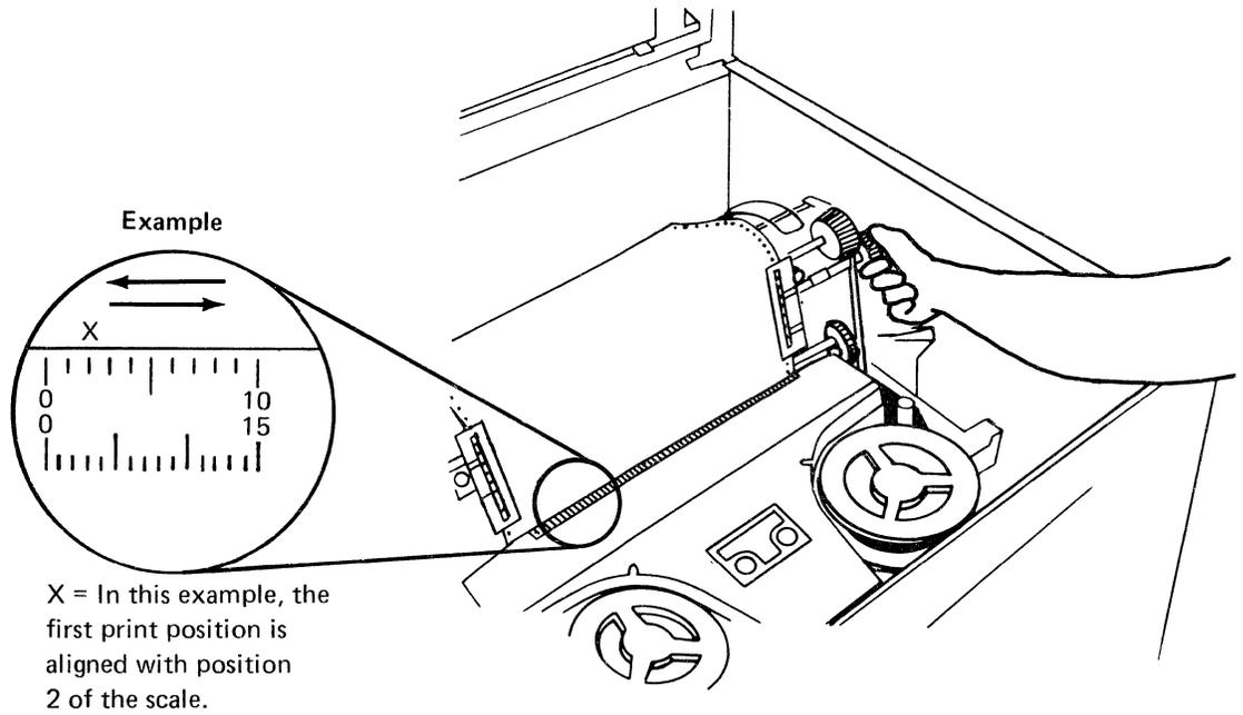
X = In this example, the first print position is aligned with position 2 of the scale.
