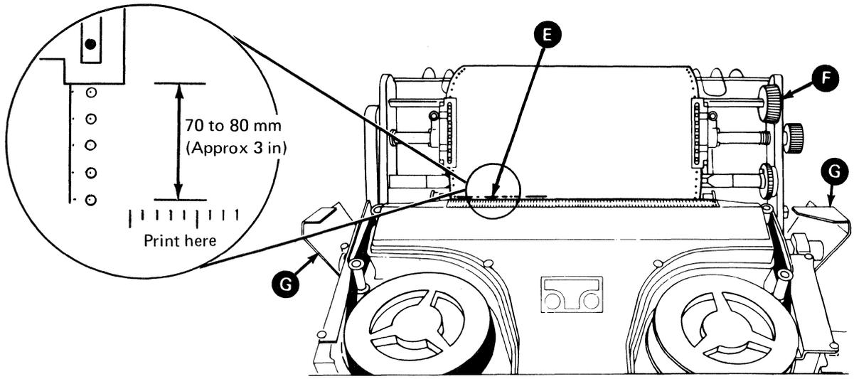
4. Push the tension fingers to the rear of the printer. Be sure the first print line is below the dark area on the tension fingers. If not, pull the tension fingers toward you and turn the vertical adjustment control to lower the first print line more. Then push the tension fingers to the rear and recheck. Repeat this procedure until the first print line is below the dark area.
