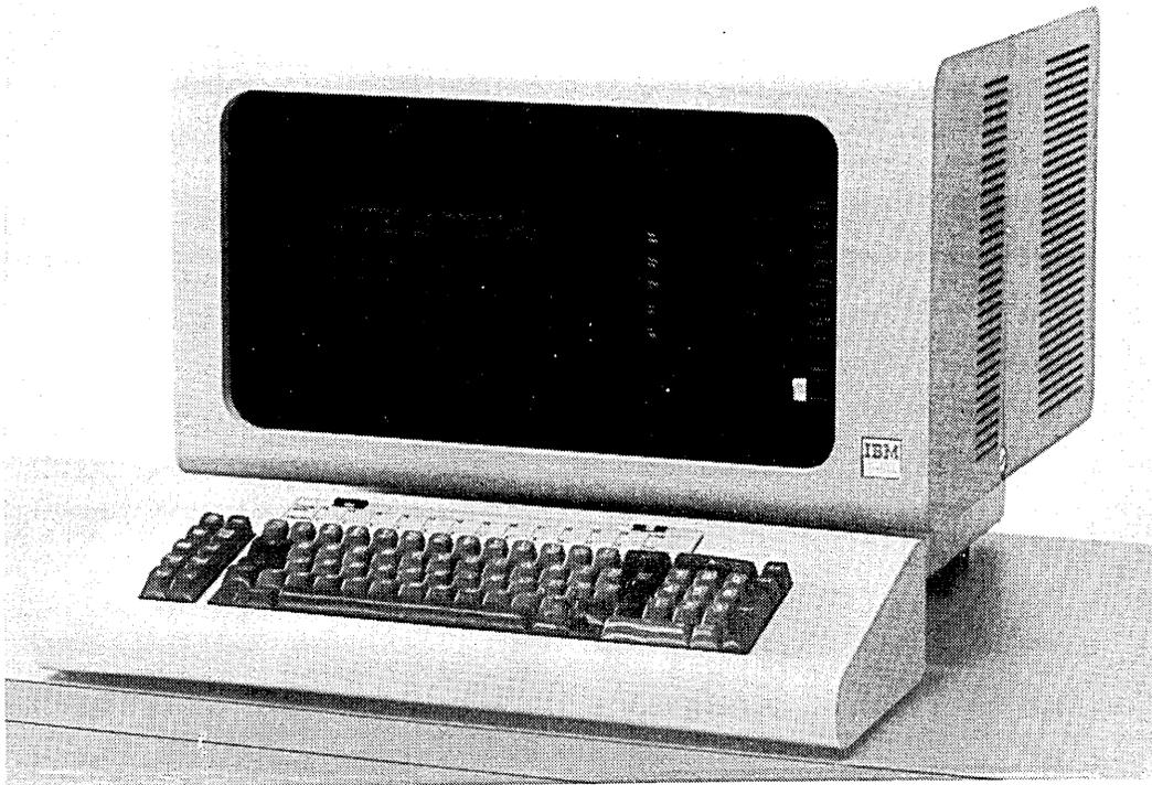
**Figure 2. IBM 5251 Model 12 Display Station**
