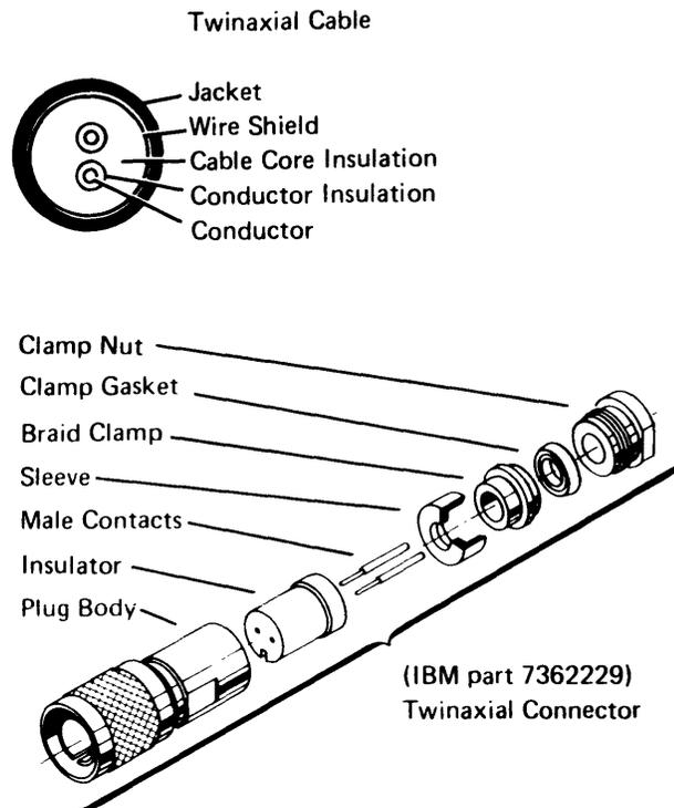
2. Cut the end of the cable sharp and square. Then slide a clamp nut and clamp gasket over the cable jacket and trim the jacket to the dimension given. Push the wire shield back to expose the inner insulation core, and cut the core and conductors to the dimension shown (16 millimeters (0.63 inch)). Slide the wire shield back over the core, and taper it to a point for ease of braid clamp assembly in step 3.
