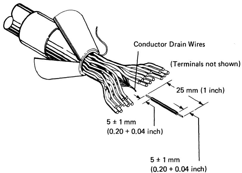
17. Use minimum heat and carefully solder the conductor drain wires and the black wire together. Ensure that the section of the black wire where the insulation has been removed remains exposed.
