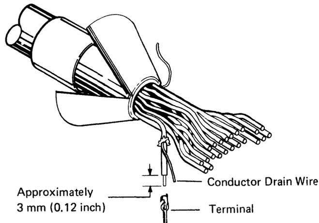
Note: Do not solder the terminal or insert it into its assigned connector hole.
