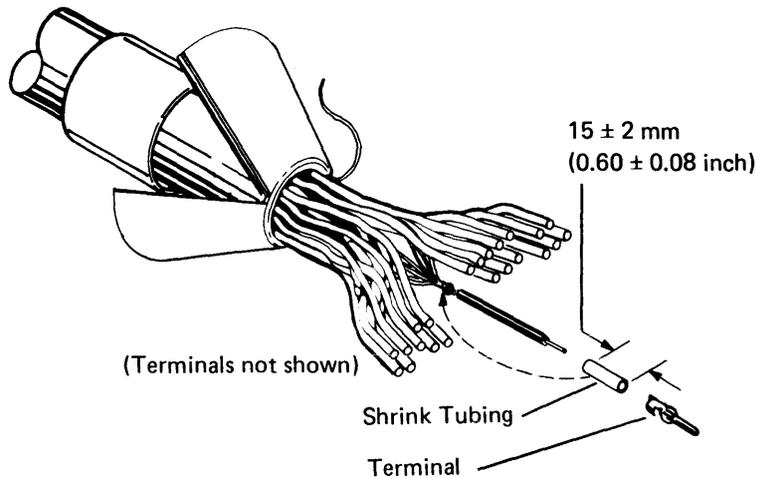
20. Use the cable chart for the cable you are assembling as a guide and insert the terminals into the assigned connector holes. Leave the spare conductor (in the 25 conductor cable) free.
