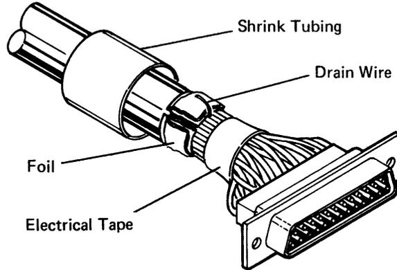
**CAUTION:** Ensure connector is correctly placed in cover as shown for a data station or a diskette drive cable.
