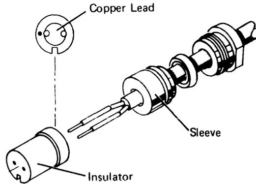
8. Insert the assembly into the connector body, aligning the polarizing slot in the insulator with the polarizing pin inside the plug body. Tighten the clamp nut with 5.7 to 6.8 newton meters (50 to 60 inch pounds) torque. (The cable and plug body should not be allowed to twist as the clamp nut is tightened.)
