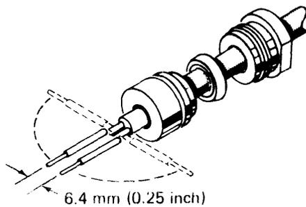
7. Slide the insulator over the contacts and the cable so that the insulator butts against the sleeve. Press all parts together. The contact on the copper lead of the cable goes into the insulator hole that has a dot next to it.
