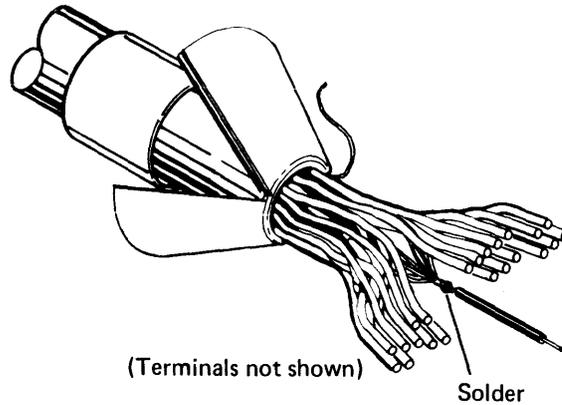
18. Apply and shrink a  $15 \pm 2$  millimeter ( $0.6 \pm 0.08$  inch) piece of shrink tubing over the soldered joint.
