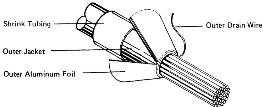
8. The exposed conductors are individually wrapped in aluminum foil and are color coded in two ways: the color of the aluminum foil wrapping and the color of the inner insulation around the conductor. The orange conductor wrapped in silver colored foil (in the 25 conductor cable) is a spare conductor; place a piece of electrical tape over the end of this conductor.
