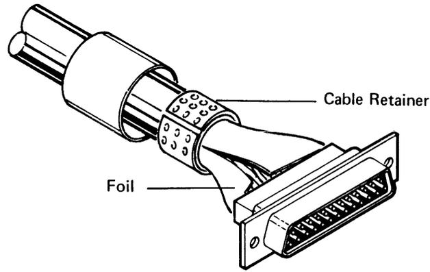
23. Fold the aluminum foil back over the retainer approximately 15 millimeter (0.6 inch) and refold forward. The silver side of the foil must be visible.
