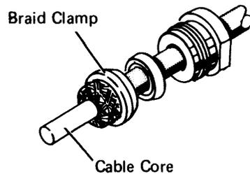
Note: Placement of braid wires over the braid clamp must be uniform to provide good rf (radio frequency) connection of the shield, and to prevent breaking the shield strands.
