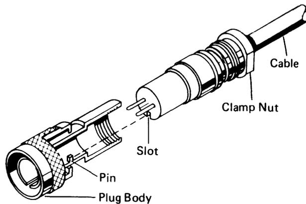
9. Check for shorts between the conductors and between each conductor and the connector body.
