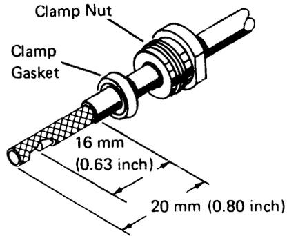
3. Slide a braid clamp over the braid so that its inner shoulder butts against the cable jacket. Then, fold the shield back over the braid clamp and trim below the shoulder.
