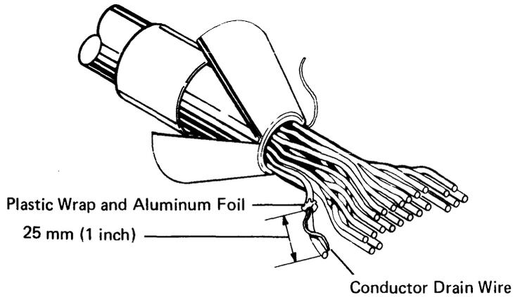
11. Bend the drain wire away from its conductor.
