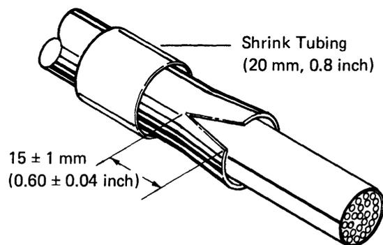
6. Fold back the outer jacket, aluminum foil, and outer drain wire that surrounds the conductors over the outer jacket.
