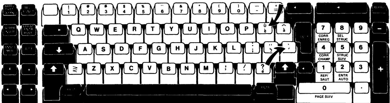
*The second method* is to press a combination of keys to obtain the desired accented character. The keyboard shows an example of a key with an accent mark on the keytop. To use this method, the following conditions must exist:
