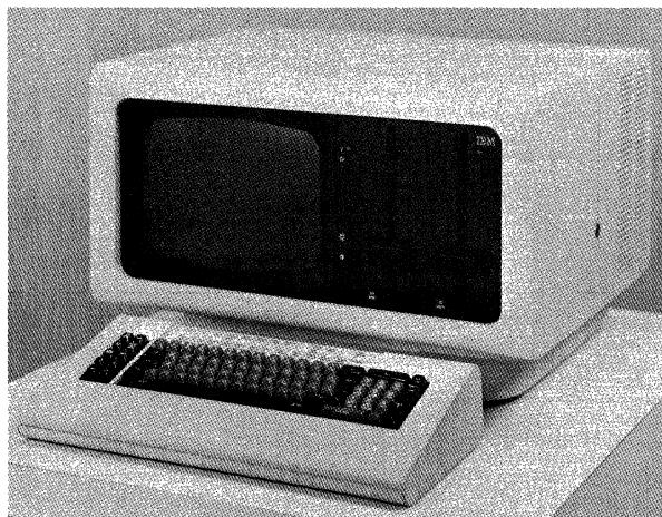
**The 5285 Programmable Data Station is a single, keyboard/display station with controller and diskette drive capability.**
