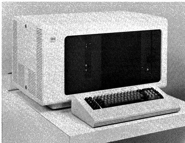
**The 5286 Dual Programmable Data Station is a dual keyboard/display station with controller and diskette drive capability.**
