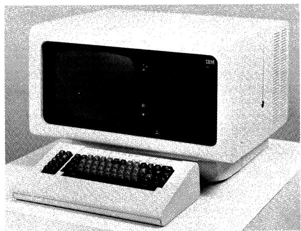
**The 5281 Data Station** is a single, auxiliary keyboard/ display
