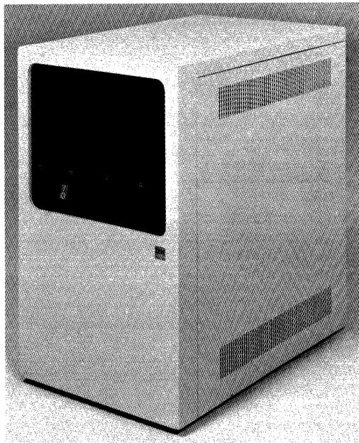
**The 5288 Programmable Control Unit** is a compact, floor-standing controller that can accommodate multiple keyboard/displays.
