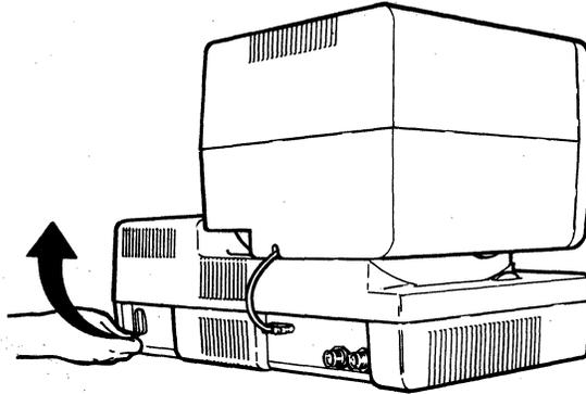
10. Plug the end of the power cord (as shown) into the lower unit.
