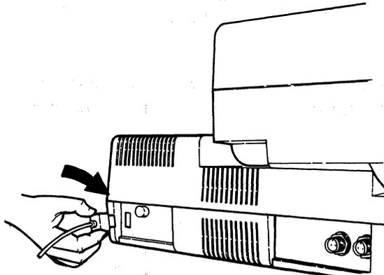
11. Plug the other end of the power cord into a grounded electrical outlet.
