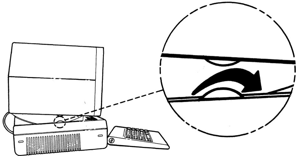
13. Set the Power switch to On. Wait a few seconds; you should hear the alarm<sup>6</sup>, which means that the lower unit is working properly.
