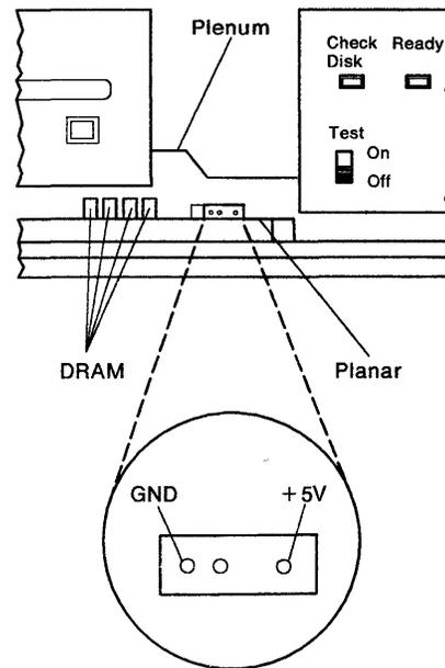
Figure 4-3. Test Connector Location
