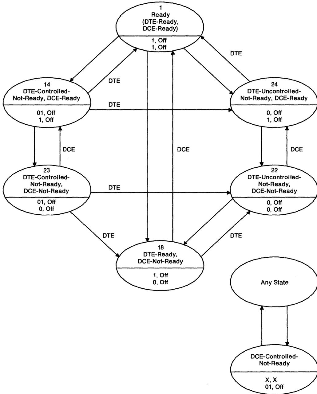
**Note:** The DCE and DTE (5394) must signal each state 24 bit-times or until the DCE or DTE indicates that the state has been recognized by changing states. The DTE (5394) must not change states as a result of the DCE changing state until the DCE-signaled state has existed for at least 16 bit-times.
