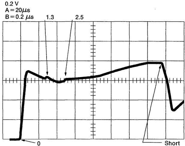
Figure 3-65. Shorted Cable (Higher Vertical Gain)
