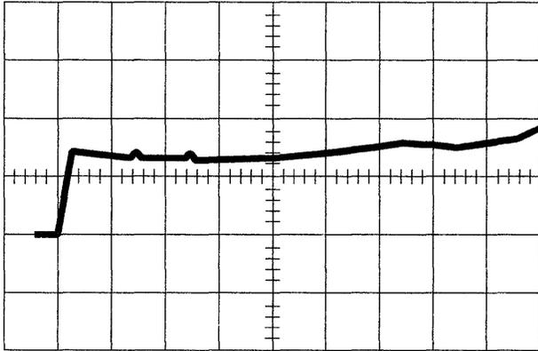
Figure 3-63. Normal Cable (Properly Terminated)
