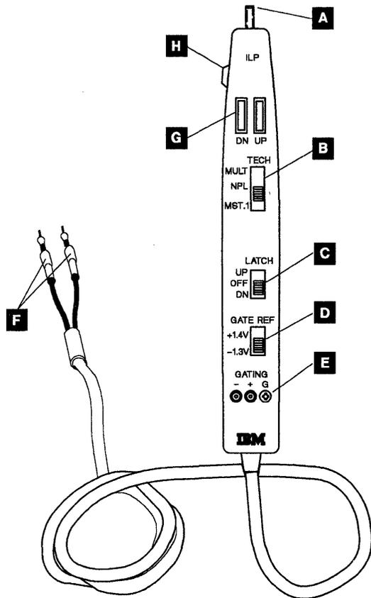
Figure 4-2. Integrated Logic Probe
