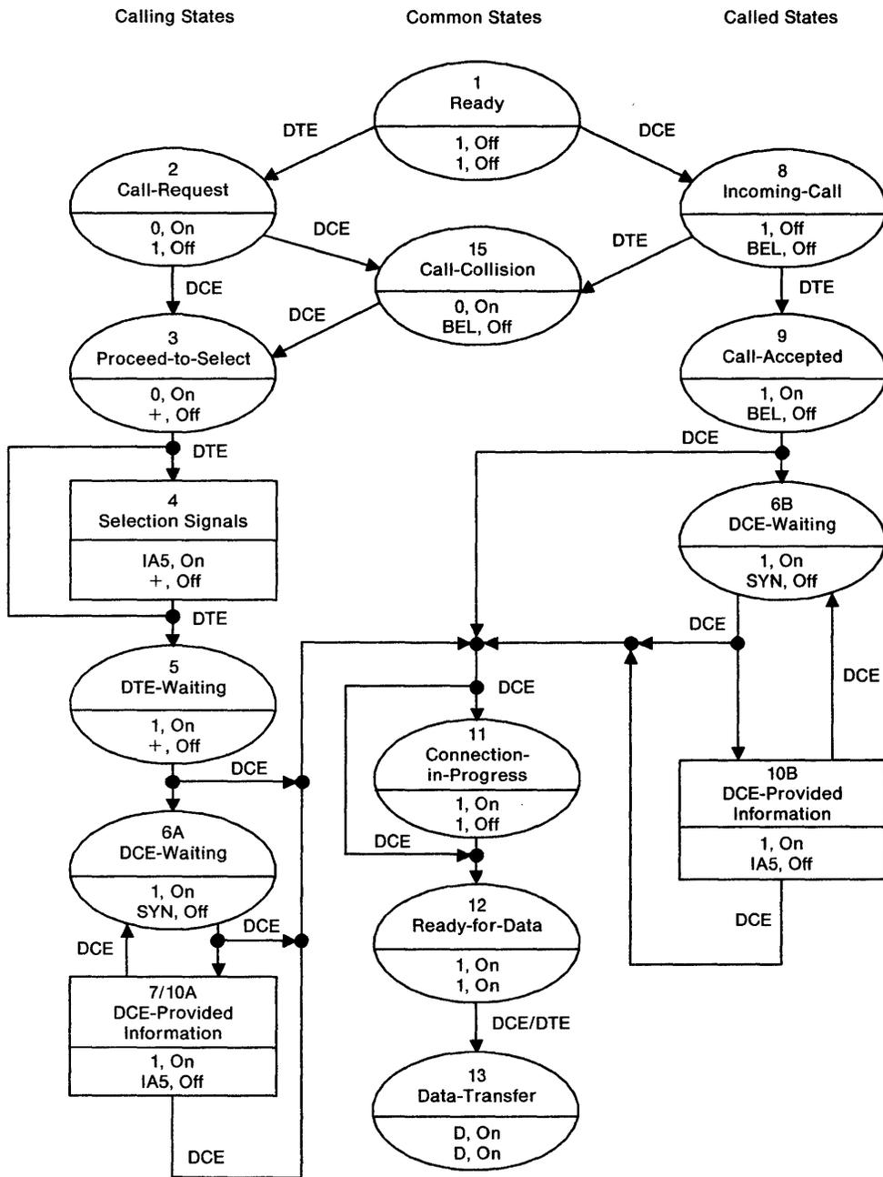
Figure 5-21. Call Establishment Phase and Data Transfer Phase Interface State Diagram: Circuit-Switched Operation
