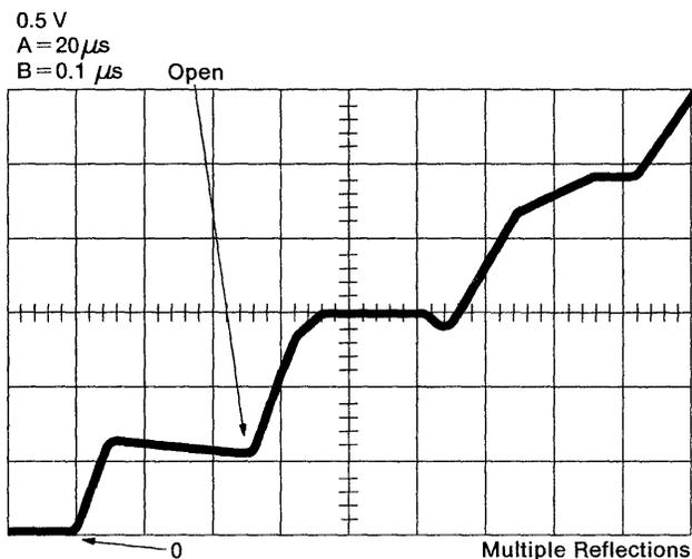
Figure 3-67. Open Cable (Wrong Oscilloscope Setting)
