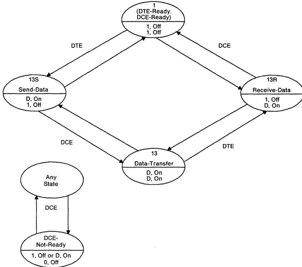
Figure 5-19. Data Transfer Phase Interface State Diagram. X.21 Nonswitched Public Data Network or X.25 Packet-Switched Network Operation with X.21 Electrical (X.24/X.27) Interface
