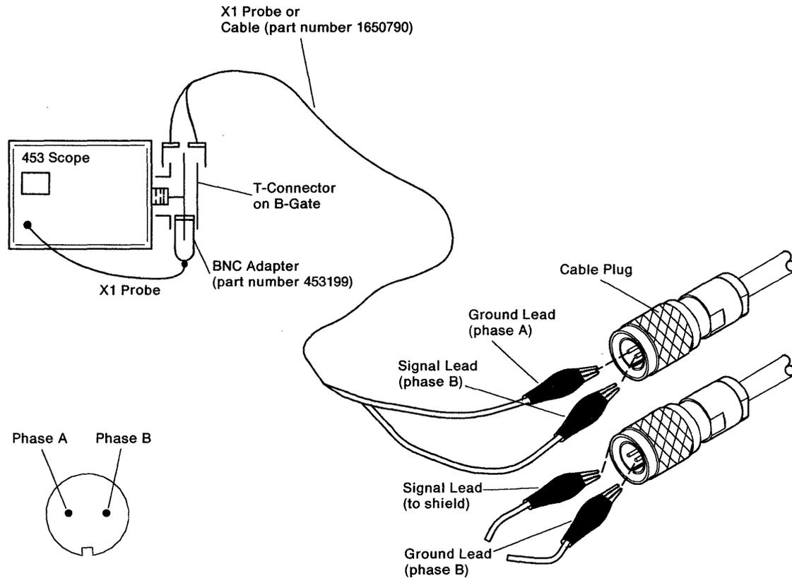
Figure 3-58. Oscilloscope Setup
