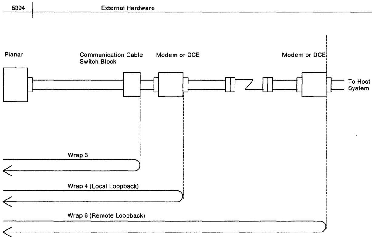
Figure 3-37. Communication Wrap Tests
