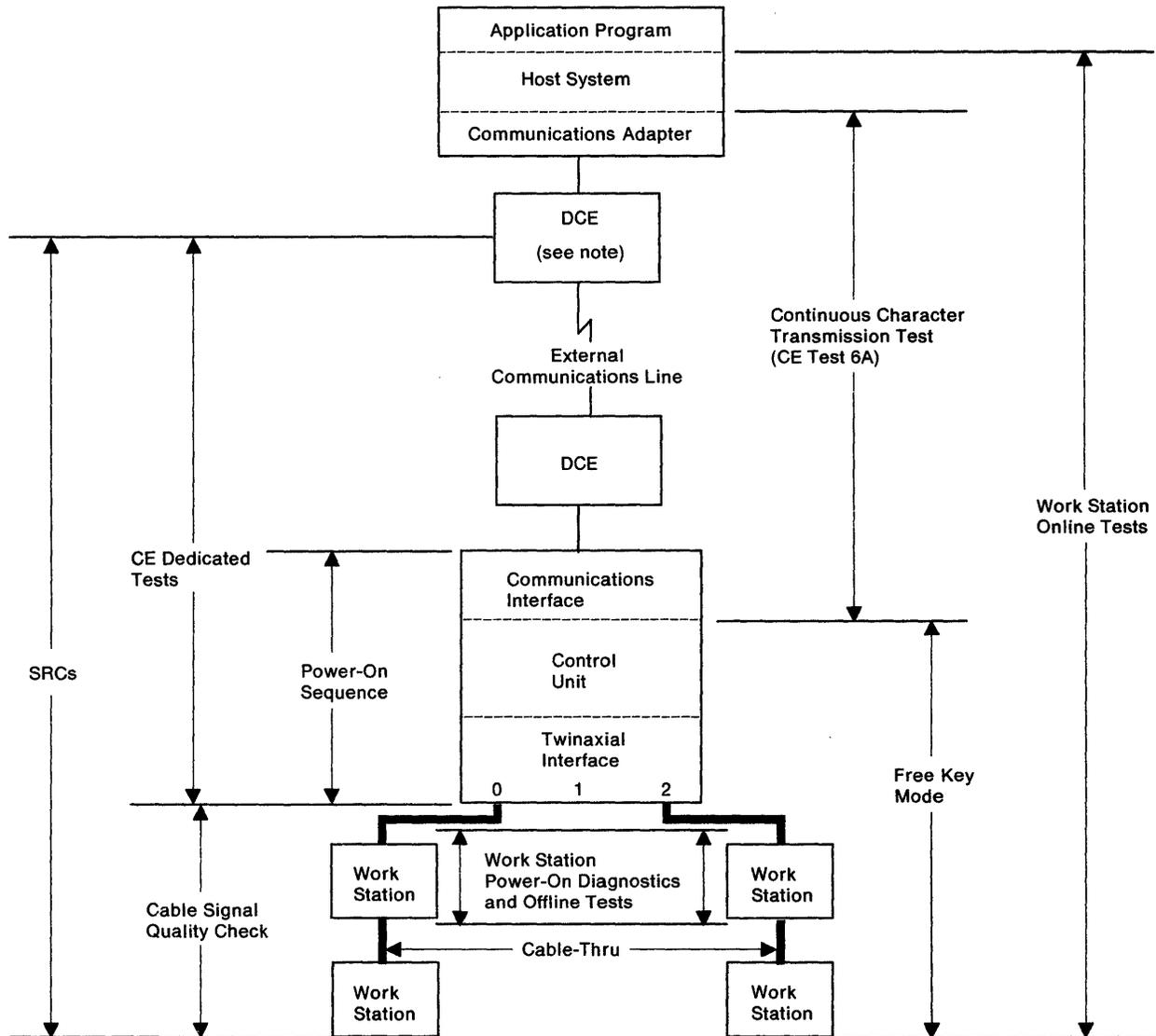
Note: The host system DCE may be an integrated modem or DCE, an external modem or DCE, or an external digital DCE.
