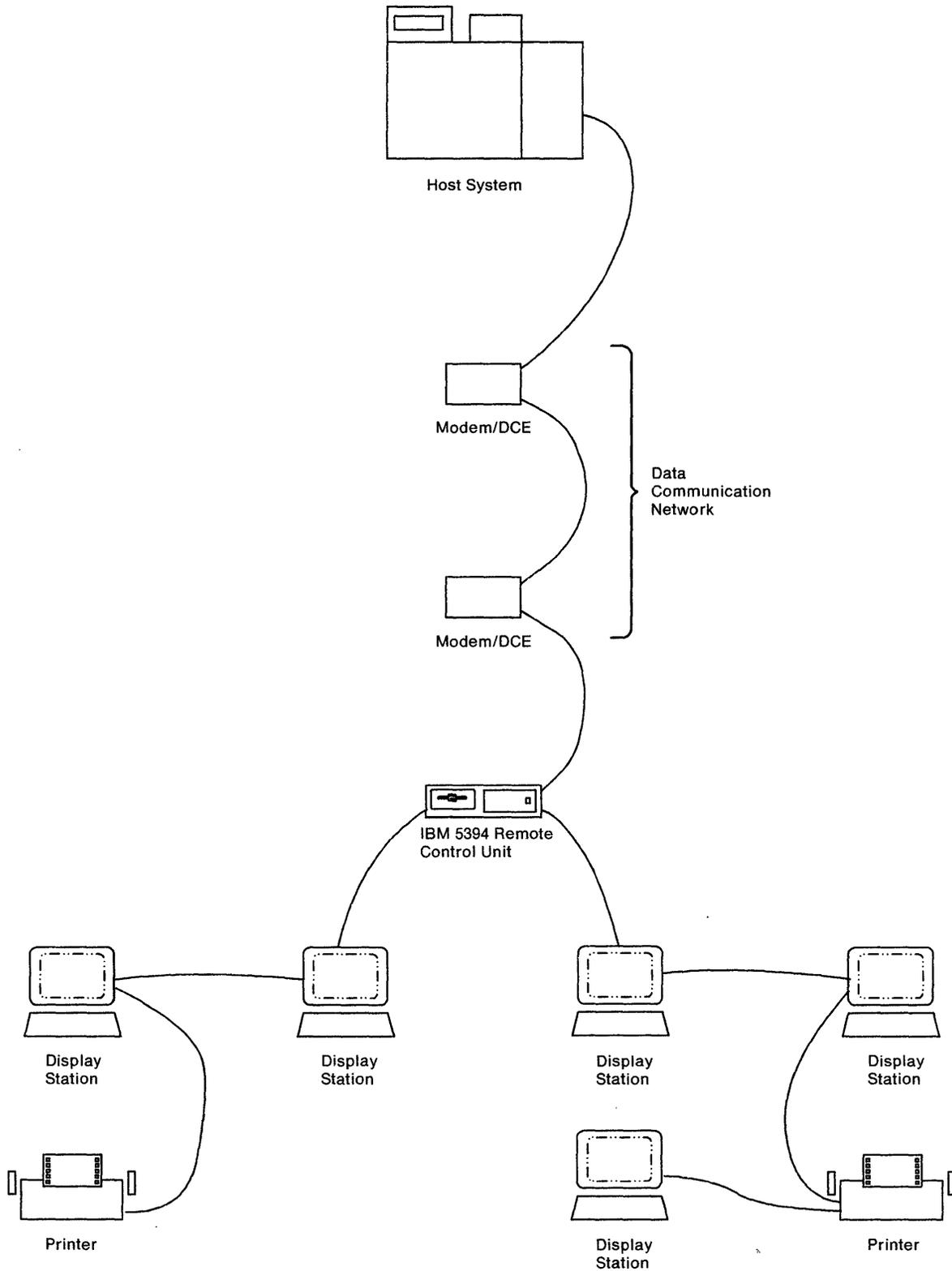
Figure 1-2. Sample Data Communication System Using the 5394
