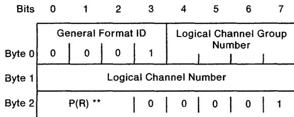
Figure 5-11. RR Packet Format in Modulo 8
