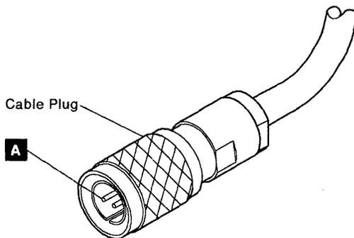
Figure 3-70. Twinaxial Cable Plug
