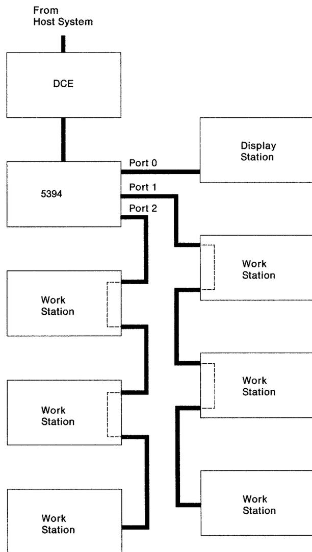
Figure 5-1. Typical 3-Port Configuration
