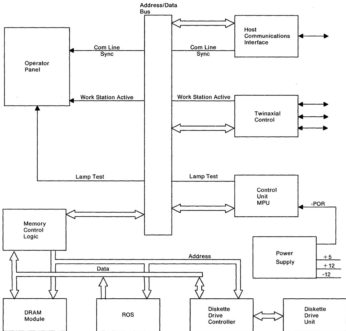
Figure 5-2. 5394 Block Diagram
