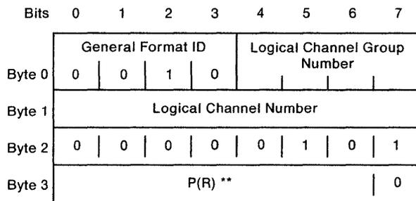
\*\* P(R) = Packet receive sequence number used to provide packet-level acknowledgment.
