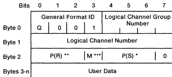
Figure 5-15. Data Packet Format in Modulo 8
