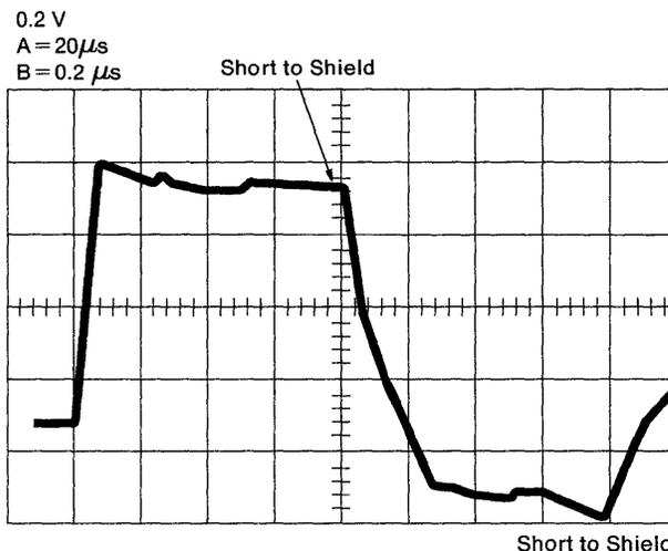
Figure 3-69. Short to Shield (Oscilloscope Leads Swapped)
