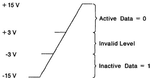
Figure 3-23. EIA 232D Signal Levels
