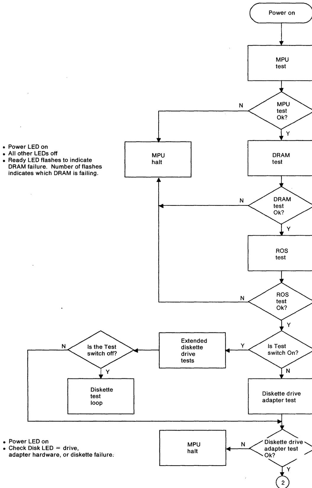
Figure 3-33 (Part 1 of 2). Power-On Sequence Flowchart
