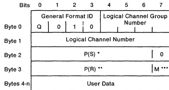
\* P(S) = Packet transmitted sequence number used to provide packet-level acknowledgment.
