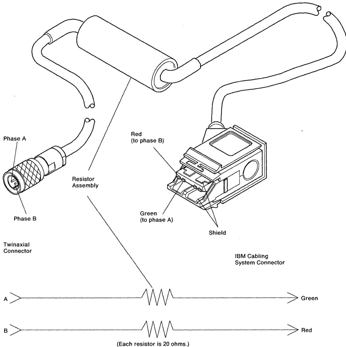
Figure 3-72. Impedance Matching Device
