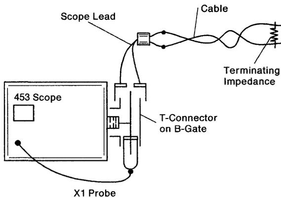
Figure 3-54. Oscilloscope Setup for Testing Cables
