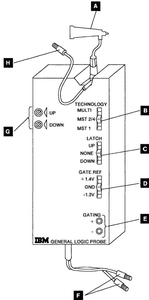
Figure 4-1. General Logic Probe
