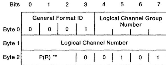
Figure 5-13. RNR Packet Format in Modulo 8
