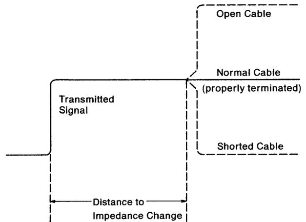
Figure 3-55. Oscilloscope Trace for Open or Shorted Cable
