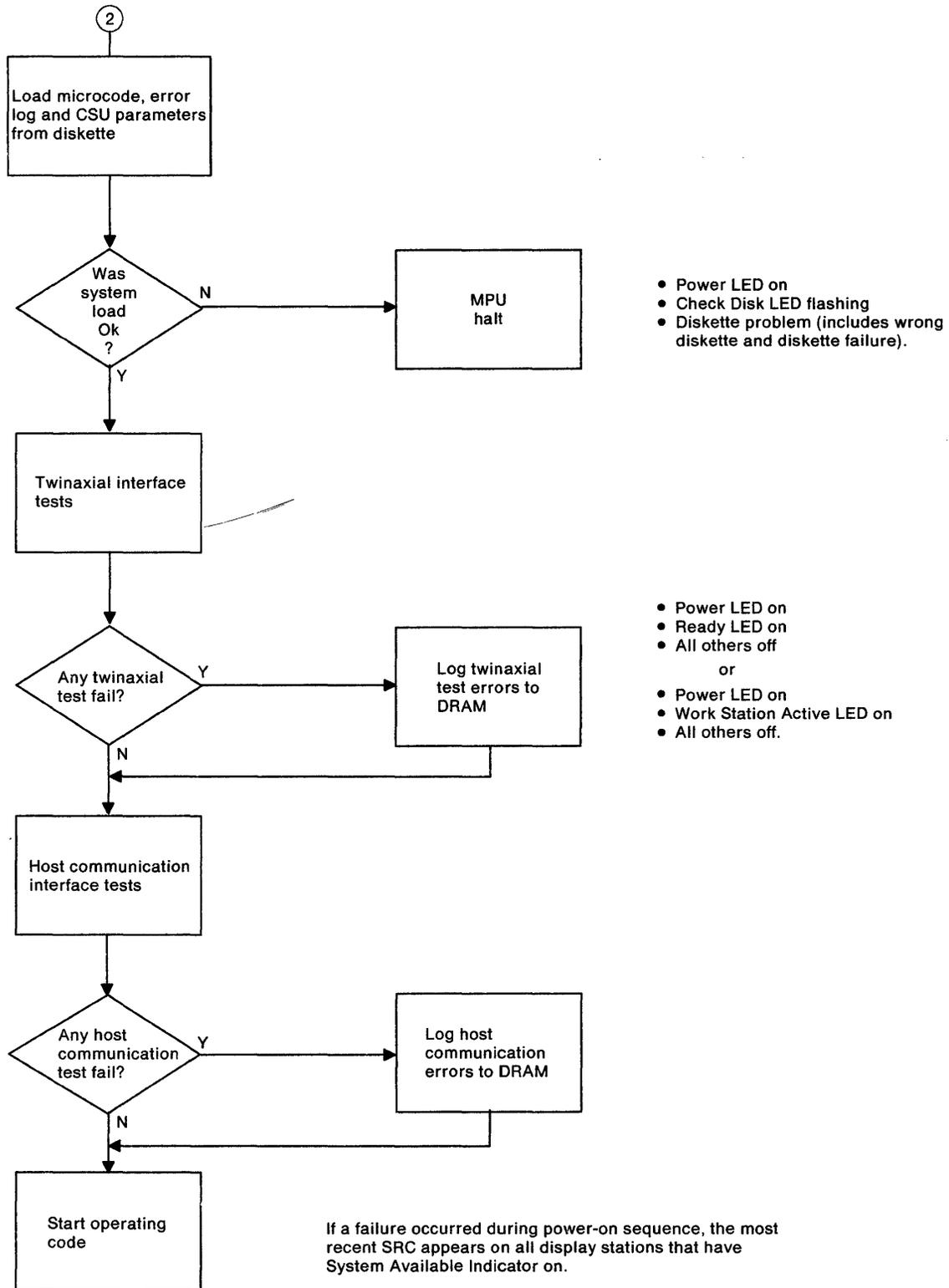
Figure 3-33 (Part 2 of 2). Power-On Sequence Flowchart
