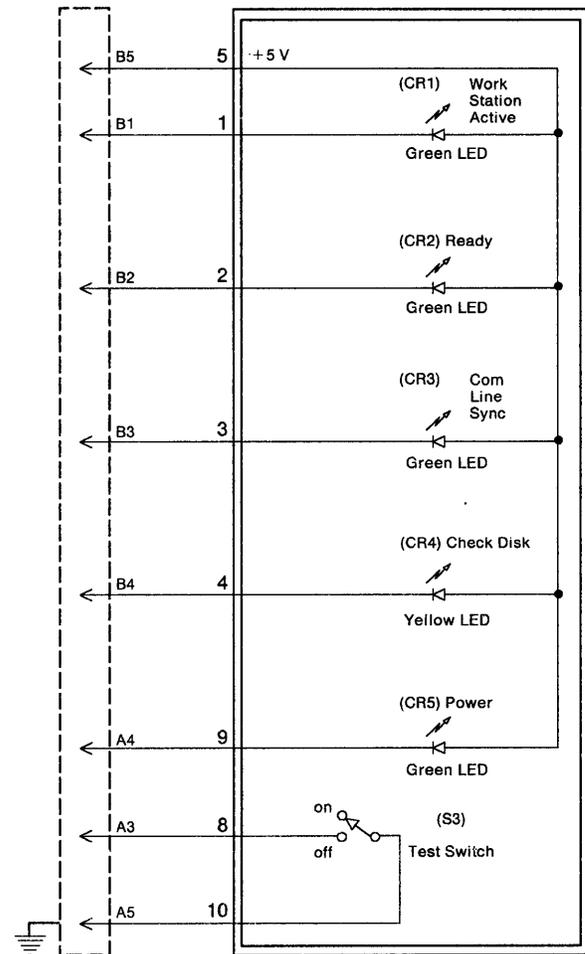
Figure 3-22. Operator Panel Wiring
