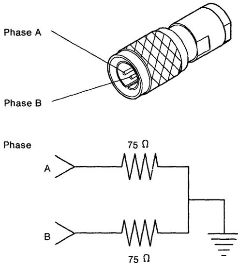
Figure 3-75. Twinaxial Terminator Assembly
