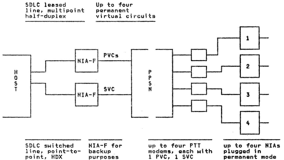
Figure 3. Typical Configuration to use SNBU with two frontal NIAs
