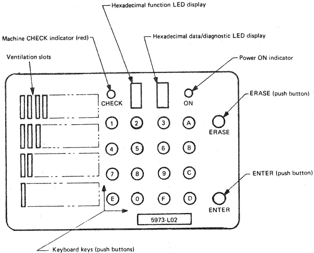
Figure 5. Details of the Operator Panel and of the Back Panel
