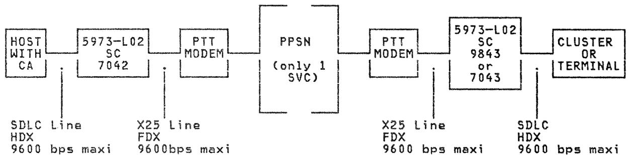
Figure 1. Typical Switched Configuration
