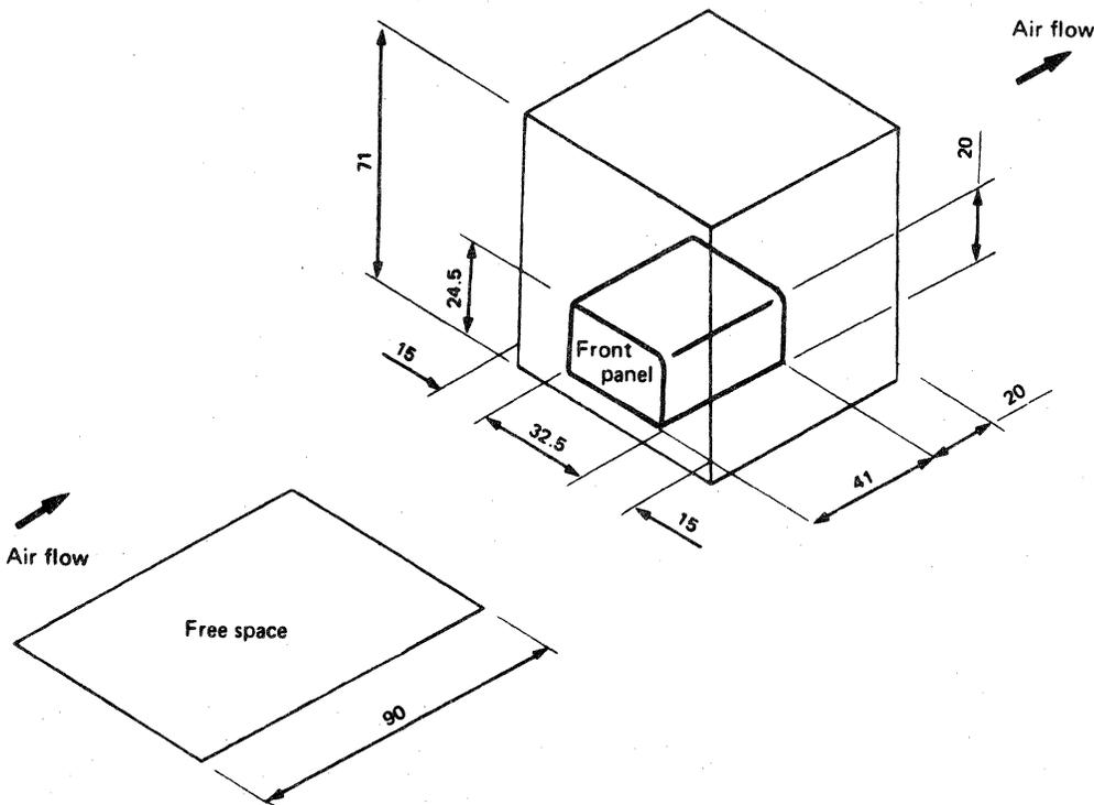
Figure 7. IBM 5973-L02 Measurements and Service Clearances
