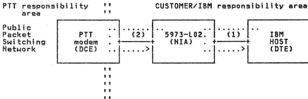
Figure 6. Simplified Configuration and NIA Tests
