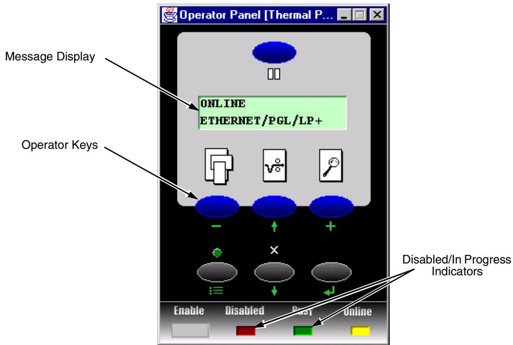
Figure 38. 4400 Series Thermal Printer Operator Panel
