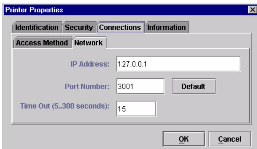
**Figure 4. Printer Properties: Connections – Network Tab**
