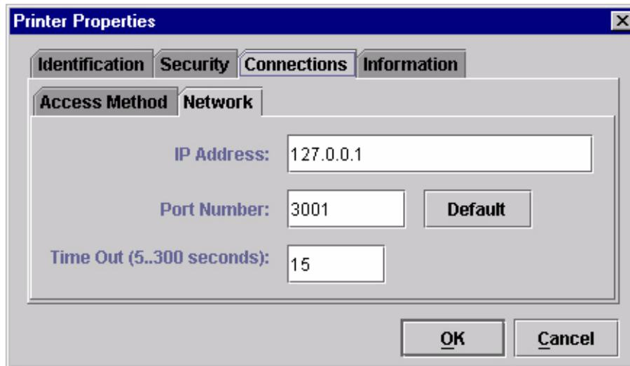
**Figure 31. Printer Properties: Connections – Network Tab**
