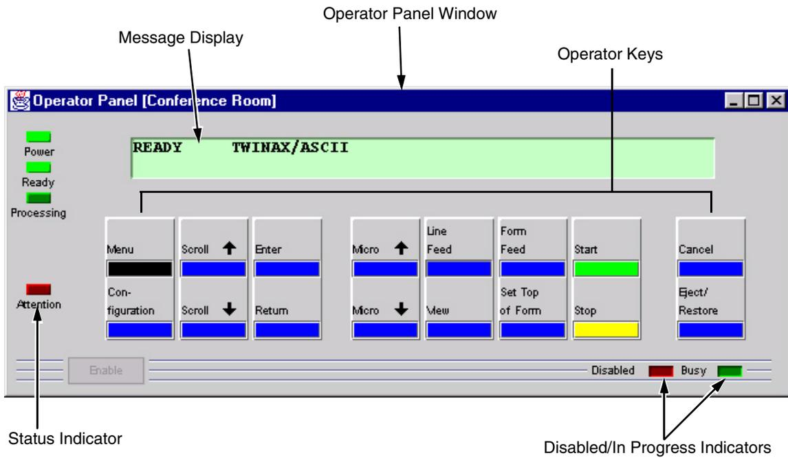
Figure 37. 6400 Series Line Matrix Printer Operator Panel
