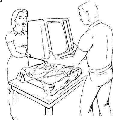
STEP 7. Place the Display on top of the Electronics Module.
