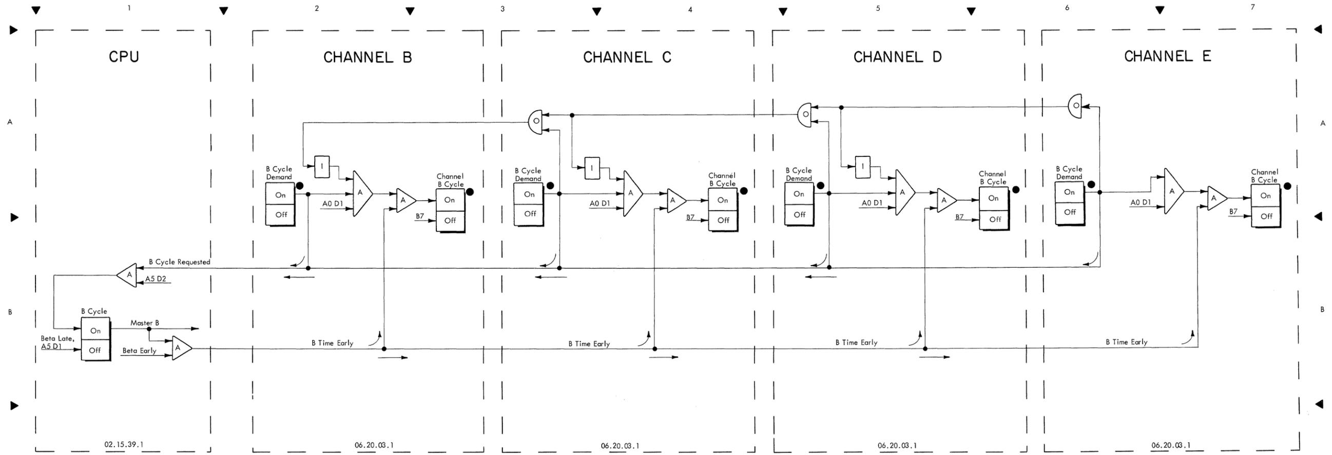
Note: Any channel's B Cycle Demand trigger on requests a B cycle of CPU. The next CPU cycle becomes the B cycle, the B cycle being granted to the requesting channel.
