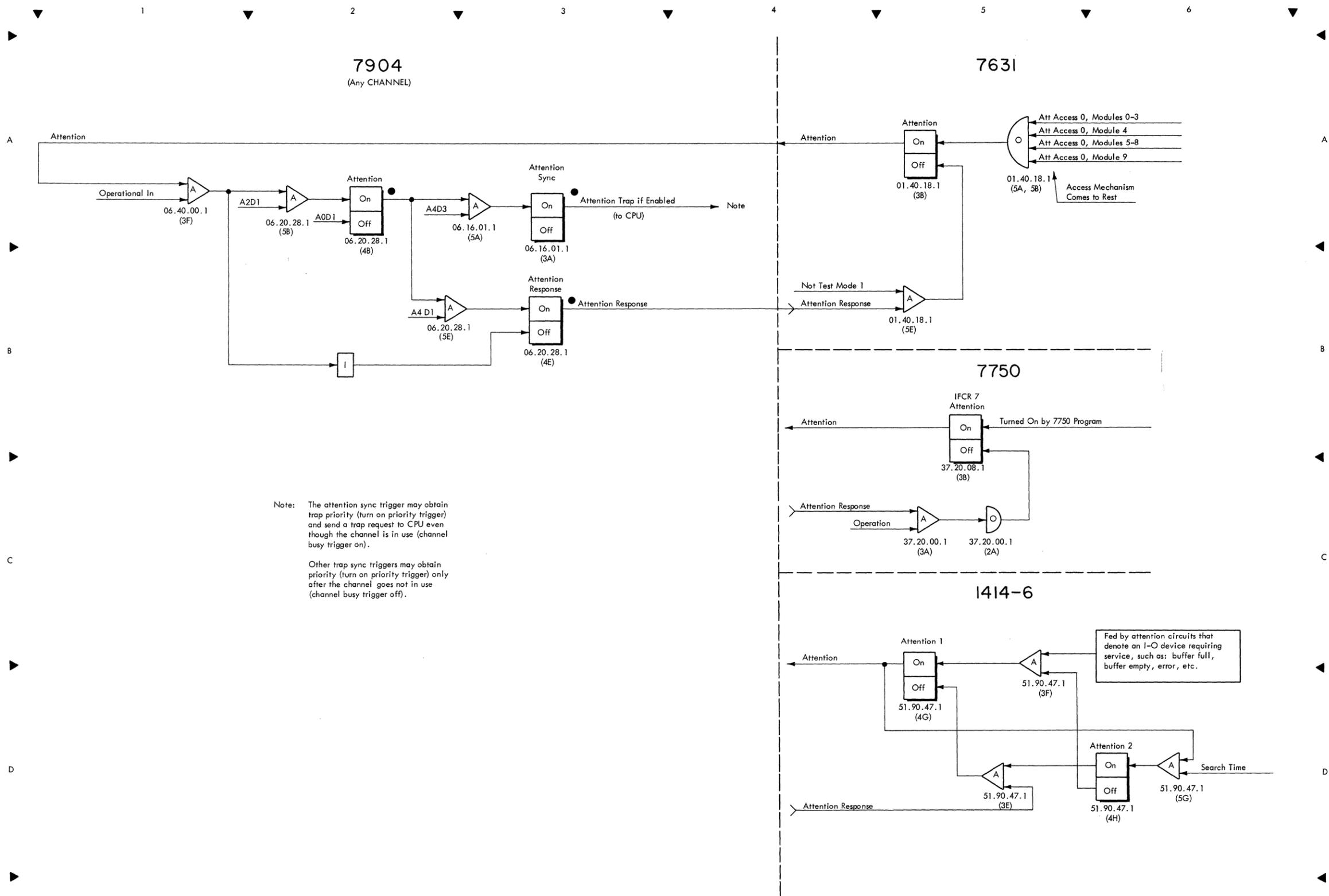
Note: The attention sync trigger may obtain trap priority (turn on priority trigger) and send a trap request to CPU even though the channel is in use (channel busy trigger on).
