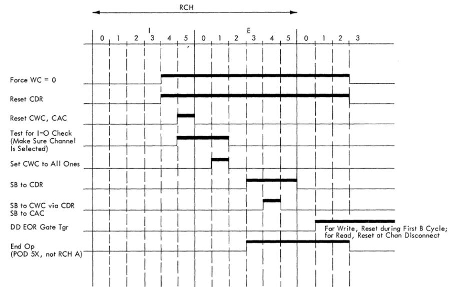
Note: The DD EOR Gate Tgr determines when the word counter is tested for a WC zero condition.
