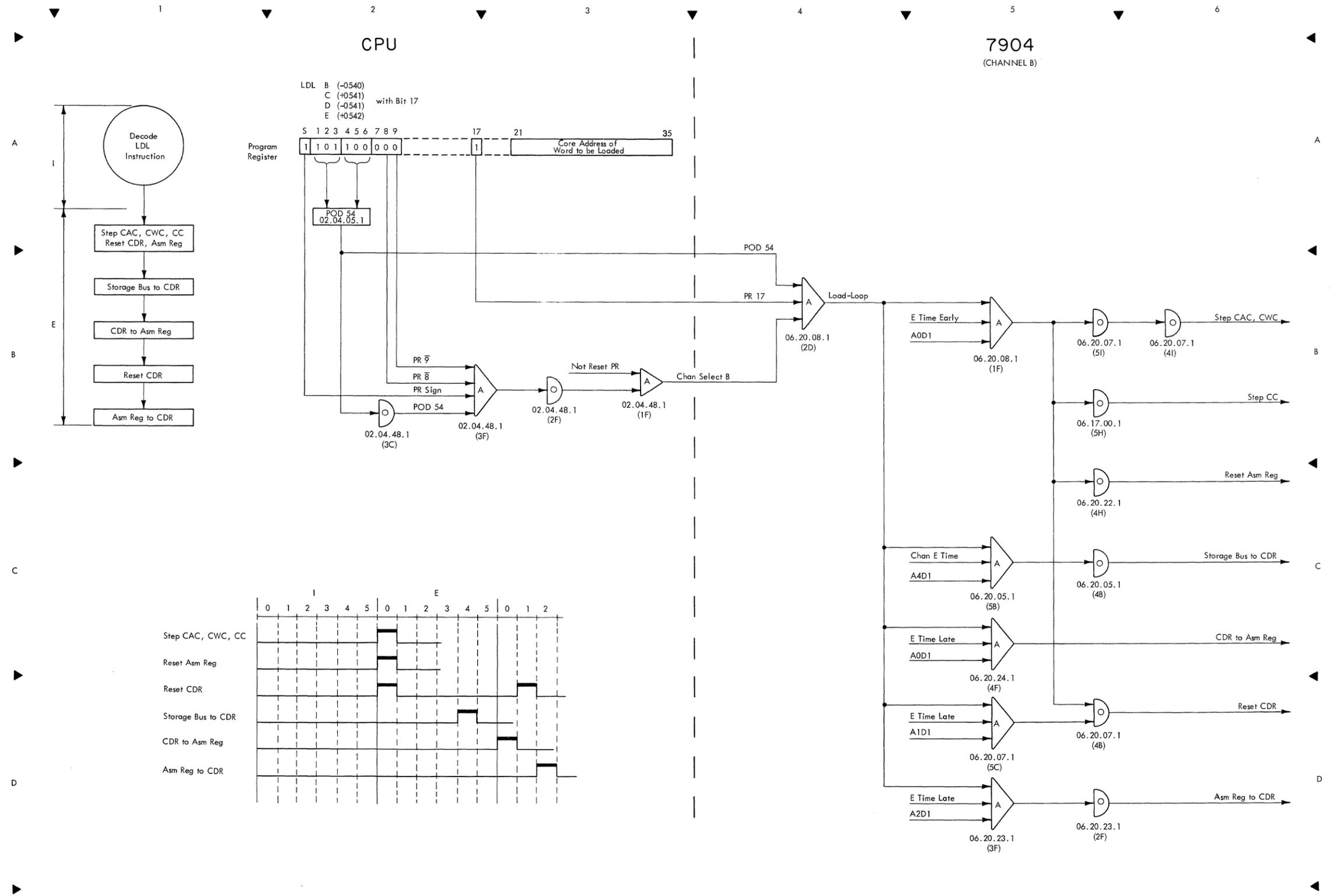
FIGURE 71. LOAD DATA REGISTER AND LOOP (LDL)
