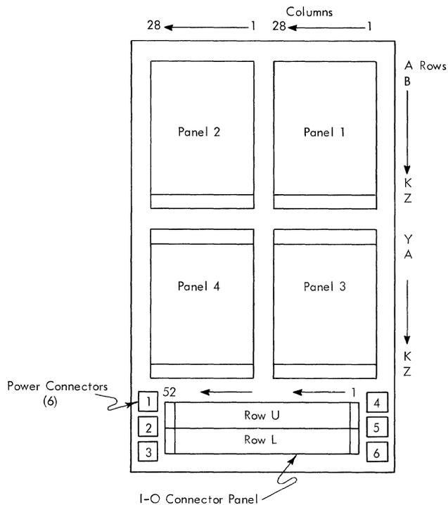
FIGURE 1. FRAME 02 - FRONT LAYOUT (WIRING SIDE)
