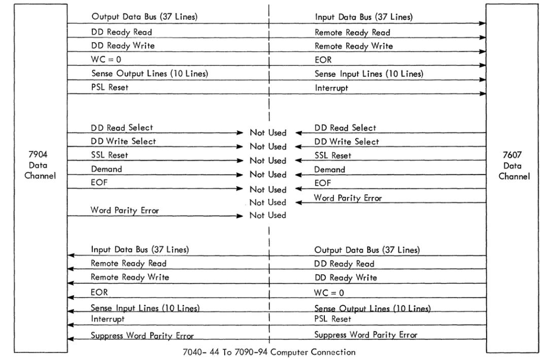
FIGURE 58. DIRECT DATA SIGNAL LINES FOR 7040-44 AND 7090-94
