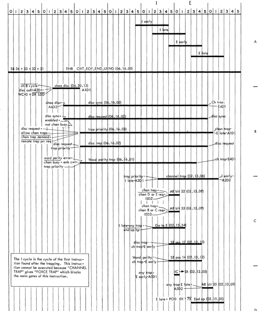
FIGURE 23. DISCONNECT TRAP TIMING
