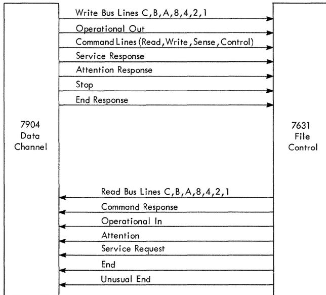
FIGURE 42. SIMPLEX INTERFACE SIGNAL LINES
