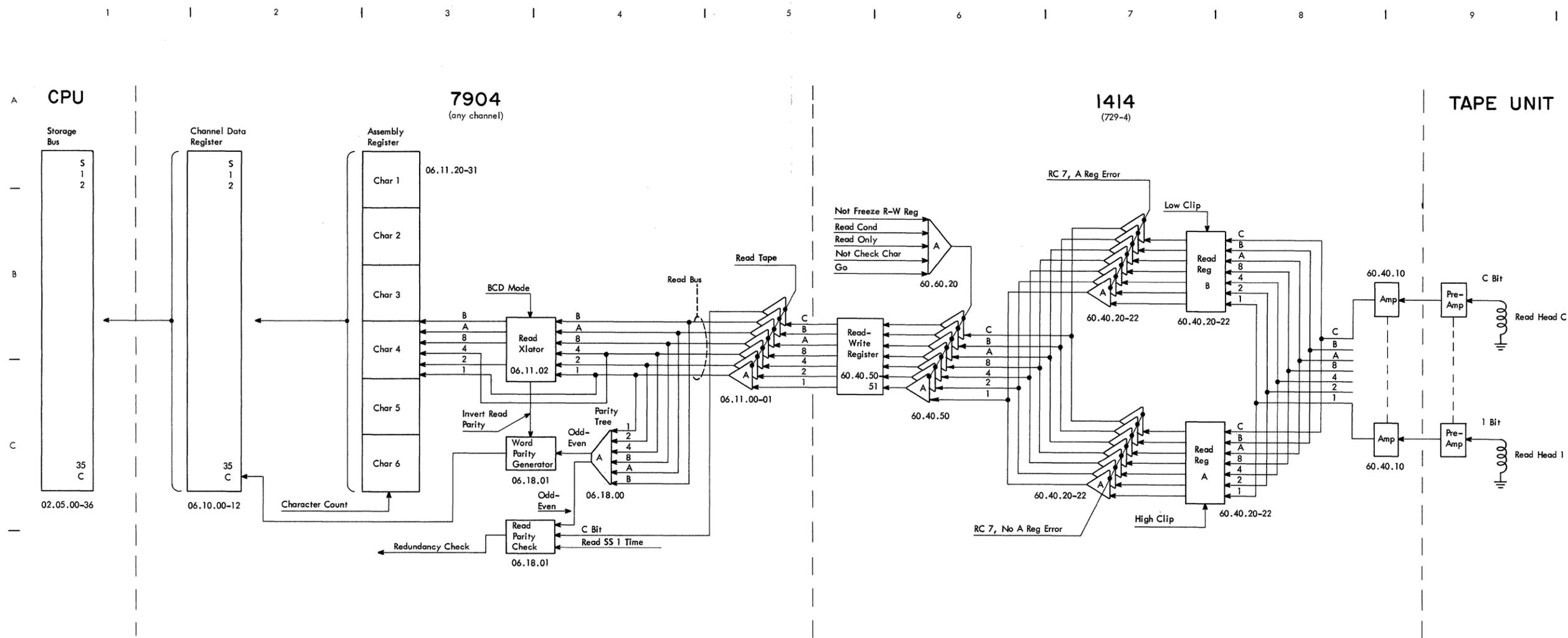
FIGURE 31. DATA FLOW, READ TAPE OPERATION
