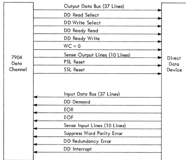
FIGURE 57. DIRECT DATA CONNECTION SIGNAL LINES
