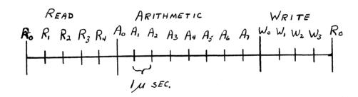
Read time is used to take information out of memory (Read memory). Arithmetic time is used to operate on the character taken from memory. Write time is used to write information back into memory.
