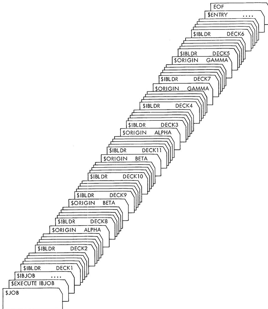
Figure 13. Sample Control Card Deck
