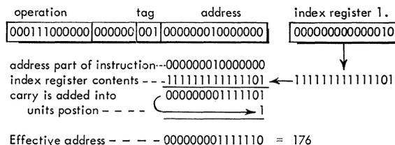
Figure 33. Index-Register Arithmetic, Subtracting
