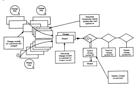
In the diagram above, the first change record matches the first master file record. The change record selects priority packet 1 where the first change to the master file record is made.
