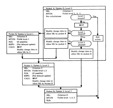
In the above example, the program does not actually transfer directly from one priority packet to another; exit is made from each priority packet to point 1.0 as shown in the object program flow charts in the appendix. Note that in packet A, when level 3 is not present, exit from the packet is made directly from the pre-calculation by use of the IGNORE macro-instruction.
