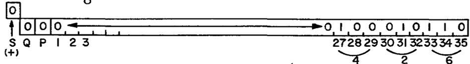
Then the add (or subtract) instruction is given, addressing the storage position where the other number is located. This will add (or subtract) into the number already stored in the AC. The result then may be moved from the AC to a specific location in storage, and further processing may continue.
