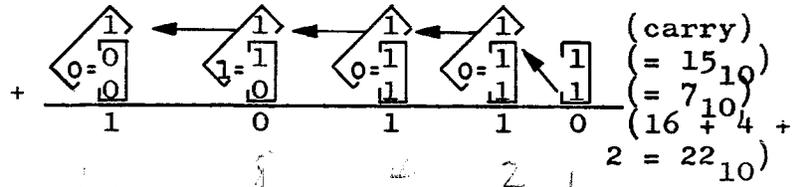
In the "ones" column, Rule 3 applies. In the "twos" column, Rule 3 applies again, but we must further add the "carry", so the result is 1 with a "carry". The same thing happens in the "fours" column. In the "eights" column, Rule 2 applies, but again we must add the "carry", so now Rule 3 takes over and we end up with zero and a "carry". In the "sixteens" column, Rule 1 applies, then add the "carry", which winds it up with a 1.
