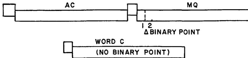
The Binary point will be between positions 1 and 2 of the MQ. As in any problem in multiplication, the product will have as many Binary points as the sum of the digits to the right of the positions in the two numbers being multiplied ( $18 + 18 = 36$ ). Since the product fills the entire AC and MQ, the 36 rightmost positions will be beyond the Binary point. Therefore, there will be no Binary point in the AC or in Word C.
