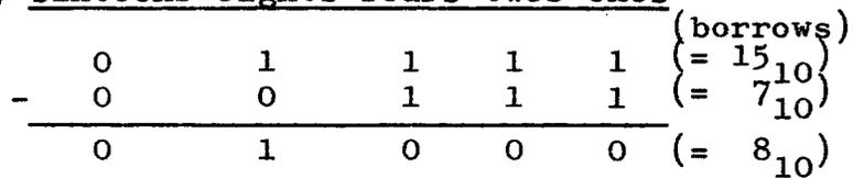
Applying the rules above, in the "ones" column, Rule 2 applies. Also in the "twos" and "fours" columns. In the "eights" column, Rule 3 applies. In the "sixteens" column, Rule 1 applies.
