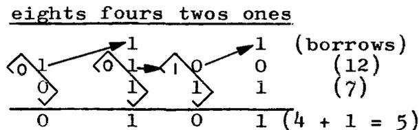
In the "ones" column, Rule 4 applies, but since there is no "1" to borrow in the "twos" column, we must get it from the "fours" column, changing the 1 to a 0 in the "fours" and the 0 to a 1 in the "twos". In the "twos" column, Rule 2 applies. In the "fours" column, 0-1 causes a "borrow" from the "eights" column, leaving it a 0, which results in 0 for the final subtraction.
