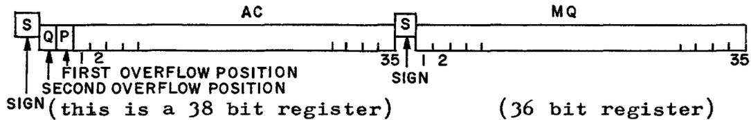
These two registers may be considered to be working together, with the MQ as the right-most extension of the AC.
