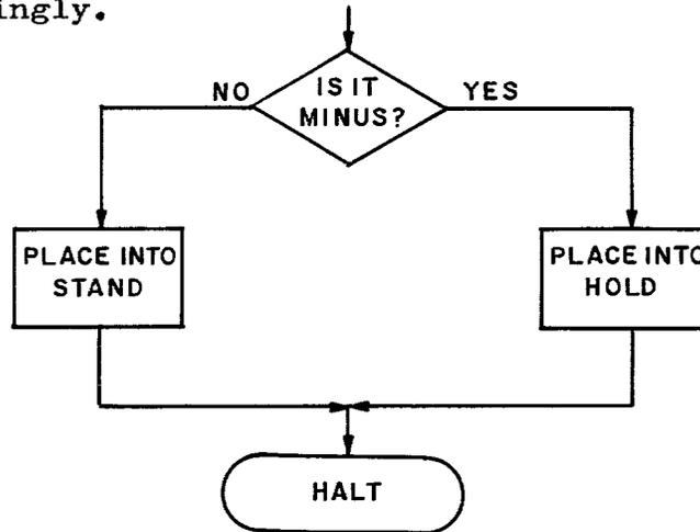
The question "Is it minus?" must be asked three times (once for each of the three possibilities in the first half of the flow chart). Once the flow chart has been developed, the process of coding becomes fairly routine. Of course, it is necessary to be familiar with the instructions and what each one can do, to make the job of coding easier.
