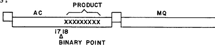
In this case, since all the action was in the AC, the ARS instruction could have been used equally effectively. The only difference is that with the LRS, the sign of the MQ is made to agree with the sign of the AC.
