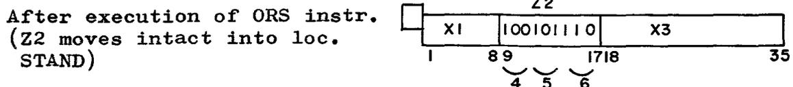
The zeros in loc. STAND are compared to  $456_8$  in the AC. Using the rules for OR, the  $456_8$  in the AC moves intact into loc. STAND and the job is finished.
