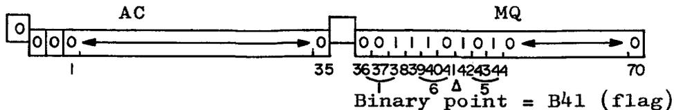
The quotient will be in the MQ and the remainder in the AC, so after divide has been accomplished, the MQ must again be considered as a 35 bit register.
