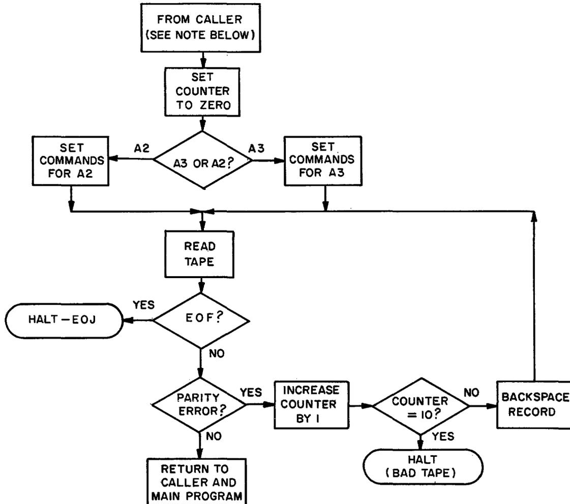
Note: The instruction in the Main Program that leads to a subroutine is named the caller. When the subroutine is finished, control is returned to the Main Program. Each time the caller is encountered in the Program, the subroutine is entered (see page 133 for subroutine linkage).
