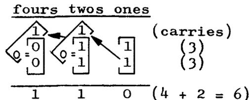
In the "ones" column, Rule 3 applies. In the "twos" column, two steps must be taken; first,  $1 + 1 = 0$  with a carry; second, the 0 (resulting from the first step) + 1 (from the previous carry) = 1. In the "fours" column, two steps must be taken; first,  $0 + 0 = 0$ , second, this 0 + 1 (from the previous carry) = 1. Each time there is a "carry", the second step must be taken.
