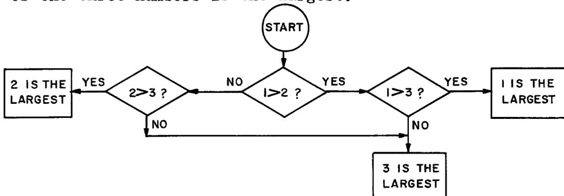
When the largest number has been located, we must discover whether it is plus or minus, then place into HOLD or STAND accordingly.
