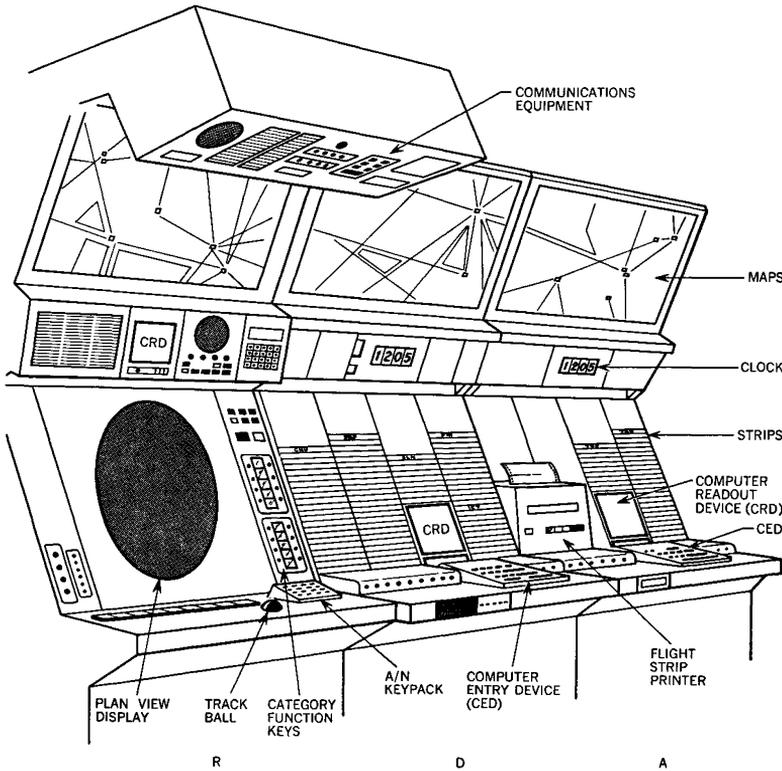
keys, the alphanumeric keypack, and the track ball. The category-function keys allow rapid input of frequently used data into the 9020 system: depression of one button defines a class of actions, and depression of a second button indicates a particular action within the class. The R controller enters supporting data with the alphanumeric keypack. The track ball permits the controller to indicate a point on his plan-view display.
