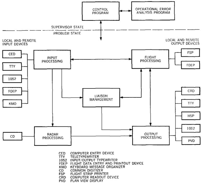
Teletype equipment at flight service stations, airline offices, and military operation offices may communicate with the 9020 system. High-speed circuits are used to pass data to and from adjacent computer-equipped centers, to and from flight-data entry and printing devices at airport control towers and Terminal Radar Approach Control Facilities (TRACON's), and from the special devices that provide digital radar data from each radar site.
