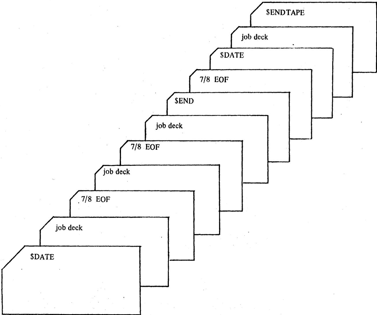
FIGURE 6-1. SAMPLE MACHINE RUN CARD DECK
