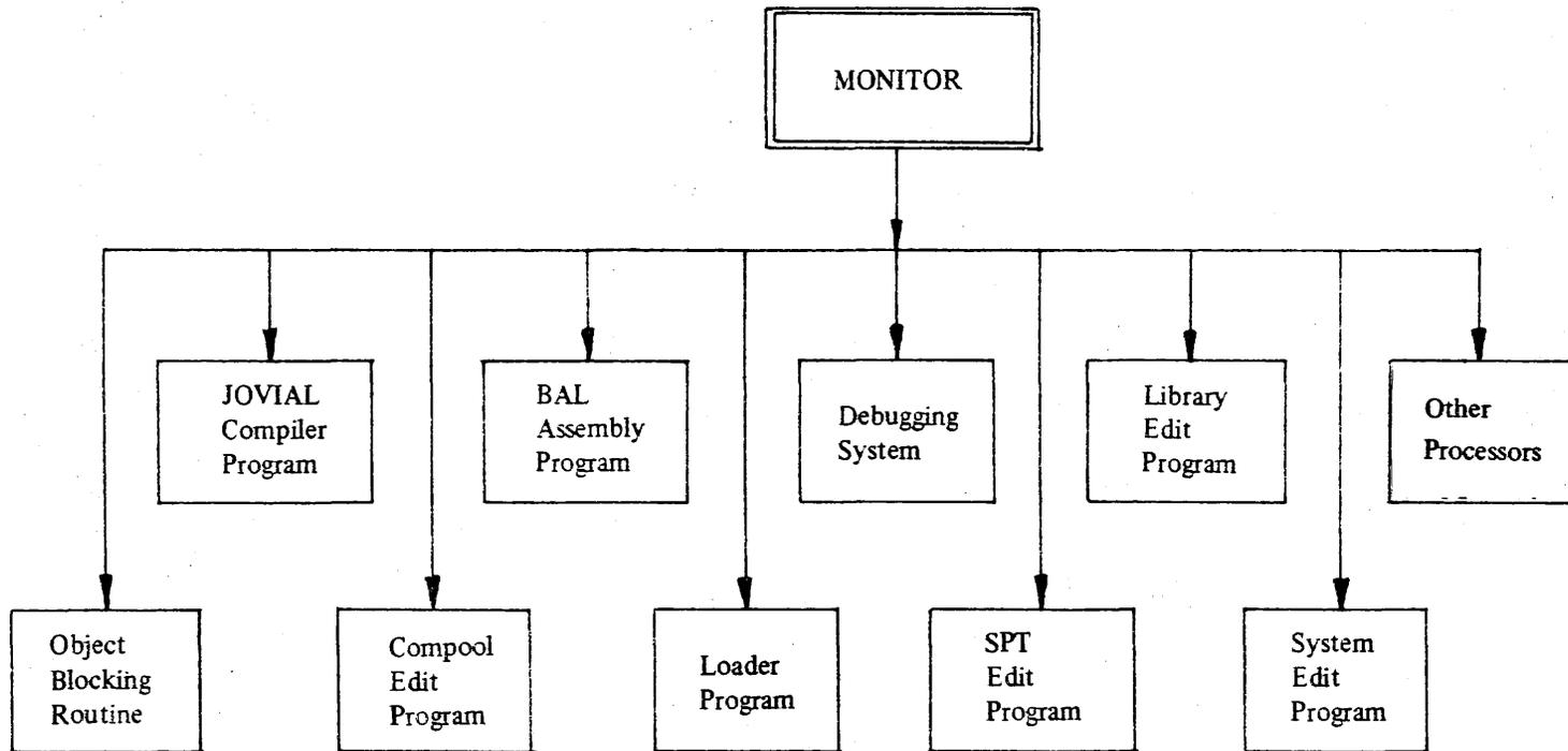
FIGURE 1-1. IBM 9020 NOSS PROGRAMMING SYSTEM
