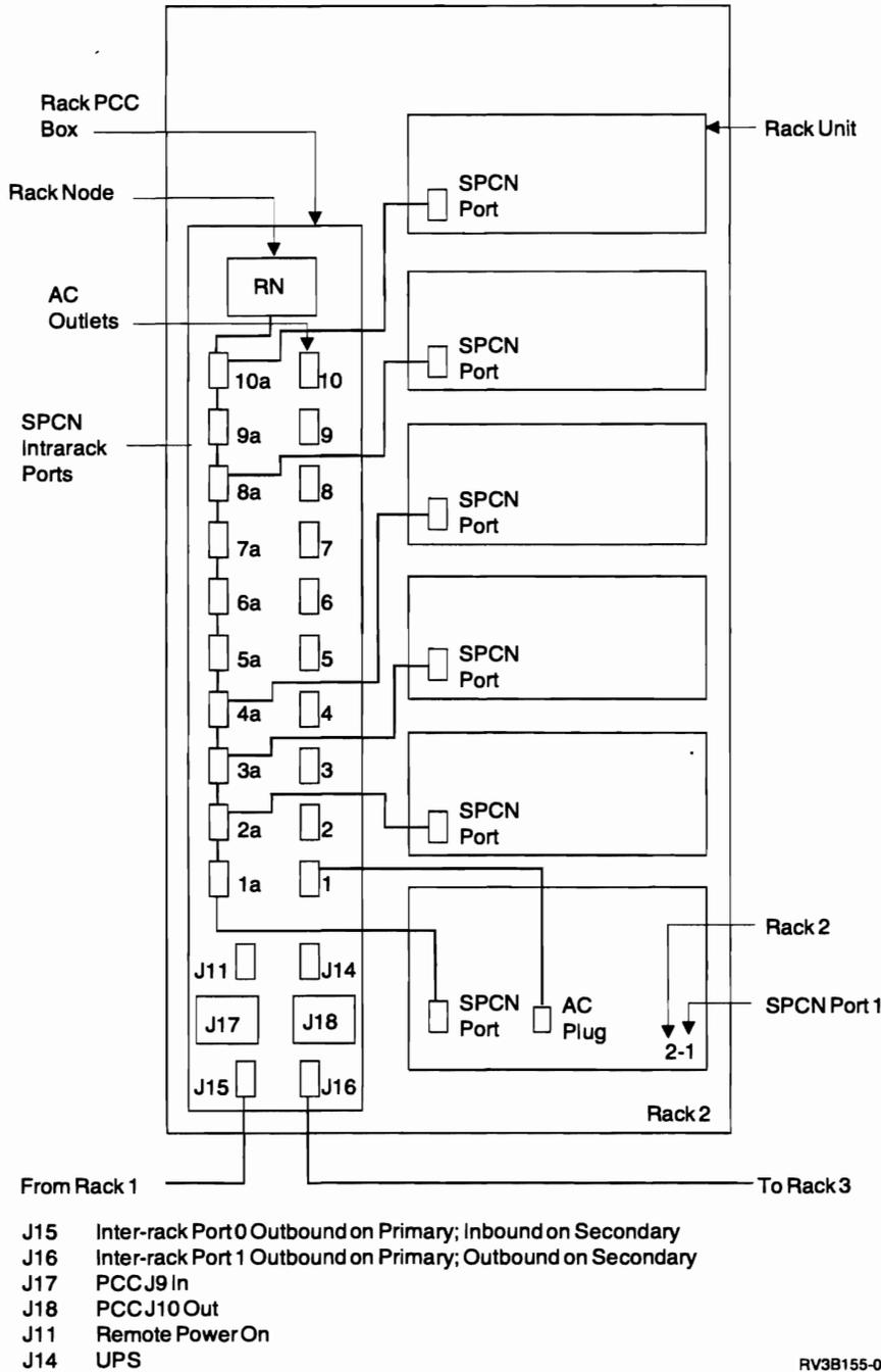
Figure 7-3. SPCN Secondary Rack Showing SPCN Addressing.
