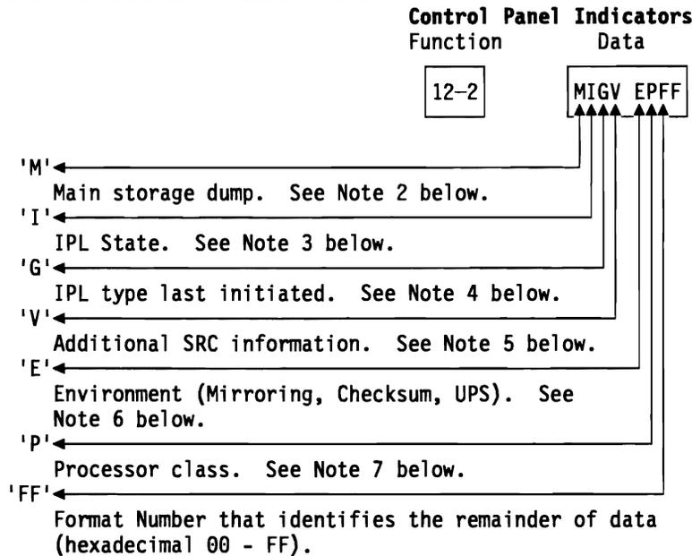
Figure 4-11. Structure of Fixed Data in Function 12-2
