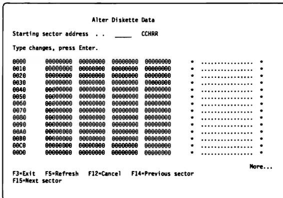
Figure 1-34. Example of Alter Diskette Data Display
