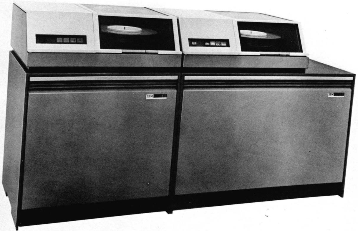
Figure 1. IBM 1311 Disk Storage Drive
