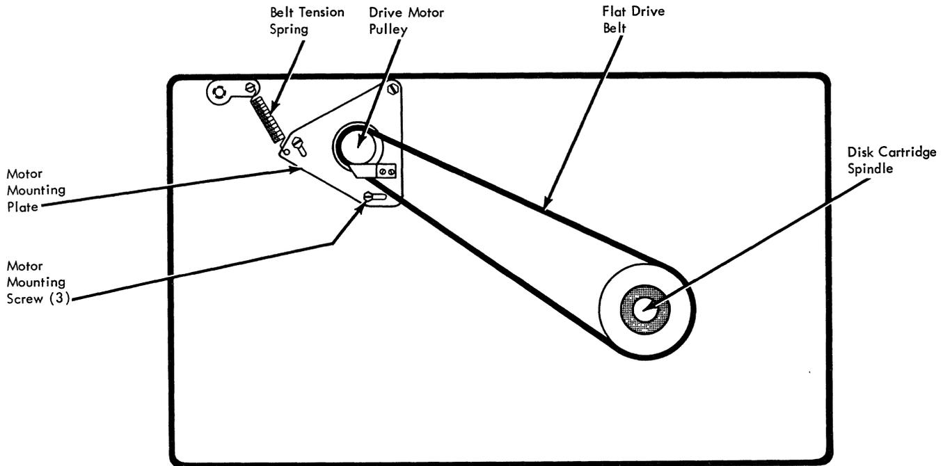
Figure 3-3. Drive Belt Adjustment
