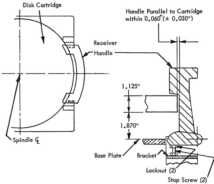
**(B) Latch Screw Clearance Adjustment**
