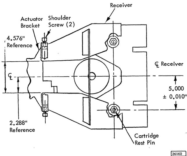
Figure 4-9. Cartridge Receiver Adjustment
