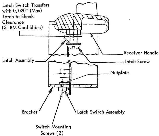
**(D) Interlock Magnet Adjustment**
