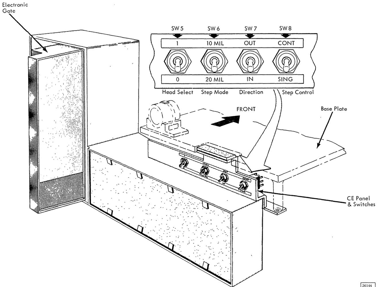
Figure 2-1. CE Panel and Switches
