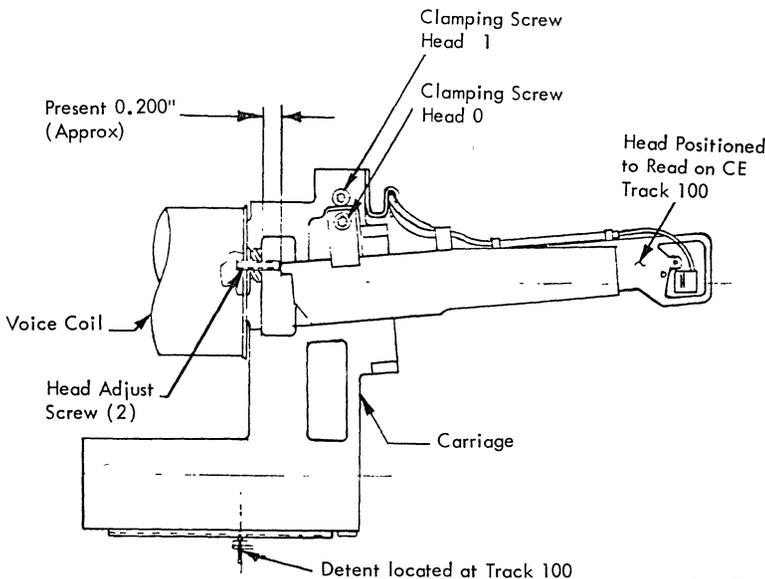
Figure 7-7. Head Arm Assembly Adjustment
