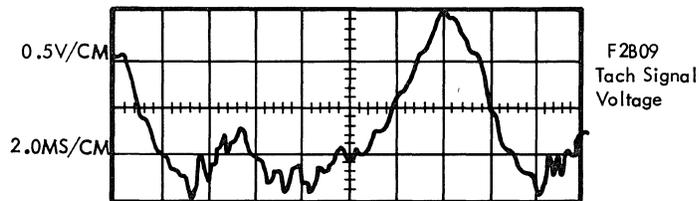
Figure 1-2. Oscilloscope Display of Access Circuits
