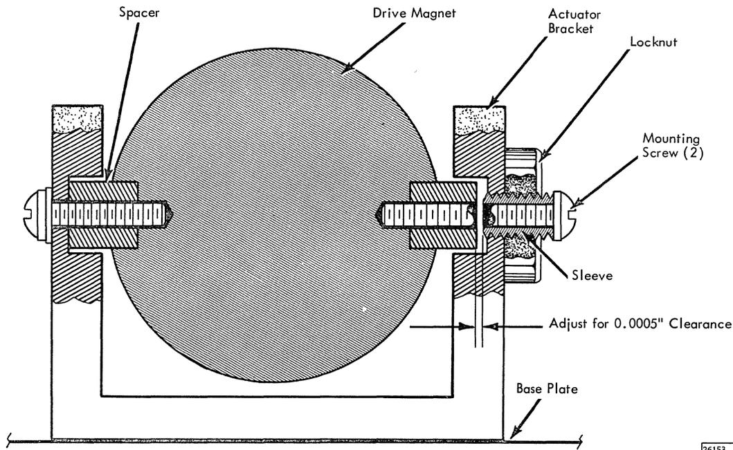
Figure 7-2. Drive Magnet Adjustment
