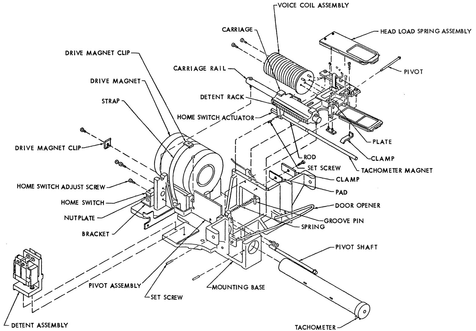
Figure 4-2. Actuator Assembly, Exploded View
