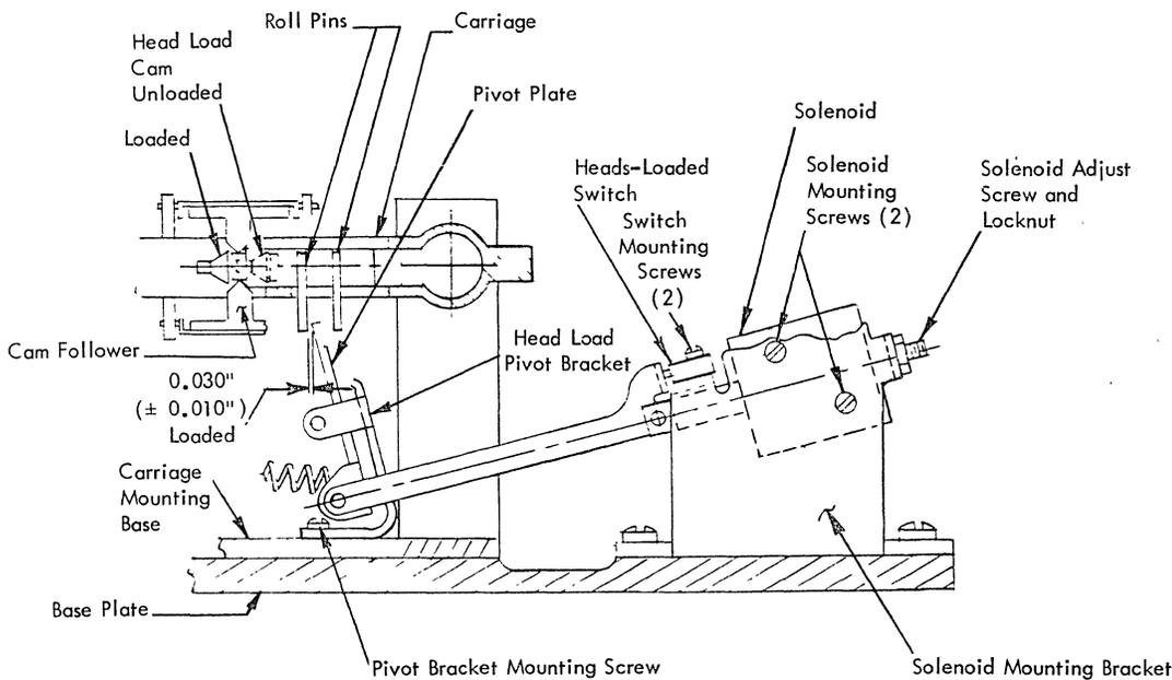
Figure 7-5. Head Load Assembly Adjustment
