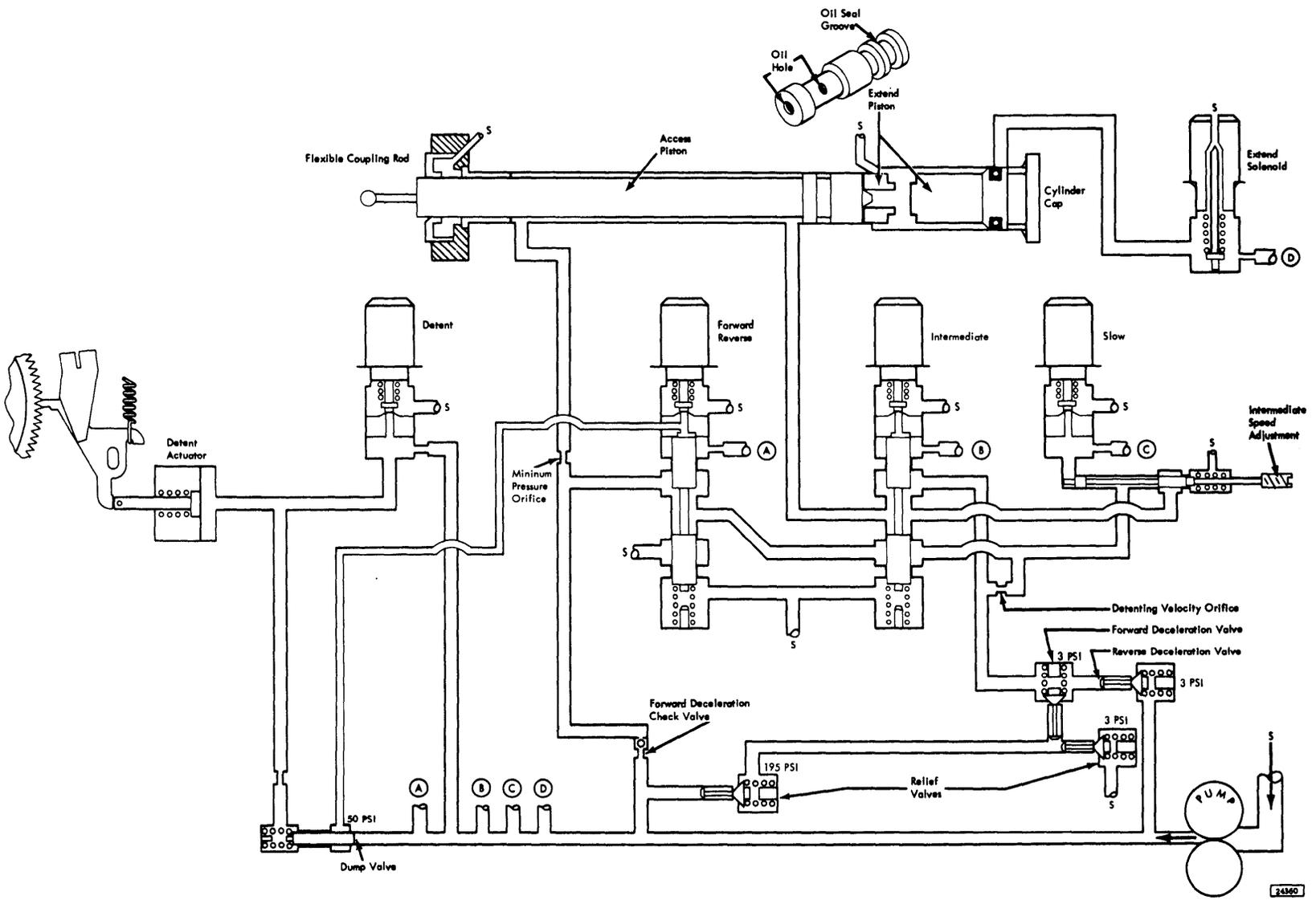
Figure 2-2. Hydraulic Actuator, Power Off
