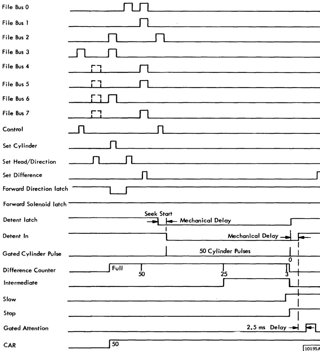
Figure 3-6. Programmed 50 Cylinder Forward Seek Model 1 (2841 SCU)
