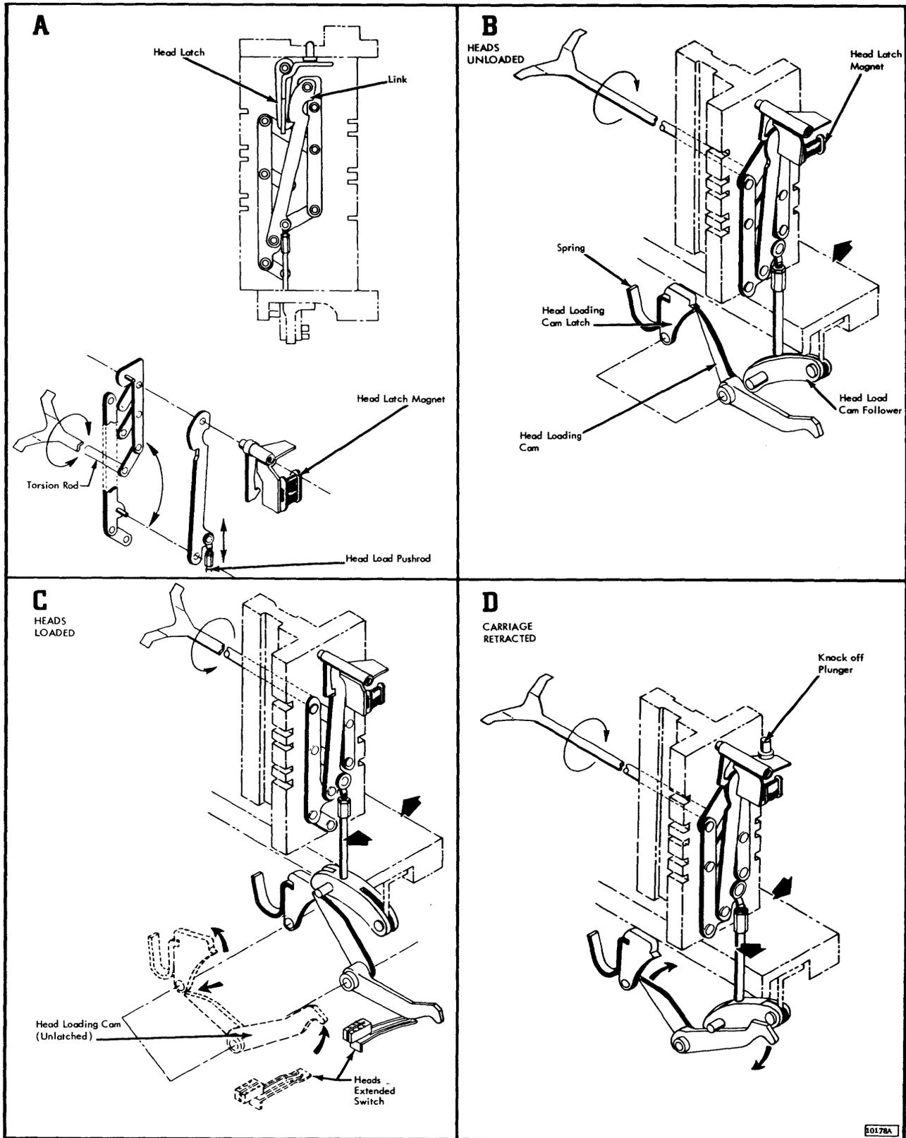
Figure 1-6. Head Load Mechanism
