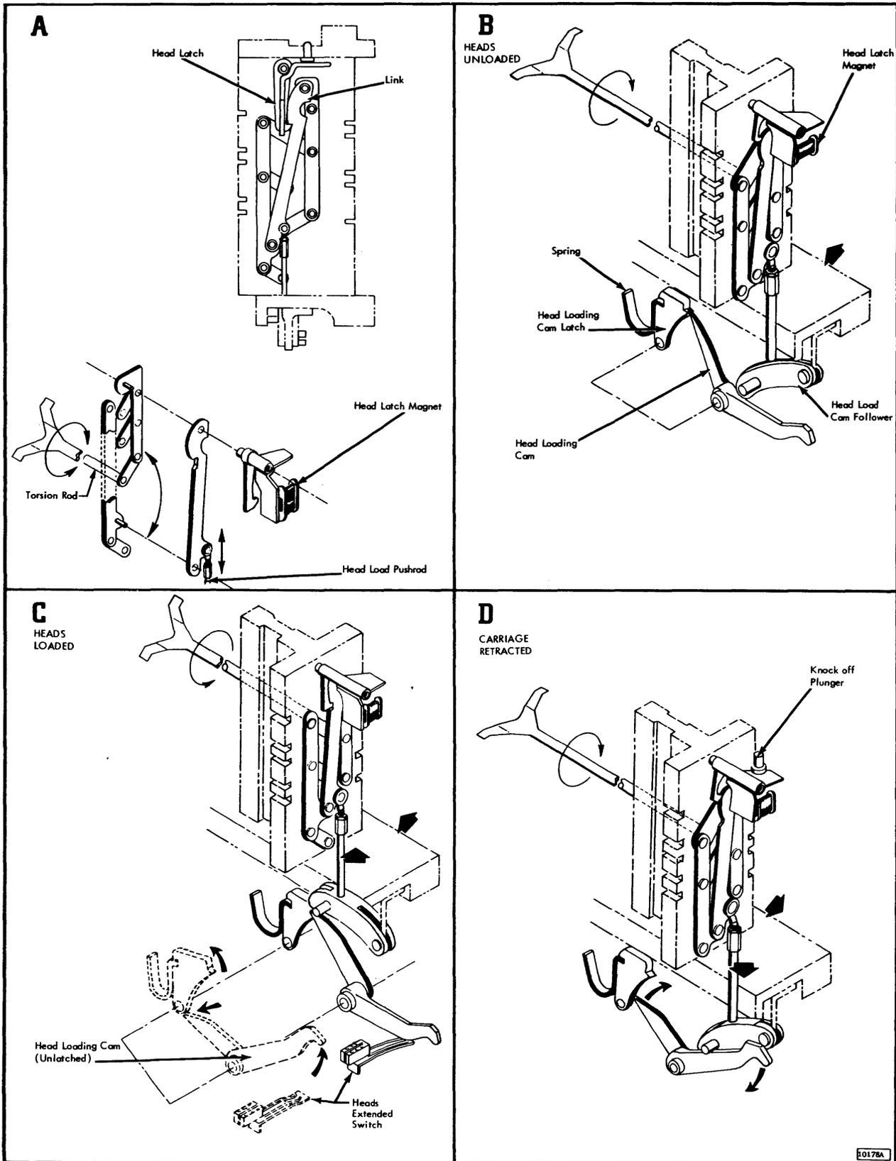
Figure 2-11. Head Load Mechanism
