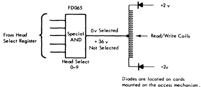
Figure 2-20. Read Write Head Selection
