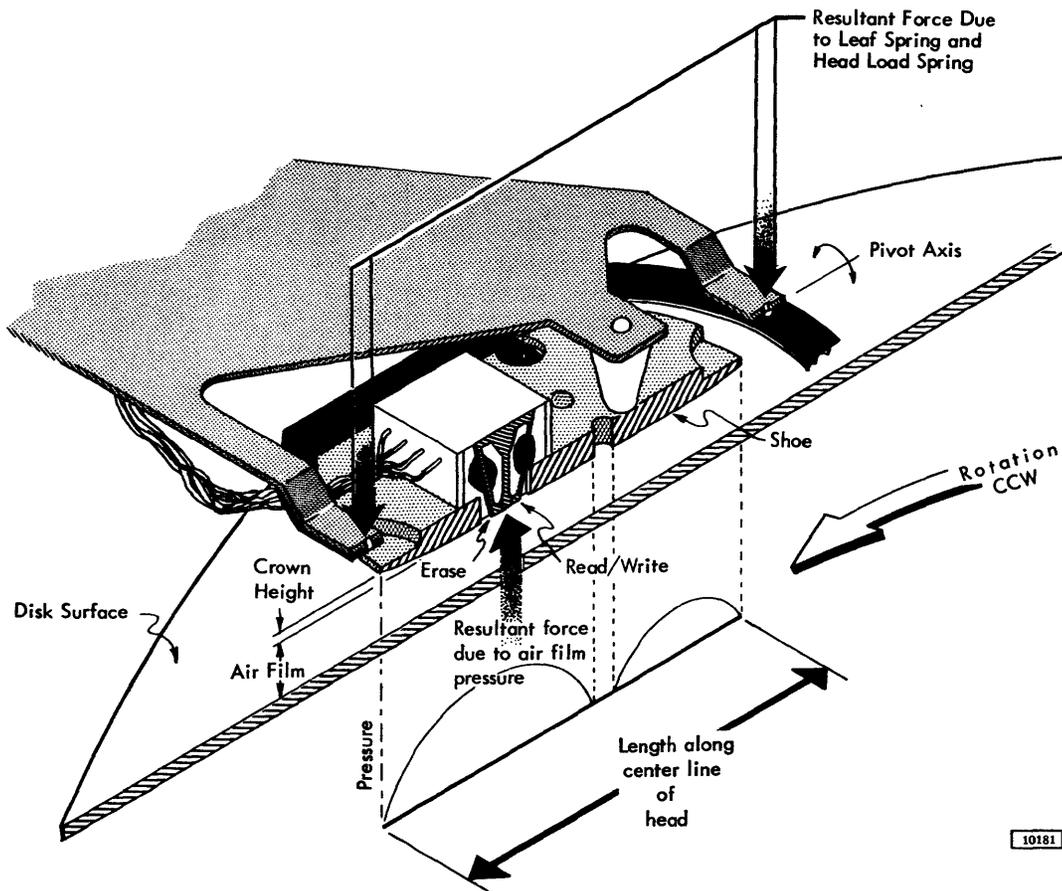
Figure 2-14. "Flying" the Read/Write Head
