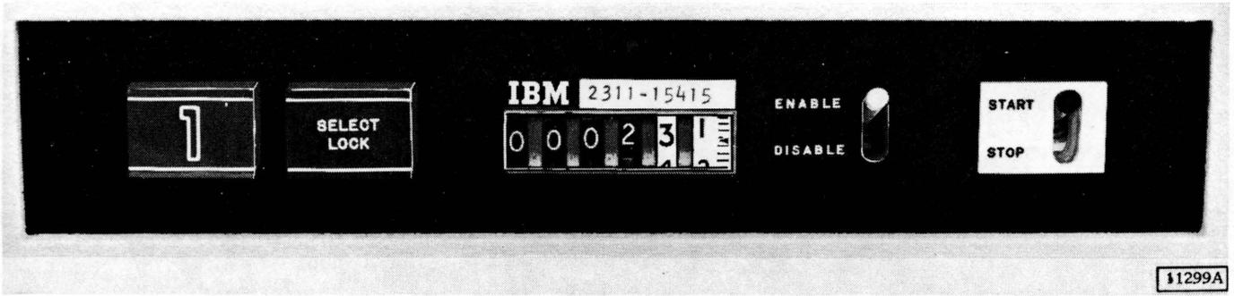
Figure 6-1. Operator Controls
