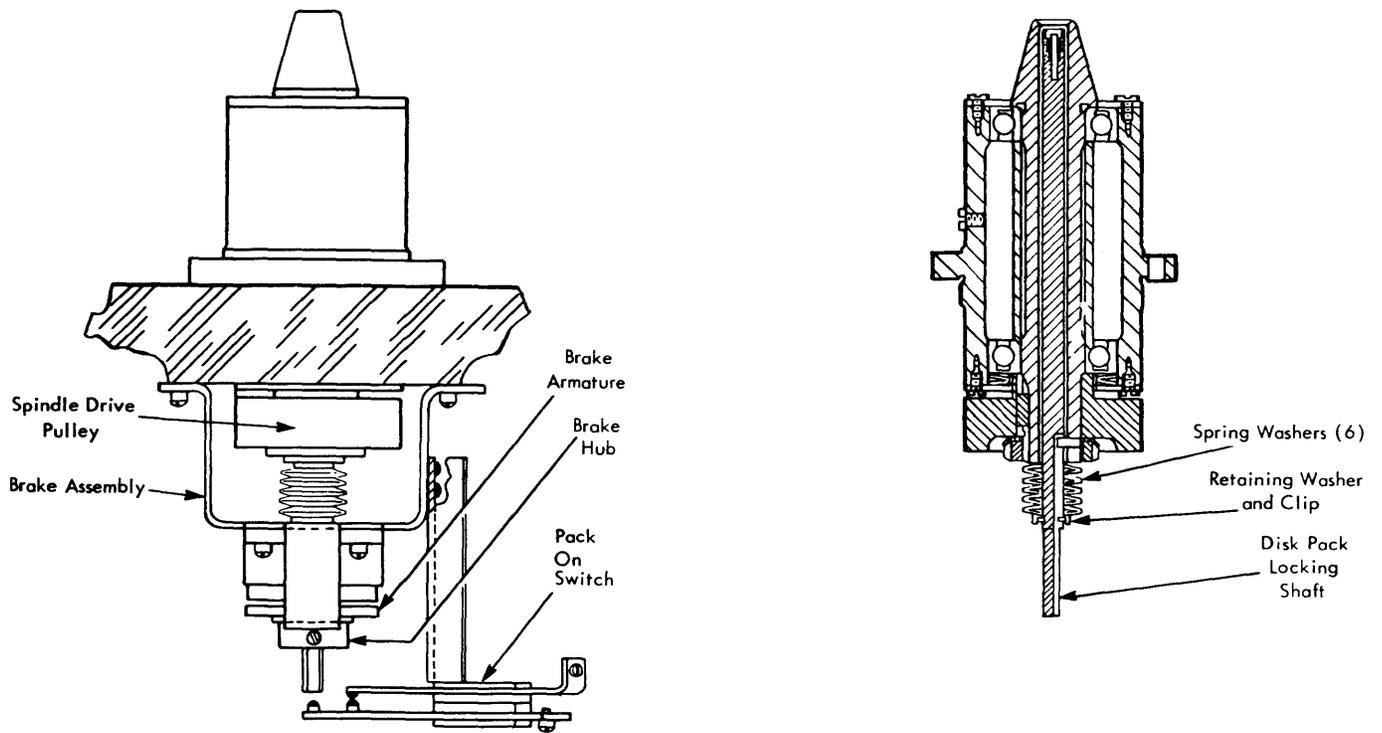
Figure 2-16. Disk Pack Spindle Assembly (Magnetic Brake)
