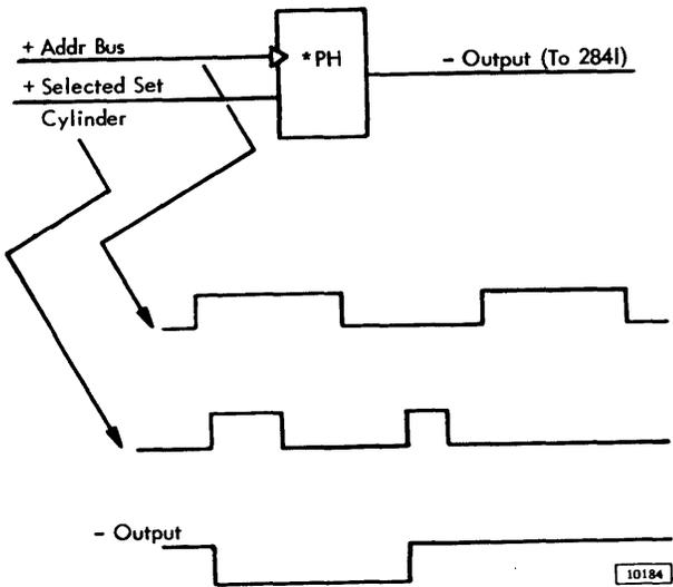
Figure 2-18. CAR Flip Latch Operation
