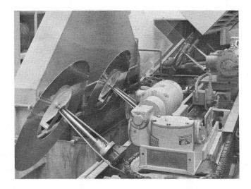
Automatic application equipment is used to apply an iron oxide coating to the disk. This coating, consisting of microscopically small iron oxide particles mixed with a binding agent, is uniformly applied over the surface of the disk. The thickness of the coating is controlled within millionths of an inch.
