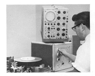
From the sonic-energy chamber, the parts are moved into a clean room. Here, the disks and the other components are carefully assembled so that the disk pack is precisely balanced—a strict requirement because of the high rotational speed of the disks on the 1311.
