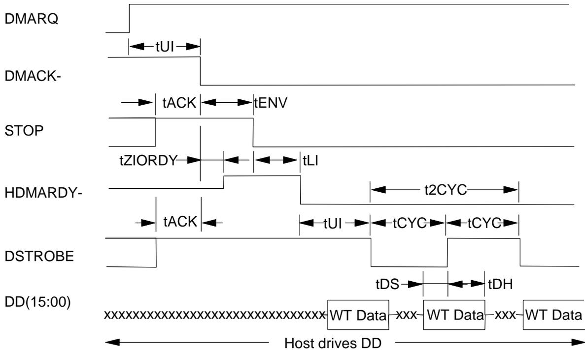
Figure 34. Ultra DMA cycle timing chart (Initiating Write)
