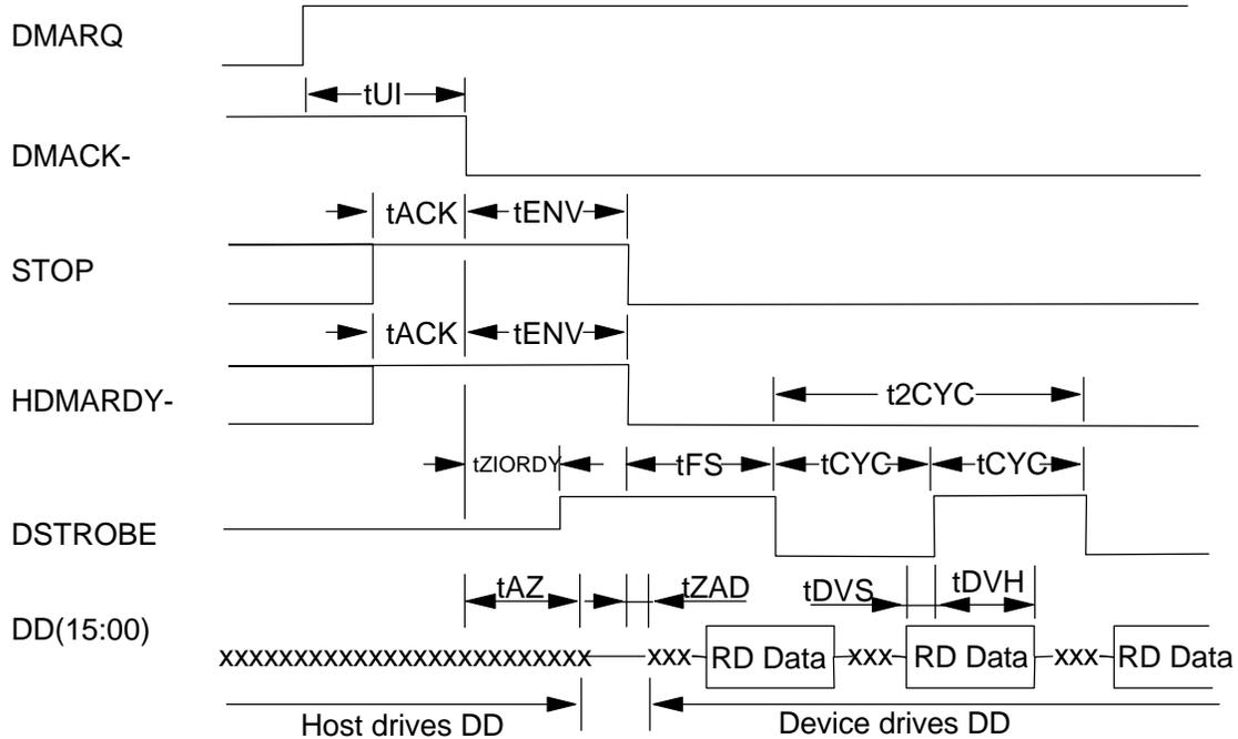
Figure 26. Ultra DMA cycle timing chart (Initiating Read)
