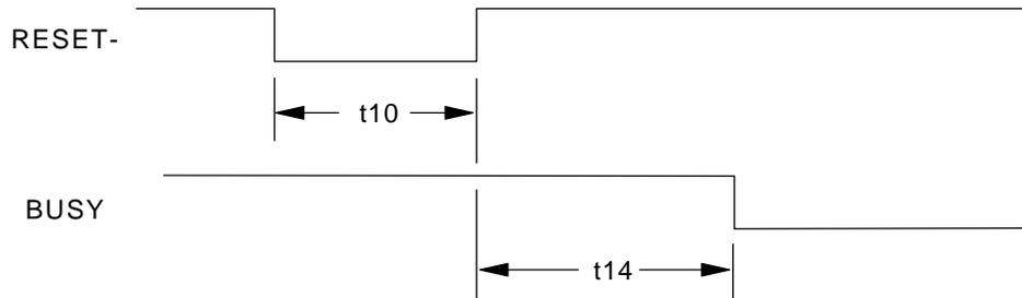
Figure 20. System reset timing chart
