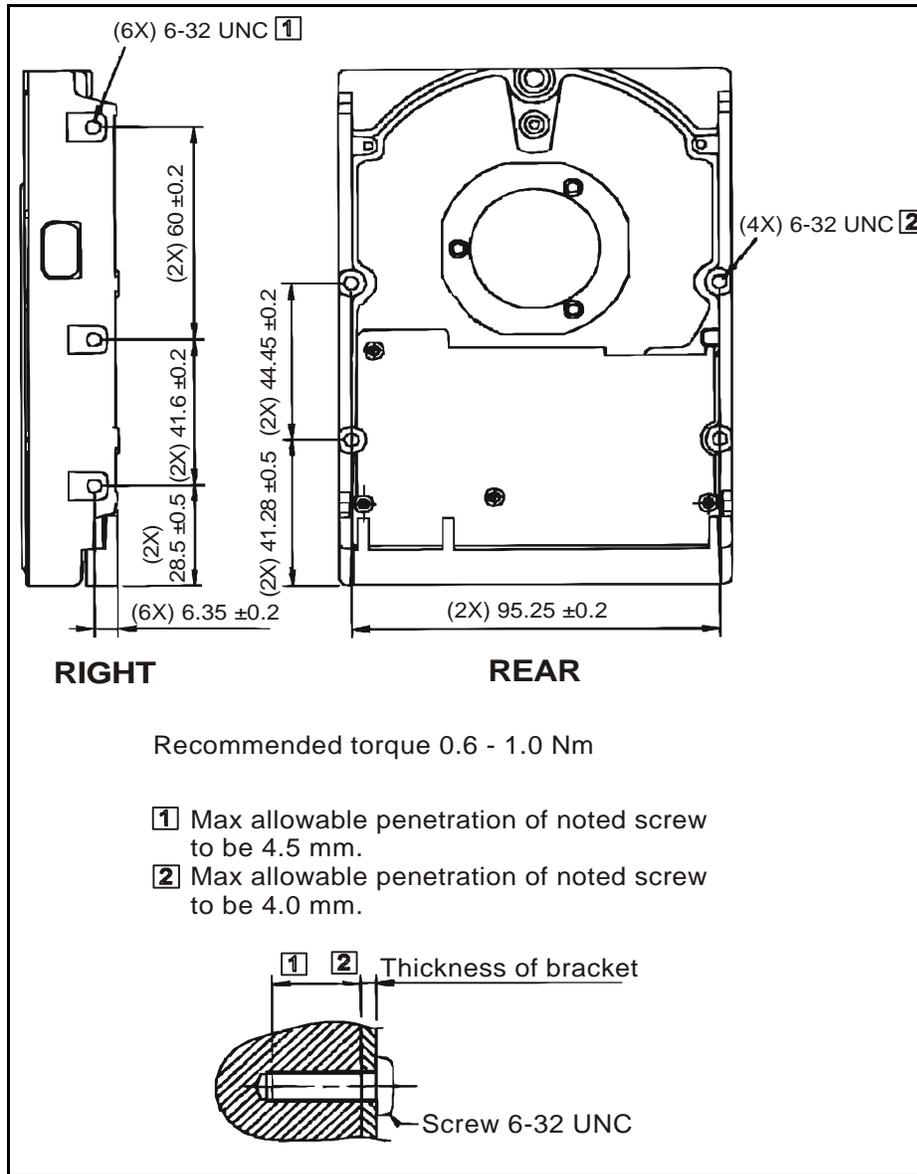
Figure 59. Mounting hole locations
