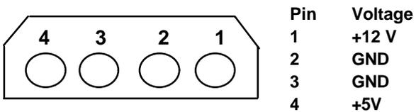
Figure 17. Power connector pin assignments
