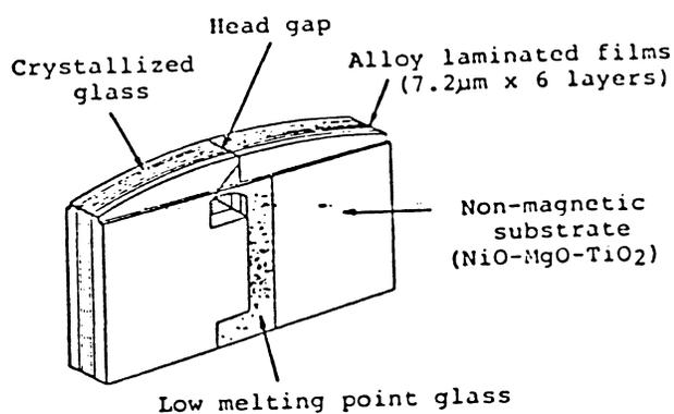
Fig.2. An outside view of the alloy laminated films head.
