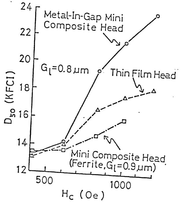
Fig. 8 Dependence of recording density  $D_{50}$  on coercive force of disk
