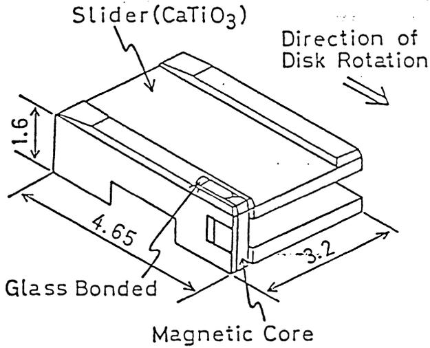
Fig. 2 Schematic structure of metal-in-gap mini composite head
