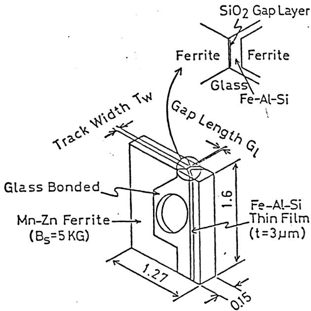
Fig. 1 Schematic structure of magnetic core
