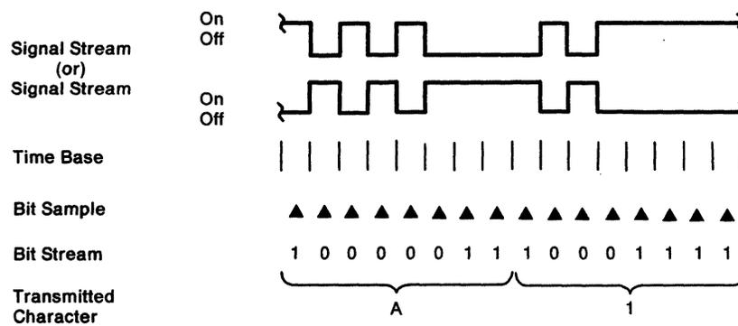
Figure 9. Invert-on-Zero Transmission Coding
