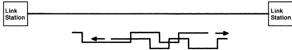
When one station transmits, the other station must receive; otherwise, no communication occurs.
