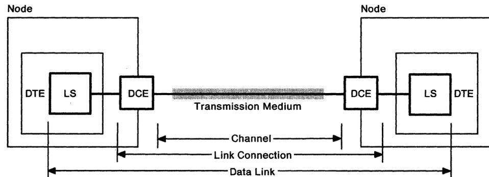
DCE Data Circuit-terminating Equipment
