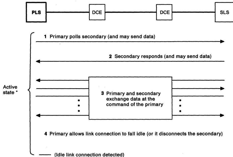
\* A half-duplex link connection is in transient state during each line turnaround
