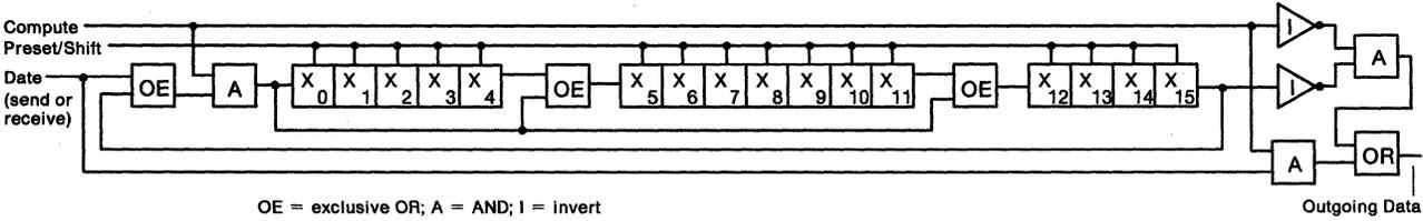
Figure 31. An Example of Cyclic Redundancy Checking
