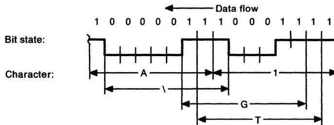
The receiver and the transmitter must be in bit and character synchronism (lack of synchronism results in inability of receiver to determine if incoming character is A, \, G, or T).
