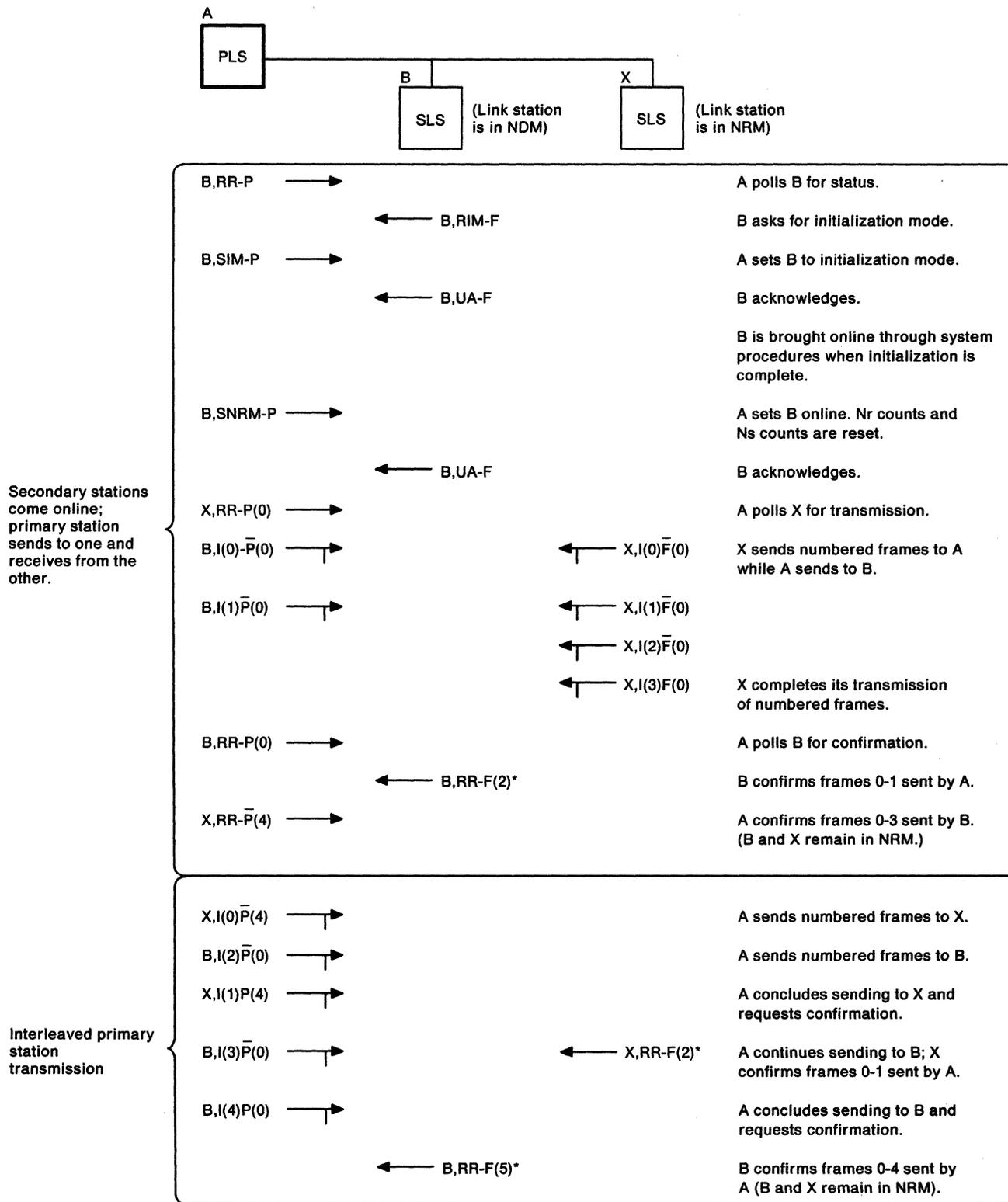
Figure 27. Two-way Simultaneous Exchanges on Nonswitched Multipoint Links
