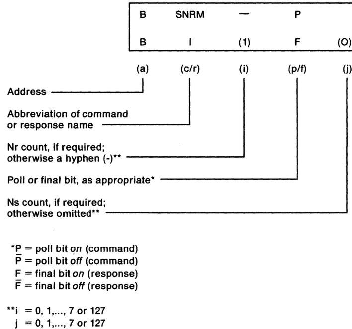
Figure 24. Format of Examples of SDLC Exchanges
