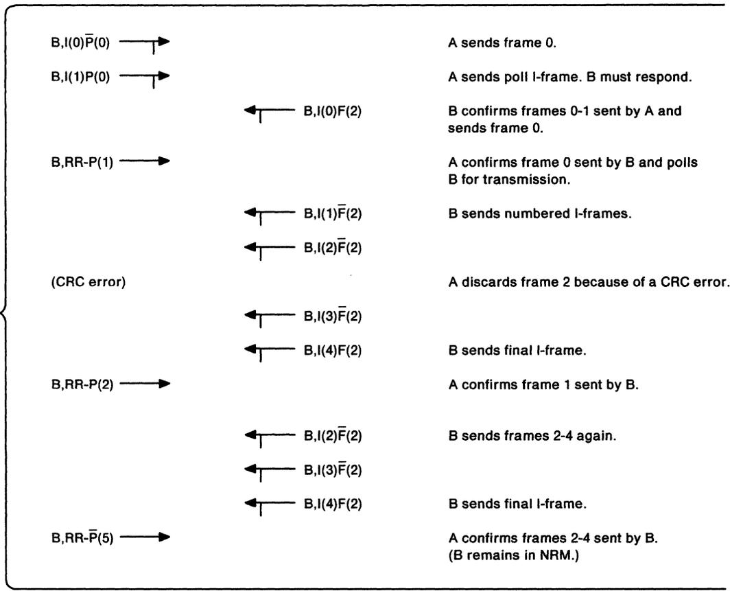
Figure 25 (Part 2 of 2). Two-way Alternate Exchanges on Nonswitched Point-to-Point Links
