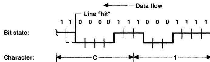
A single binary digit is changed by a transmission error. The receiver must recognize that the error has occurred.
