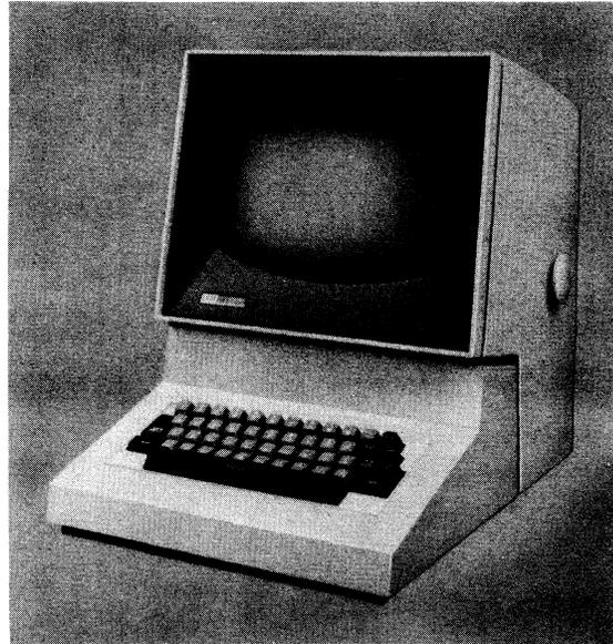
Figure 5. IBM 2260 Display Station
