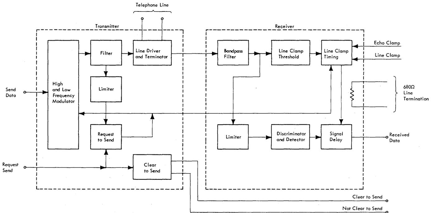
FIGURE 2-25. IBM LIMITED DISTANCE ADAPTER, TYPE 2B
