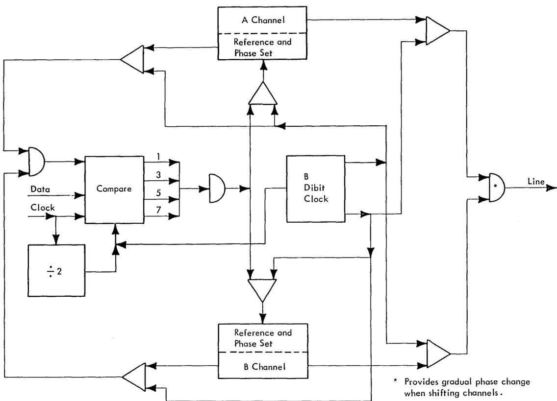
FIGURE 3-1. FOUR PHASE DATA SET - TRANSMIT CONCEPT
