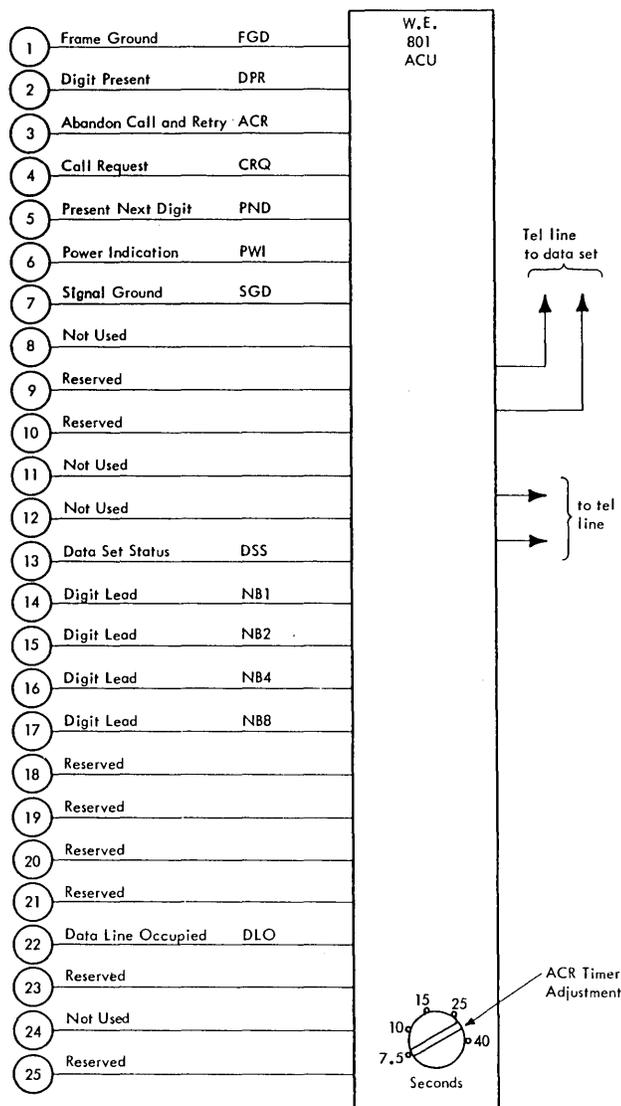
FIGURE 2-32. AUTOMATIC CALLING UNIT, WE 801A INTERFACE
