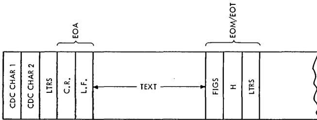
FIGURE 1-33. FORMAT OF TAPE MESSAGE, 83B2 SYSTEM
