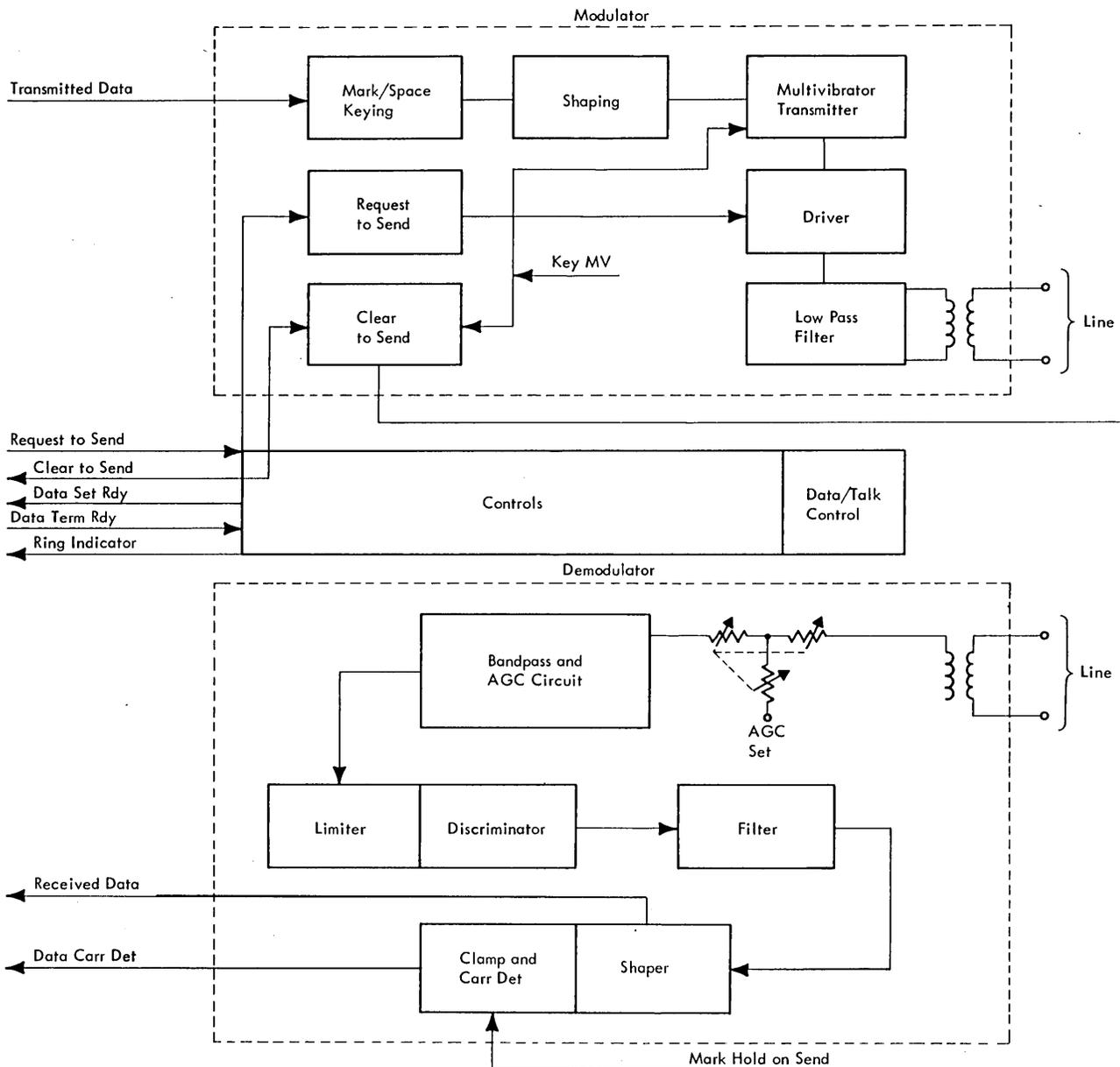
FIGURE 2-30. DATA SET WE 202, BLOCK DIAGRAM
