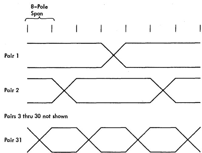
FIGURE 2-19. LINE TRANSPOSITION
