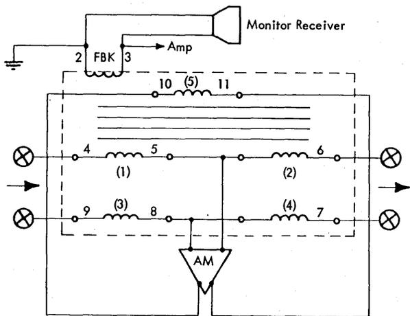
FIGURE 2-16. SIMPLE TWO-WIRE REPEATER
