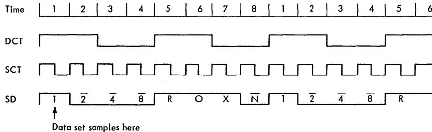
FIGURE 3-4. RELATION OF DCT, SCT, AND SD
