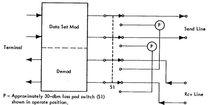
FIGURE 2-33. LOOPBACK TEST SWITCH
