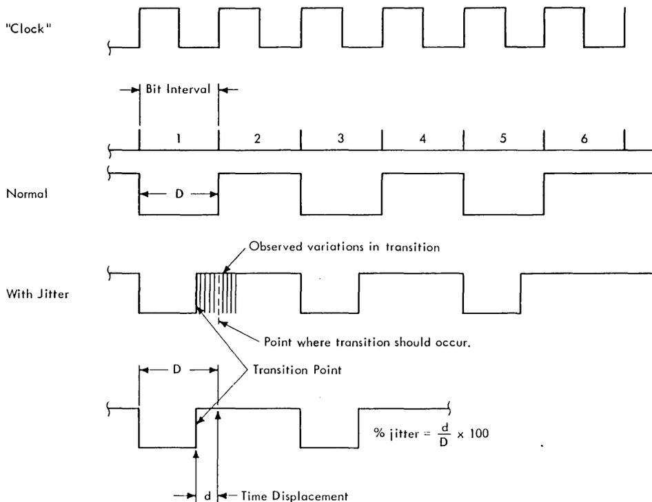
FIGURE 2-34. JITTER MEASUREMENT
