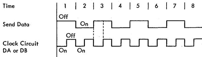
FIGURE 2-23. TRANSMIT CLOCK
