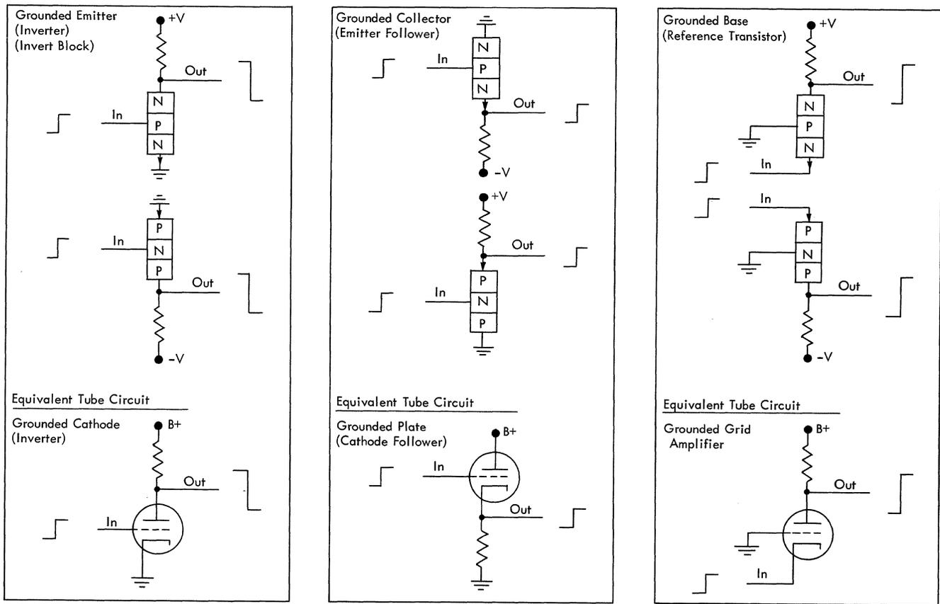
Figure 2. Transistor Circuit Configurations
