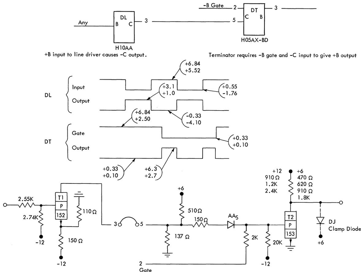
Figure 58. C Level Driver and Terminator
