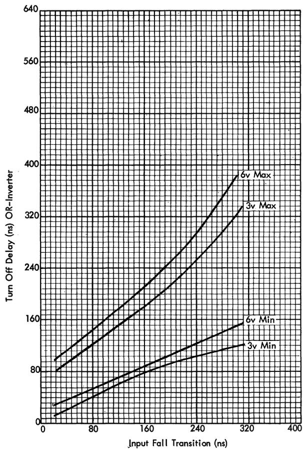
Figure 88. Turn-Off Delay of OR Inverter
