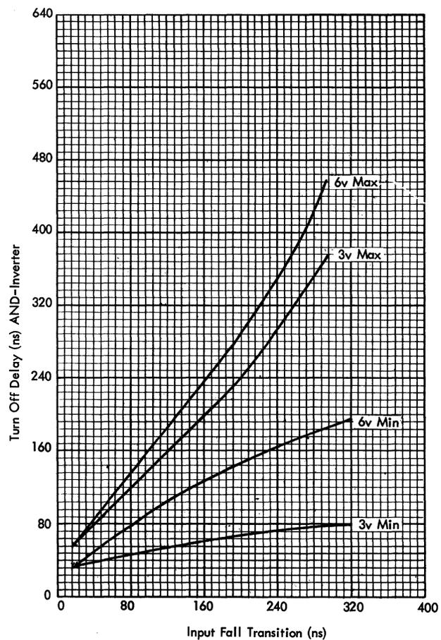
Figure 89. Turn-Off Delay of AND Inverter
