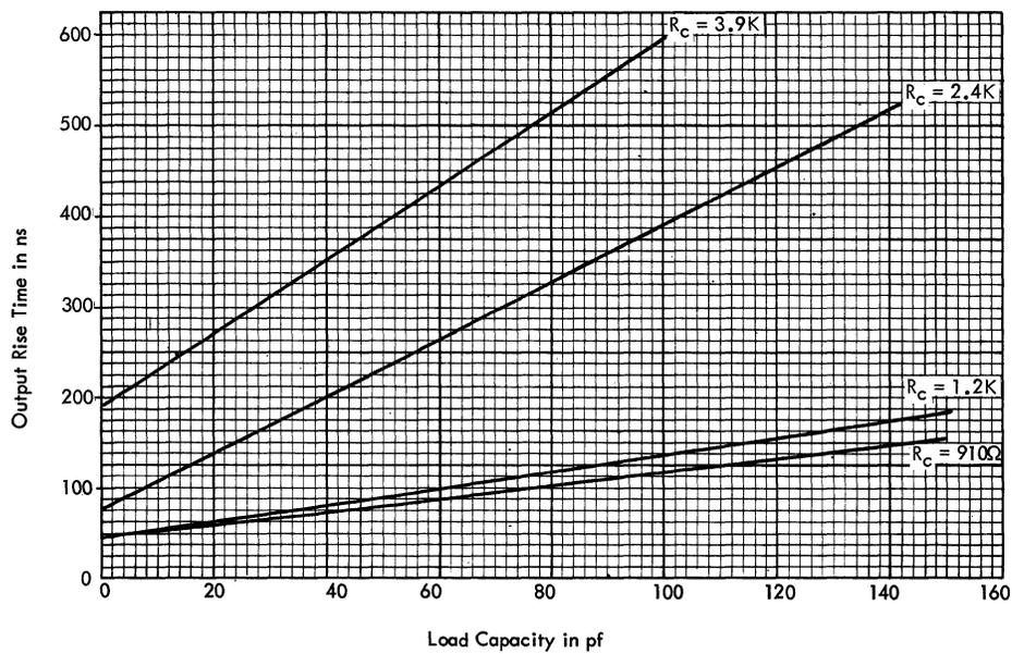
Figure 93. Output Rise Transition of Clamped Basic Inverter
