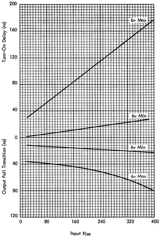
Figure 98. Turn-On Delay and Fall Transition of AND LLPI
