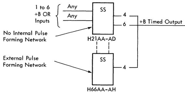
Figure 50. Pulse Former Single-Shot without Internal Network
