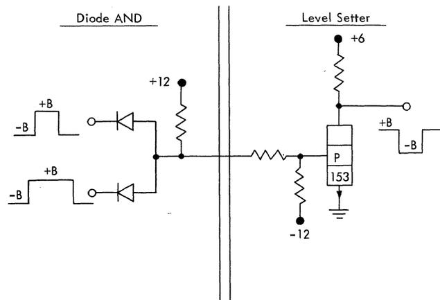
Figure 23. Level Setting Circuit
