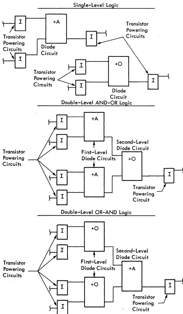
Figure 11. Single-Level and Double-Level Logic
