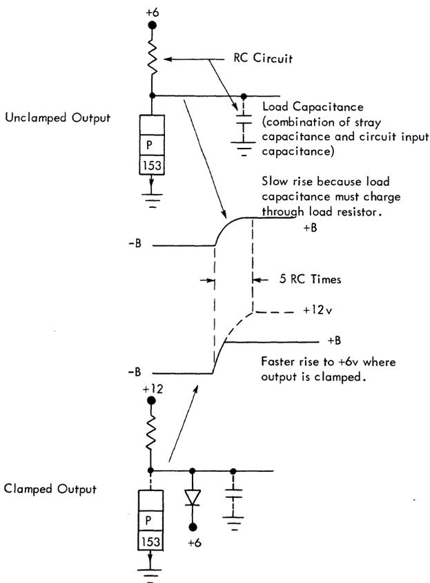
Figure 19. Rise Times of Clamped and Unclamped Outputs
