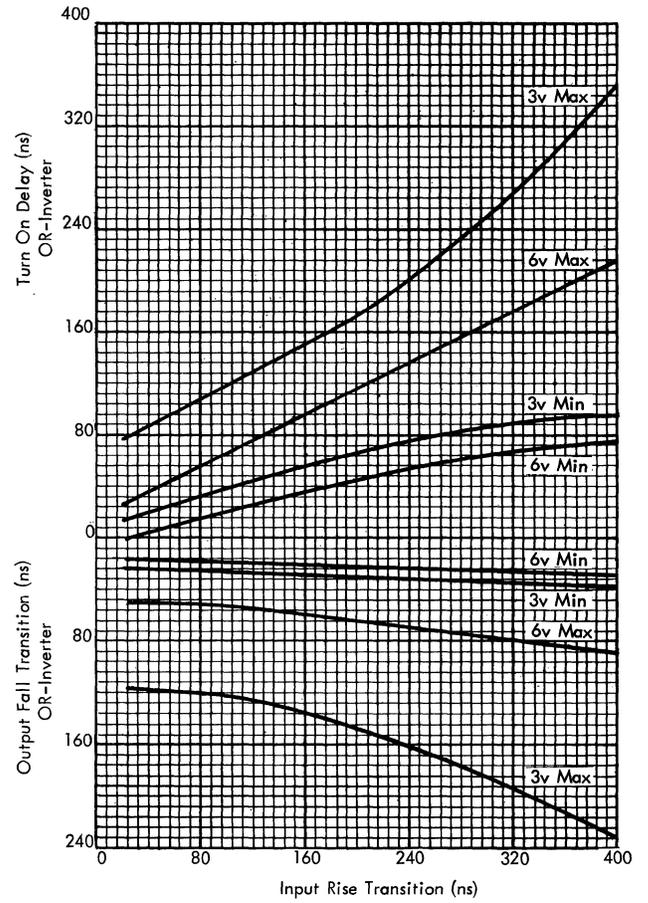
Figure 83. Turn-On Delay and Fall Transition of OR Inverter
