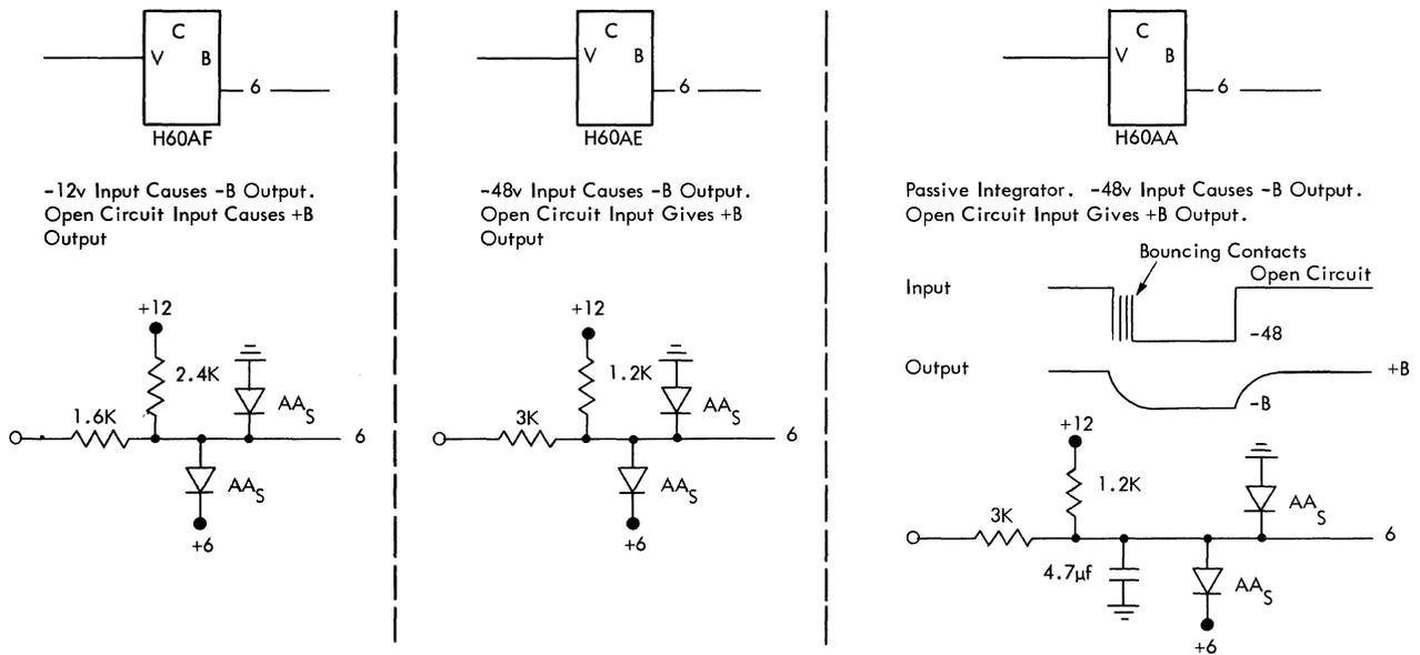
Figure 64. V to B Converters
