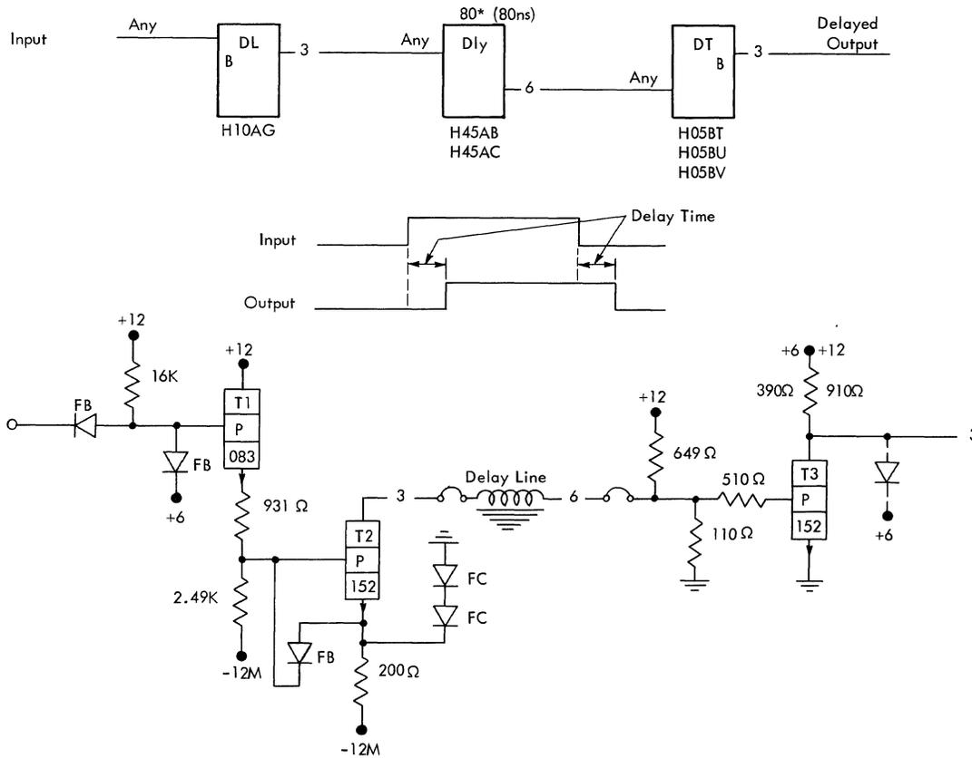
Figure 57. Delay Line Driver and Terminator
