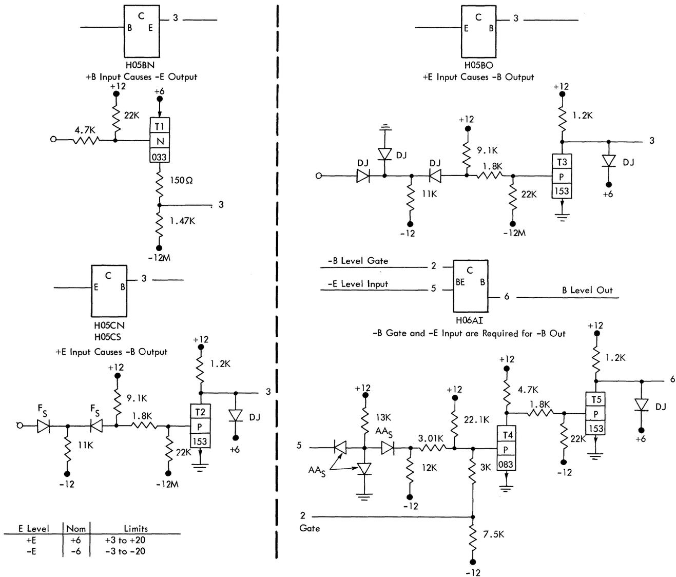
Figure 60. B to E and E to B Converters
