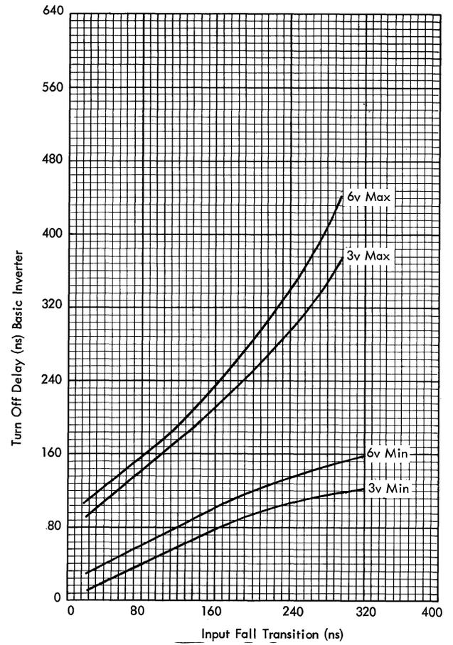
Figure 87. Turn-Off Delay of Basic Inverter
