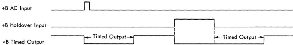
If holdover input is +B, output is -B. When the holdover input goes to -B, output remains minus for time duration of SS. Only if the holdover input is -B, can the AC input fire the SS.
