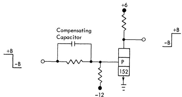
Figure 20. Logical Low Power Inverter
