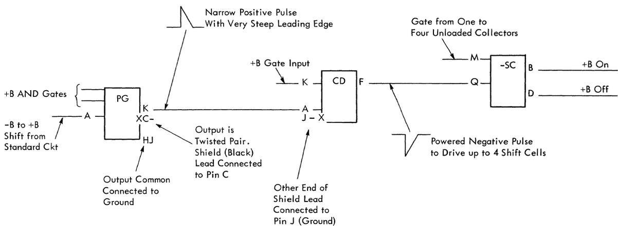
Figure 41. Shift Cell Circuits
