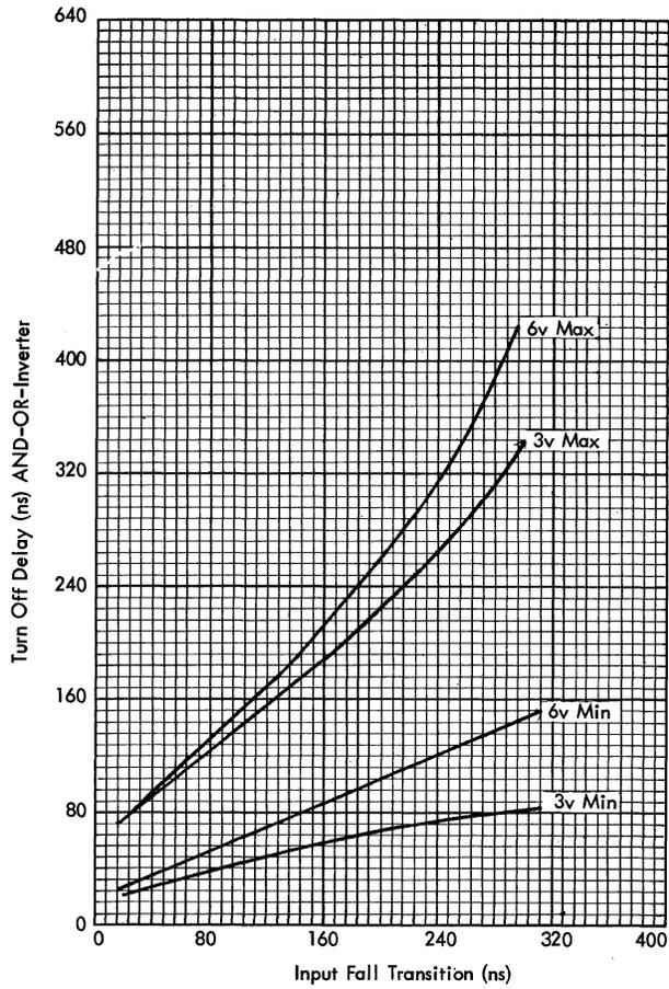
Figure 90. Turn-Off Delay of AND-OR Inverter
