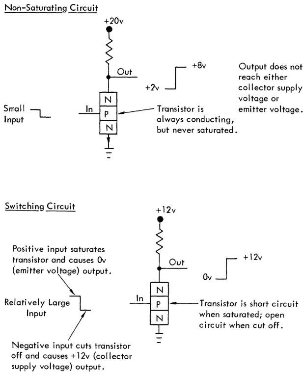
Figure 4. Transistor Operating Modes
