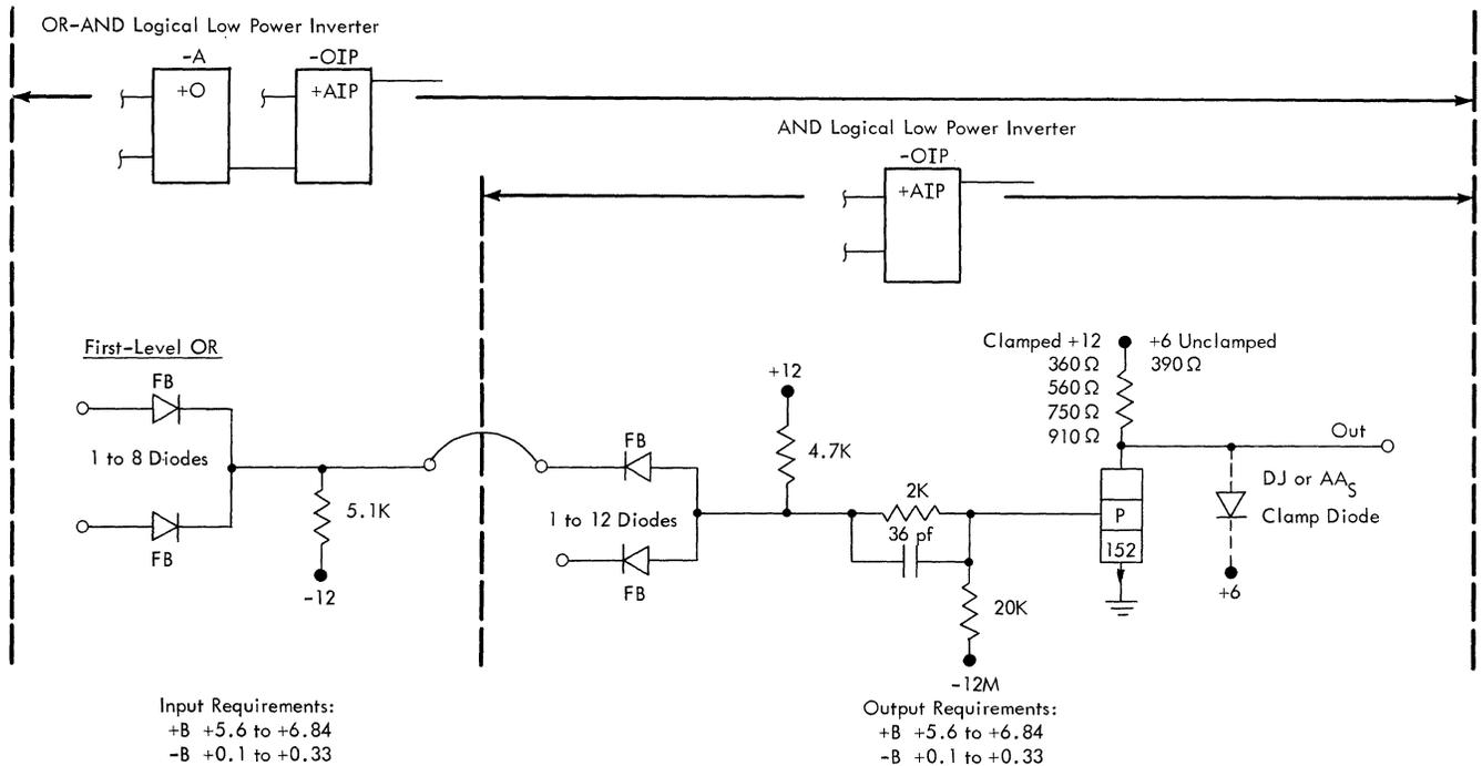
Figure 30. AND Logical Low Power Inverter
