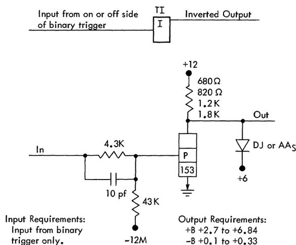
Figure 37. Binary Trigger Inverter
