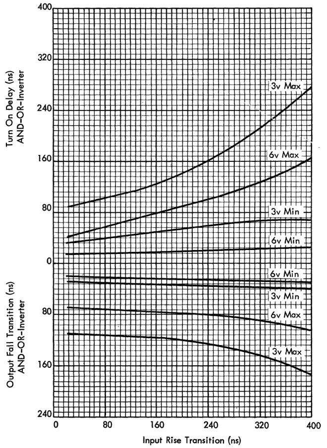
Figure 85. Turn-On Delay and Fall Transition of AND-OR Inverter
