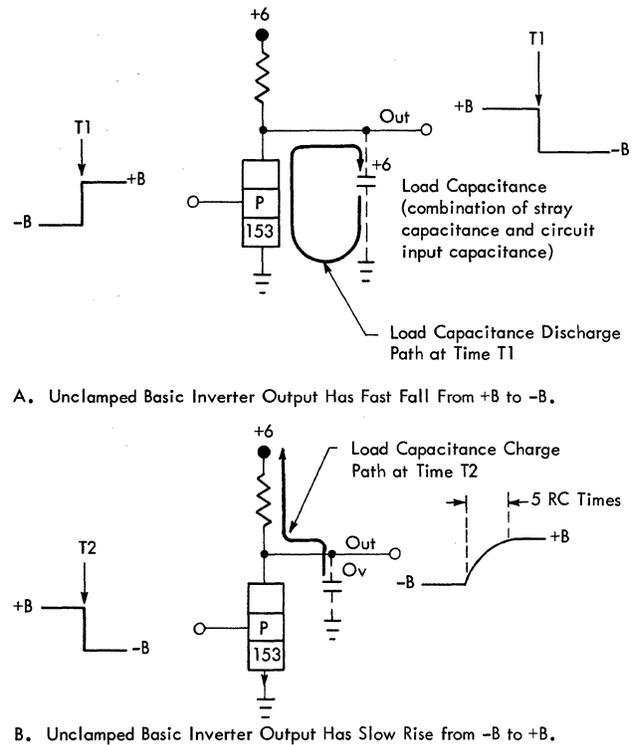
Figure 18. Basic Inverter Output Rise and Fall
