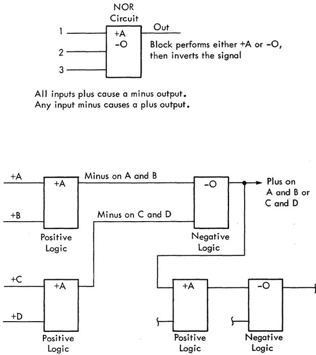
Figure 8. Alternate Positive and Negative Logic
