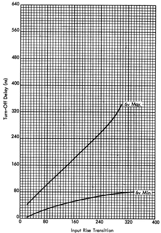
Figure 99. Turn-Off Delay of AND LLPI
