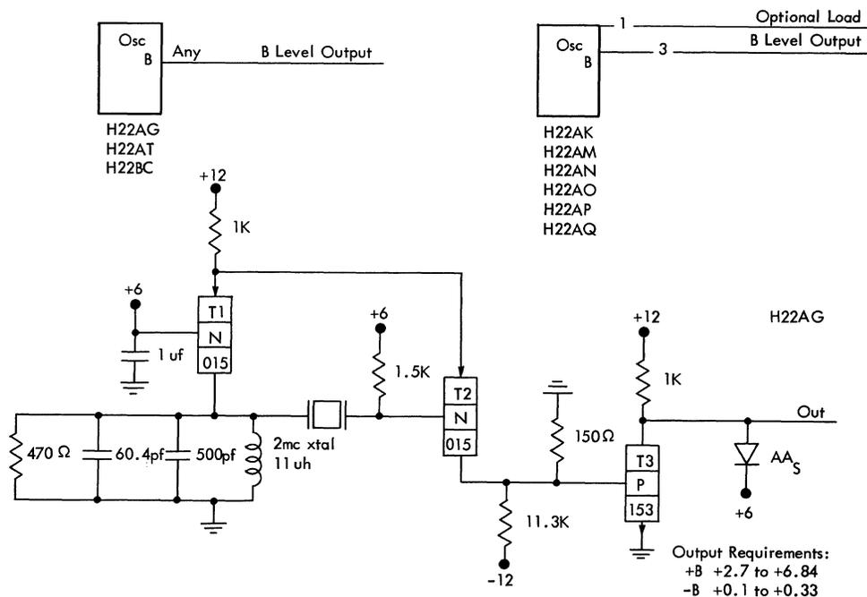
Figure 53. Crystal-Controlled Oscillator, Example 1
