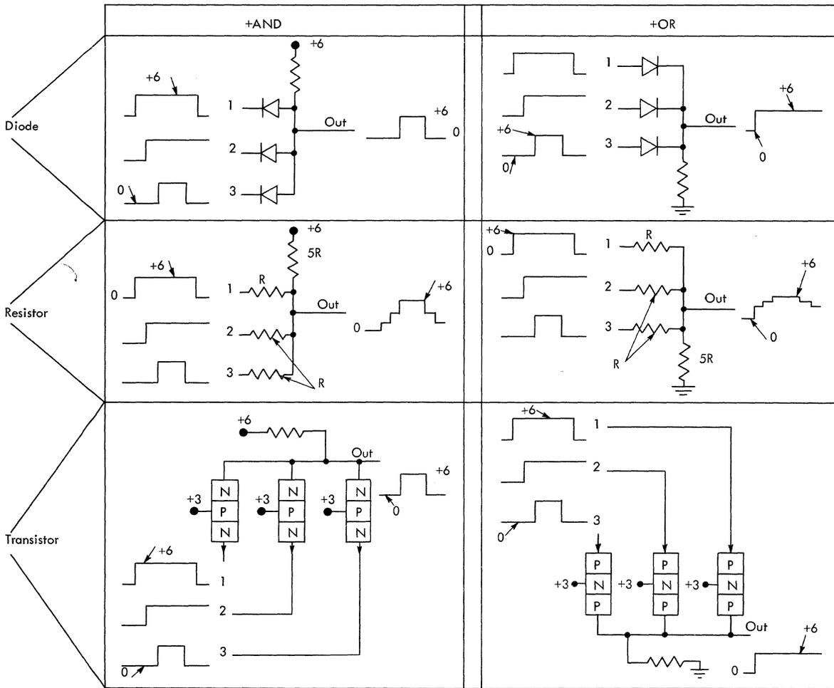
Figure 5. Logic-Performing Circuits
