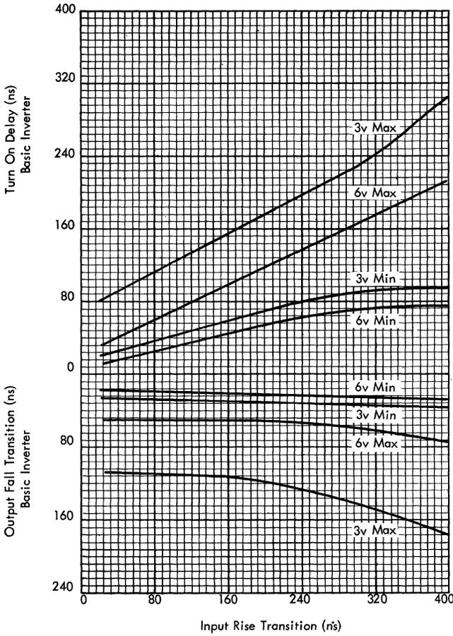
Figure 82. Turn-On Delay and Fall Transition of Basic Inverter
