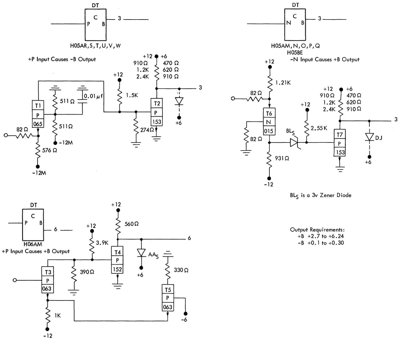
Figure 62. Current Switching to DDTL Converters
