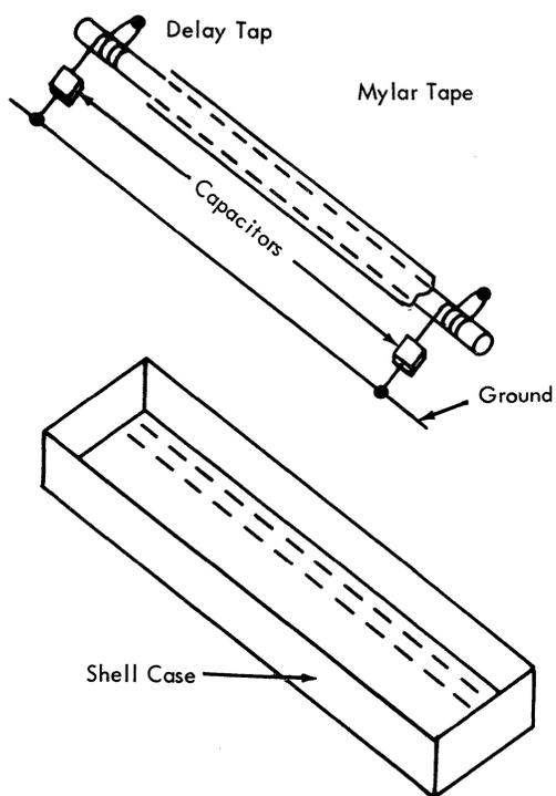
Figure 6-35. Distributed Constant Delay Line
