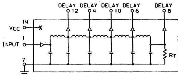
Figure 6-36. Active Delay Line Schematic
