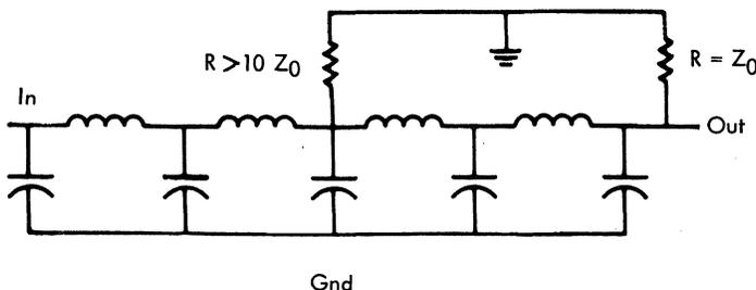
Figure 6-42. Tapped Delay Line Loading Circuit
