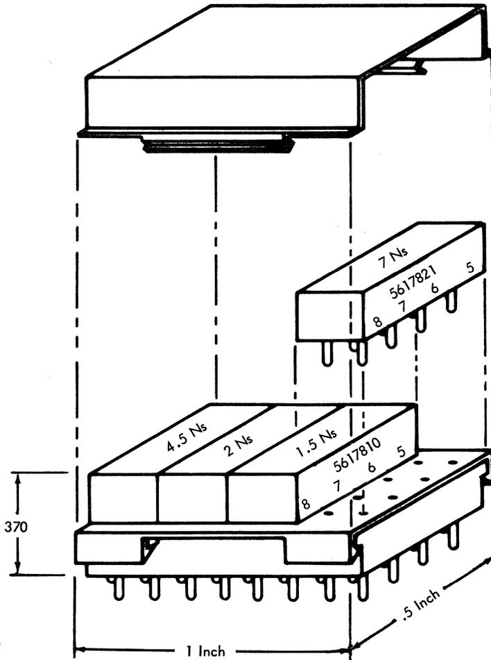
Figure 6-41. Pluggable Delay Line and Socket
