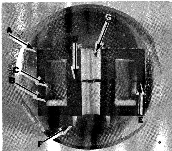
Figure 6-16. Mid-Plane Section through a Typical AF Pot Core Transformer/ Inductor Assembly Showing:
