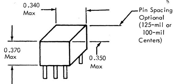
Figure 6-20. Laminated-Core Transformer
