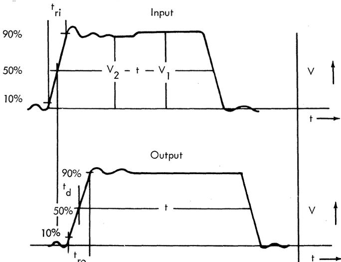
Figure 6-38. Typical Pulse Waveforms
