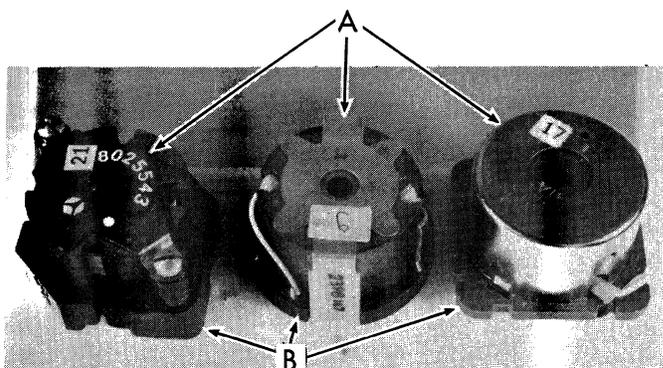
Figure 6-17. Some Examples of Older, Costly AF Transformer/Inductor Construction Practices
