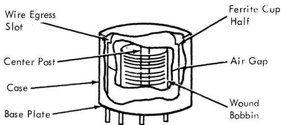
Figure 6-19. Pot-Core Transformer
