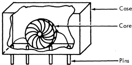
Figure 6-18. Toroidal-Core Transformer
