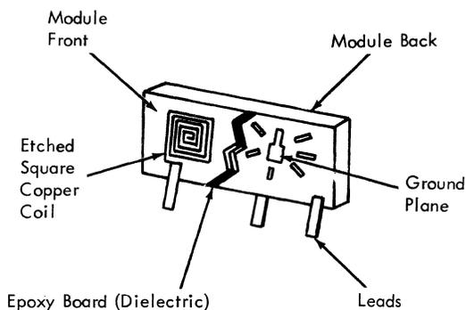
Figure 6-37. Typical R-Pac Delay Line Construction
