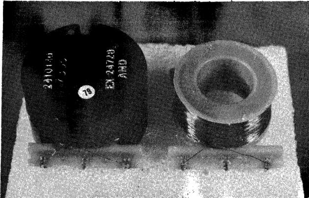
Figure 6-14. Typical Pot Core AF Transformer/Inductor Construction; Complete Unit on Left, Coil/Bobbin/Pin Unit on Right
