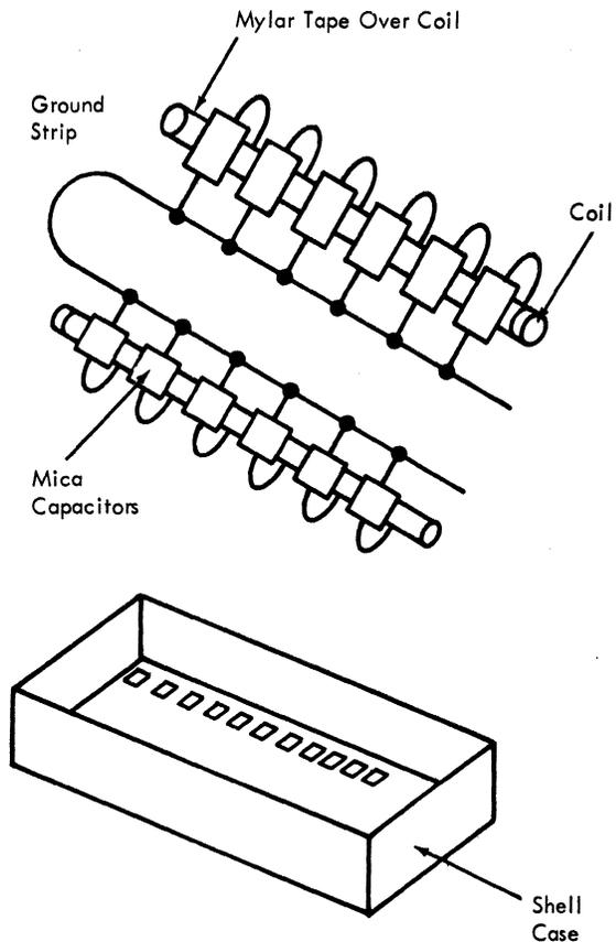
Figure 6-33. Lumped Constant Delay Line
