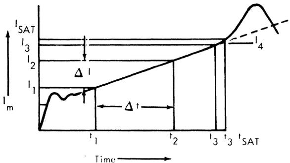
Figure 6-31. Magnetizing Current,  $I_{MAG}$  versus Time
