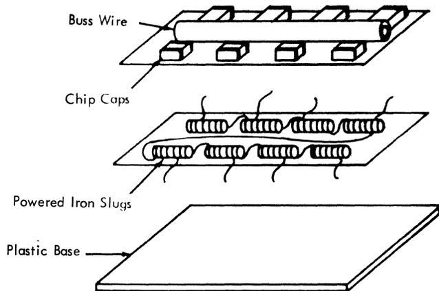
Figure 6-34. Typical Chip Capacitor Assembly
