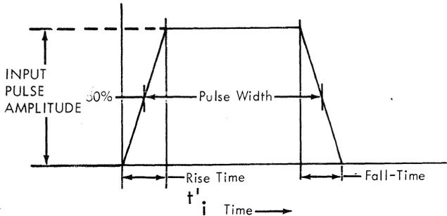
Figure 6-25. Typical Input Pulse Waveform and Characteristics
