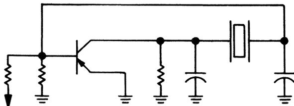
Figure 7-10B. Typical Transistor Sine Wave Oscillator Schematic
