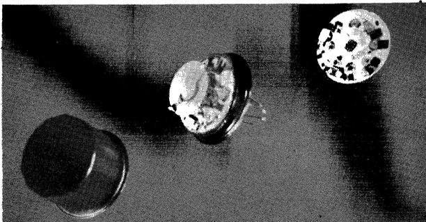
Figure 7-12. Sequence from Substrate to Final Package
