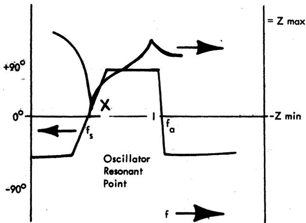
Figure 7-3. Frequency Performance of Crystal Resonator
