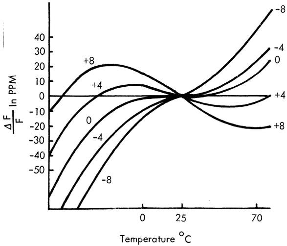
Figure 7-8. Frequency versus Temperature for an AT Cut Crystal (Theoretical)
