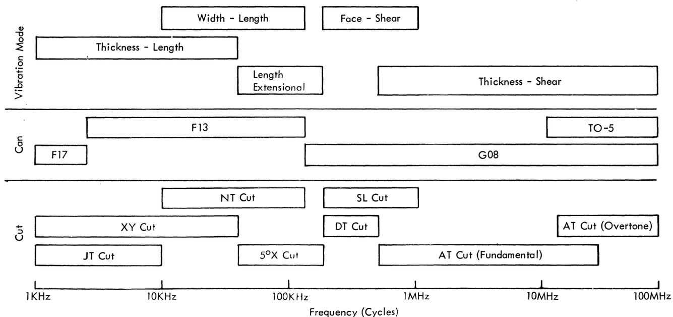
Figure 7-5. Frequency Range Versus Vibration Mode, Package Size, and Cut
