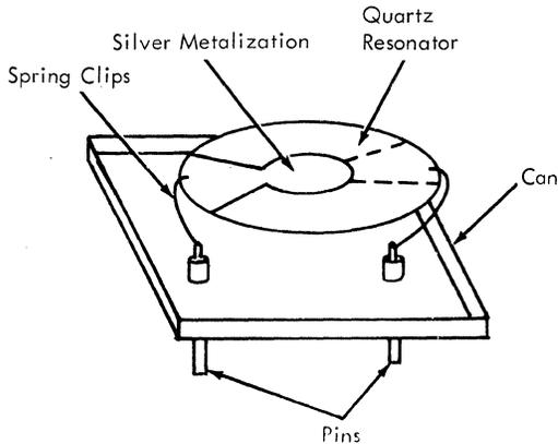
Figure 7-7B. Typical Construction (AT Cut)
