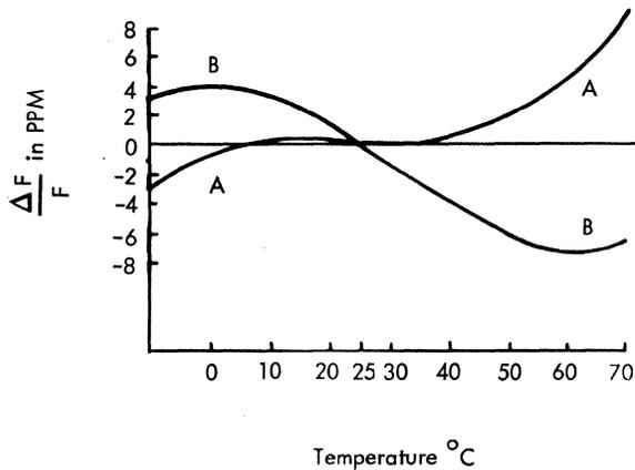
Figure 7-15. Frequency versus Temperature for Hybrid Oscillator (Experimental)
