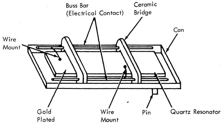
Figure 7-7A. Typical Construction (Non-AT Cut)
