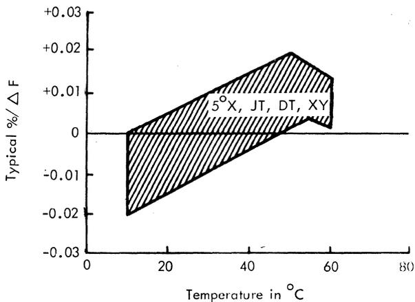
Figure 7-9. Typical Percent Change in Frequency versus Temperature, Non-AT-Cut
