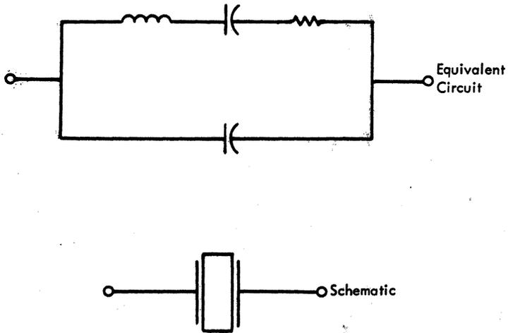
Figure 7-2. Crystal Resonator Equivalent Circuit and Schematic
