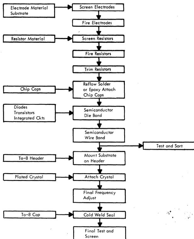
Figure 7-13. Generalized Process Flow Chart for Hybrid Oscillator
