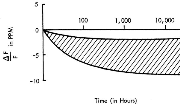
Figure 7-17. Oscillator Aging at 85°C
