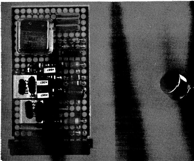
Figure 7-11. Size Relationship Between Printed Circuit Board Layout and Hybrid Package
