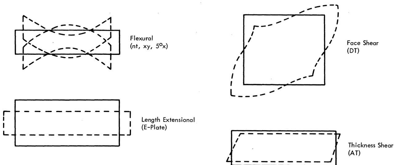
Figure 7-4. Vibration Modes for Various Crystal Cuts
