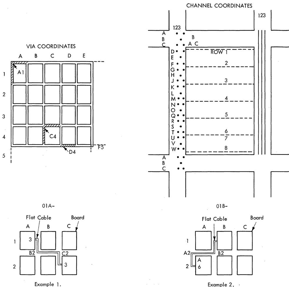
●Figure 21. Cable Routing
