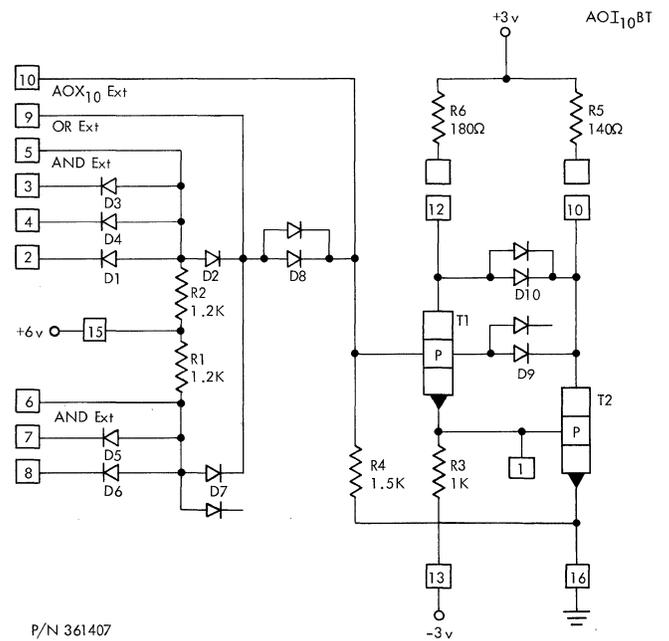
Figure 119. (AOI<sub>10</sub>BT) AND-OR-Inverter-Terminate, High-Speed
