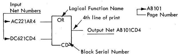
The line name is generally a description of the line function and is signed plus (+) or minus (-), depending upon the active condition of the line at that point. If most of the lines in the box are plus (+), the sign may not appear unless it is minus (-).
