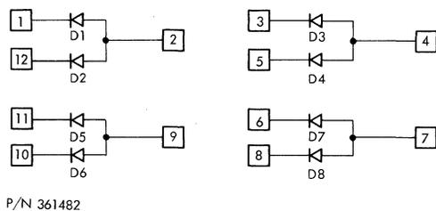
Figure 41. Four Double Diodes, High-Speed (FDD)
