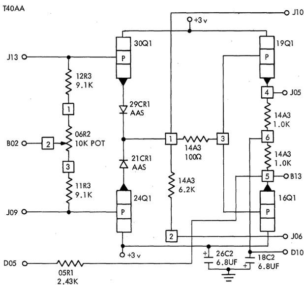
•Figure 109. T40AA, NPL Final Amplifier Rectifier and Channel Separator
