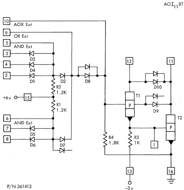
Figure 124. (AOI<sub>11</sub>BT) AND-OR-Inverter, High-Speed
