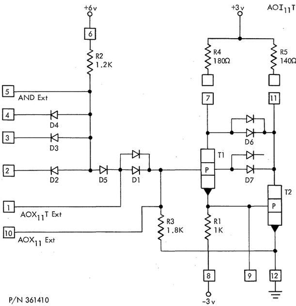
Figure 122. (AOI<sub>11</sub>T) AND-OR-Inverter-Terminate, High-Speed
