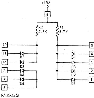
Figure 34. AND-OR-Power-Extender, Low-Speed (AOPX-1)
