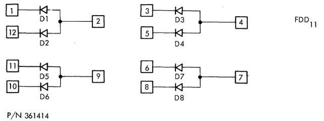
Figure 125. (FDD<sub>11</sub>) Four Double Diodes, High-Speed
