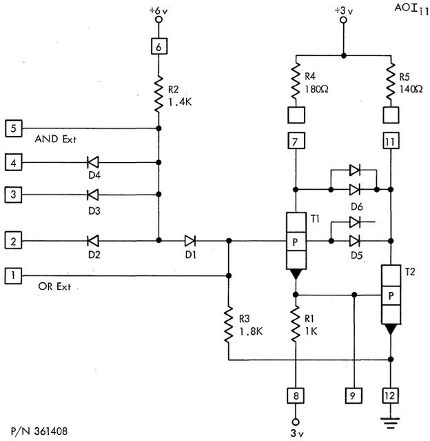
Figure 120. (AOI<sub>11</sub>) AND-OR-Inverter, High-Speed
