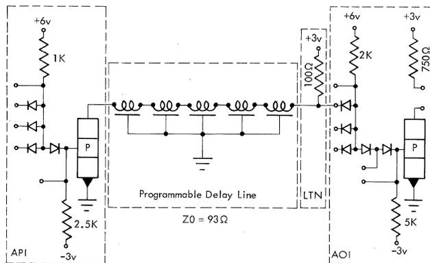
Figure 65. Delay Line Driver and Terminator (DLD)
