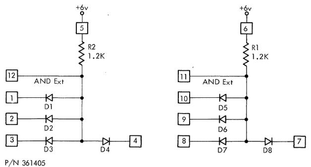
Figure 40. AND-OR-Extender, High-Speed (AOX<sub>10</sub>T)
