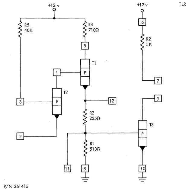
Figure 126. (TLR) Transmission Line Receiver, Low-Speed
