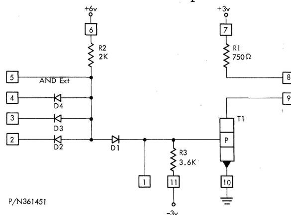
•Figure 27. AND-Inverter, Medium-Speed (AI)
