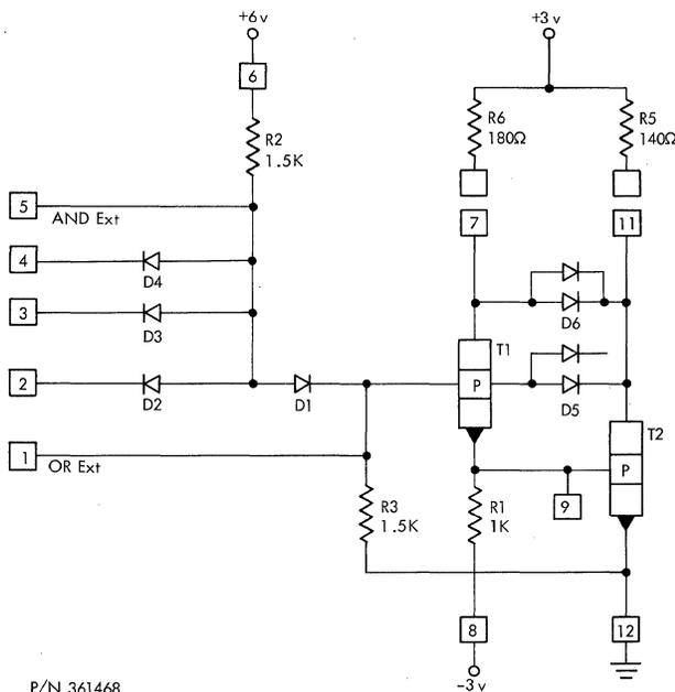
Figure 37. AND-OR-Inverter, High-Speed (AOI<sub>10</sub>)
