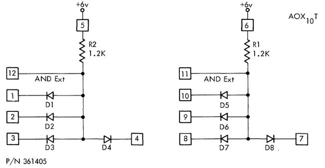
Figure 117. (AOX<sub>10</sub>T) AND-OR-Extender-Terminate, High-Speed
