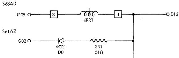
Figure 113. S63AD, Coil Six-Pole Reed Relay
