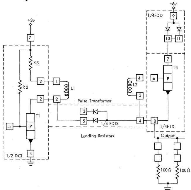
Figure 70. Sample Pulse Driver, Medium-Speed (SPD)
