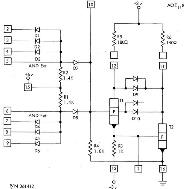
Figure 123. (AOI<sub>11</sub>B) AND-OR-Inverter (Two-Way OR), High-Speed
