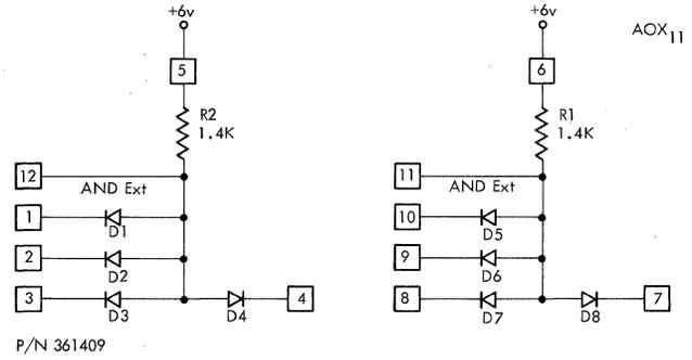
Figure 121. (AOX<sub>11</sub>) AND-OR-Extender, High-Speed
