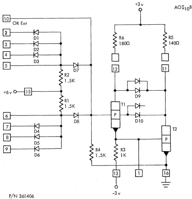
Figure 118. (AOI<sub>10</sub>B) AND-OR-Inverter, High-Speed
