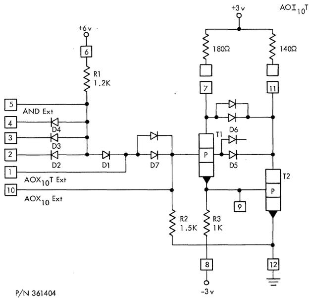
Figure 116. (AOI<sub>10</sub>T) AND-OR-Inverter-Terminate, High-Speed
