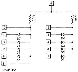
Figure 33. AND-OR-Extender, Medium-Speed (AOXB)
