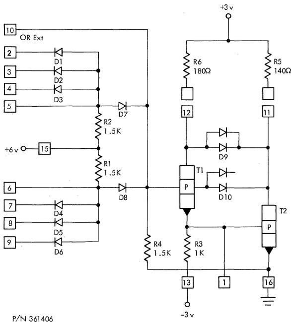
Figure 38. AND-OR-Inverter, High-Speed (AOI<sub>10</sub>B)
