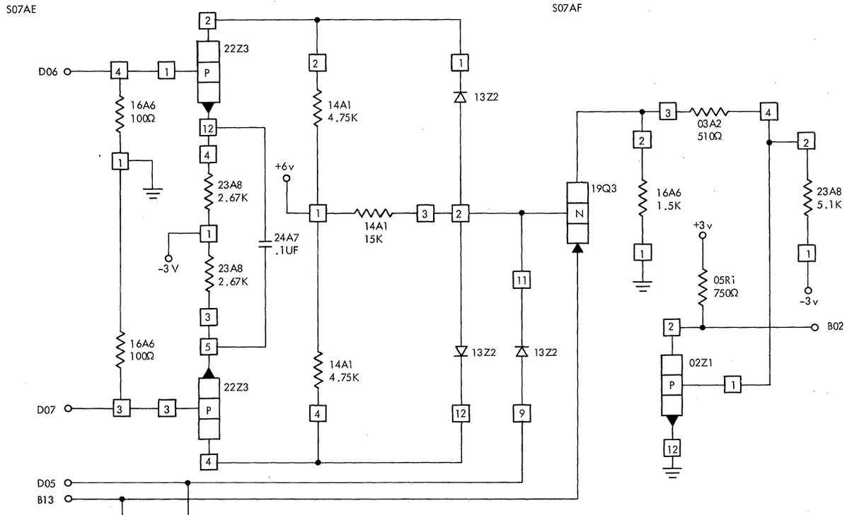
Figure 97. S07AE, Sense Amplifier 2 Part B
