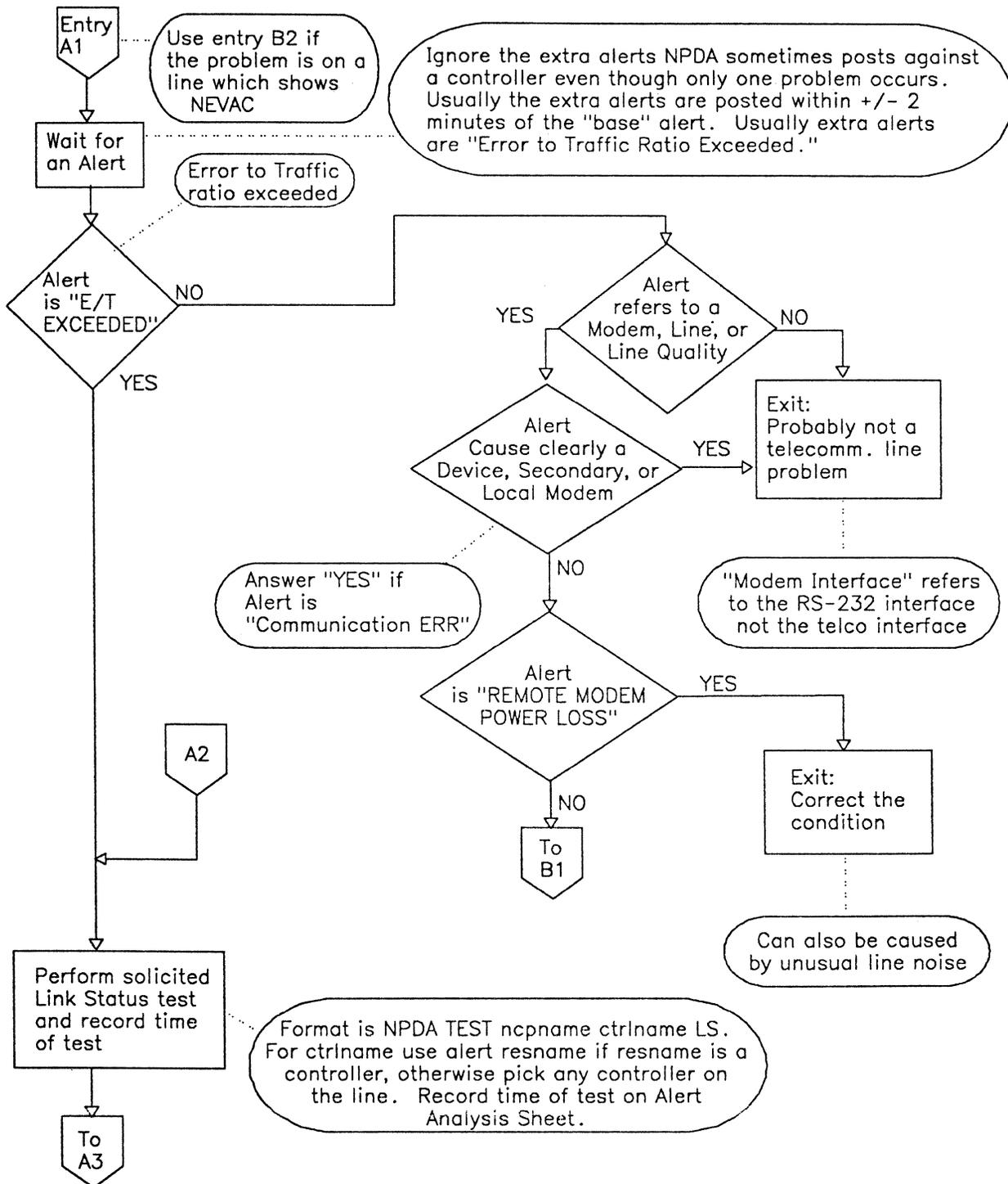
Figure 4. Chart A - Alert and LS Test Screening
