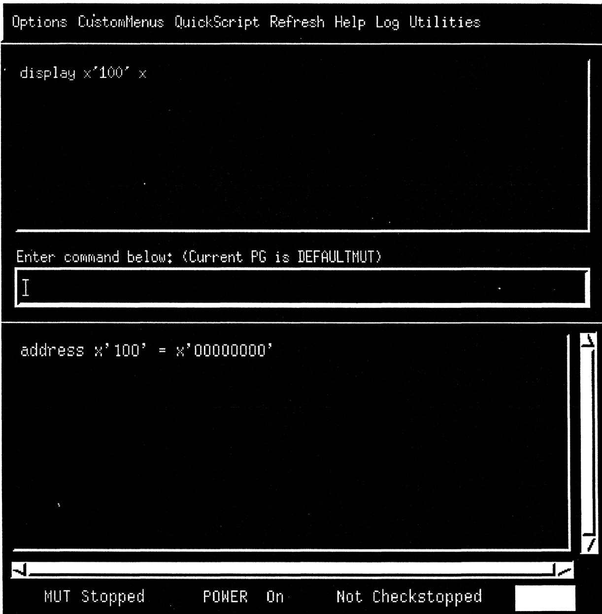
ESP has a Motif Window Interface. The first thing the user sees when ESP is executed is the console window. (See Figure 1.) This X-Window is comprised of five sections: The Menu Bar at the top, the Command History List just below, followed by the Command Line, the TTY Section, and finally the MUT Status.
