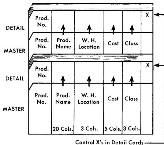
Figure 38. Automatic Coding by Gangpunching
