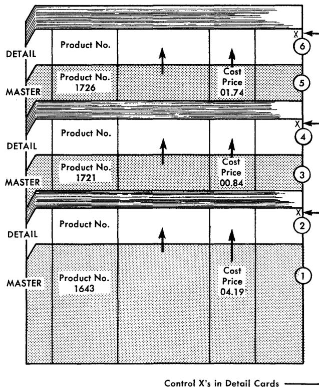
Figure 37. Automatic Pricing by Gangpunching
