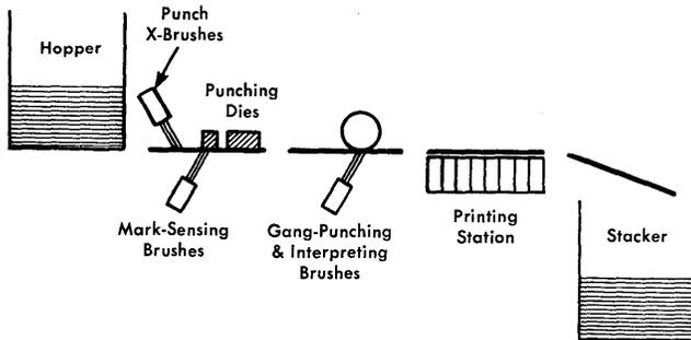
Figure 21. Sketch of Punch Feed with Printing Station
