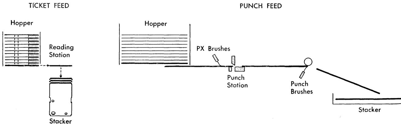
Figure 51. Schematic of Ticket and Punch Feeds
