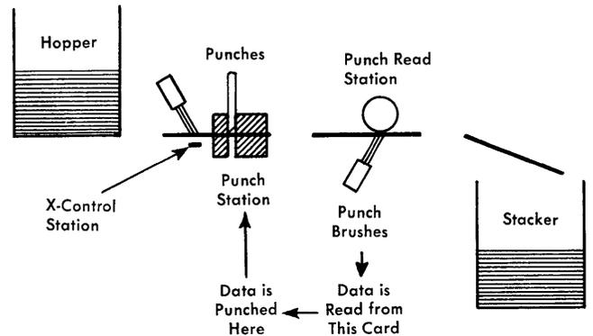
Figure 29. Schematic of Gangpunching
