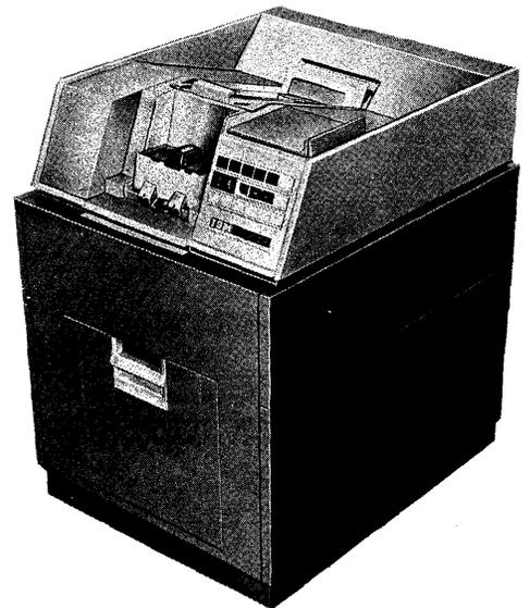
Figure 58. IBM 542 Card Read Punch
