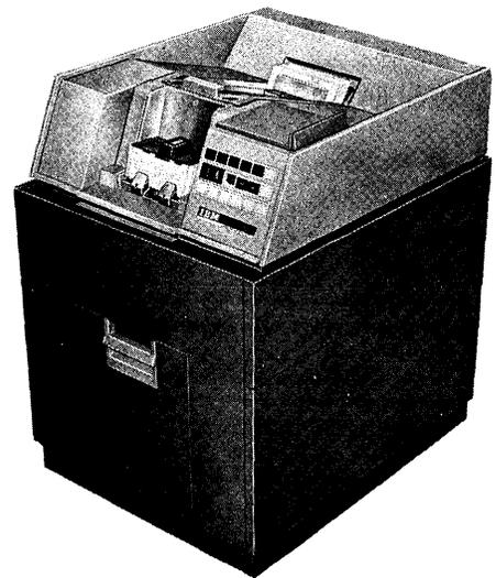
Figure 57. IBM 541 Card Read Punch
