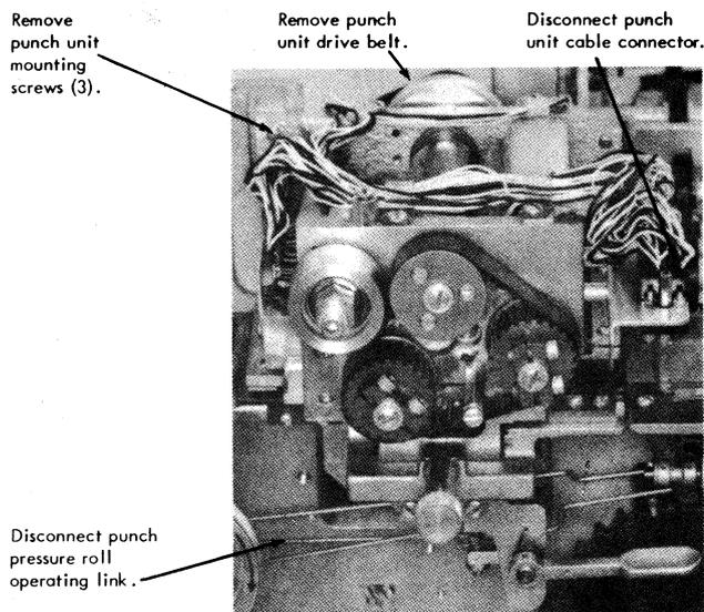
Figure 4-36. Punch Unit Removal
