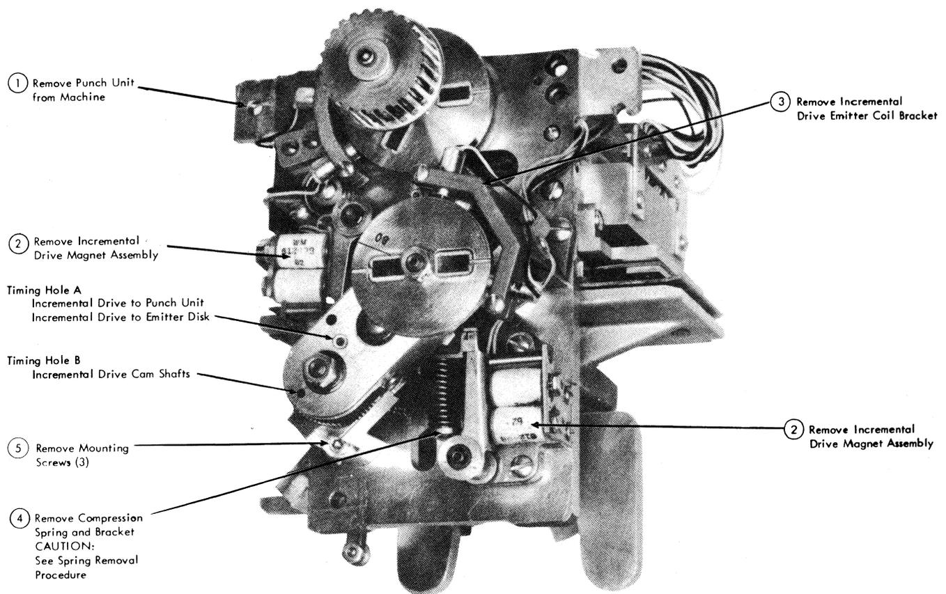
Figure 4-49. Incremental Drive Unit Removal
