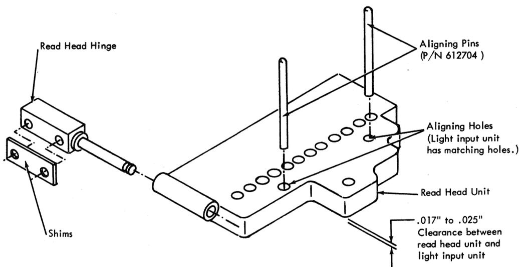
● Figure 4-16. Read Head Unit Adjustment
