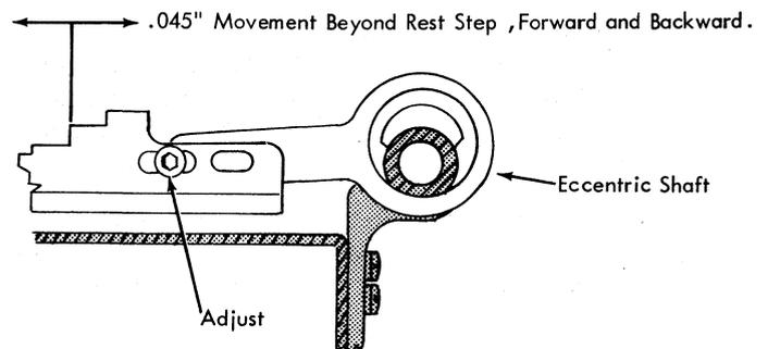
Figure 4-33. Joggler Operating Arm Slide (Isolated)
