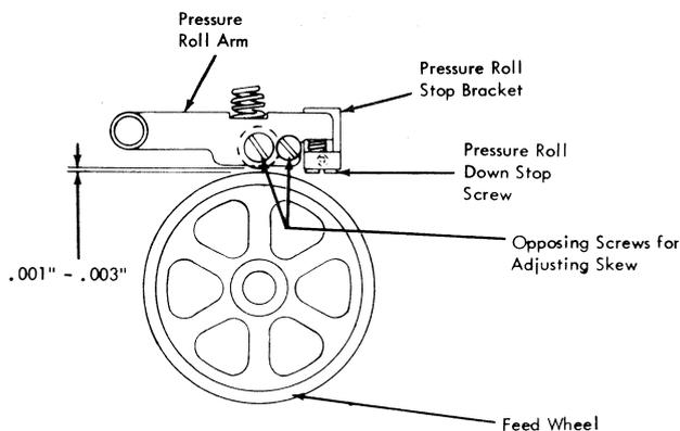
Figure 4-39. Downstop Adjustment
