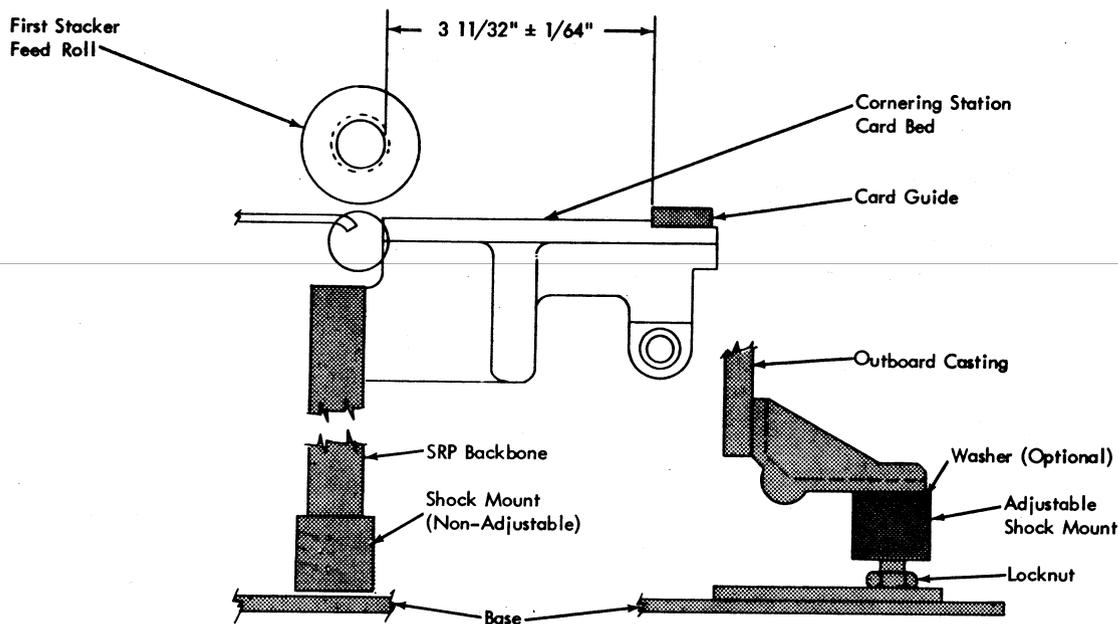
Figure 4-34. Stacker Alignment
