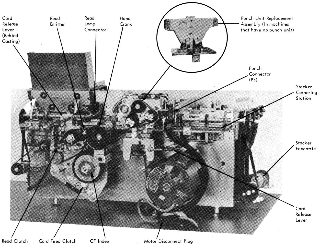
Figure 5-2. Serial Reader Punch, Rear View
