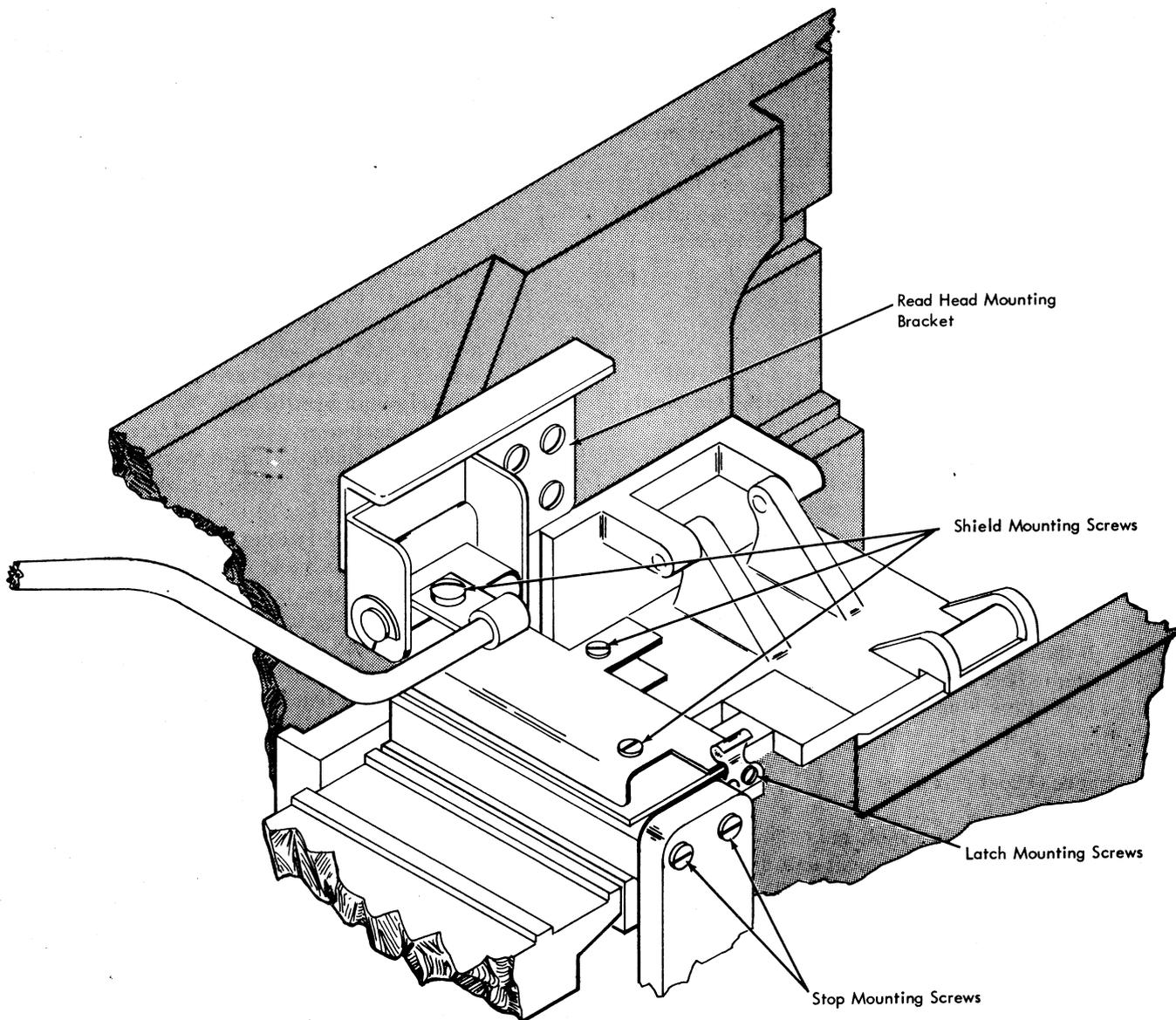
Figure 4-17. Front Mounted Read Head
