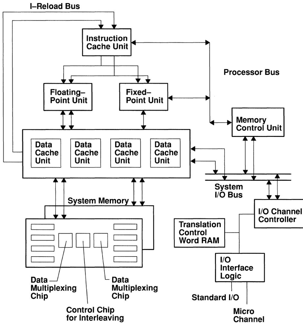
Figure 1. The RISC System/6000 Central Electronics Complex for the Model 530, Model 540, Model 730, and Model 930.
