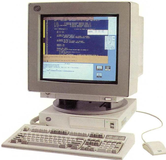
Figure 7. The Xstation 120 shown here consists of a 101-key keyboard, a 3-button mouse, and an optional 6091 Color Display, Model 19.
