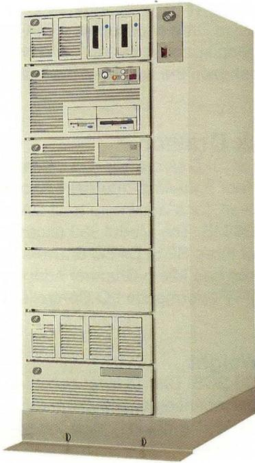
Figure 6. The rack-mounted Model 930 system unit with optional Async Expansion Drawer and SCSI Disk Drawer.
