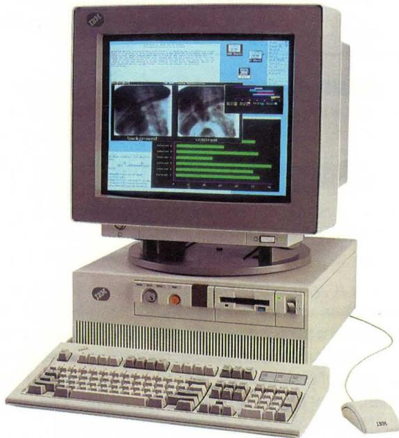
Figure 3. The desktop Model 320 with an optional 6091 Color Display, Model 19, and optional keyboard and mouse.
