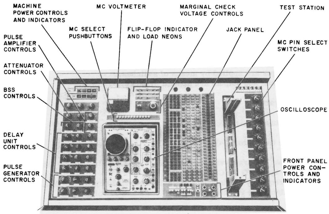
Figure 6-9. Tester, Front Panel
