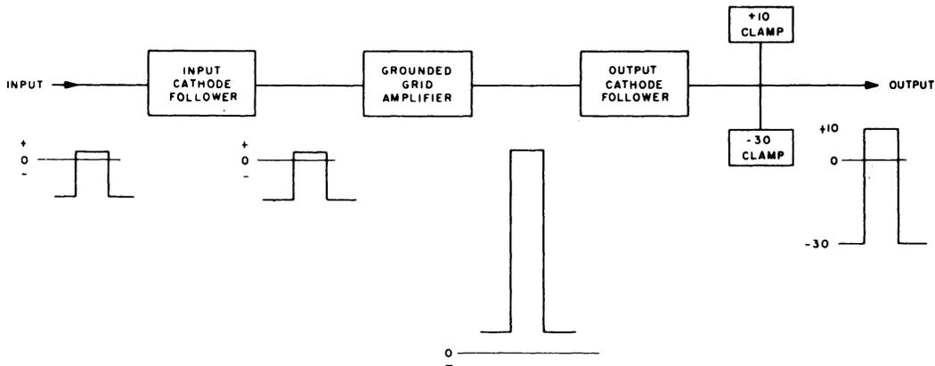
Figure 4-35. D-C Level Setter, Block Diagram
