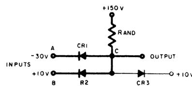
Figure 4-16. Two Way AND Circuit
