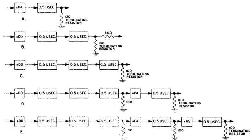
Figure 4-60. Typical Arrangements of Delay Units
