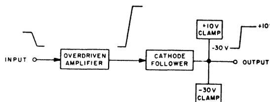
Figure 4-42. D-C Inverter, Simplified Block Diagram
