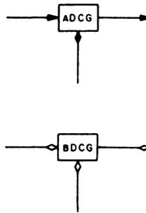
Figure 4-62. Diode Capacitor Gate, Models A and B, Logic Block Symbols
