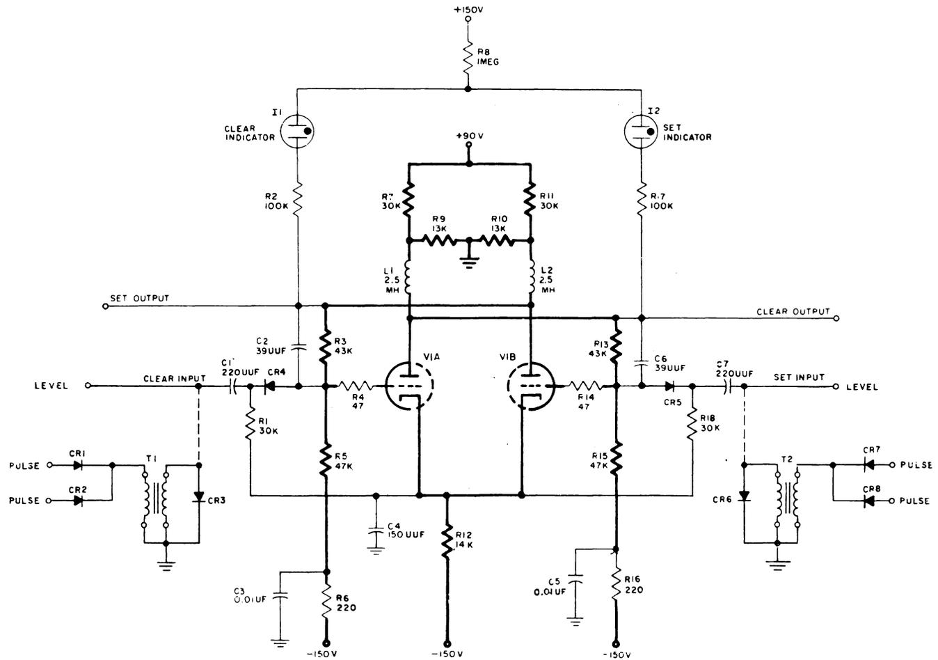
Figure 4-45. Flip-Flop, Model B, Schematic Diagram
