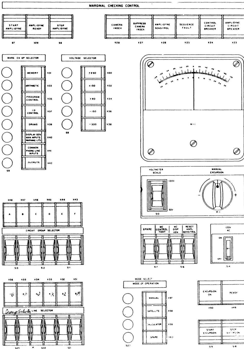
Figure 7-27. Module "H" Duplex Maintenance Console
