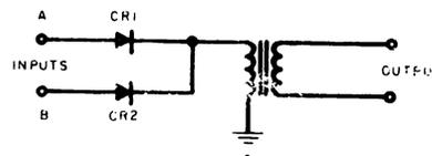
Figure 4-20.  $Y_{OR}$  Circuit Schematic Diagram
