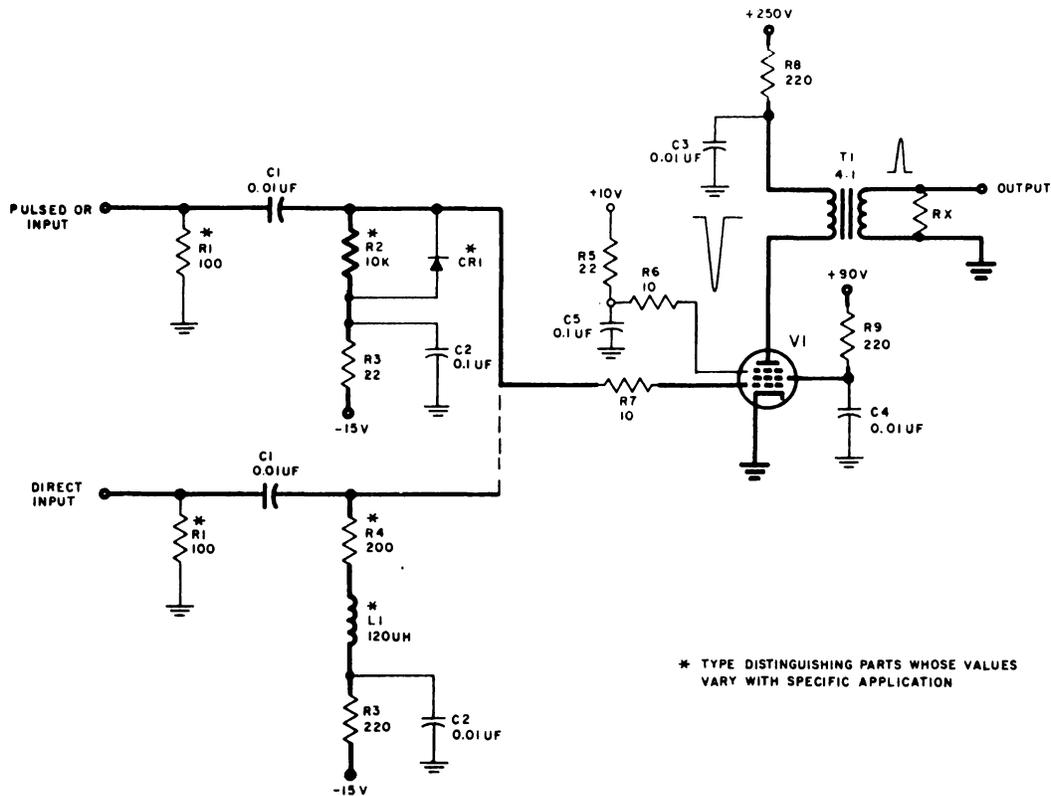
Figure 4-24. Pulse Amplifier, Model A, Schematic Diagram
