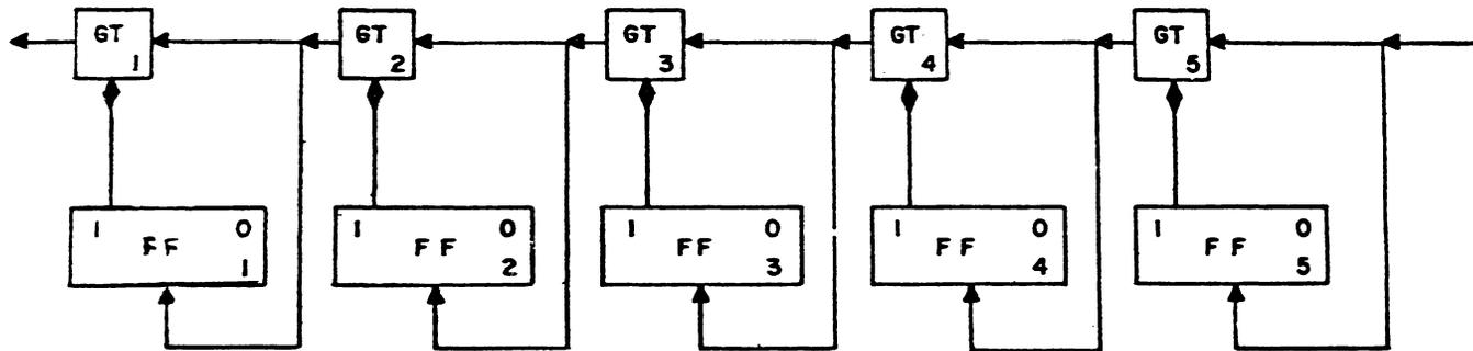
Figure 5-7. 5 Stage Flip Flop Counter
