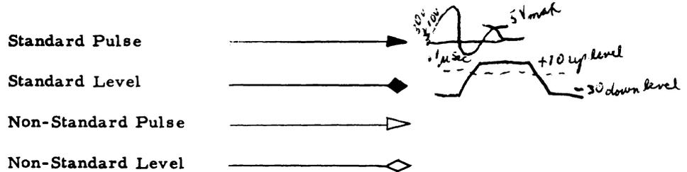
Figure 4-3. Logic Representation of Pulses and Levels
