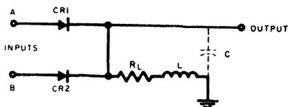
Figure 4-19. Pulsed OR Circuit Schematic Diagram
