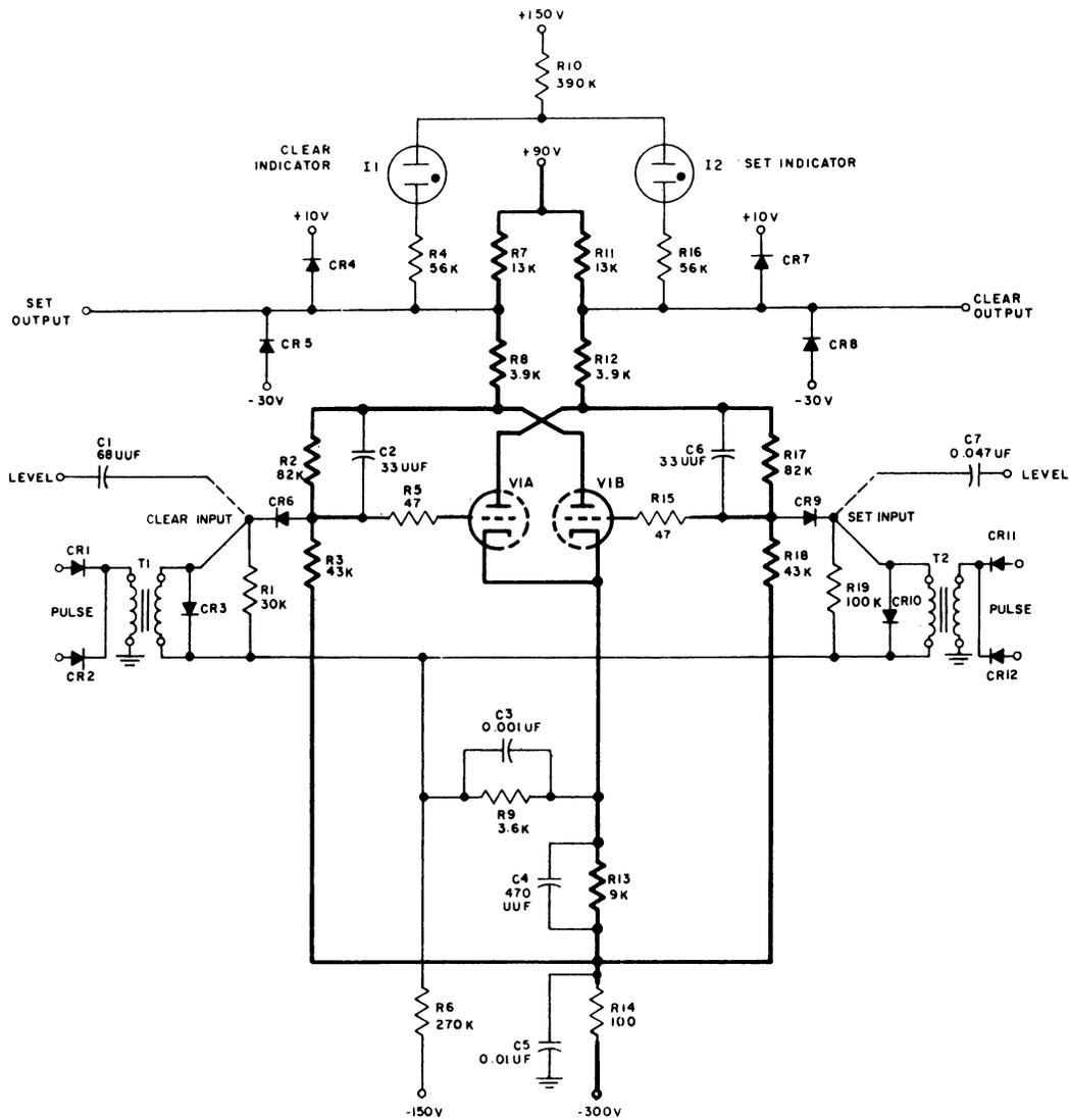
Figure 4-46. Flip-Flop, Model C, Schematic Diagram
