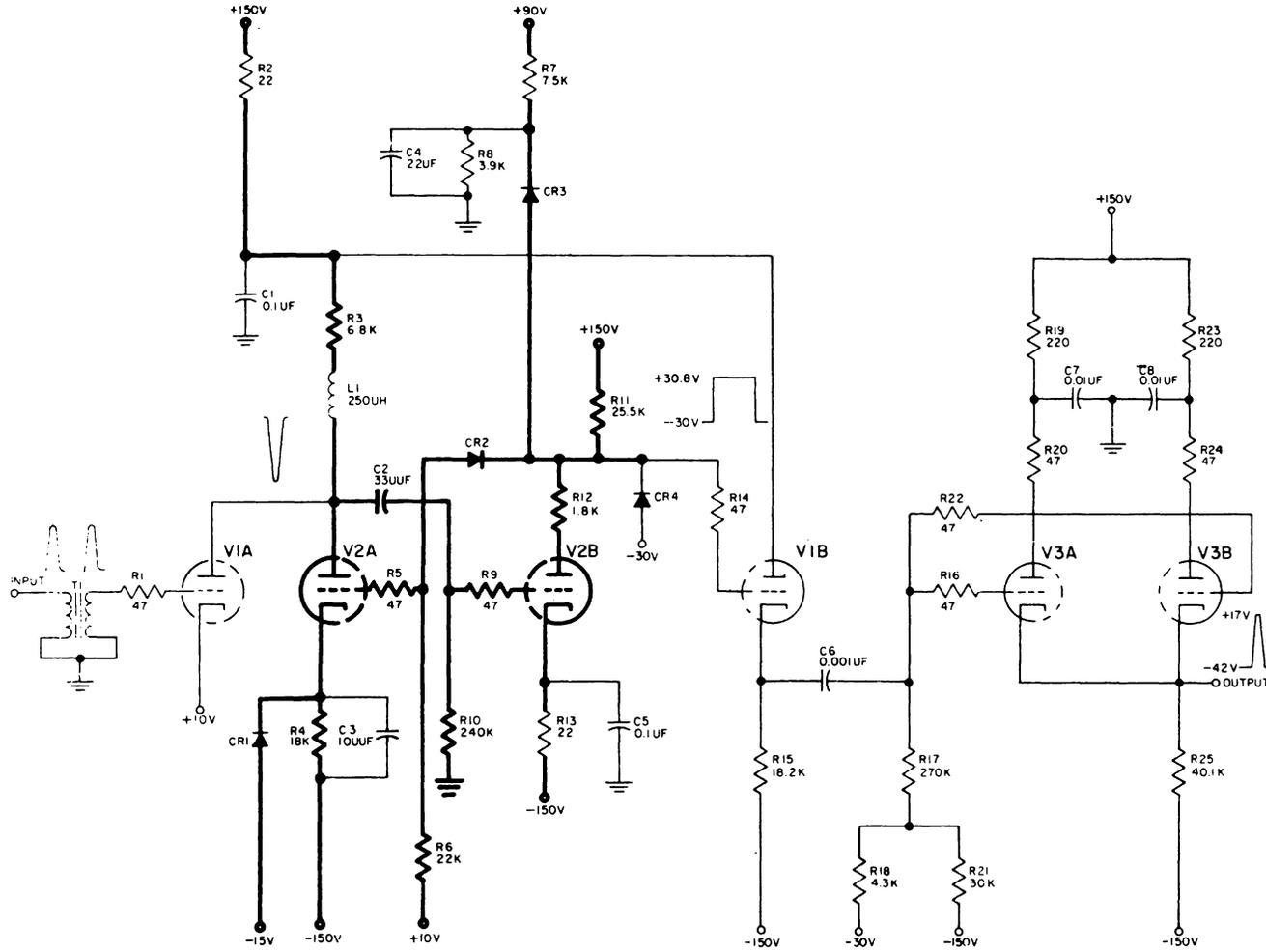
Figure 4-55. Single-Shot, Model D, Schematic Diagram
