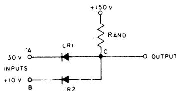
Figure 4-15. Two Way AND Circuit
