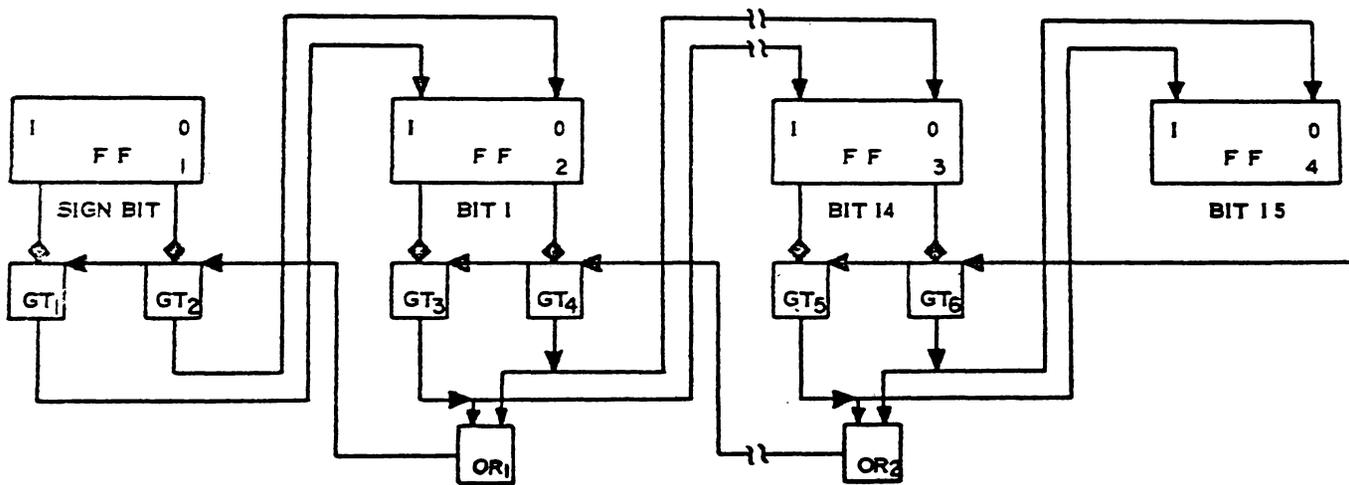
Figure 5-6. Ripple Shift Right
