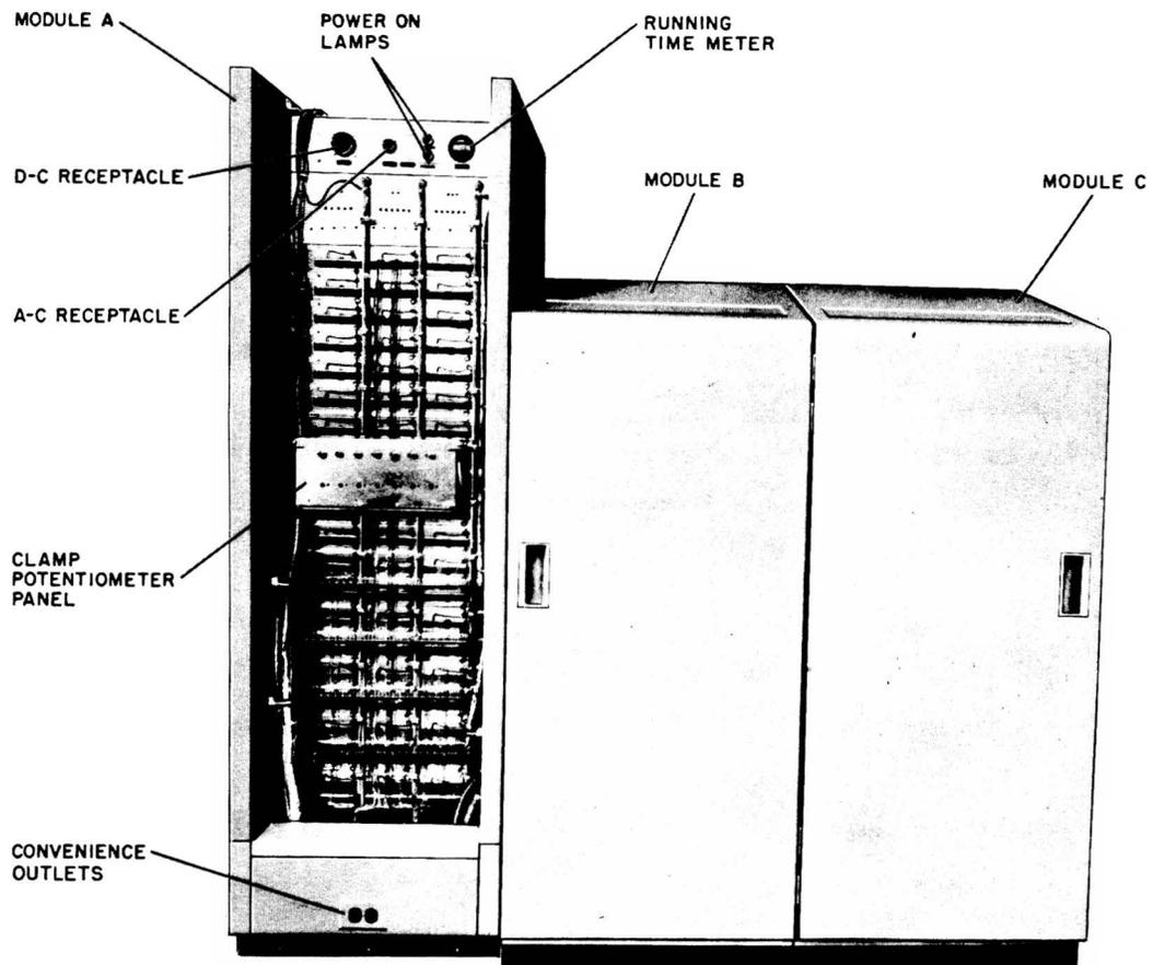
Figure 6-7. Tester, Rear View
