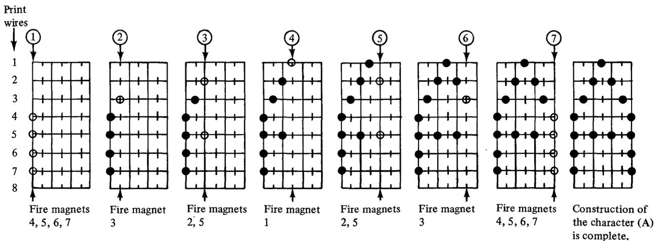
This illustrates how the character A is formed by firing a combination of 7 print wires within a matrix (a character position). The numbers of the print wires are shown at the far left. The sequence of firing positions, within the matrix is shown from left-to-right across the page. Note that no magnet is fired in successive firing positions.
