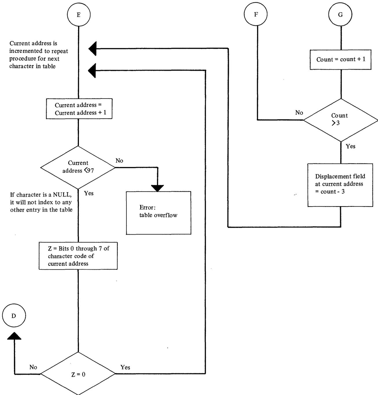
Figure C-2 (Part 3 of 3). Flowchart for calculating displacement fields for characters in the Wire Image Table
