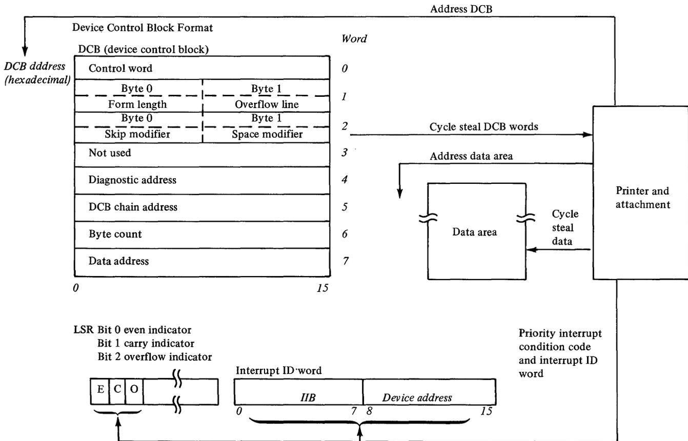
**Note.** DCB format is shown for a start command. The DCB format for a start cycle steal status command appears later in this chapter.
