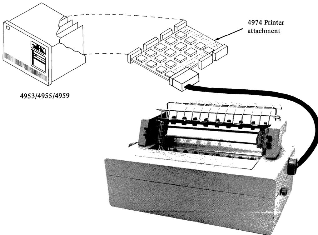
Figure 1-1. IBM Series/1 4974 Printer and attachment card
