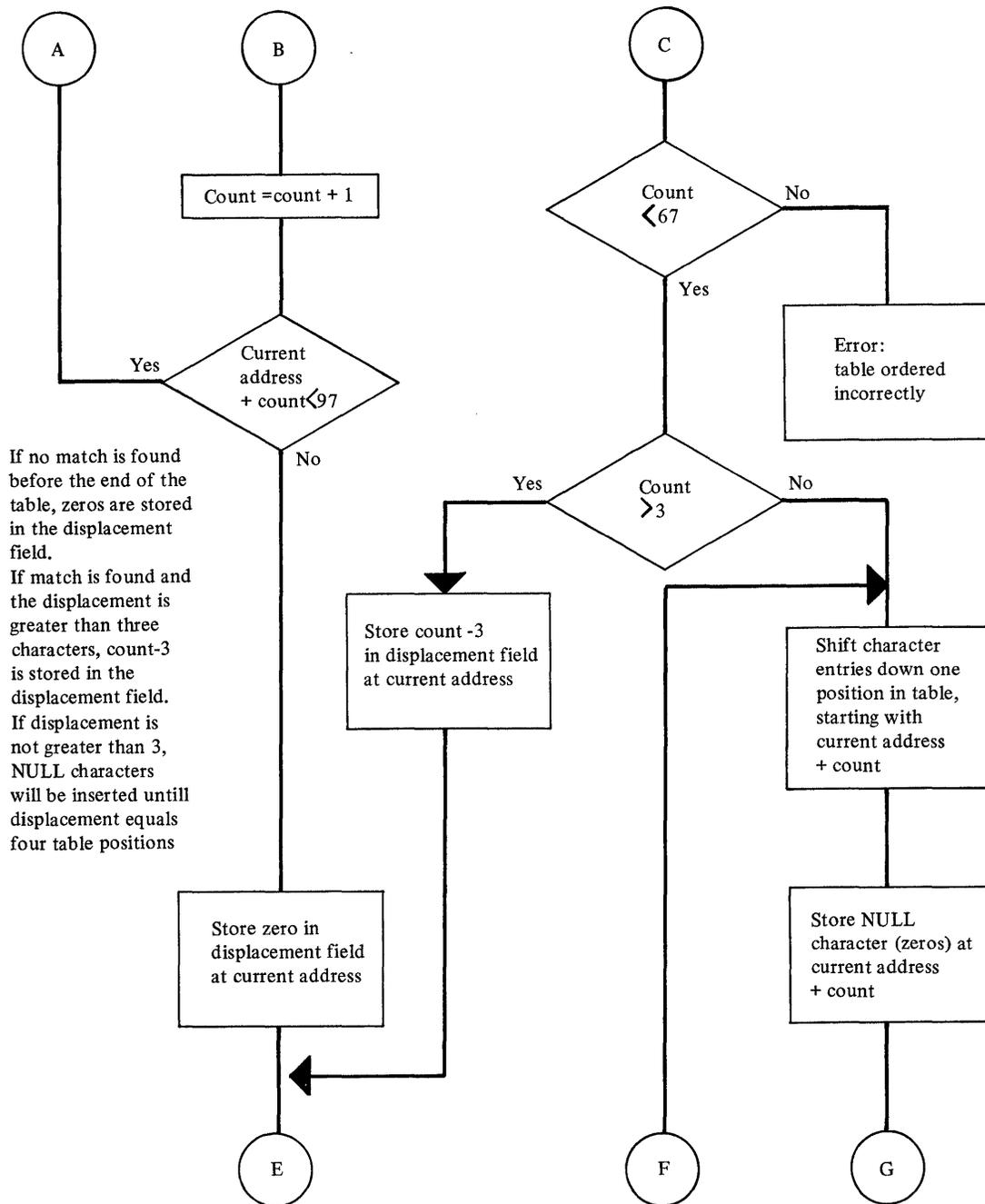
Figure C-2 (Part 2 of 3). Flowchart for calculating displacement fields for characters in the Wire Image Table
