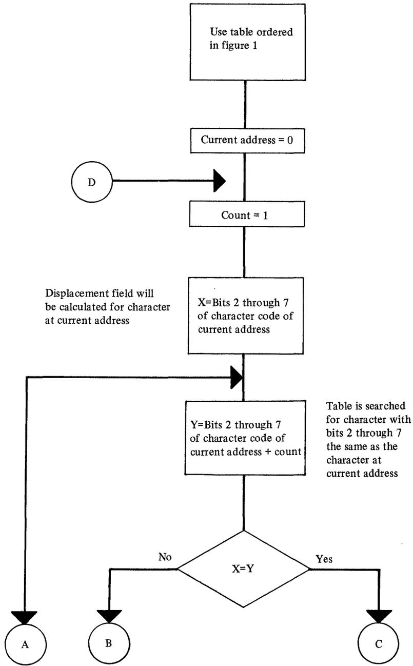
Figure C-2 (Part 1 of 3). Flowchart for calculating displacement fields for characters in the Wire Image Table
