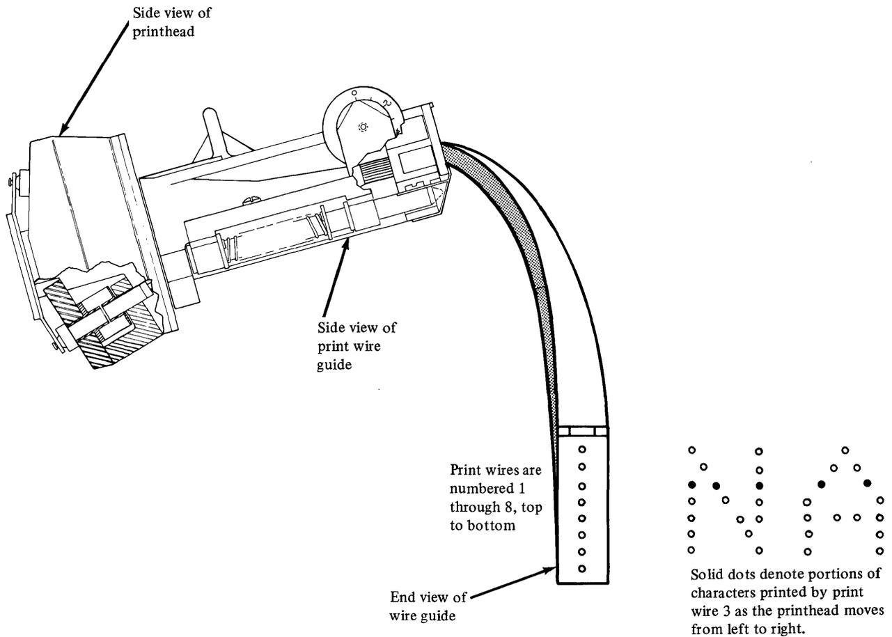
Figure 1-2. Printhead and printwires
