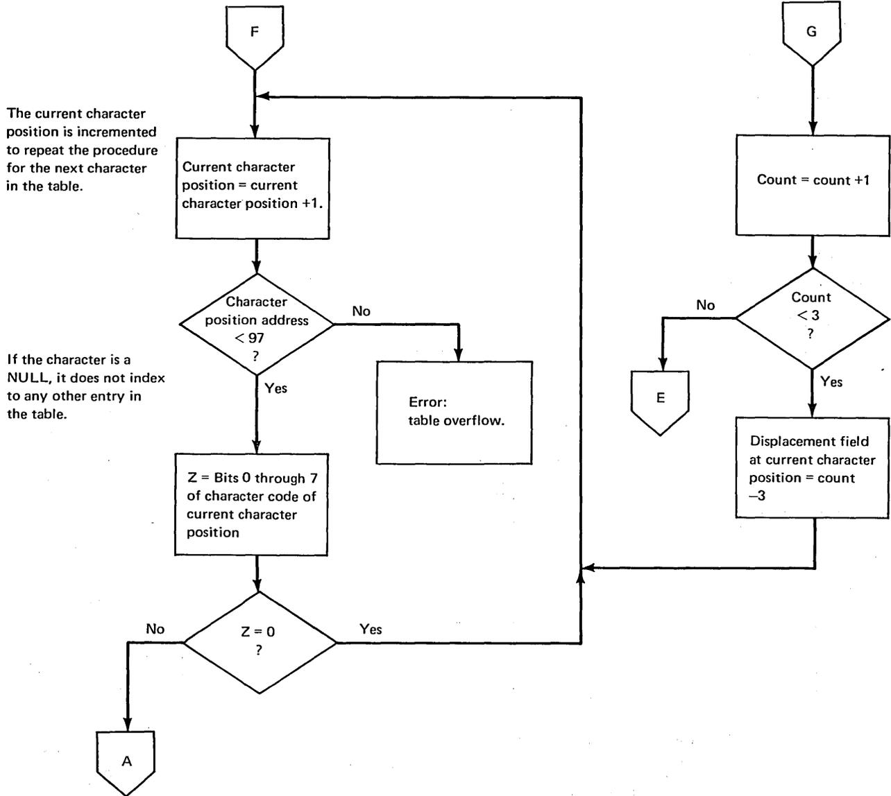
Figure 2-14 (Part 3 of 3) Flowchart for calculating displacement fields for characters in the wire-image table
