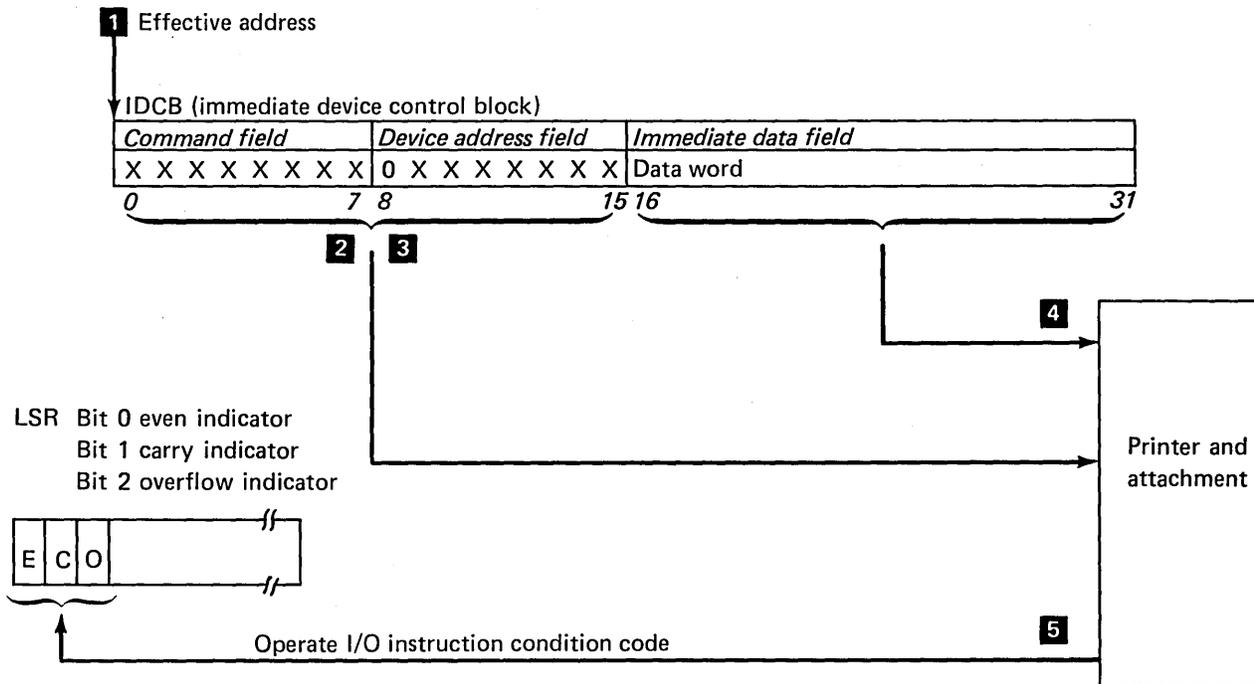
Figure 2-2. Direct program control (DPC) operation
