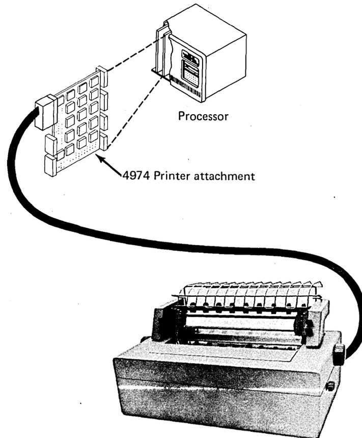
Figure 1-1. IBM Series/1 4974 Printer and attachment feature card
