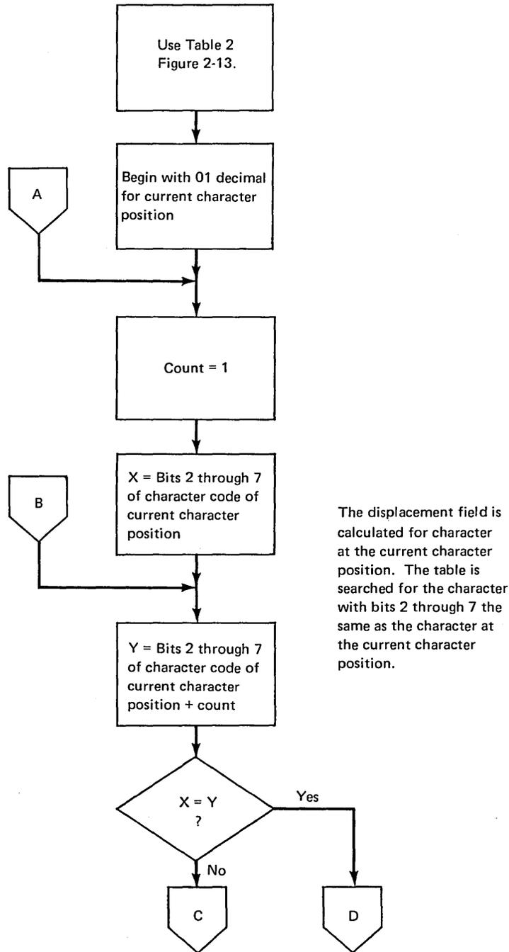
Figure 2-14 (Part 1 of 3). Flowchart for calculating displacement fields for characters in the wire-image table
