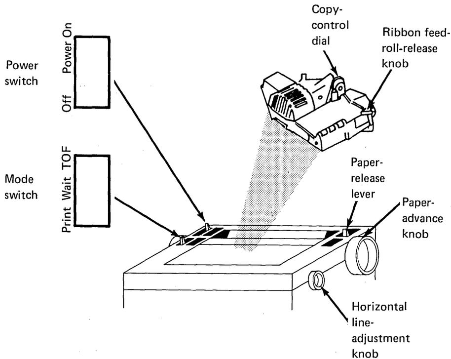
Figure 1-5. Printer controls
