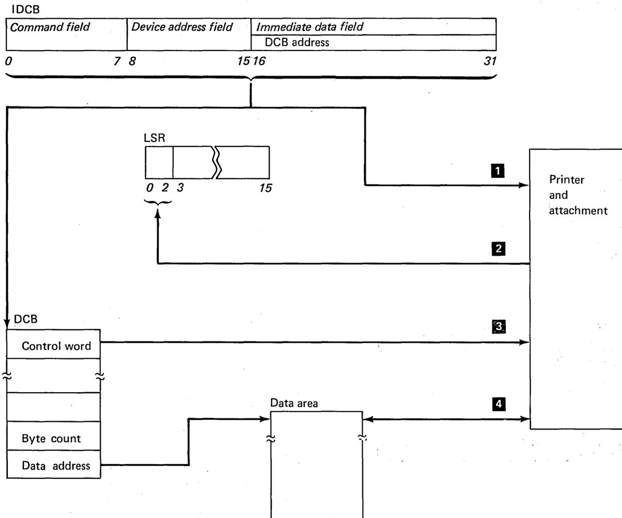
Figure 2-3. Cycle-steal operation
