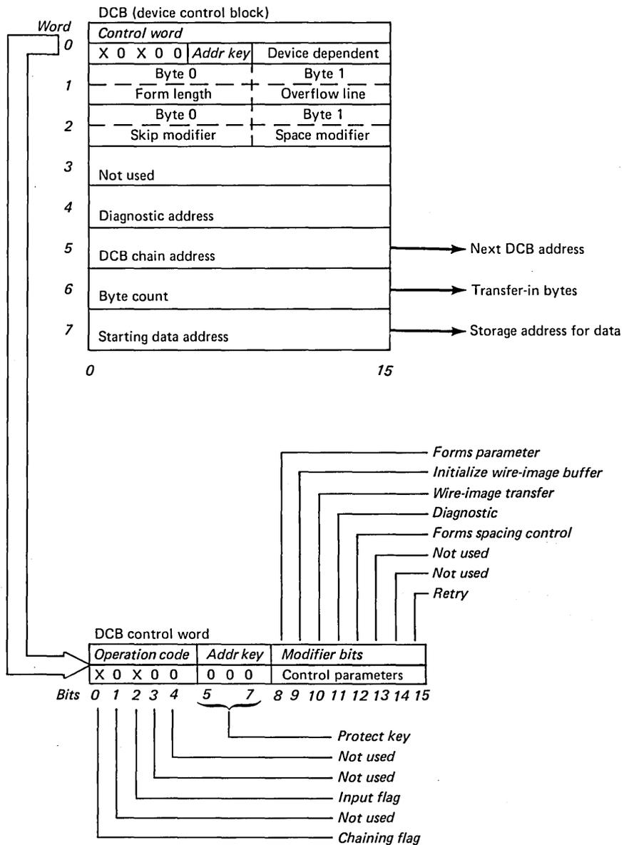
Figure 2-4. Device control block
