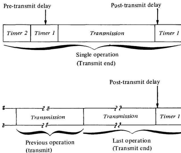
**Transmit Allow Break.** This operation is the same as the *Transmit* operation, except that it allows the receiving station to stop the transmission. To do this, the receiving station “breaks” the line for at least 150 milliseconds. If the attachment detects this condition, it resets transmit mode and ‘request to send’, and presents an exception interrupt with bit 0 on in the Interrupt Status Byte. The attachment does not reset RTS if it is permanently jumpered “on.”
