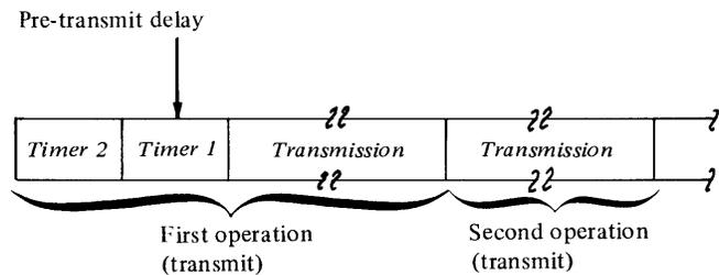
*Note.* Timer 1 should be set for a pre-transmit delay of approximately six milliseconds when the receiving station is a program controlled device and is directly connected or connected through a full-duplex modem.
