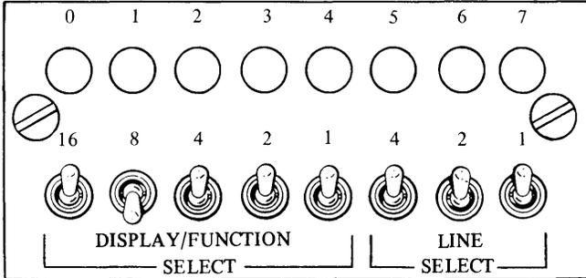
The indicator panel may be used with any of the communications features one at a time. The panel's cable plugs into a connector on a feature control card, and the panel can be moved between processor units and I/O expansion units. Therefore, it is not necessary to have more than one indicator panel. The panel does not attach to the 4953 models A and C.
