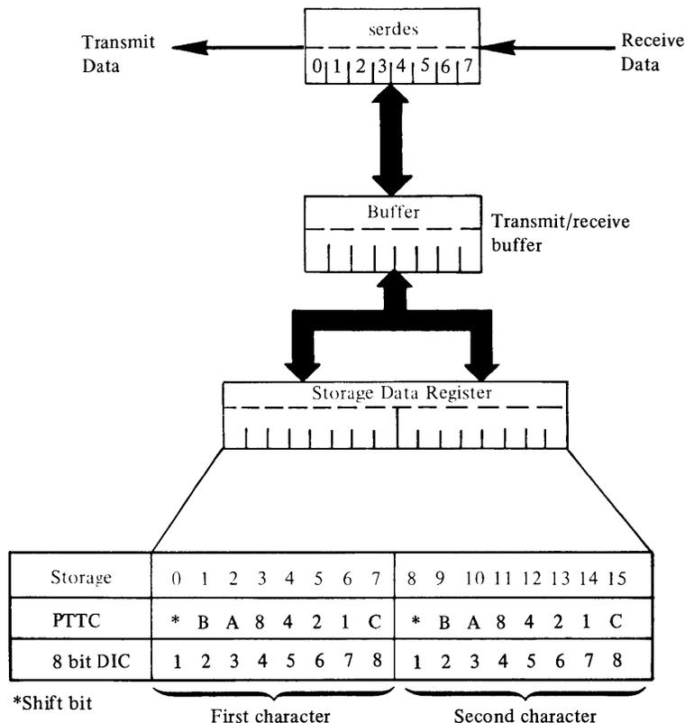
Figure 2-1. ACC feature data flow
