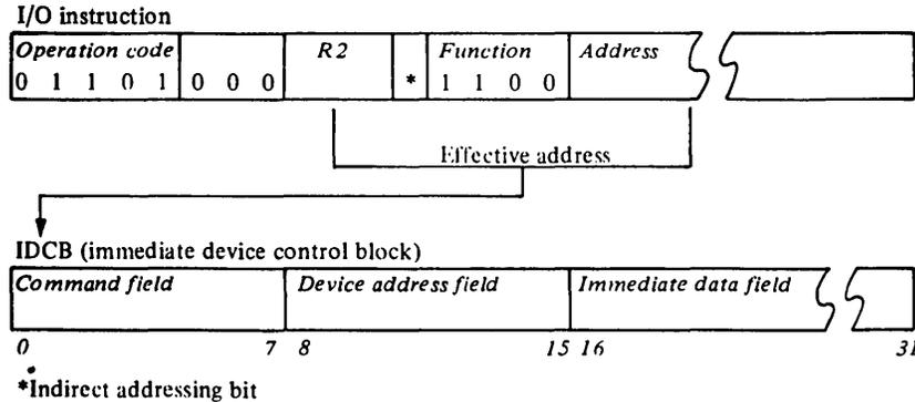
The address field (bits 16–31) and the contents of the register specified in the R2 field (bits 8–10) of the Operate I/O instruction generate an effective address that points to a main-storage location containing an immediate device control block (IDCB). IDCBS are doubleword blocks of storage reserved by programs for storage of device-directed commands.
