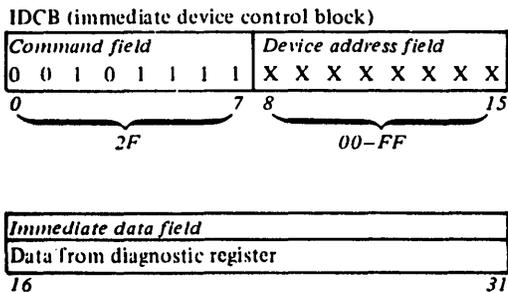
The Read Diagnostic Data command transfers the 16 bits from from the diagnostic register into the immediate data field of the IDCB. The diagnostic register is not reset.
