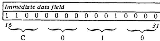
The Read ID (identification) command transfers a one-word identification field, called the DI ID word, into the immediate data field of the IDCB. The hexadecimal value of the integrated digital I/O feature DI ID word is C010. The device-identification word contains a unique identification code and physical information about the device, and can be used to determine the devices that are attached to the system.
