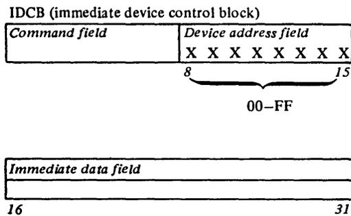
Bits 8–14 address the attachment card. Individual timer addresses are selected at installation time. These addresses are programmed on the cards by field-installable connectors (jumpers). These jumpers allow any 7-bit address (using bits 8–14) to be selected.
