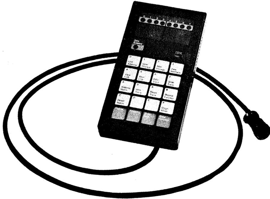
**Figure 7-8. 4990 Model 1 Communications Console for the 4987**
