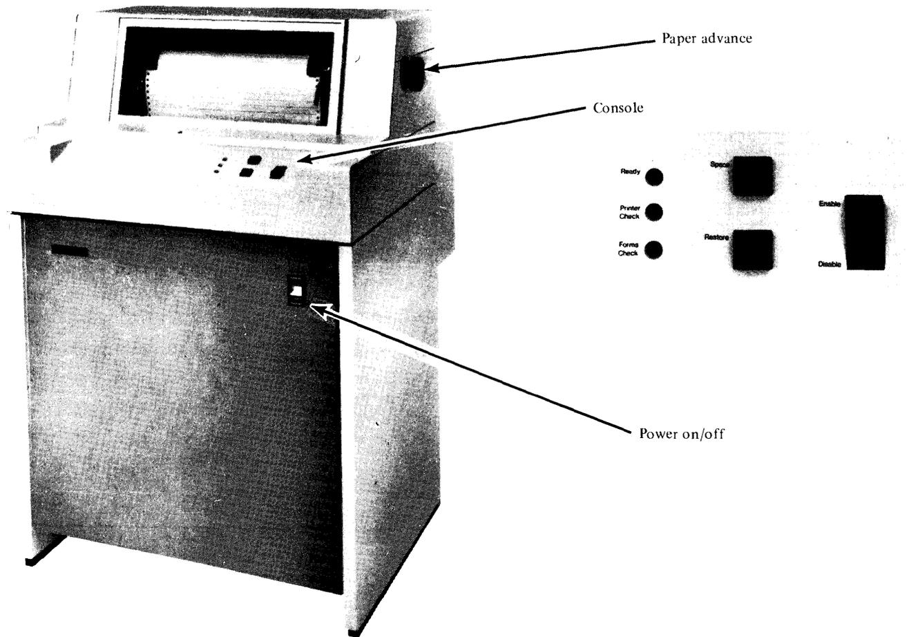
Figure 1-3. Printer Console
