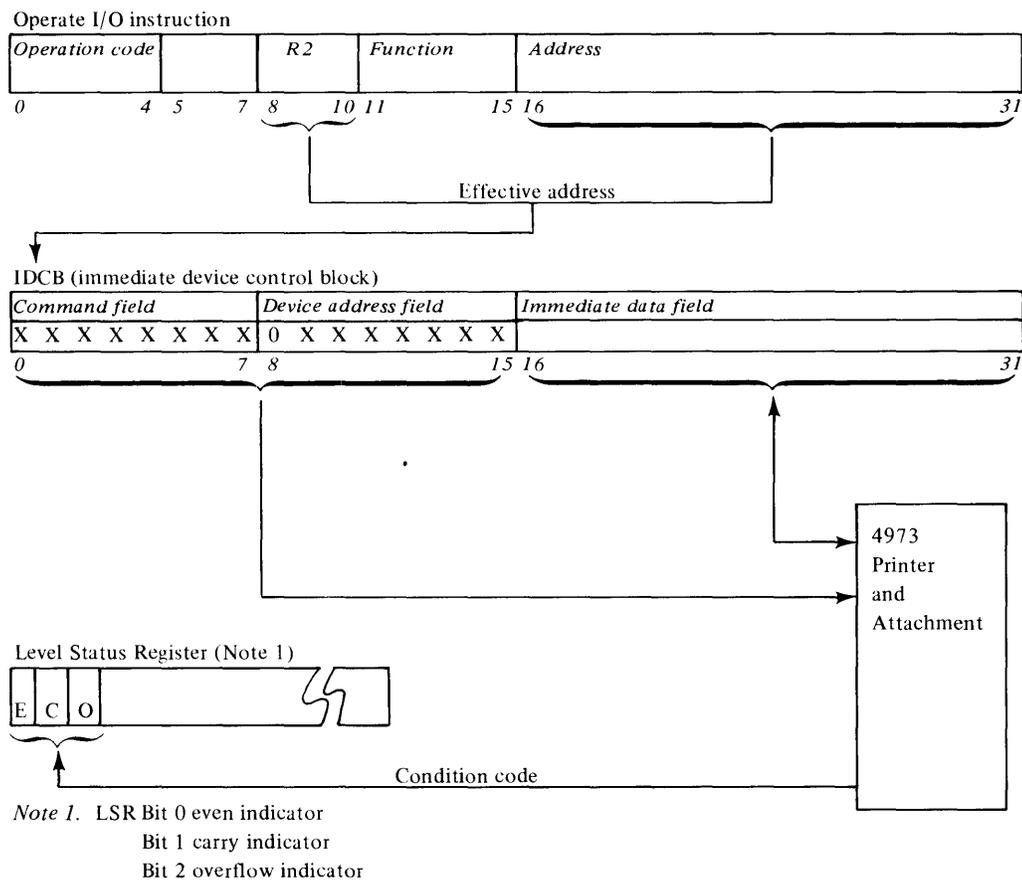
Figure 2-4. Direct Program Control I/O Operation
