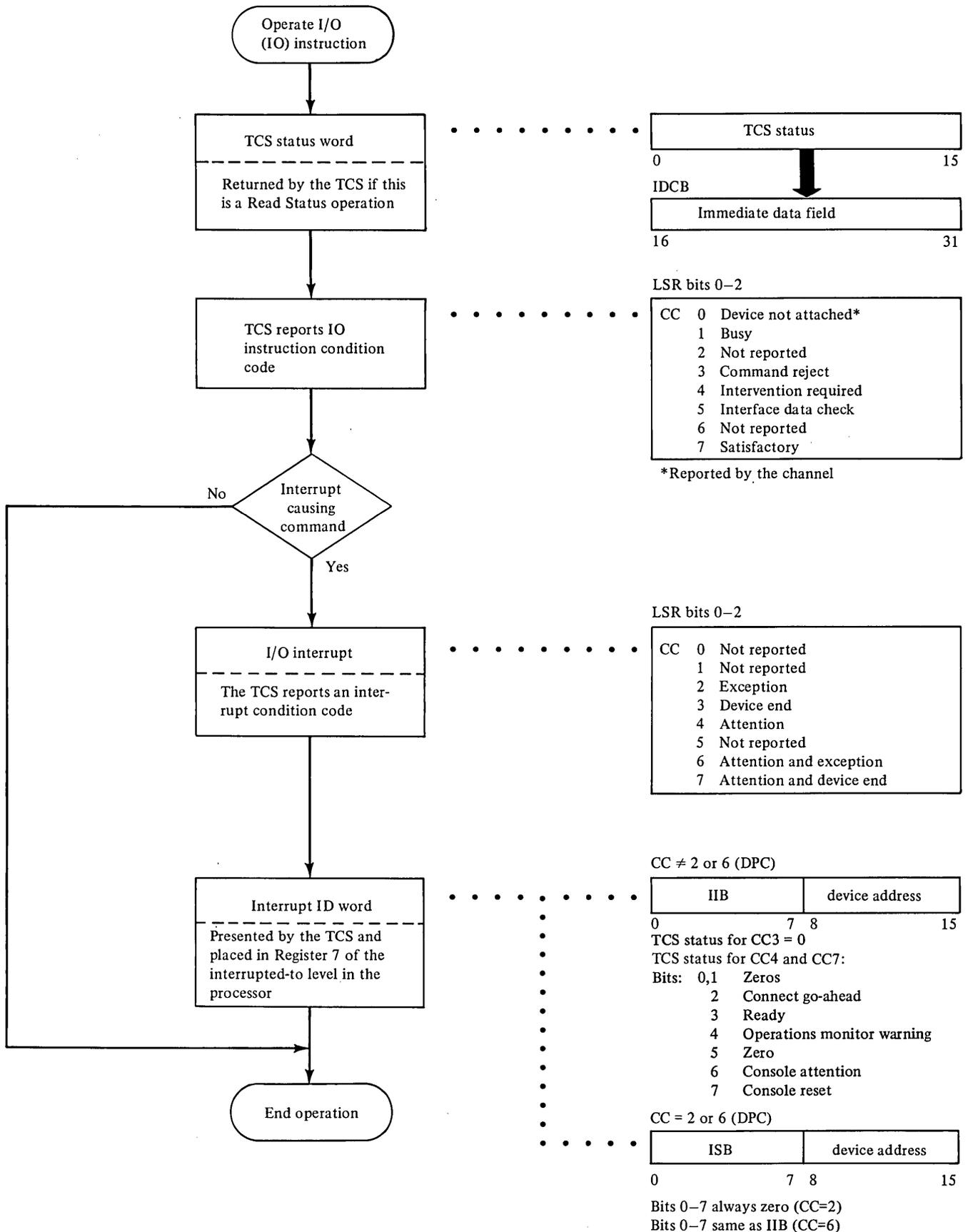
Figure 2-4. Condition codes and status sent to processor
