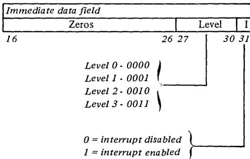
A priority interrupt level is assigned to the TCS by the *level* field. The I-bit (device mask) controls the interrupt capability of the TCS. If the I-bit equals 0, the TCS is not allowed to interrupt. If the I-bit equals 1, the TCS is allowed to interrupt.
