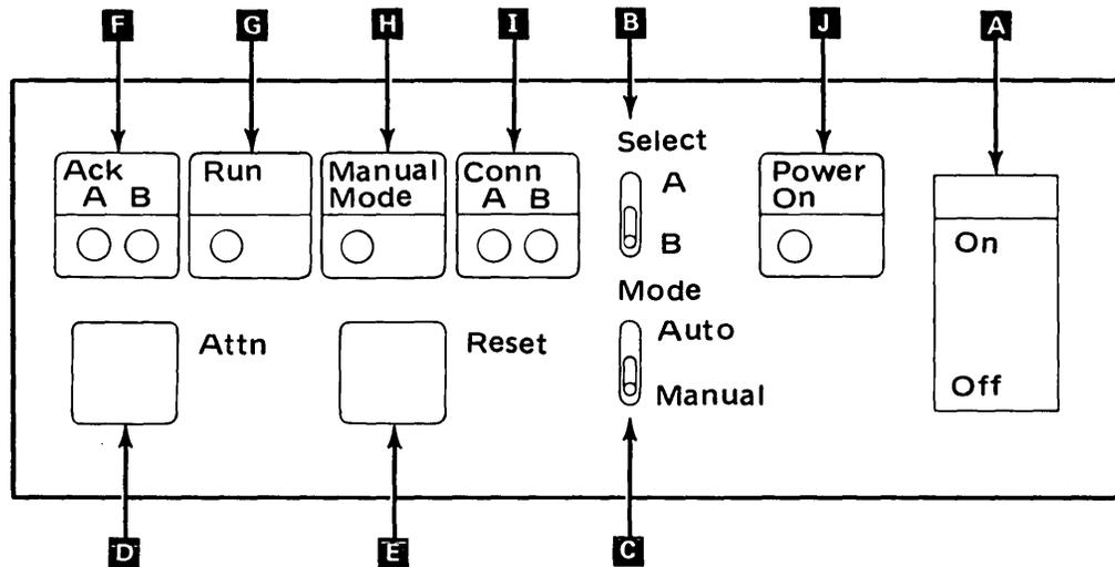
Figure 3-1. TCS Console Controls and Indicators.
