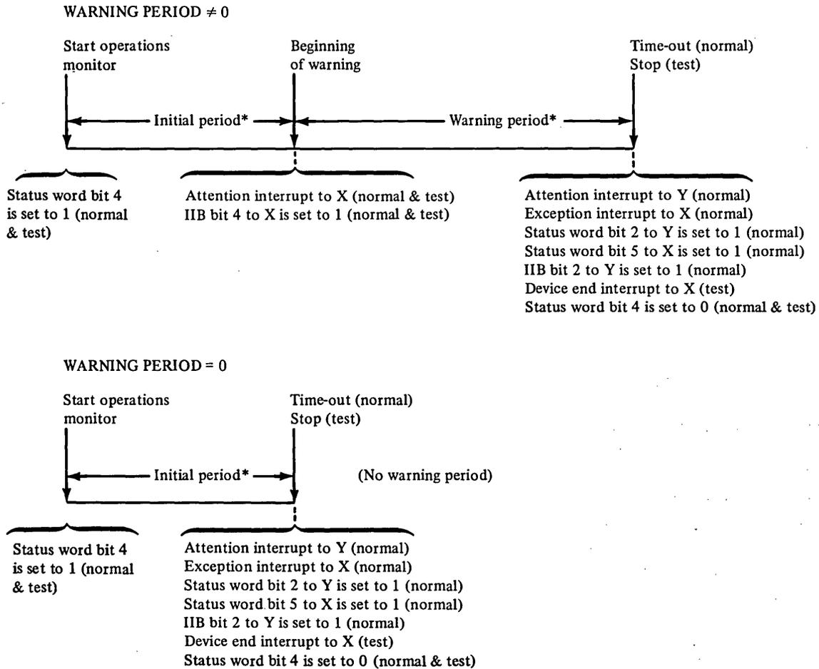
X is processor connected to common I/O and using timer.
