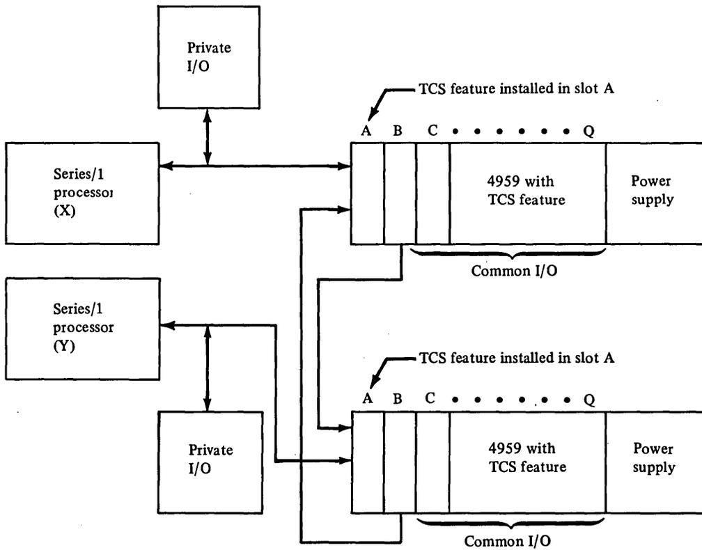
Figure 1-3. Typical system configurations using TCS feature
