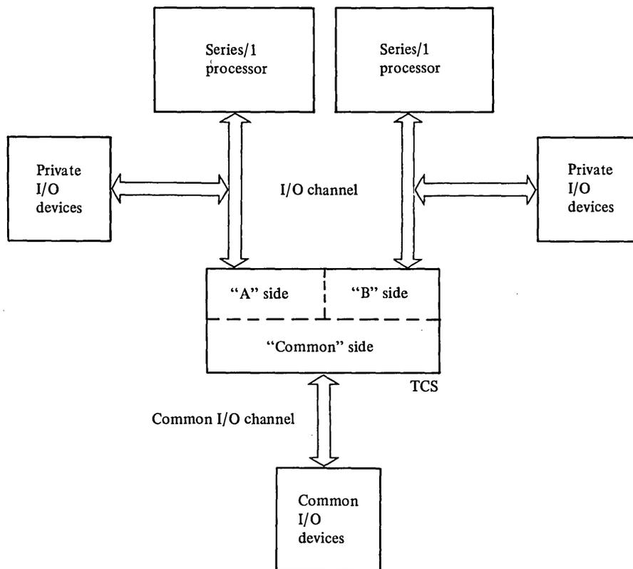
*Note.* Either processor can be designated as primary or backup and can be connected to either the "A" or "B" side of the TCS.
