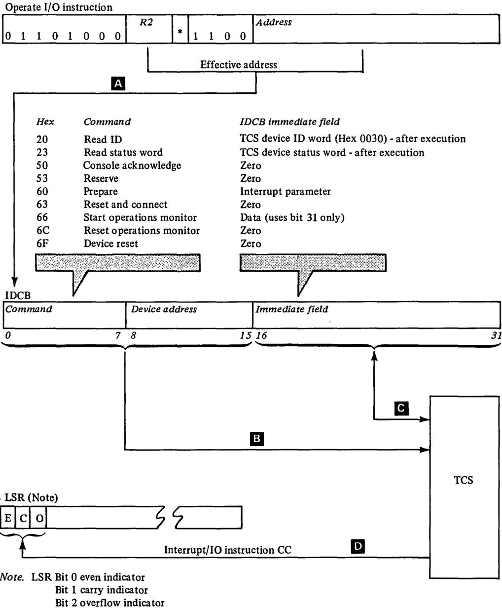
Figure 2-2. Direct program control I/O operation corresponding to the issuing processor
