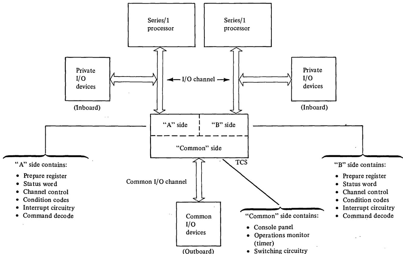
Figure 2-1. Block diagram of typical cabling arrangement
