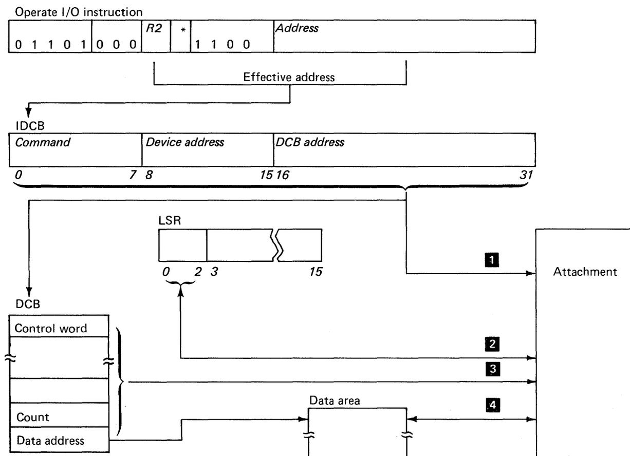
Figure 2-6. Cycle steal operation
