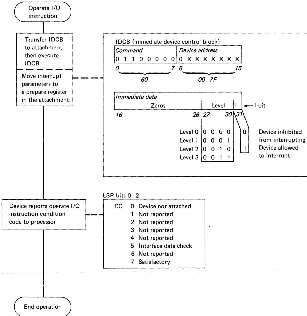
Figure 2-4. Prepare command operation
