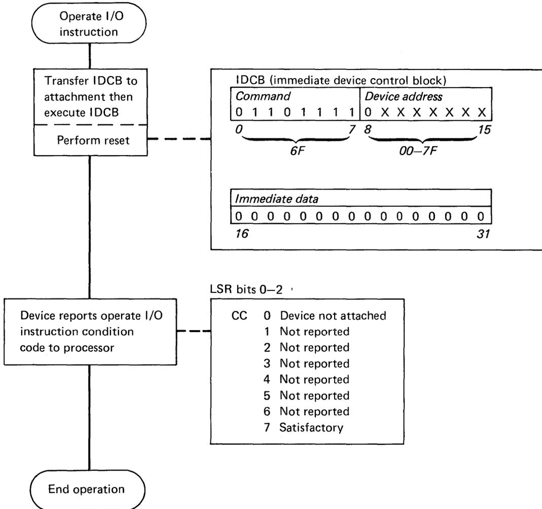
Figure 2-5. Device reset command operation
