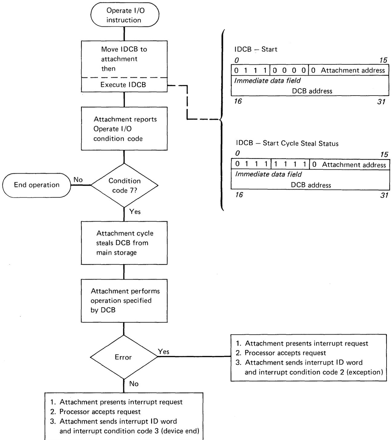
**Figure 2-7. Start and Start Cycle Steal Status commands sequence**
