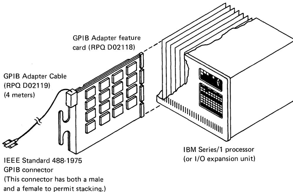
**Figure 1-1. GPIB Adapter and Cable**
