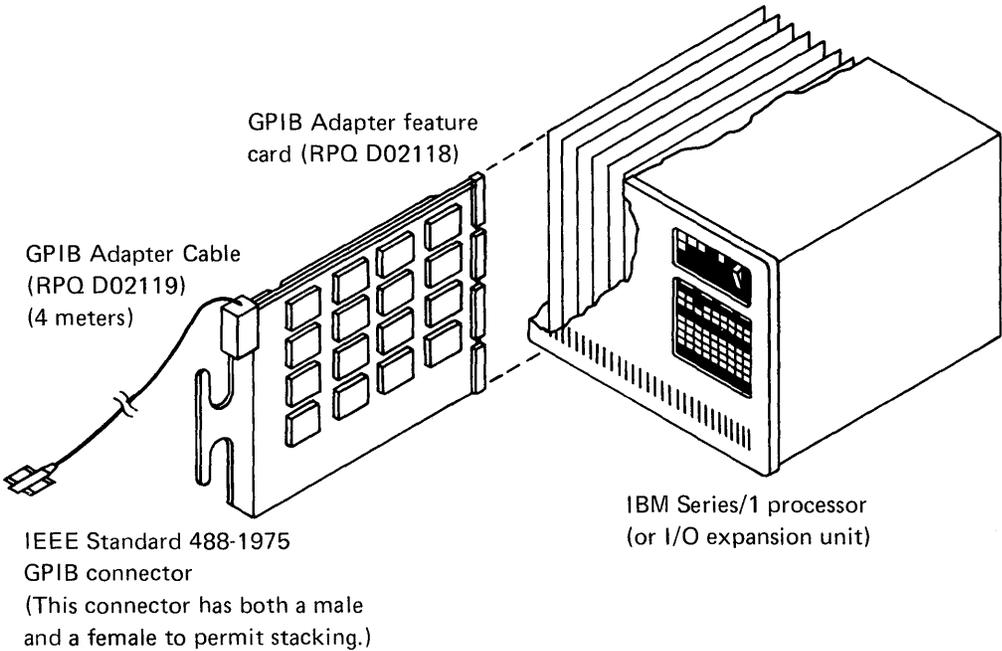
Figure 3-1. GPIB adapter
