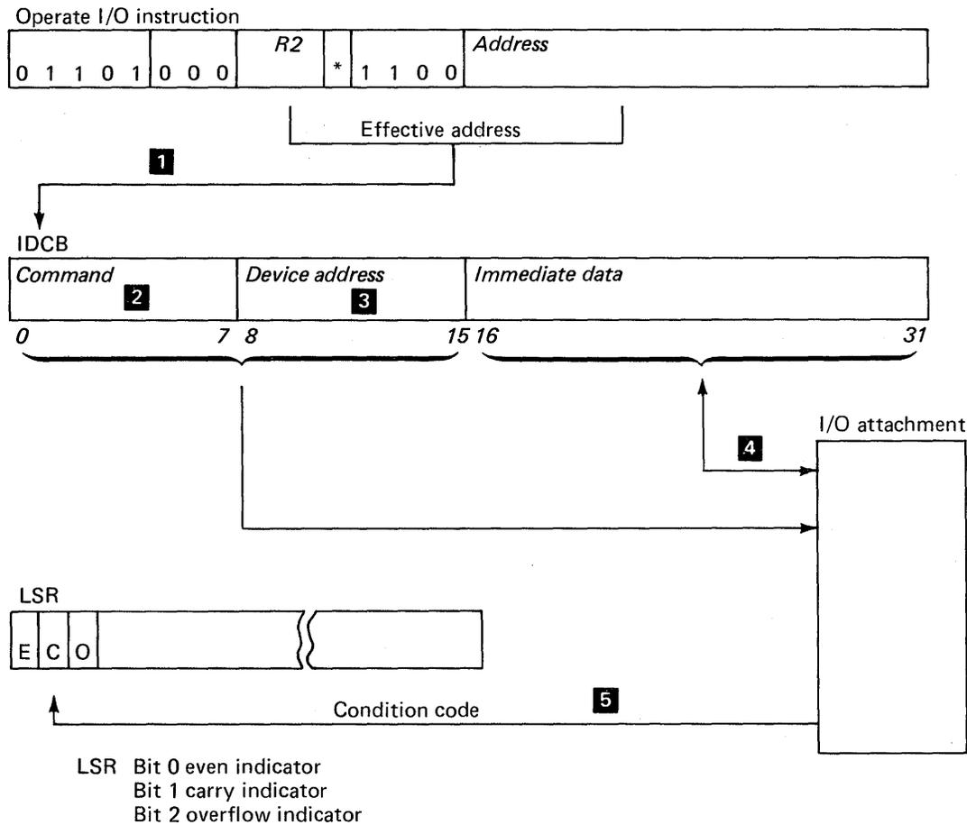
Figure 2-2. Direct program control I/O operation
