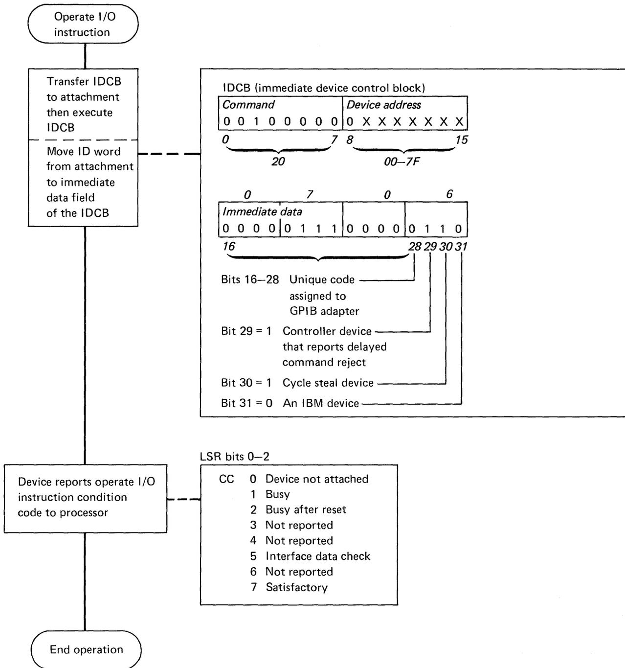
Figure 2-3. Read ID command operation
