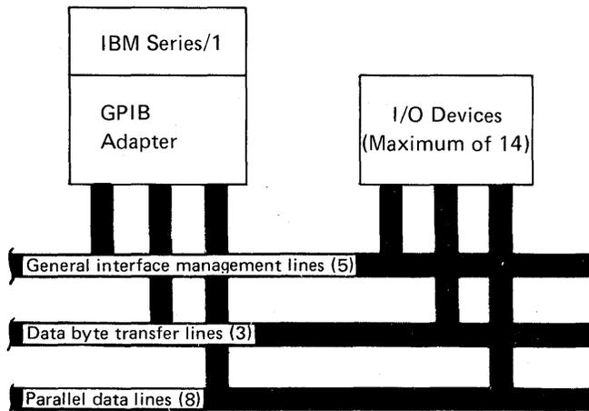
Figure 1-2. Interface structure
