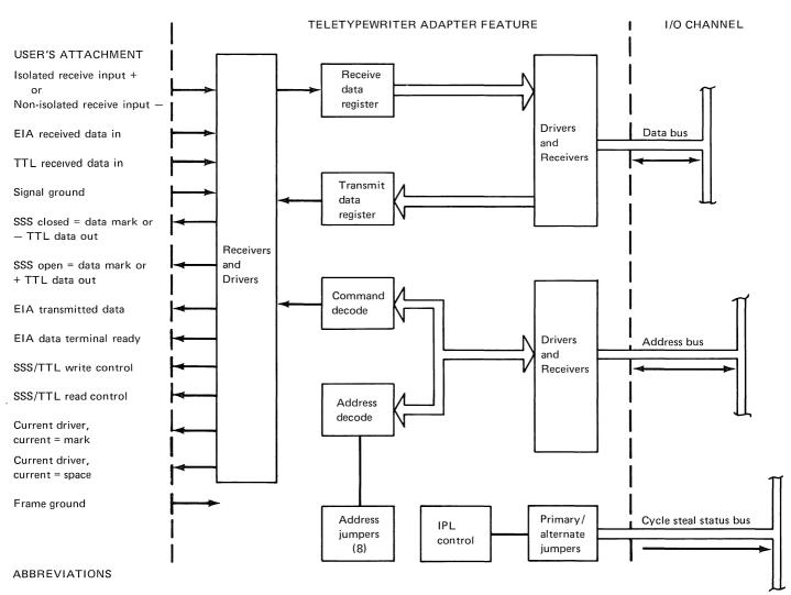
TTL = transistor-transistor logic
