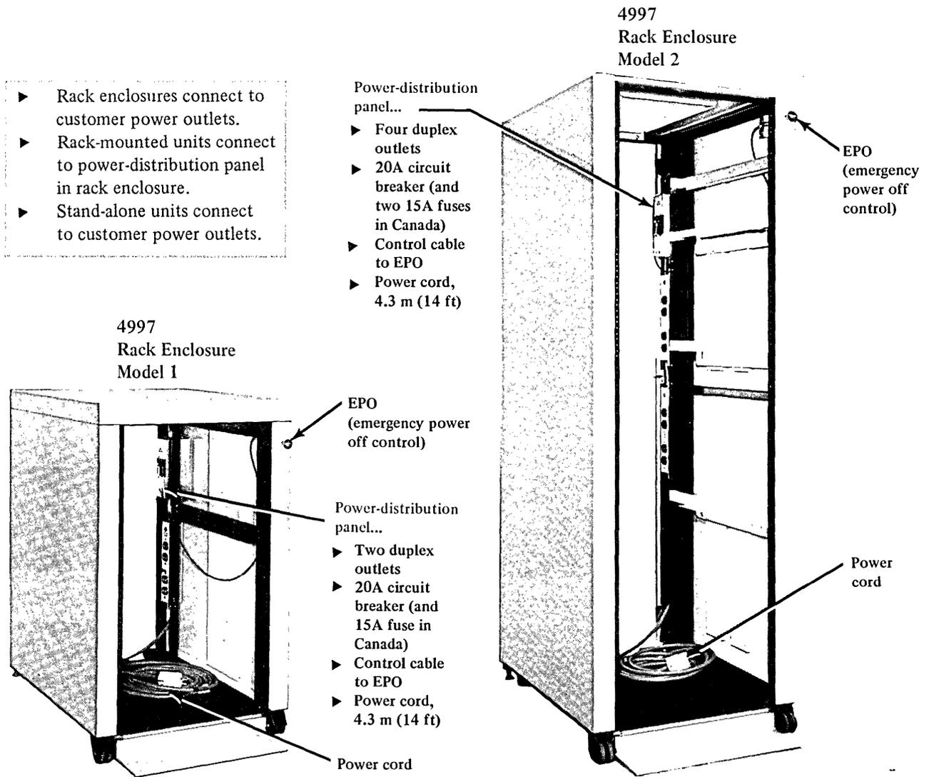
Figure 7-1. Series/1 rack-enclosure power distribution
