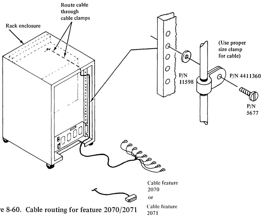
Figure 8-60. Cable routing for feature 2070/2071
