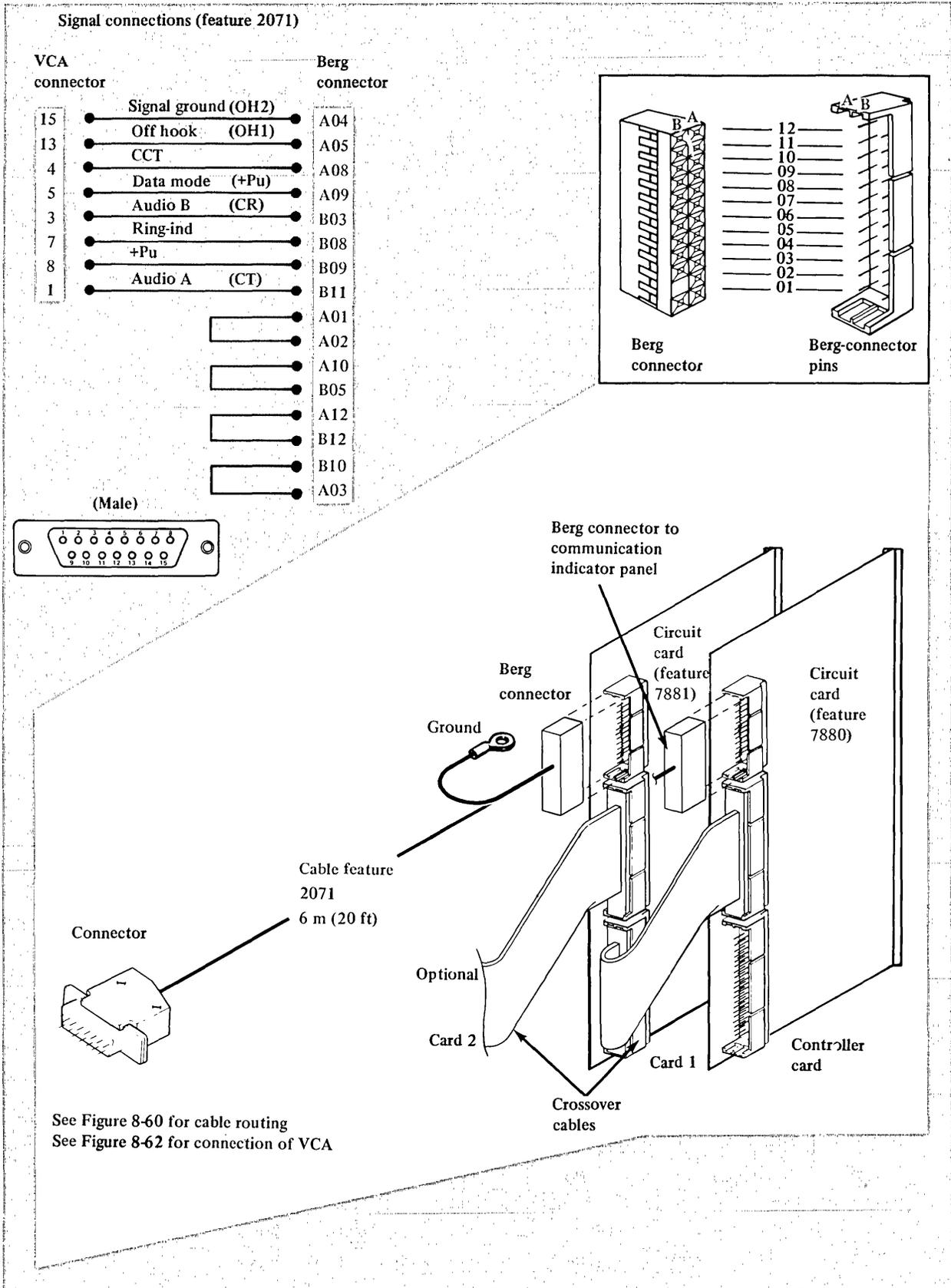
Figure 8-59. Cable and signal connections for feature 2071
