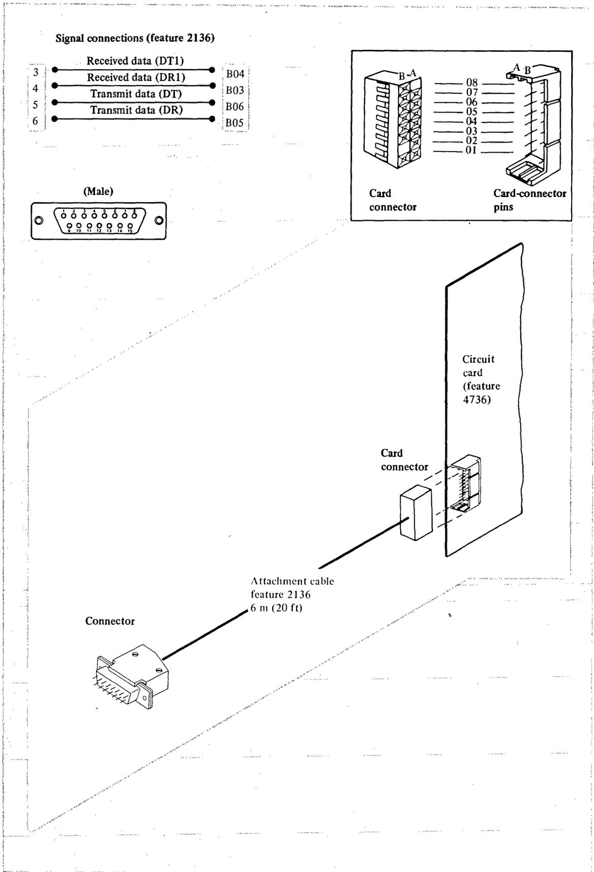
Figure 6-26. Cable and signal connections for DATA-PHONE Digital Service attachment feature
