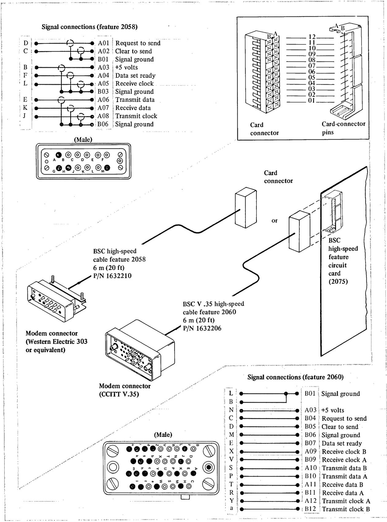
Figure 6-12. Cable and signal connections for high-speed BSC features
