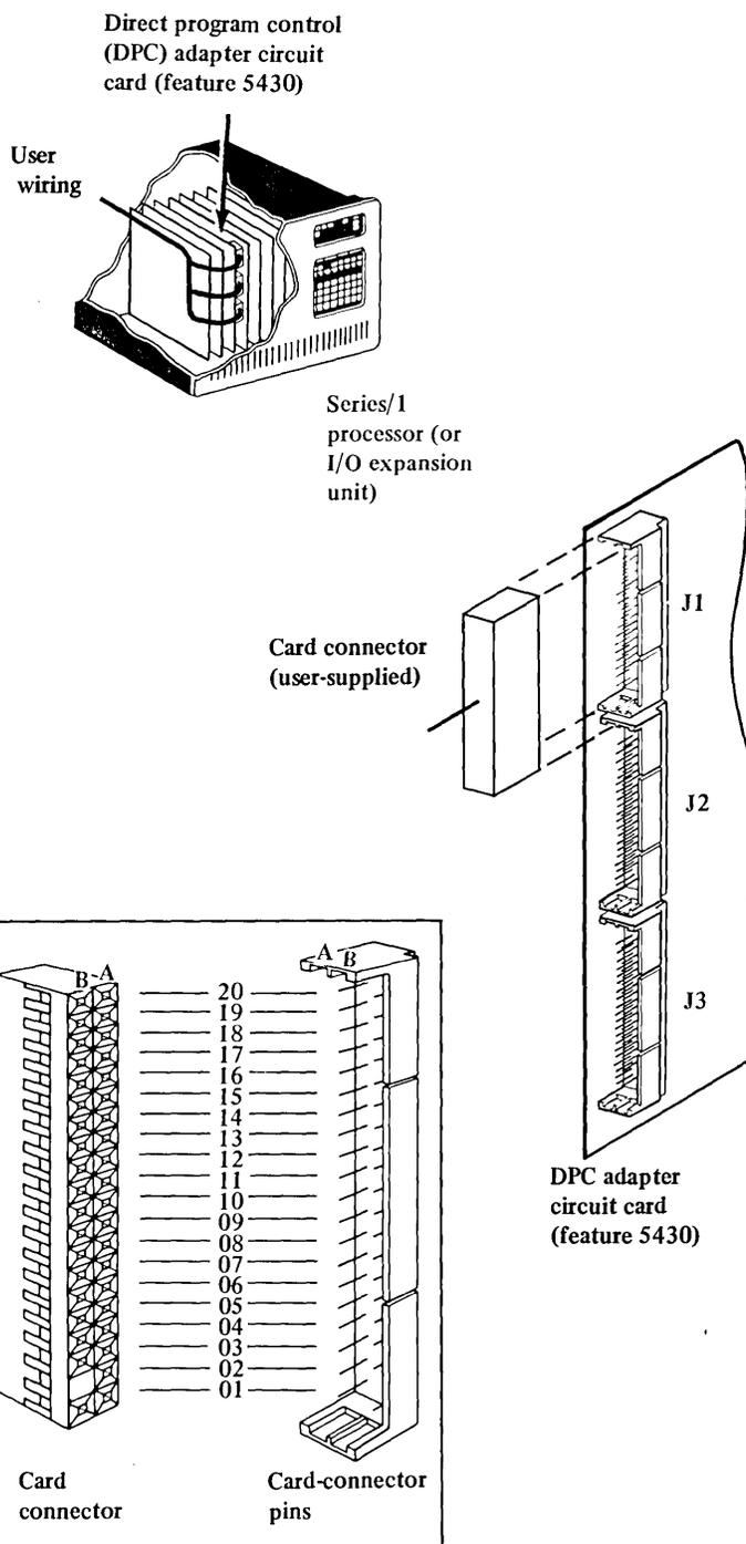
Figure 8-35. User connection directly to DPC adapter card
