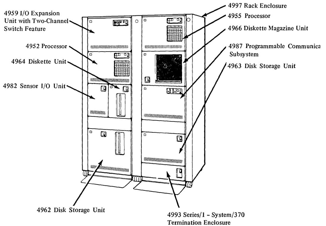
Figure 2-1. (Part 1 of 3) Series/1 machine units
