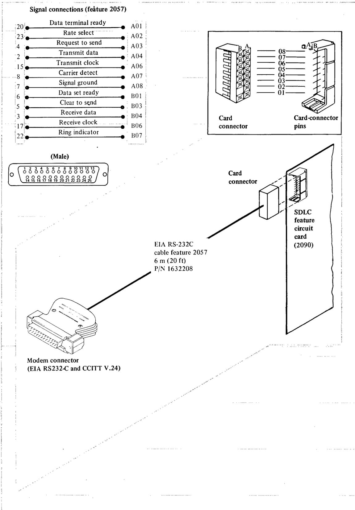
Figure 6-14. (Part 1 of 4) Cable and signal connections for feature 2090
