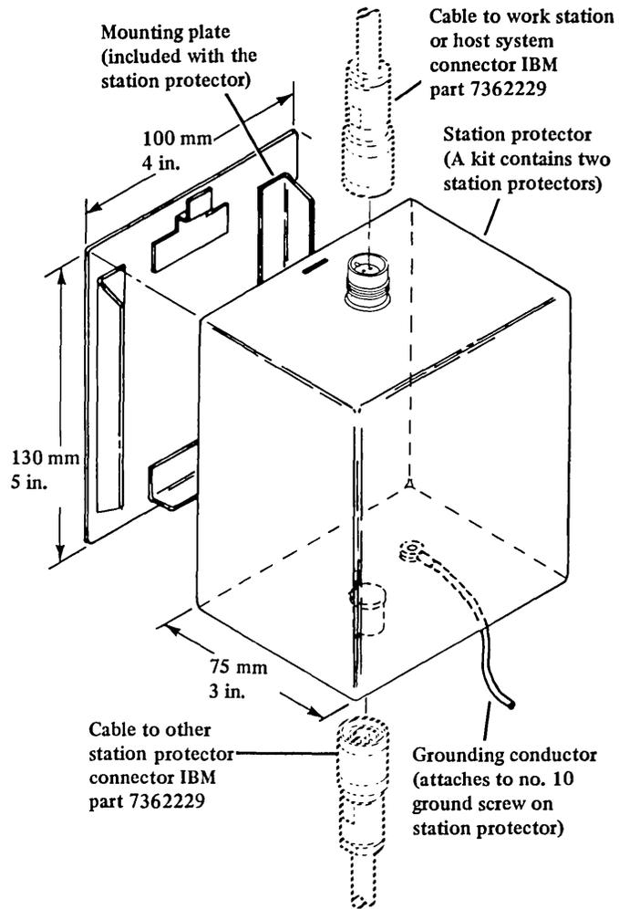
Figure 8-55. Station protector with entering/exiting cables
