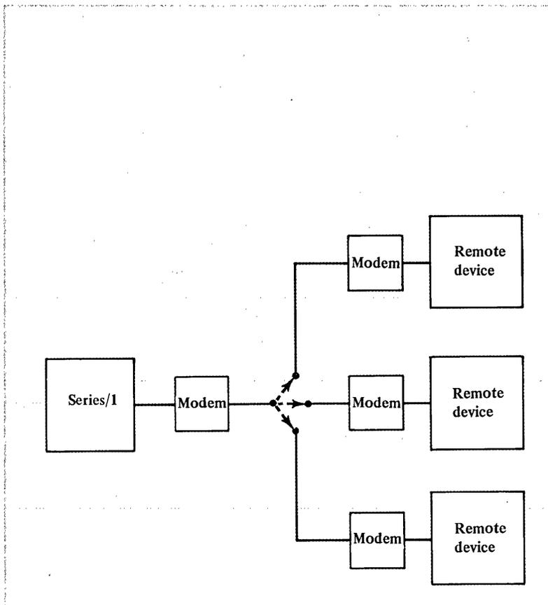
Figure 6-4. Sample communication network (point-to-point), switched)
