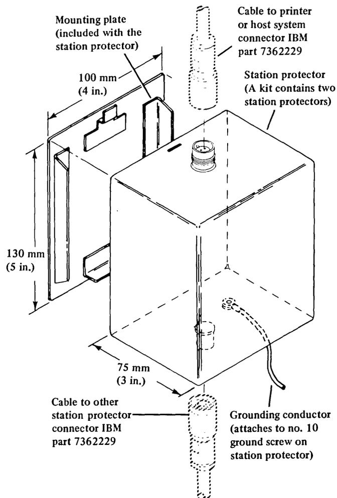
Figure 8-78. Station protector with entering/exiting cables
