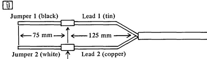
Solder Jumper 1 to Lead 1 and Jumper 2 to Lead 2. Cover each splice with 25 mm of shrink tubing (IBM 5700530 or Raychem RNF 100 Type 1 0.50 ID expanded/0.27 ID recovered).
