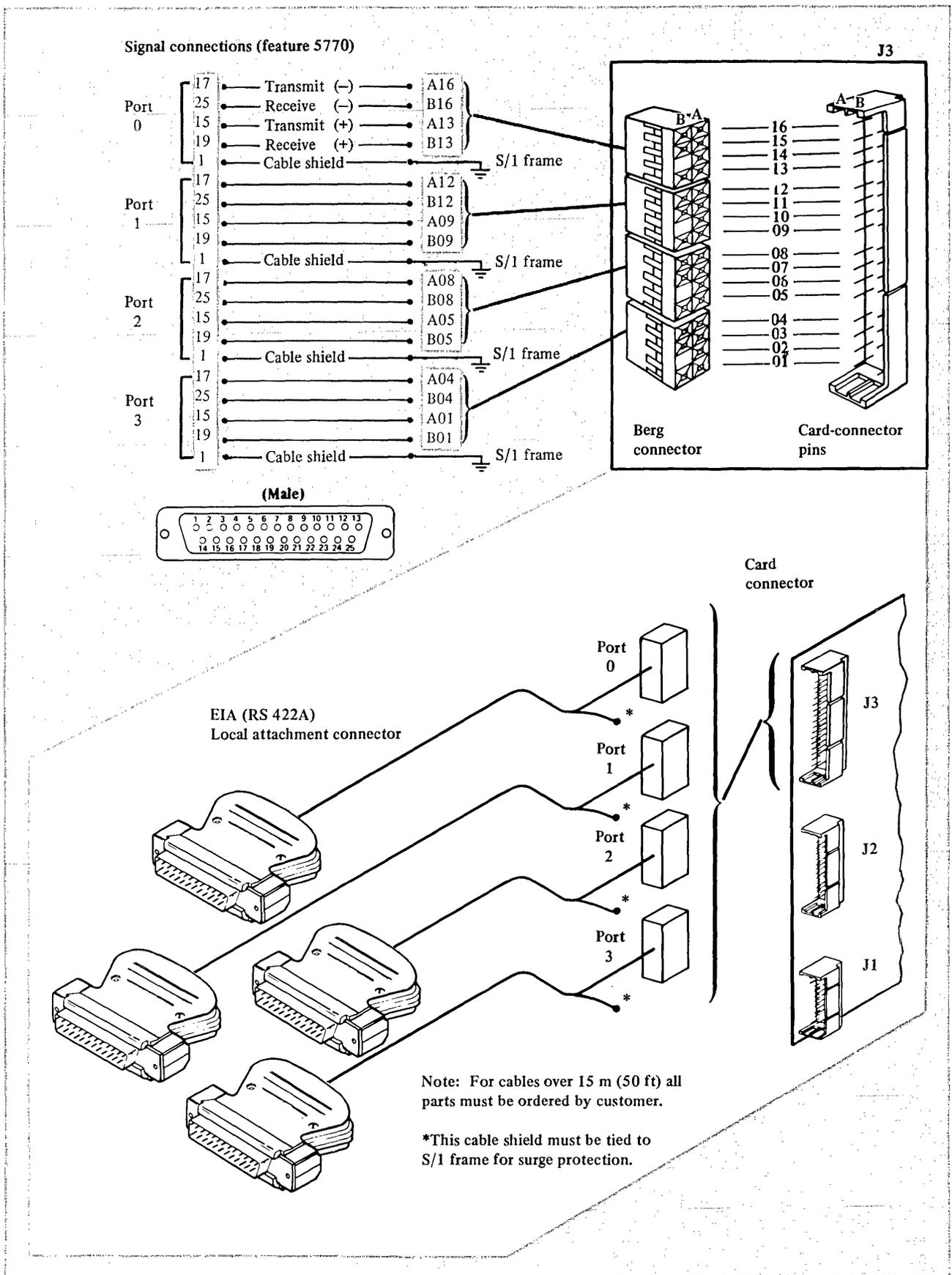
Figure 8-66 (Part 1). Feature 1310 cable and signal connections for 5770 cables
