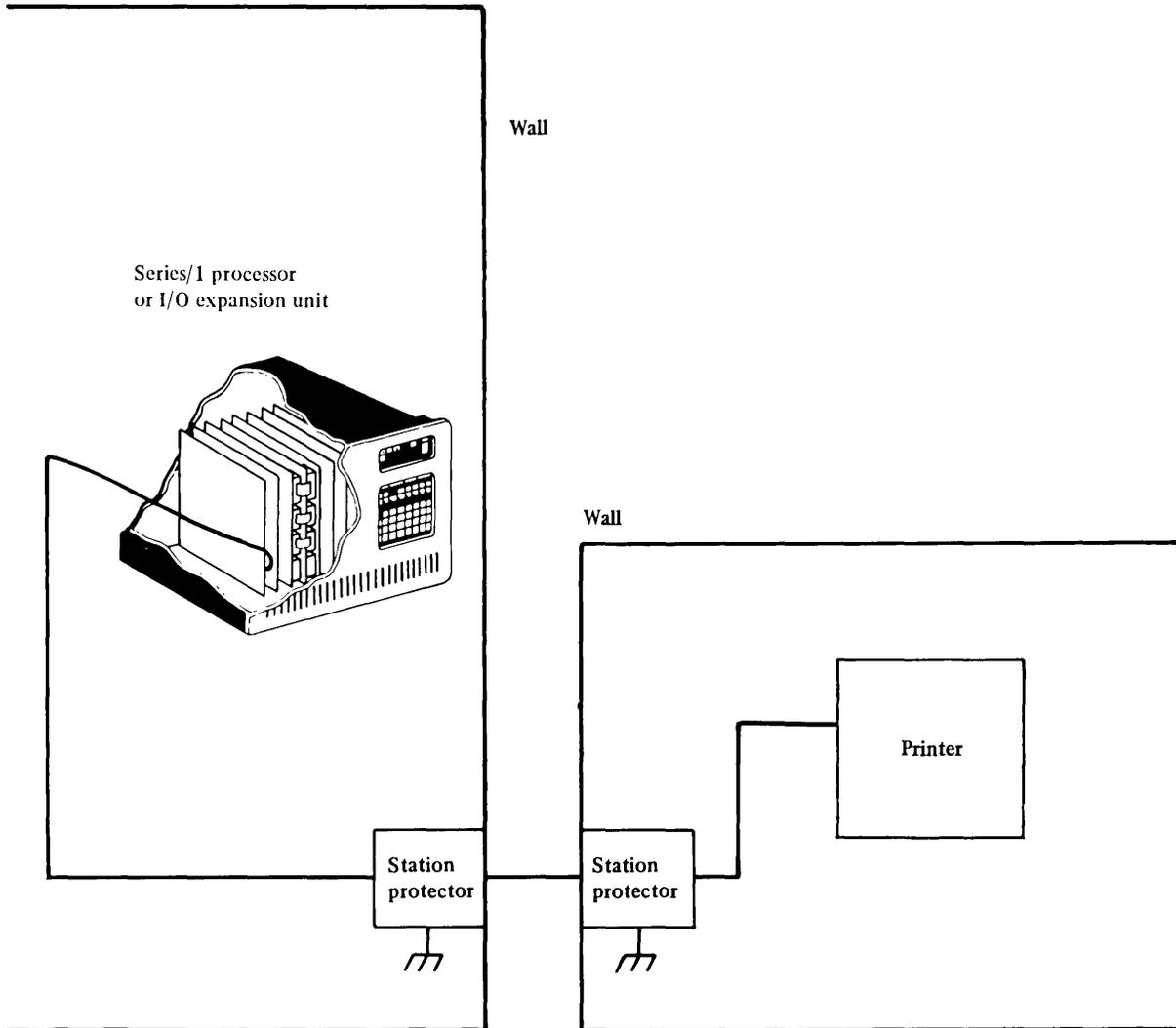
Figure 8-79. Sample station protector installation
