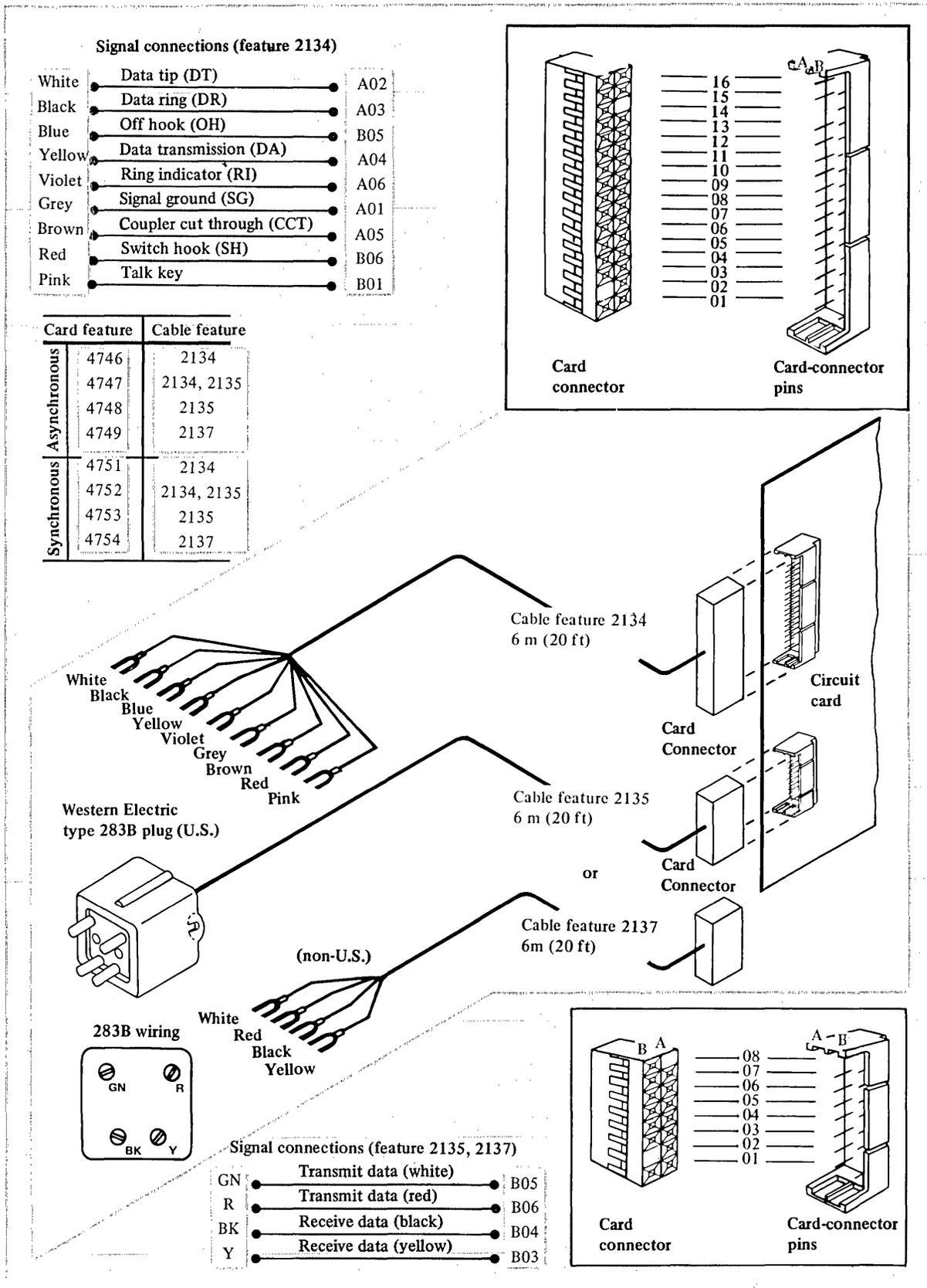
Figure 6-32. Cable and signal connections for integrated-modem attachment features
