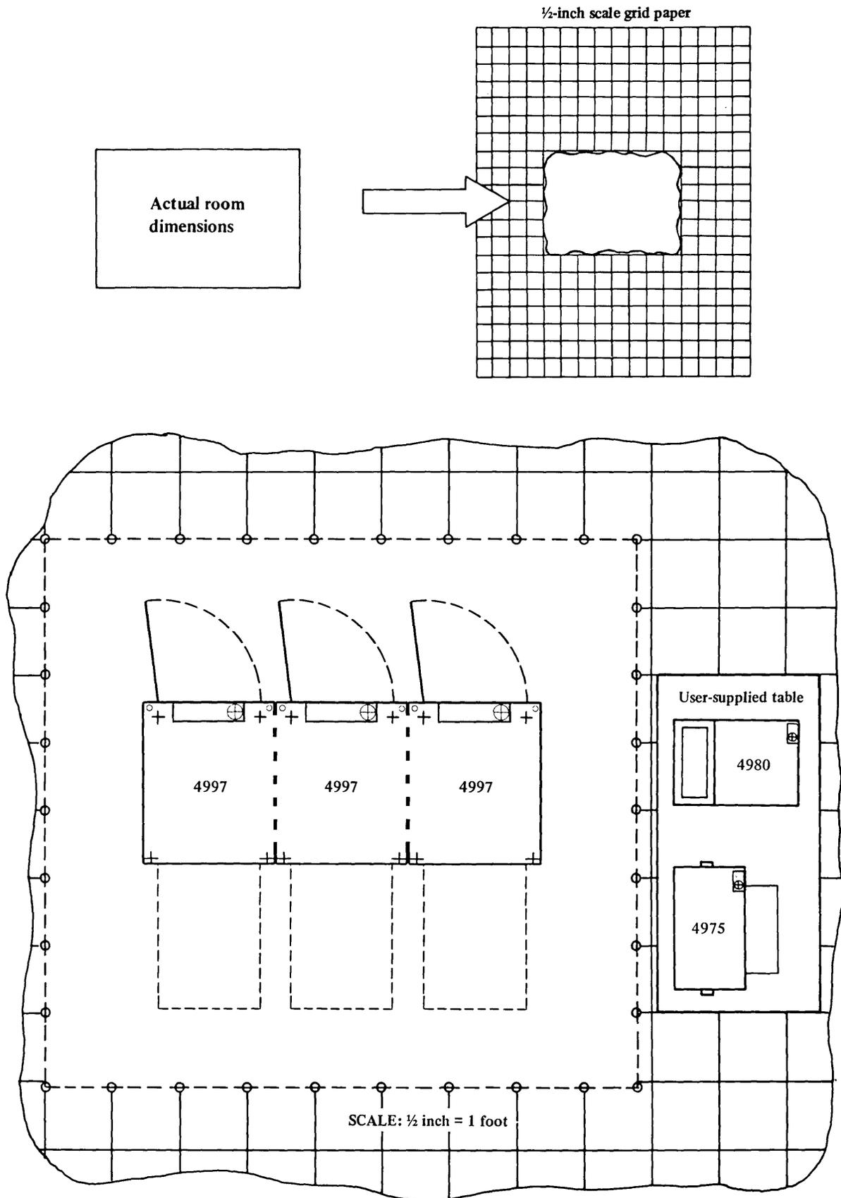
Figure 2-4. Sample floor layout for multiple rack enclosures
