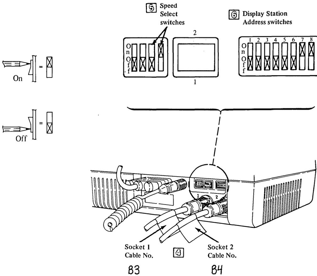
Each cable that you are connecting to your 4980 Display Station should be labeled. The label on the cable should indicate which socket on the display station the cable connects to. If there is no Cable No. given for socket 2, there should not be a cable connected to that socket.
