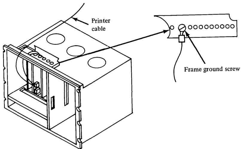
Figure 8-76. Card file cable installation for feature 5640
