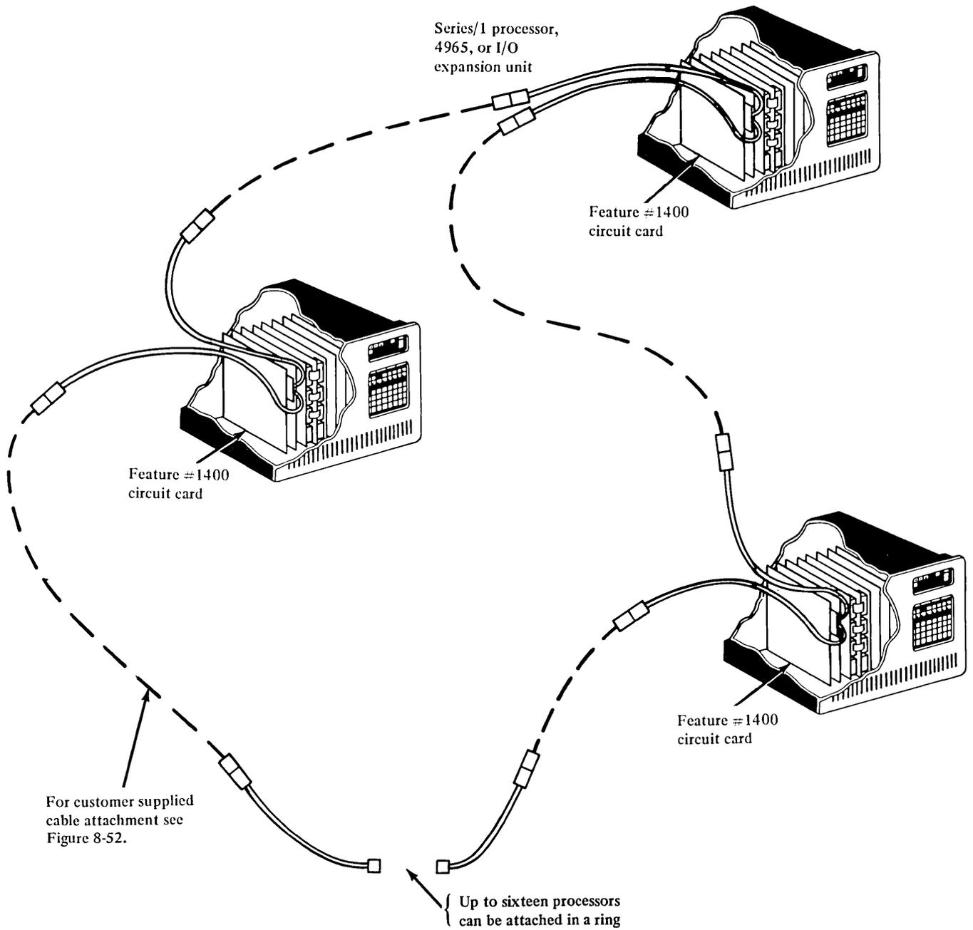
Figure 8-51. Feature 1400 sample configuration
