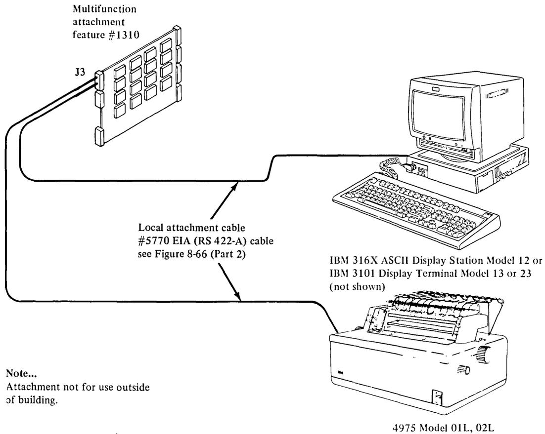
Figure 8-69 (Part 1). Feature 1310 local attachment of IBM 4975 and 316X
