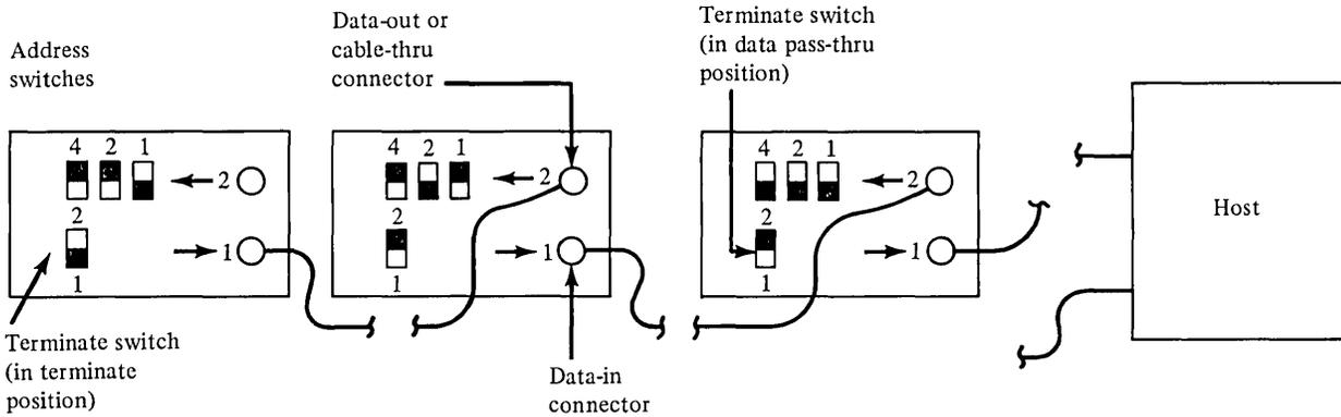
Each address switch in a string of printers must be set to its own unique value that
