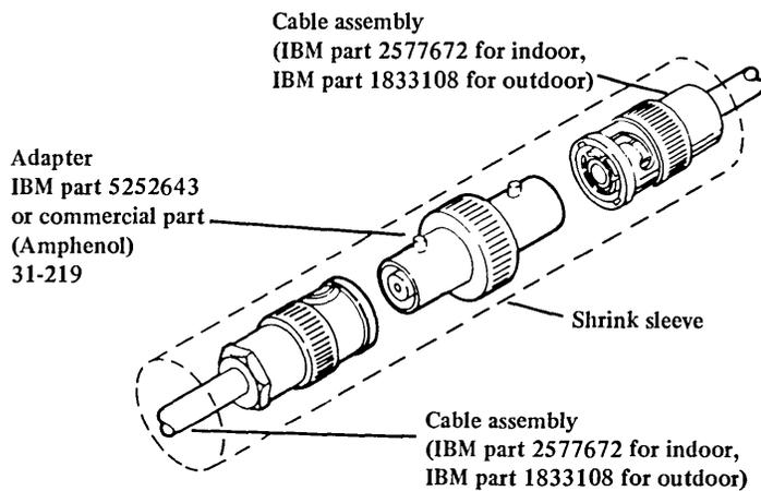
Figure 8-54. Cable adapter for splicing coaxial cables
