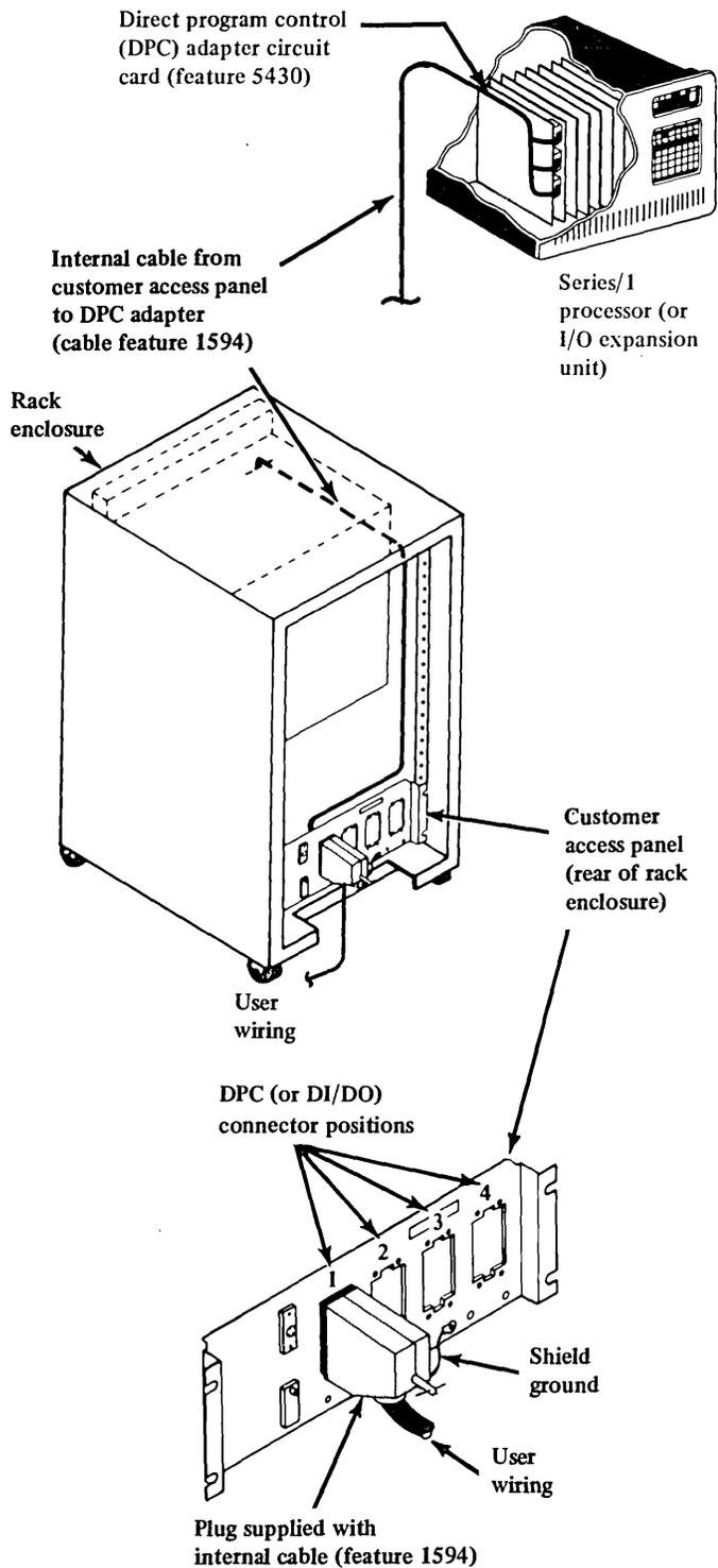
Figure 8-37. User connection to customer access panel for DPC adapter
