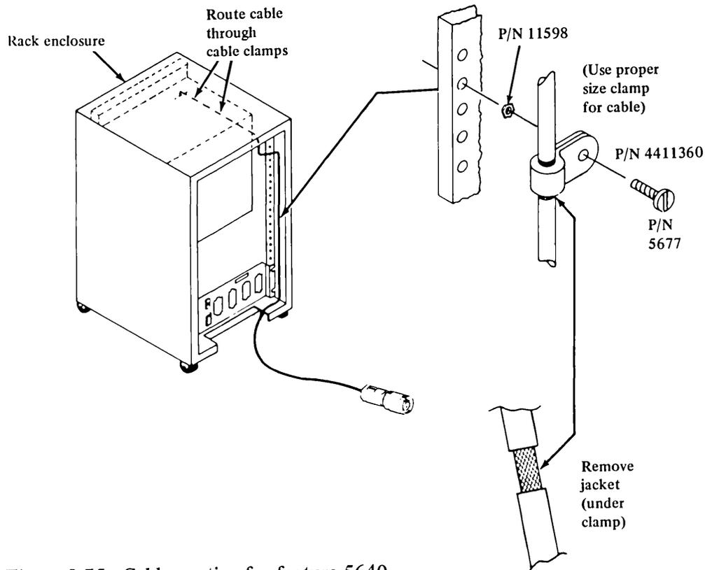
Figure 8-75. Cable routing for feature 5640
