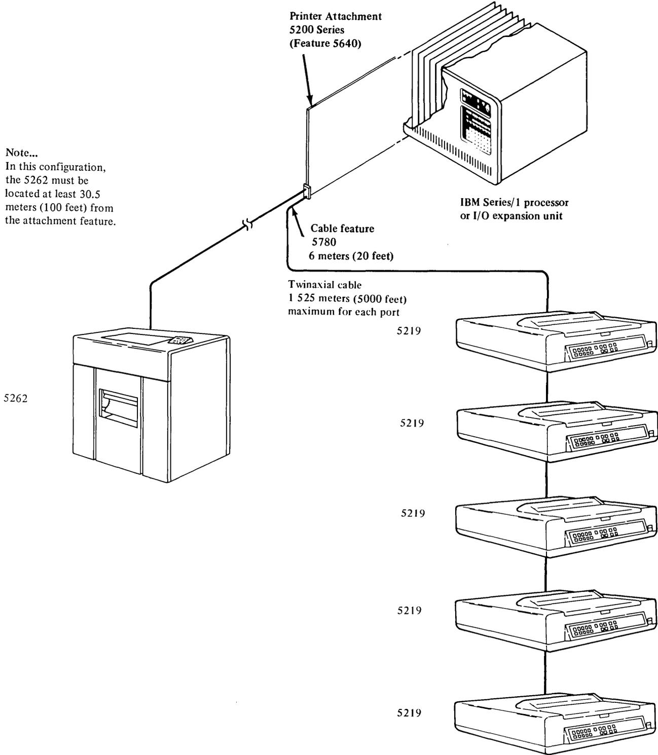
Figure 8-72A Sample configuration for feature 5640
