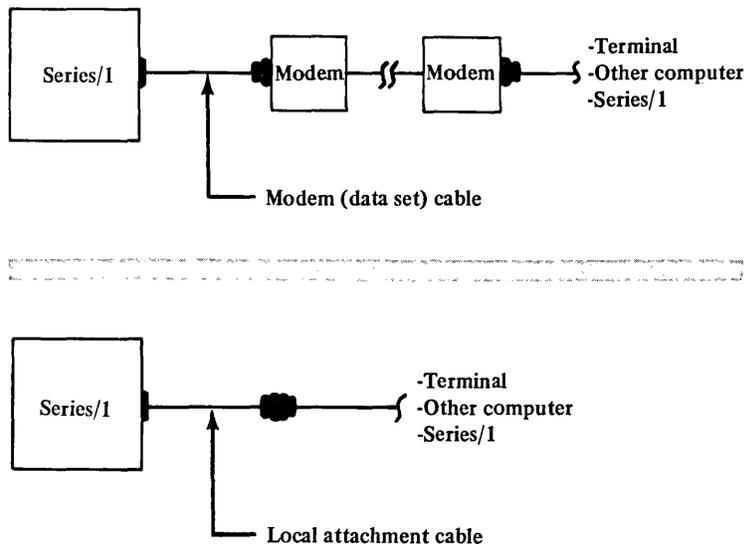
Figure 6-2. Modem and direct connections
