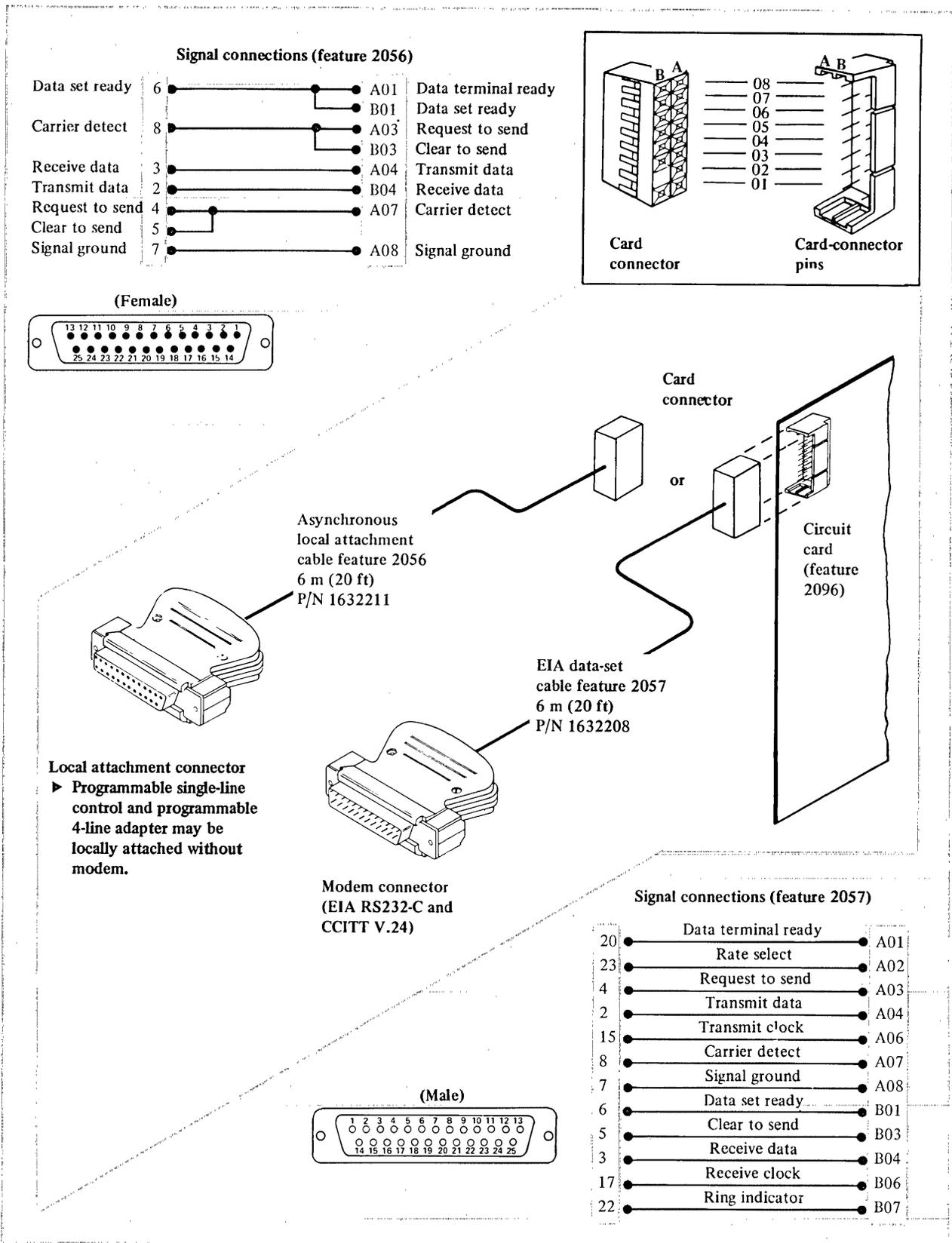
Figure 6-17. Cable and signal connections for Feature-Programmable Multi-Line attachments
