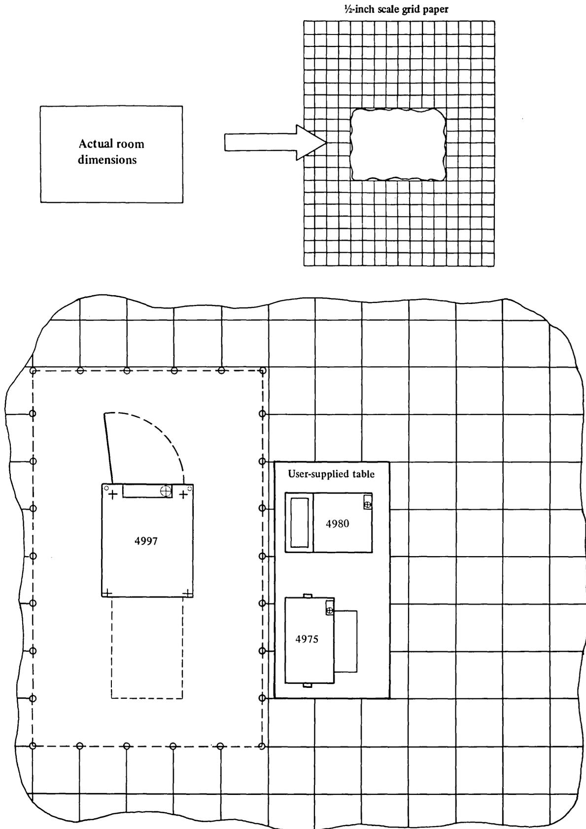
Figure 2-3. Sample floor layout for single rack enclosure
