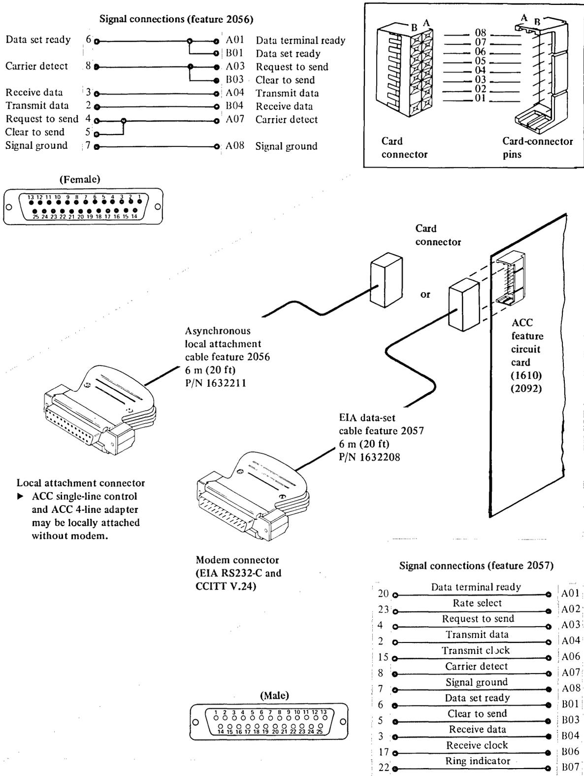
Figure 6-9. Cable and signal connections for ACC features
