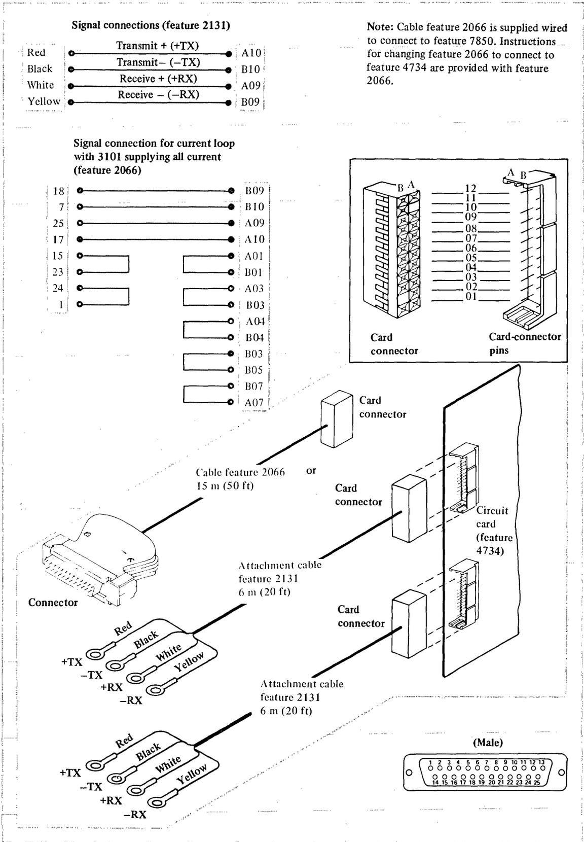
Figure 6-24. Cable and signal connections for TTY current loop attachment feature
