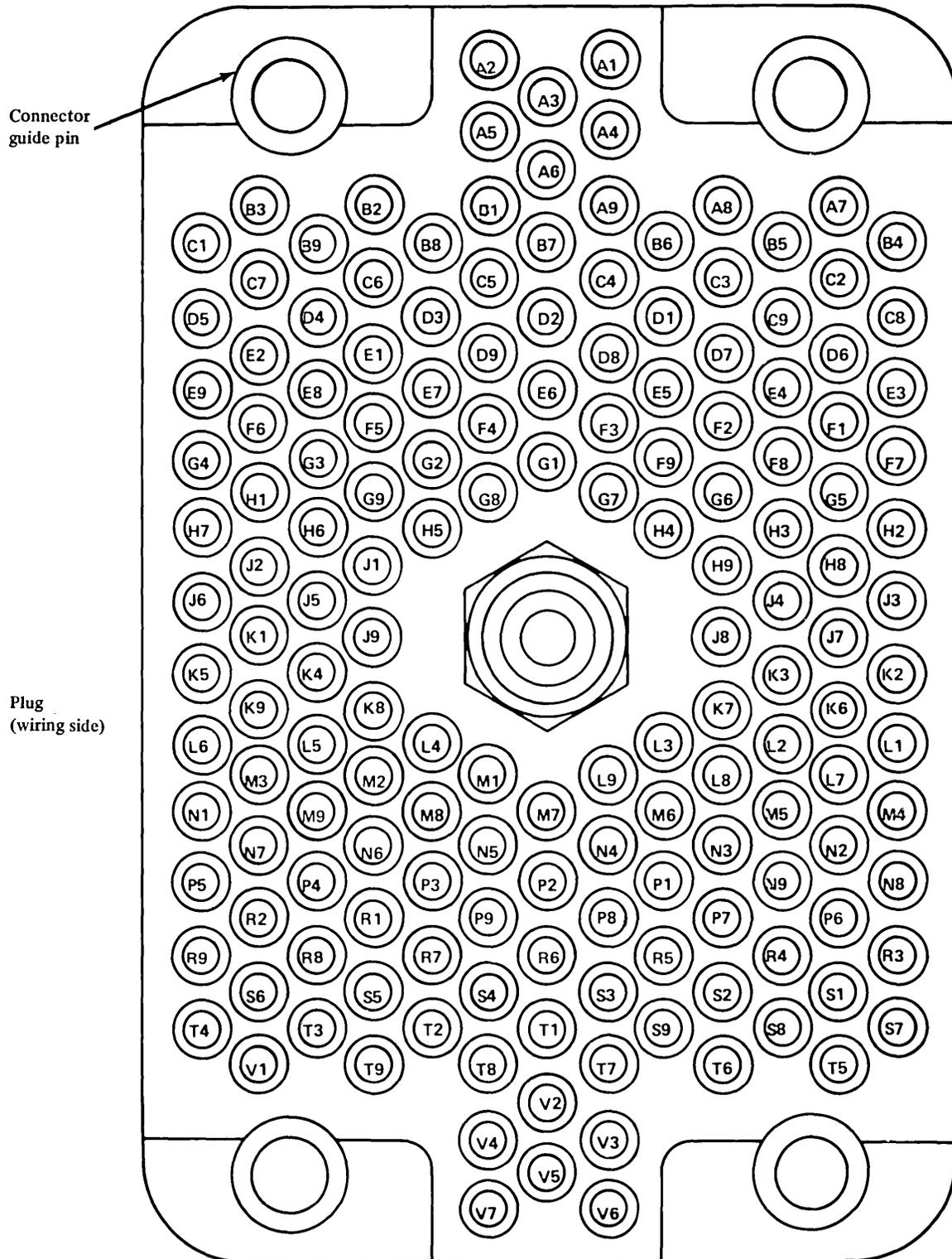
Figure 8-34. Signal connections for integrated DI/DO
