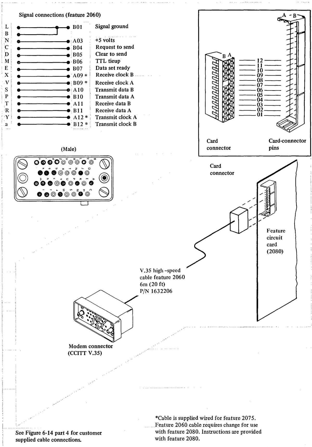
Figure 6-14. (Part 3 of 4) Cable and signal connections for feature 2080
