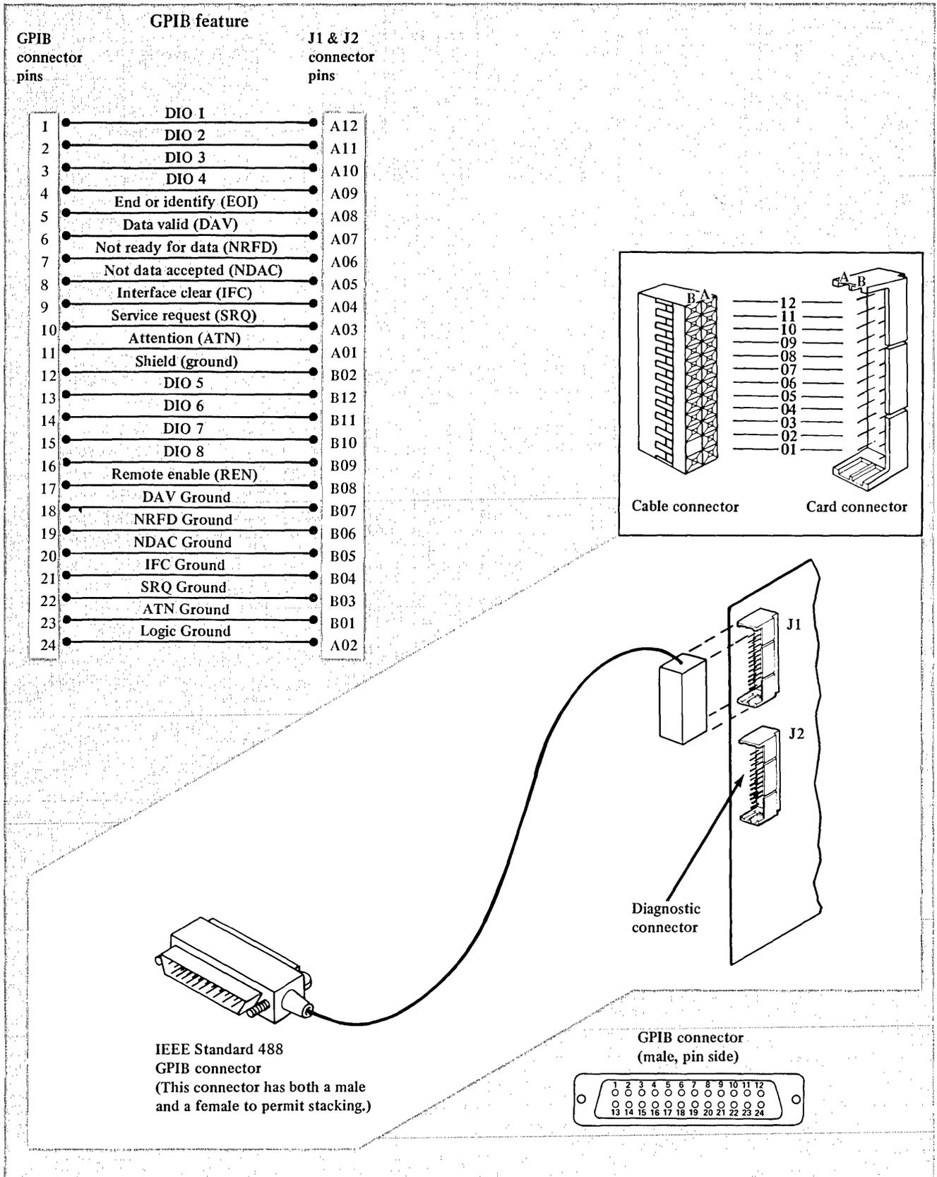
Figure 8-47. User connection directly to GPIB-feature card
