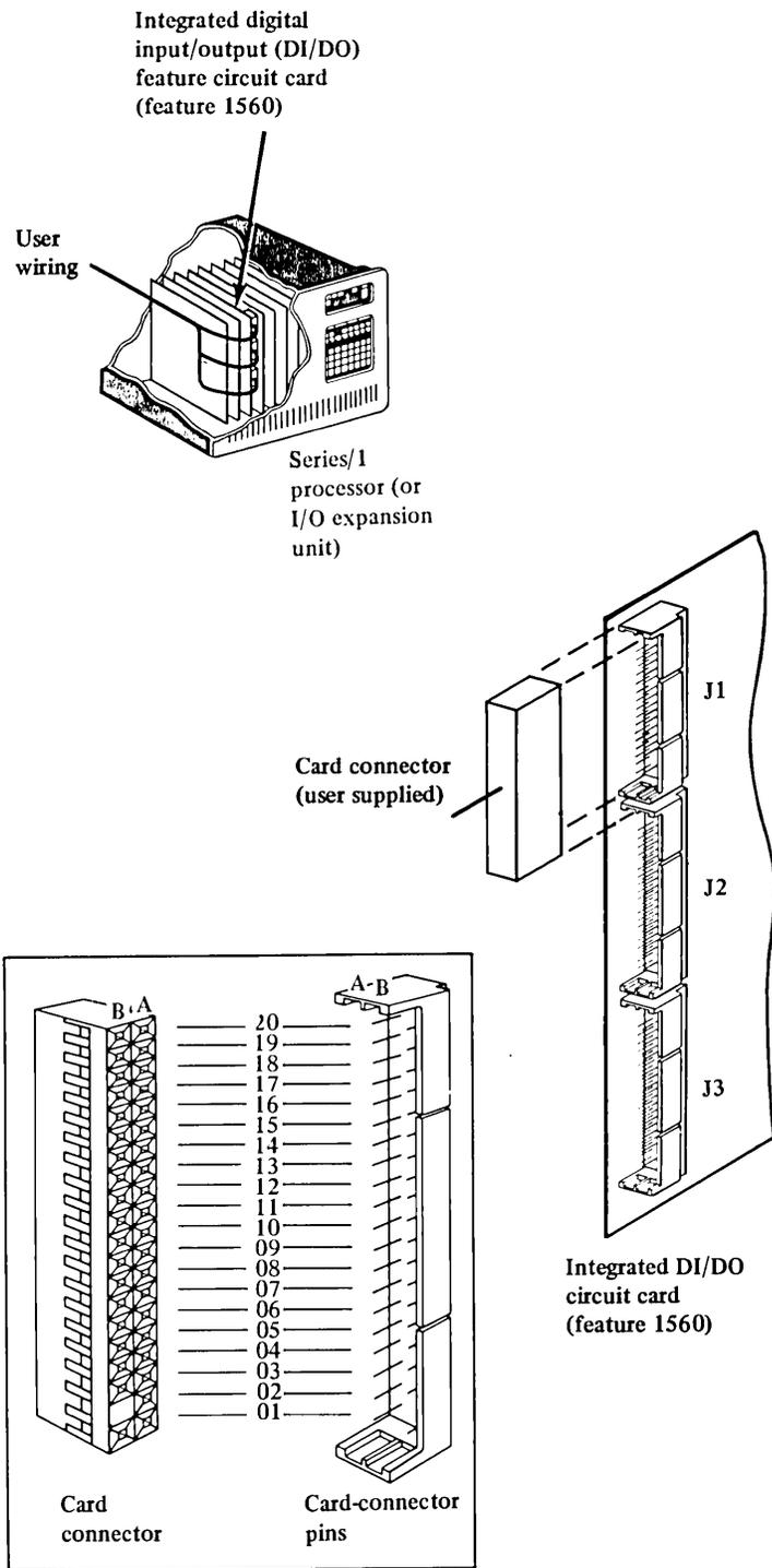
Figure 8-30. User connection directly to integrated DI/DO feature card
