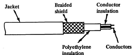
Figure 8-4. Types of signal cable .
