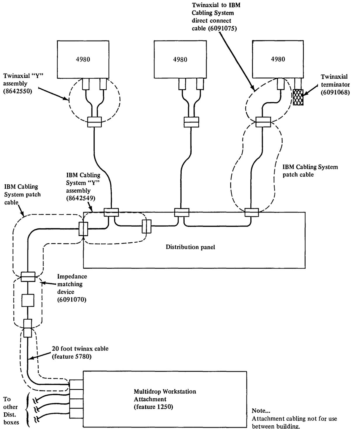
Figure 8-84 (Part 2). Sample configuration for feature 1250 (IBM Cabling System media)
