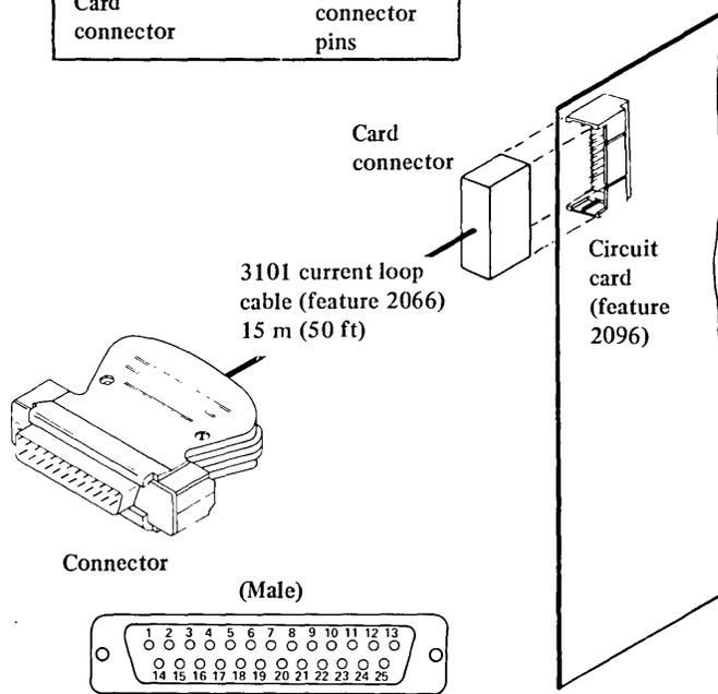
Figure 6-19 (Part 1). Current loop interface for Feature—Programmable Multi-line attachment
