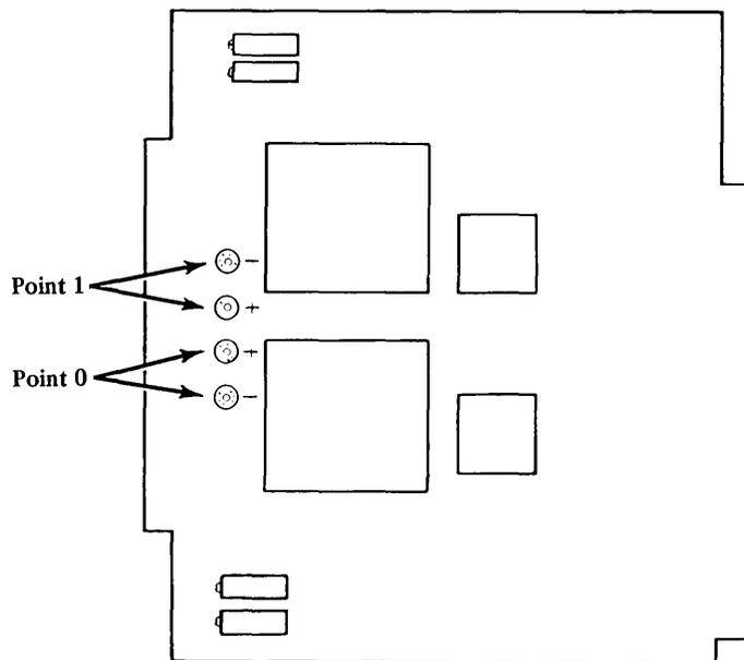
AO connections are made directly to the AO feature card with screw connectors on the card.
