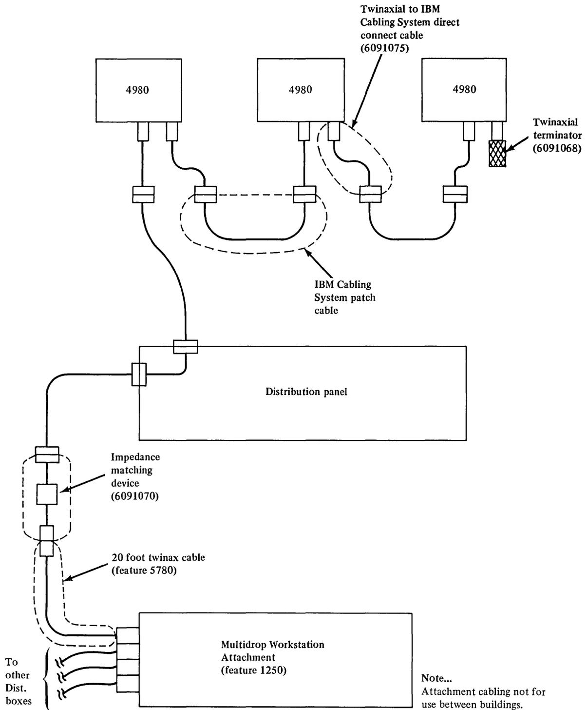
Figure 8-84 (Part 3). Sample configuration for feature 1250 (IBM Cabling System media)
