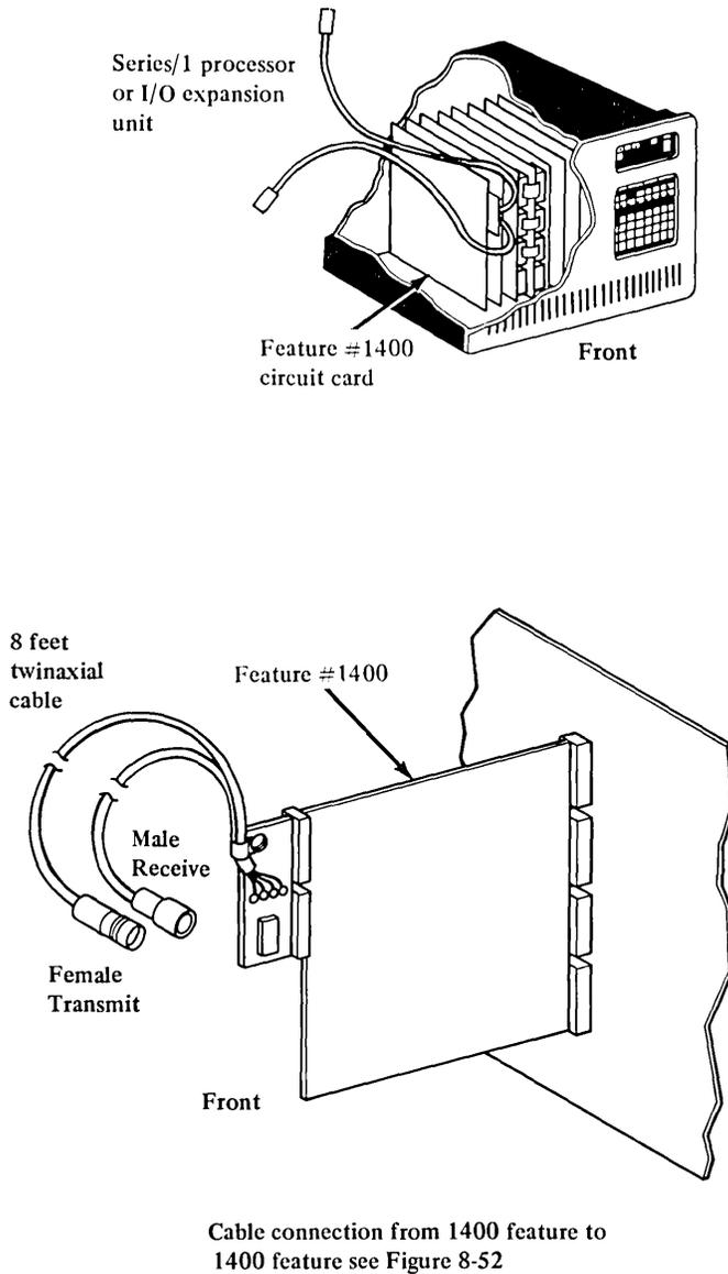
Figure 8-48. Series/1 Local Communications Controller feature
