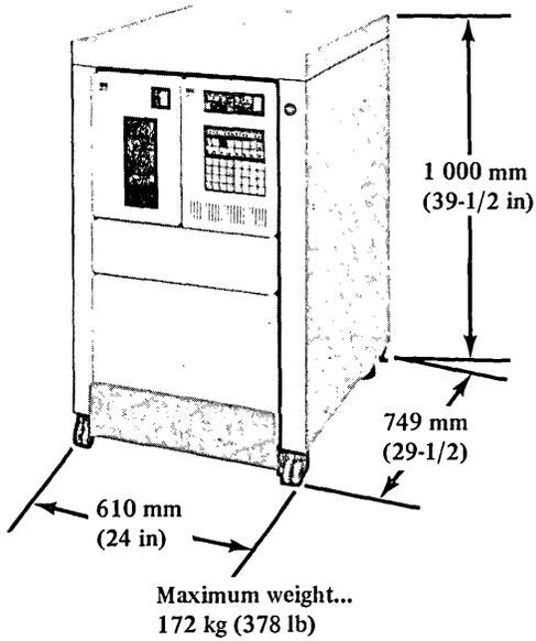
Figure 4-2. Series/1 shipped without a pallet (or ballast)
