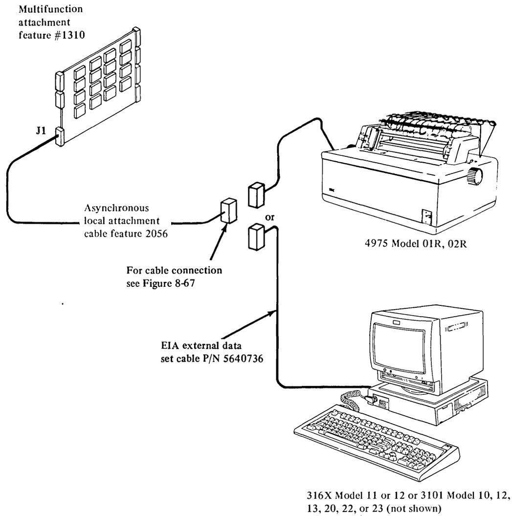
Figure 8-68. Feature 1310 direct connect of IBM 4975 and 316X
