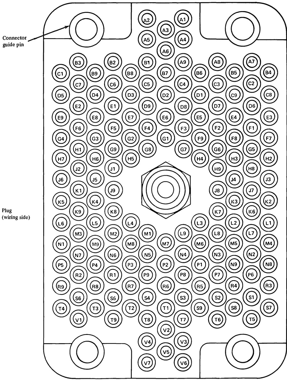
Figure 8-39. Signal connections for DPC connector on customer access panel
