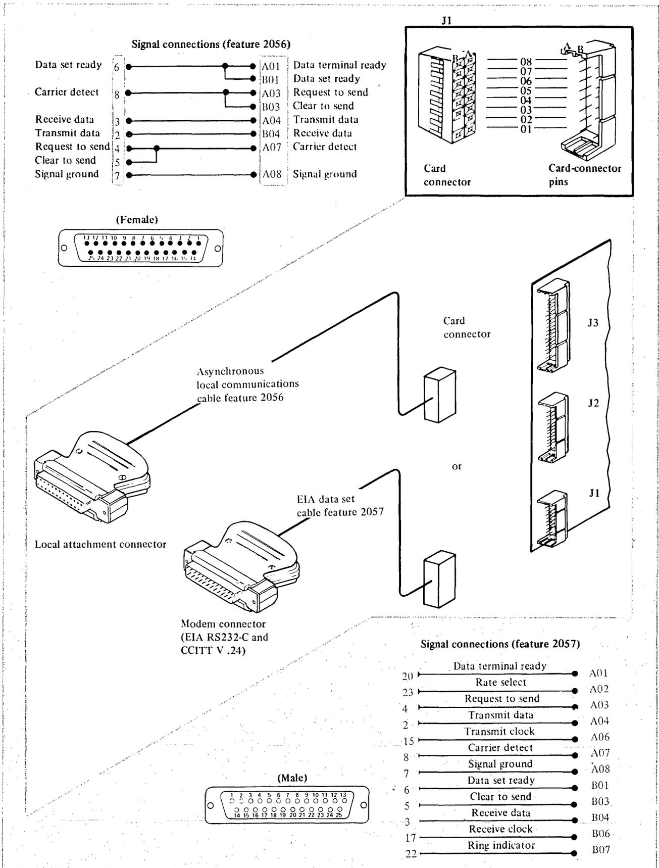
Figure 8-67. Feature 1310 cable and signal connections for 2056 and 2057 cables
