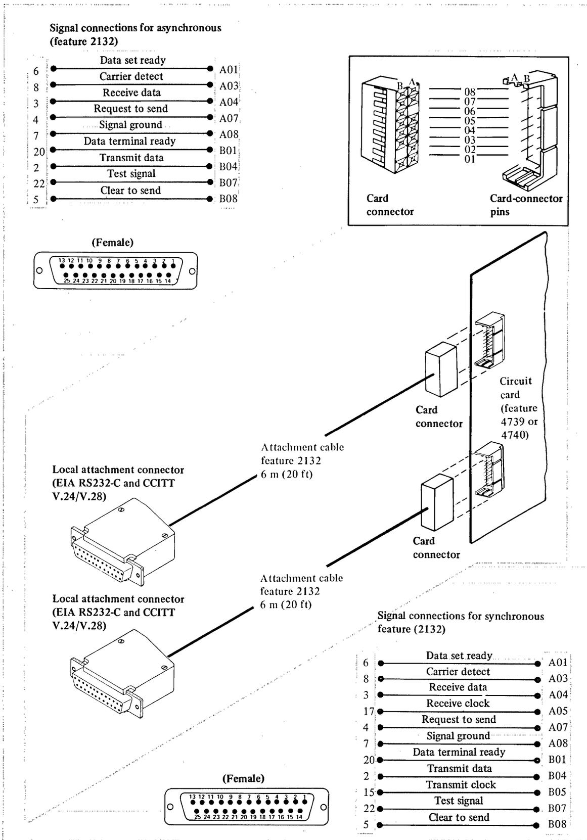
Figure 6-28. Cable and signal connections for local attachment features
