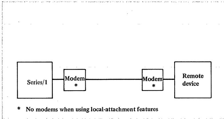
Figure 6-3. Sample communication network (point-to-point, nonswitched)
