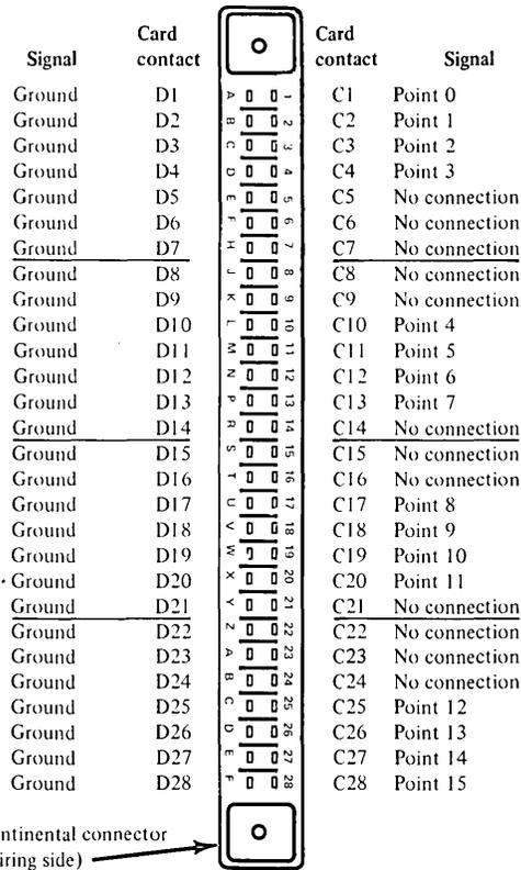
Figure 8-28. Signal connections for sensor I/O feature cards
