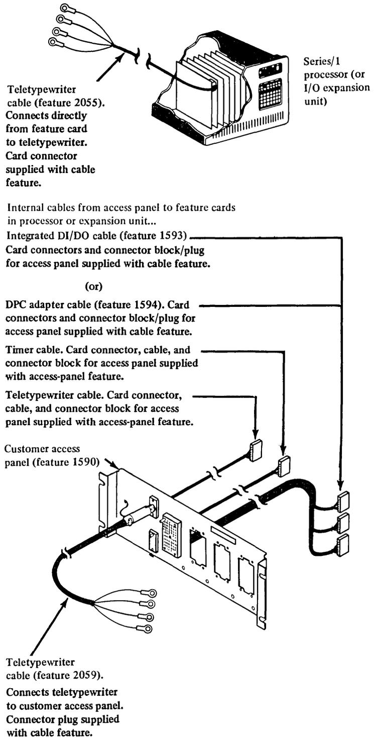
Figure 8-10. User-attachment cable features
