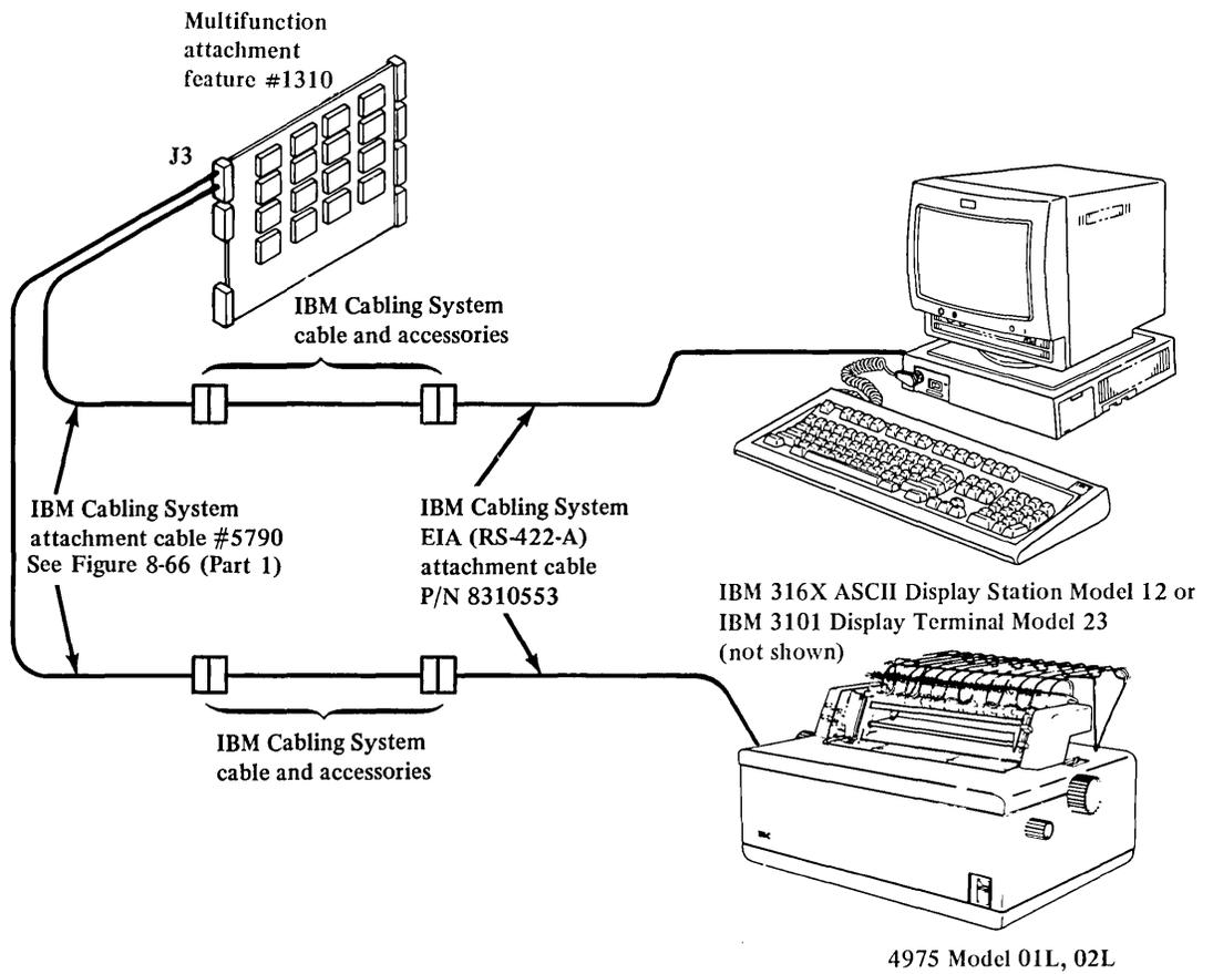
Figure 8-69 (Part 2). Feature 1310 IBM Cabling System attachment of IBM 4975 and 316X
