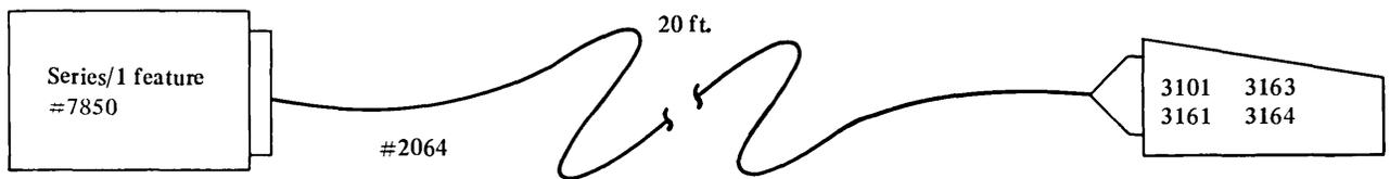
**Figure 8-19. 3101, 3161, 3163, 3164 teletypewriter adapter cable with EIA male connector**
