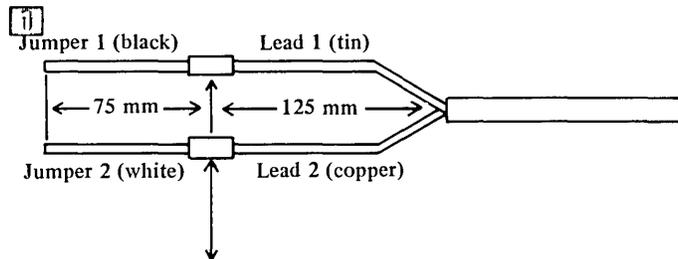
Solder Jumper 1 to Lead 1 and Jumper 2 to Lead 2. Cover each splice with 25 mm of shrink tubing (IBM 5700530 or Raychem RNF 100 Type 1 0.50 ID expanded/0.27 ID recovered).
