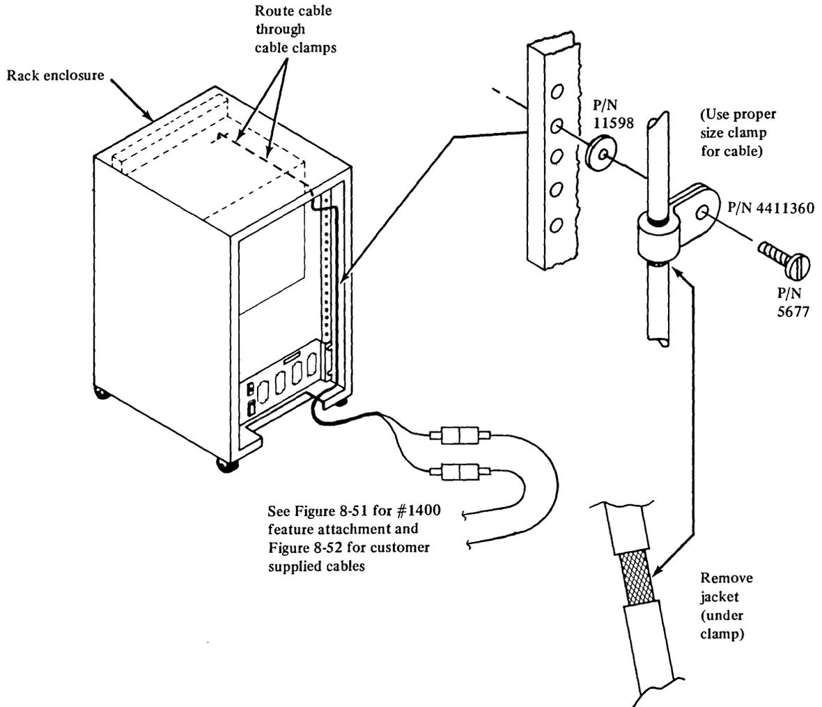
Figure 8-50. Cable routing for feature 1400
