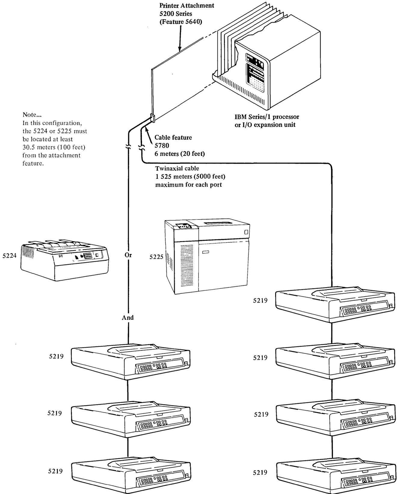
Figure 8-71. Sample configuration for feature 5640
