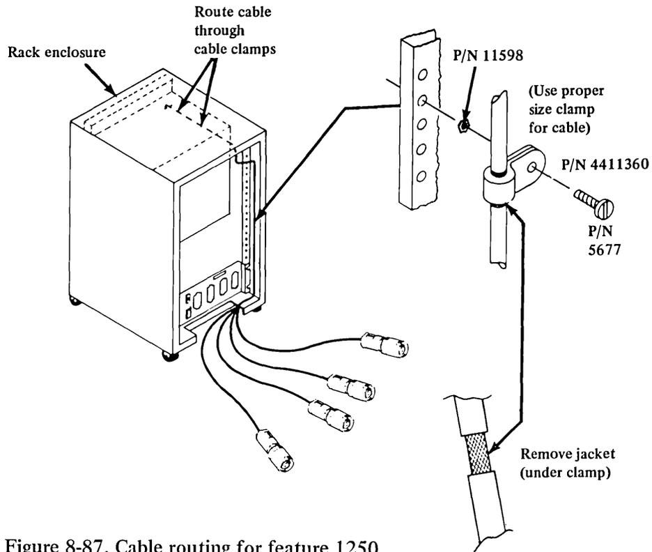
Figure 8-87. Cable routing for feature 1250
