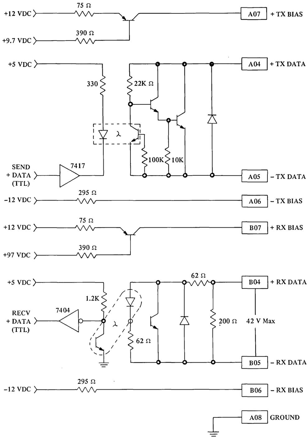
Figure 6-19 (Part 2). Current loop interface for Feature-Programmable Multi-line attachment
