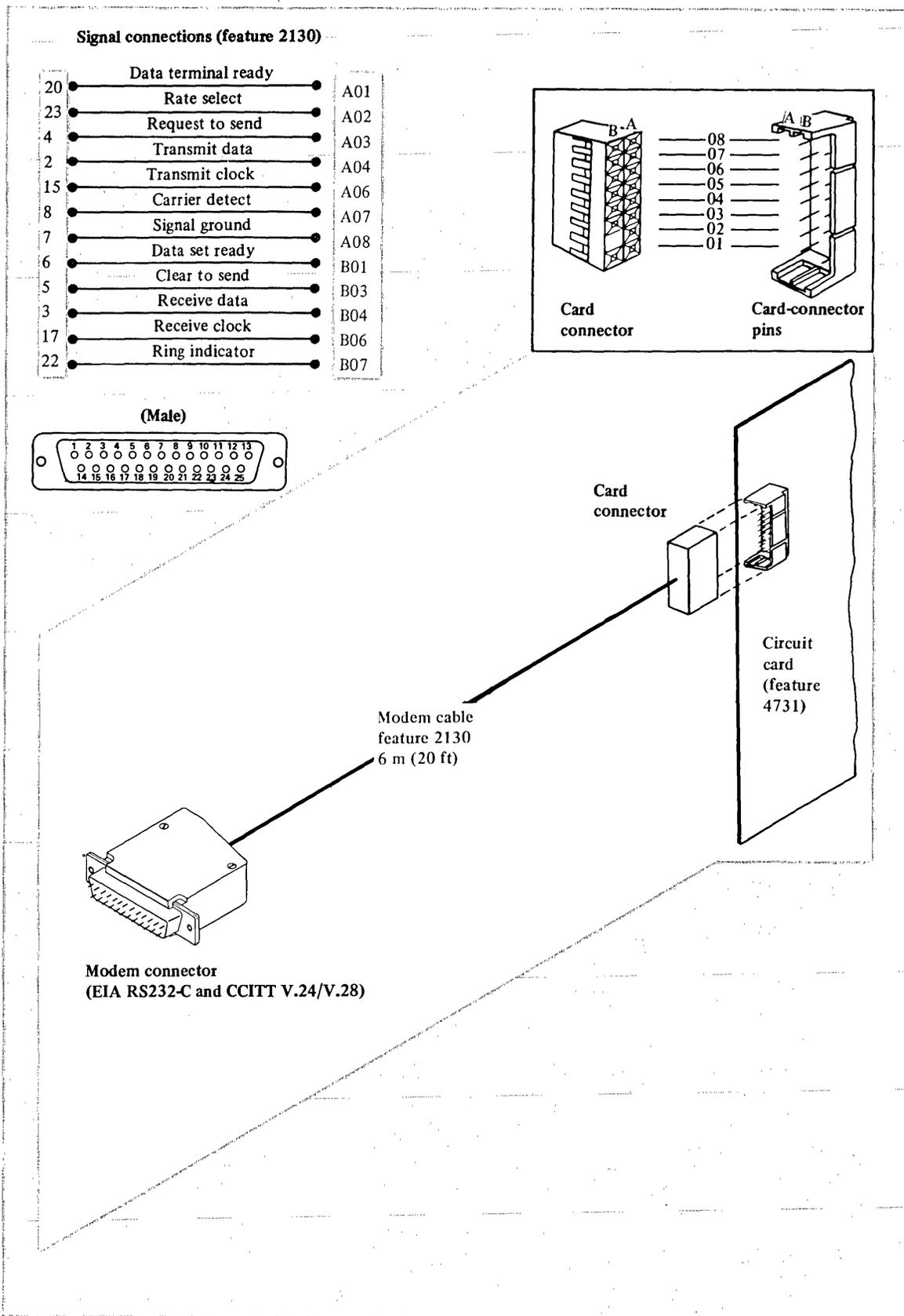
Figure 6-22. Cable and signal connections for full-duplex DCE data-set attachment feature
