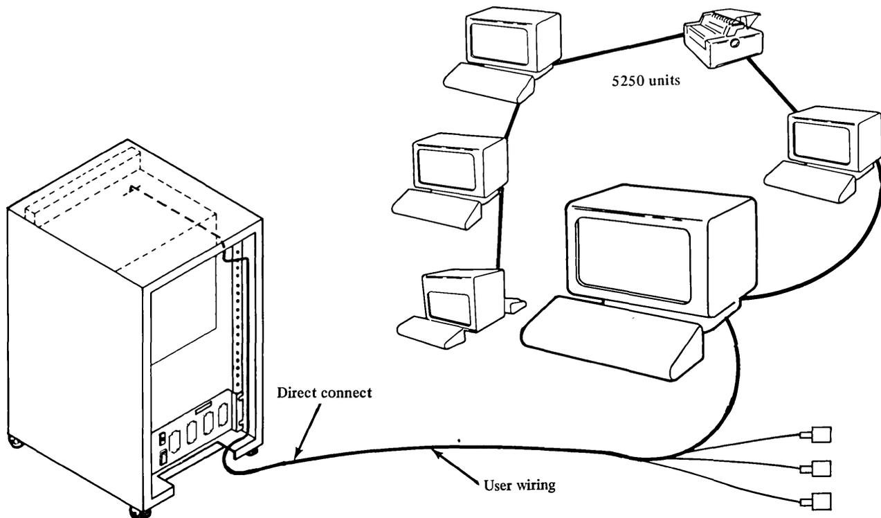
Figure 8-14. Feature 5760 and direct connect attachment
