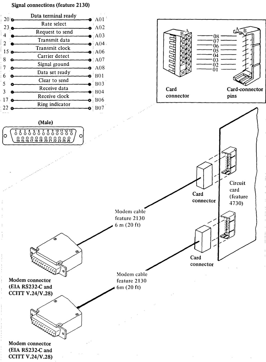
Figure 6-21. Cable and signal connections for half-duplex DCE data-set attachment feature
