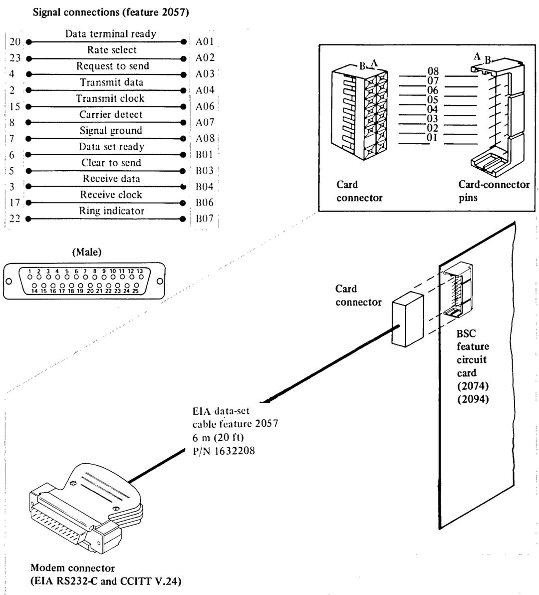
Figure 6-11. Cable and signal connections for medium-speed BSC features
