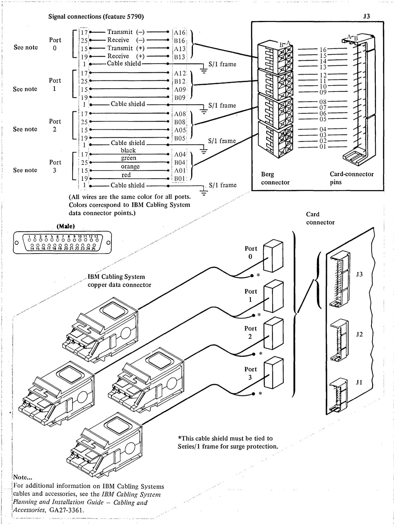
Figure 8-66 (Part 2). Feature 1310 cable and signal connections for 5790 cables
