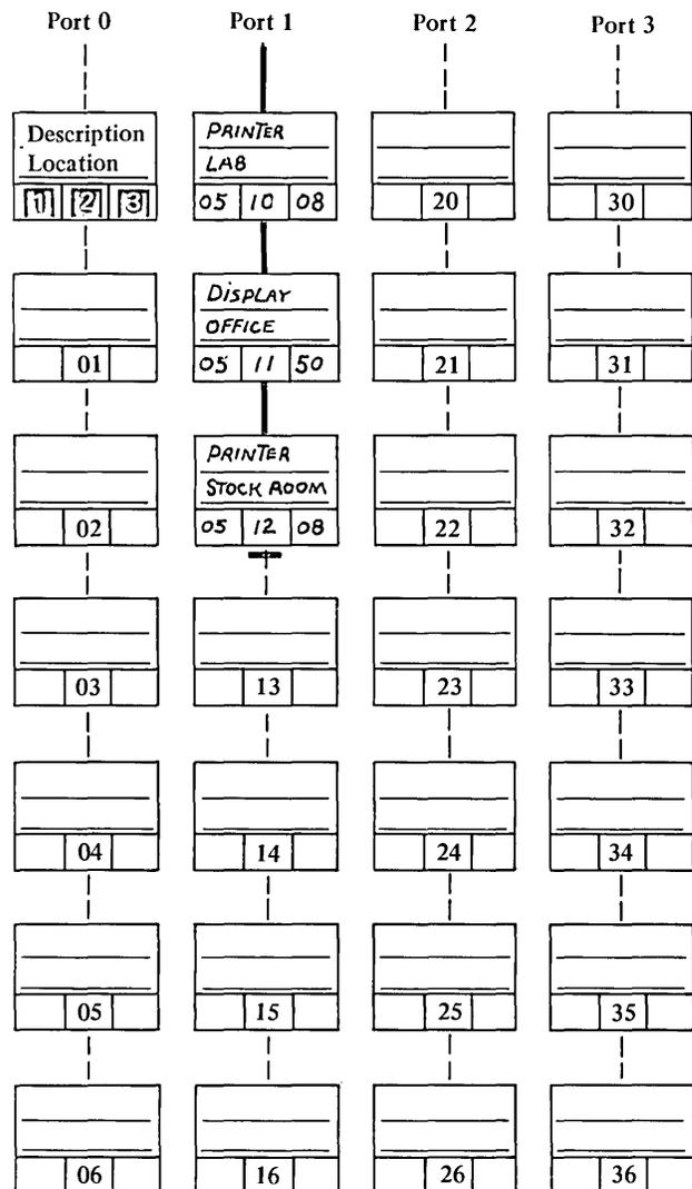
Figure 8-15. Sample 5250 Information Display System attachment planning worksheet
