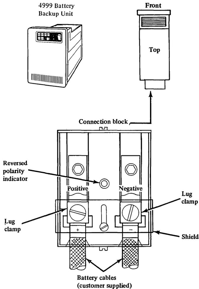
Figure 7-4. Battery connection for 4999 Battery Backup Unit
