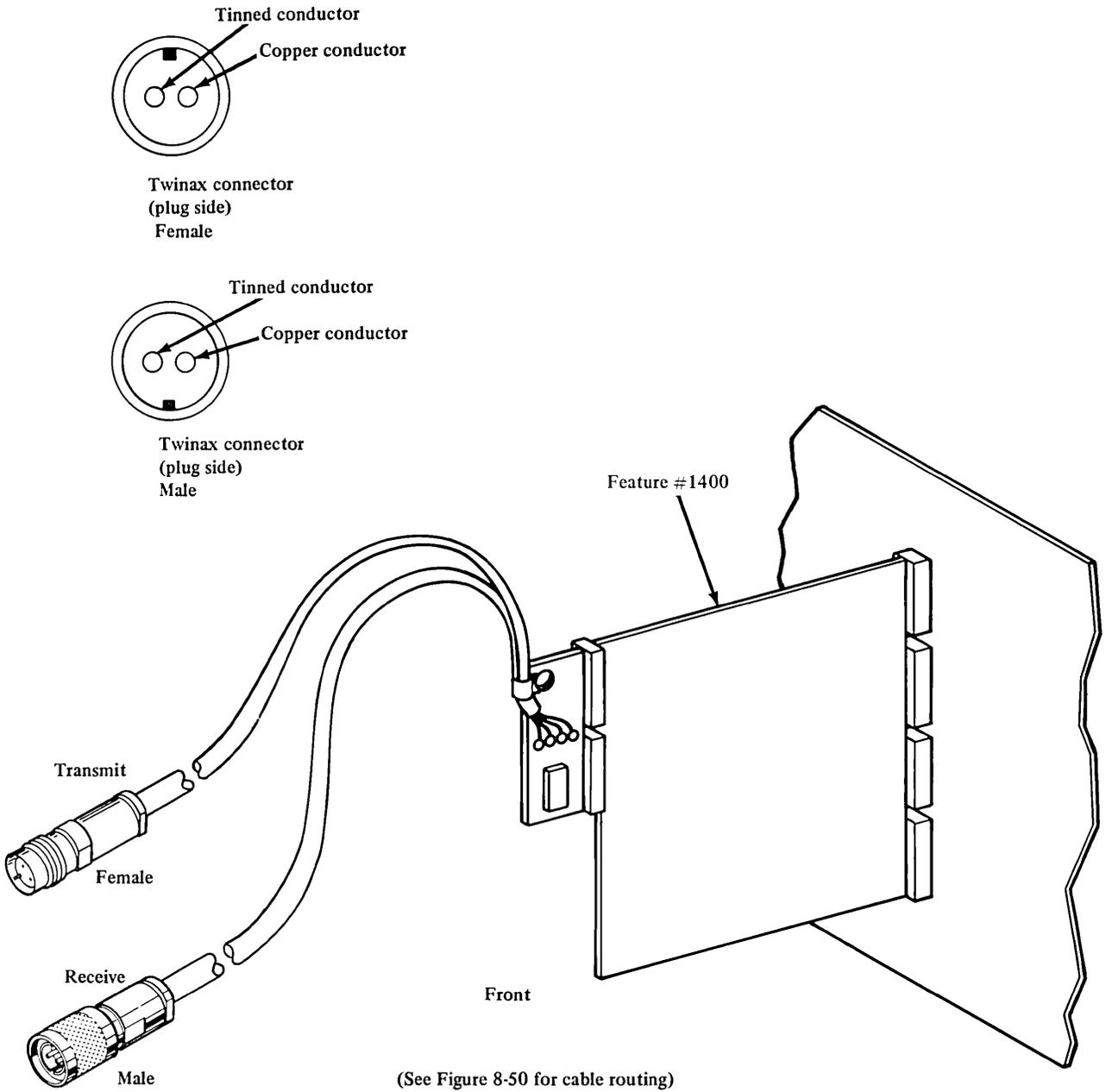
Figure 8-49. Cable connections for feature 1400
