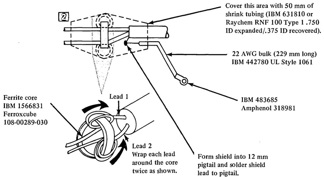
Figure 8-74. Cable assembly for feature 5640
