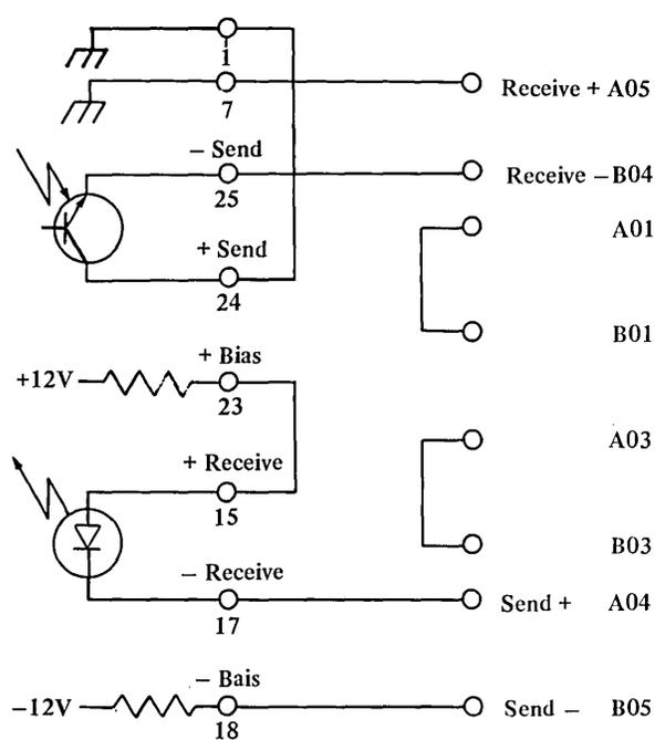
Current loop with feature 2096 supplying all current (attach to 3101)
