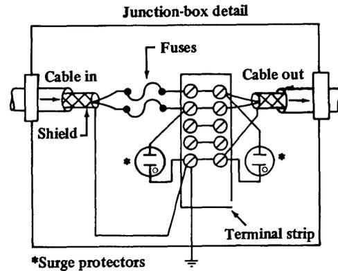
Figure 8-5. Sample shunt-type lightning protector
