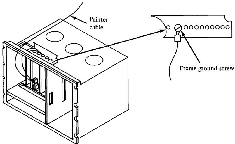
Figure 8-88. Card file cable installation for feature 1250
