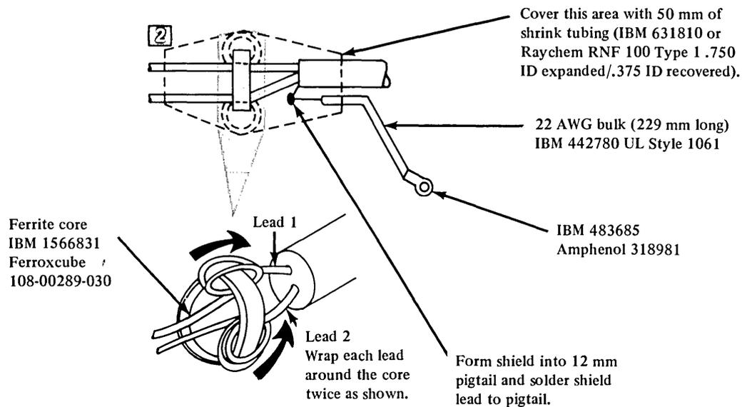
Figure 8-86. Cable assembly for feature 1250
