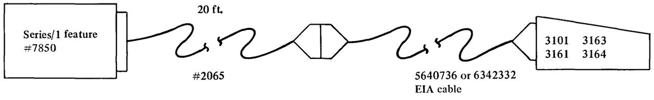
**Figure 8-20. 3101, 3161, 3163, 3164 teletypewriter adapter cable with EIA female connector**
