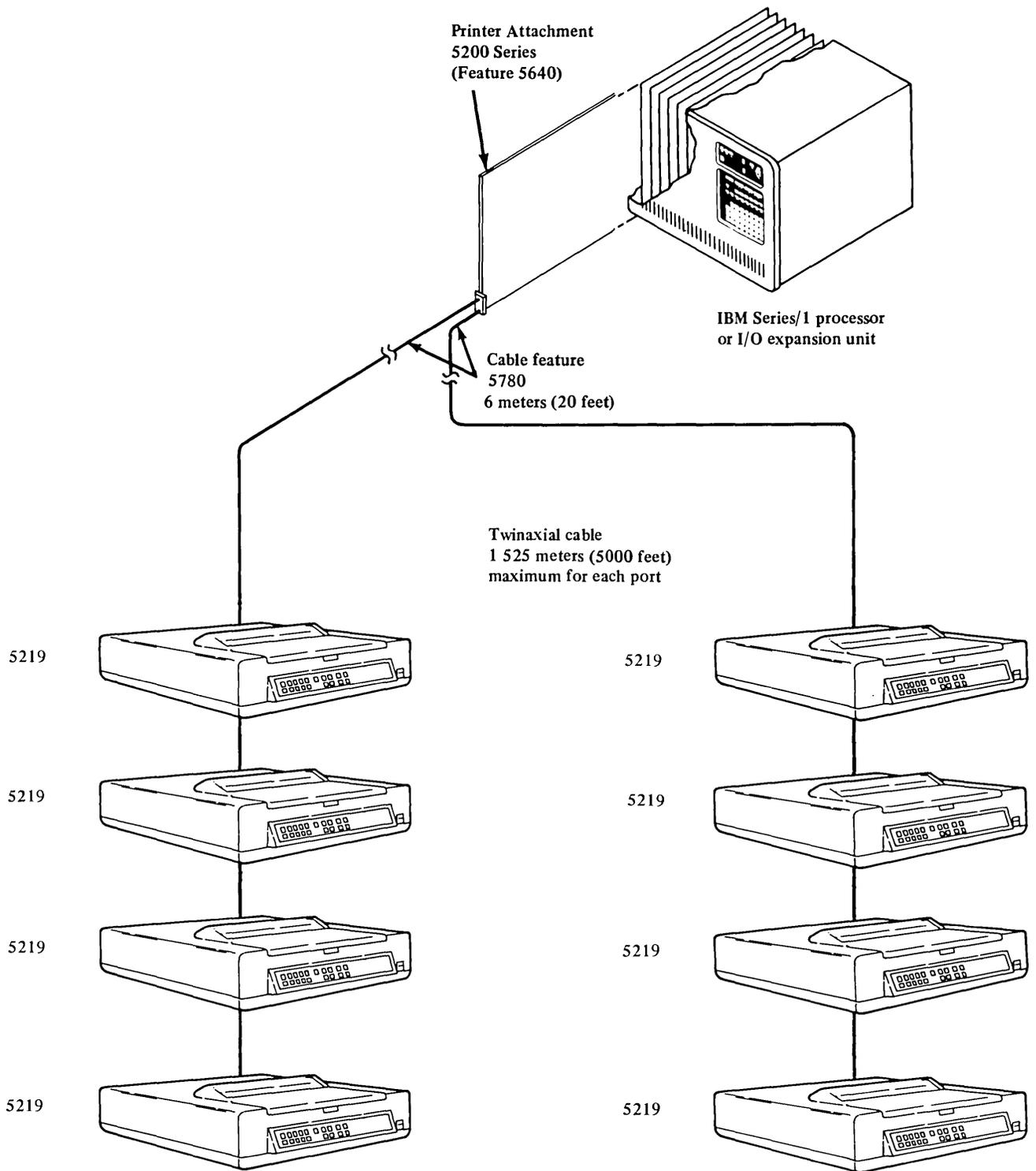
Figure 8-72. Sample configuration for feature 5640
