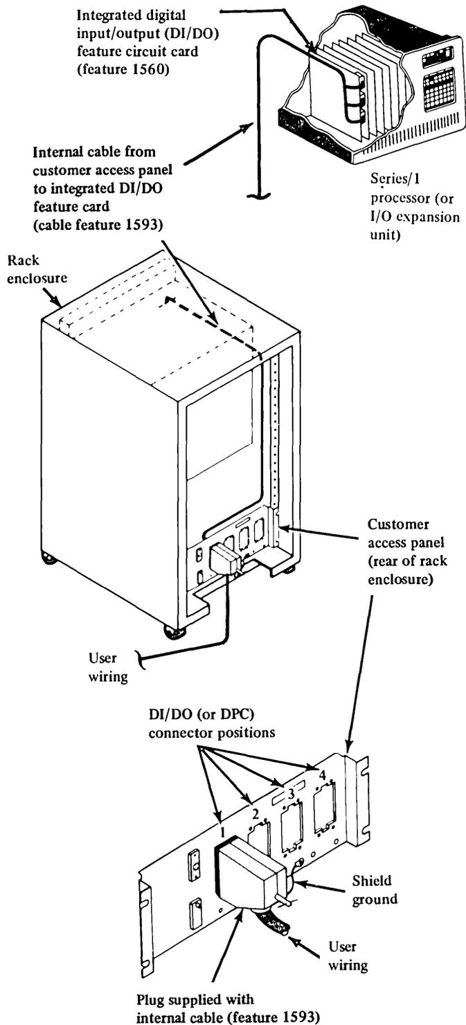
Figure 8-32. User connection to customer access panel for integrated DI/DO feature
