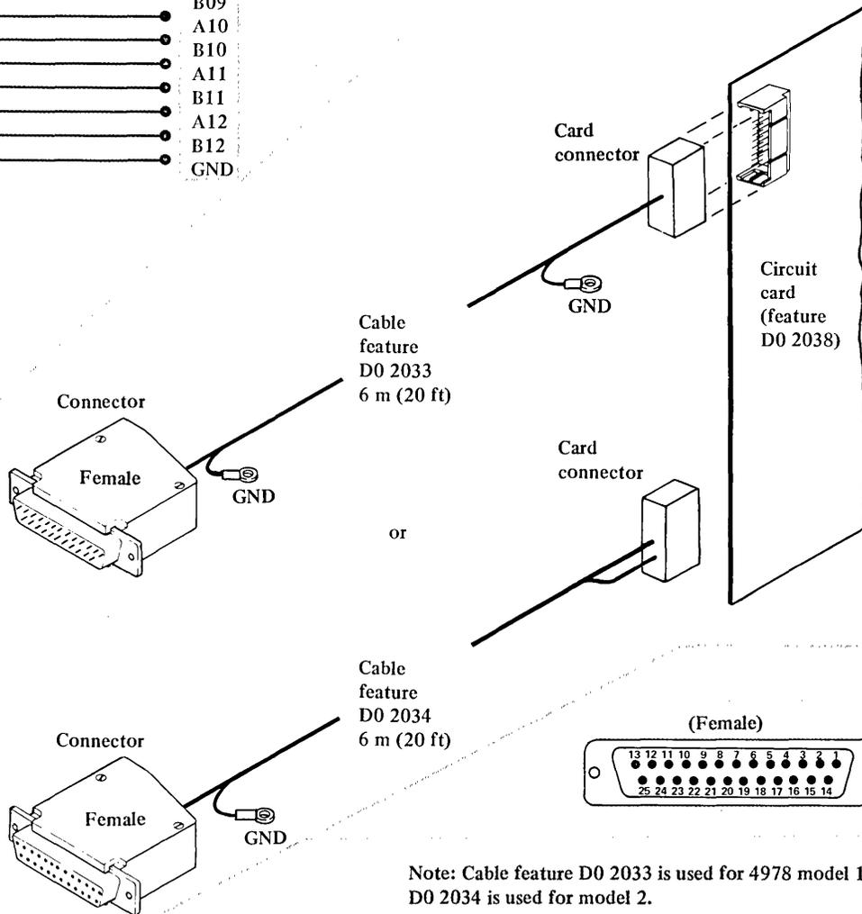
Figure 8-43. Cable connections for 4978 display station attachment
