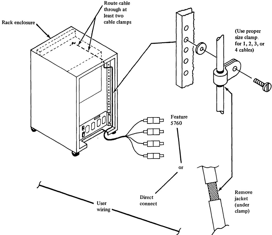
Figure 8-13. Cable routing for feature 5760 or direct connect
