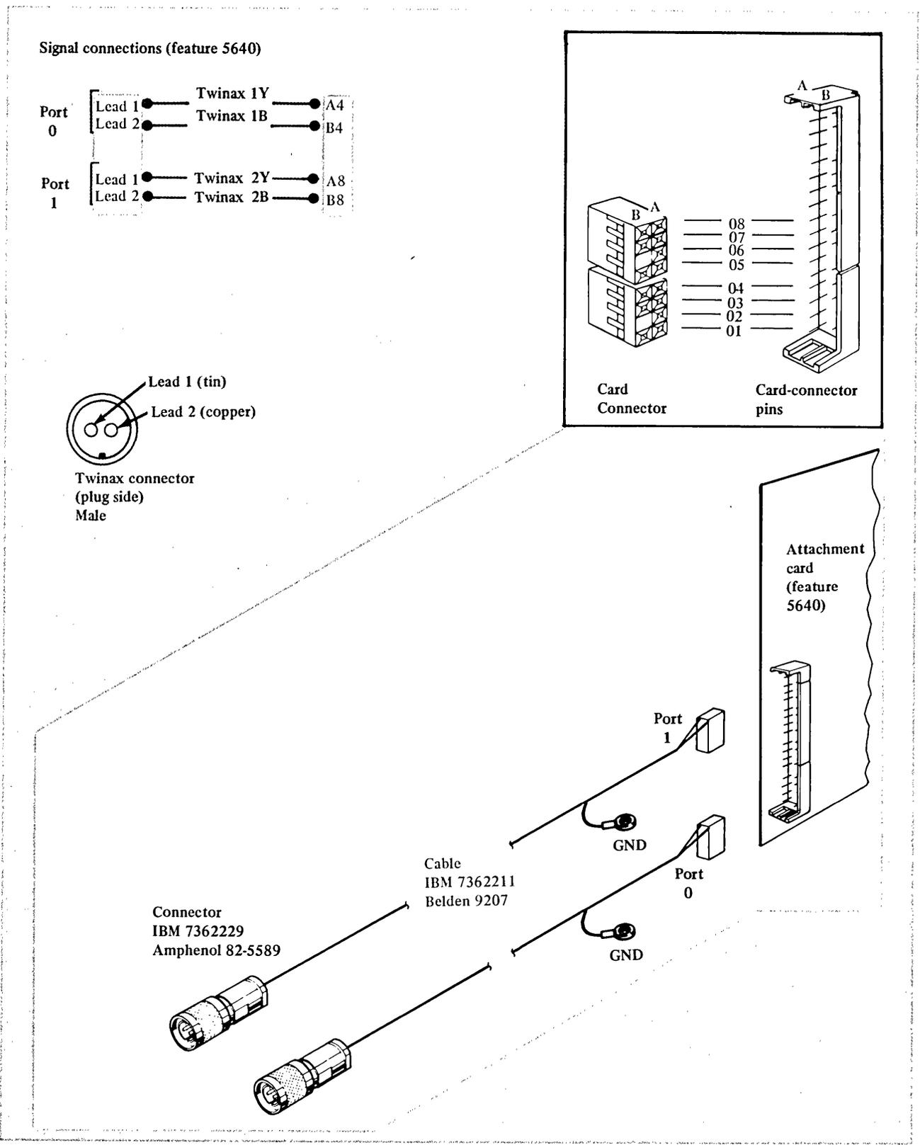
Figure 8-73. Feature 5640 cable and signal connections for 5780 cables
