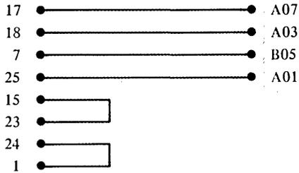
Current loop with feature 7850 supplying all current (attached to 3101)
