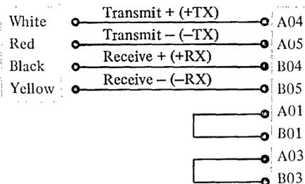
Figure 6-18. Cable and signal connections for Feature-Programmable Multi-Line attachment
