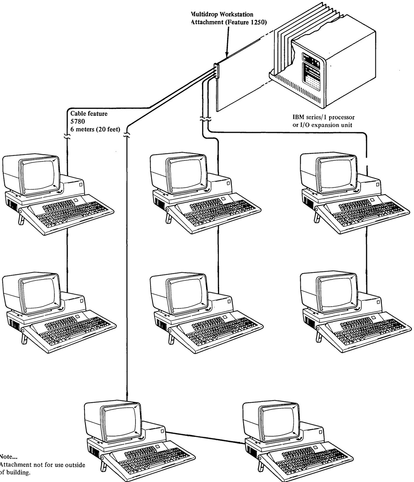
Figure 8-84 (Part 1). Sample configuration for feature 1250 (Twinaxial media)
