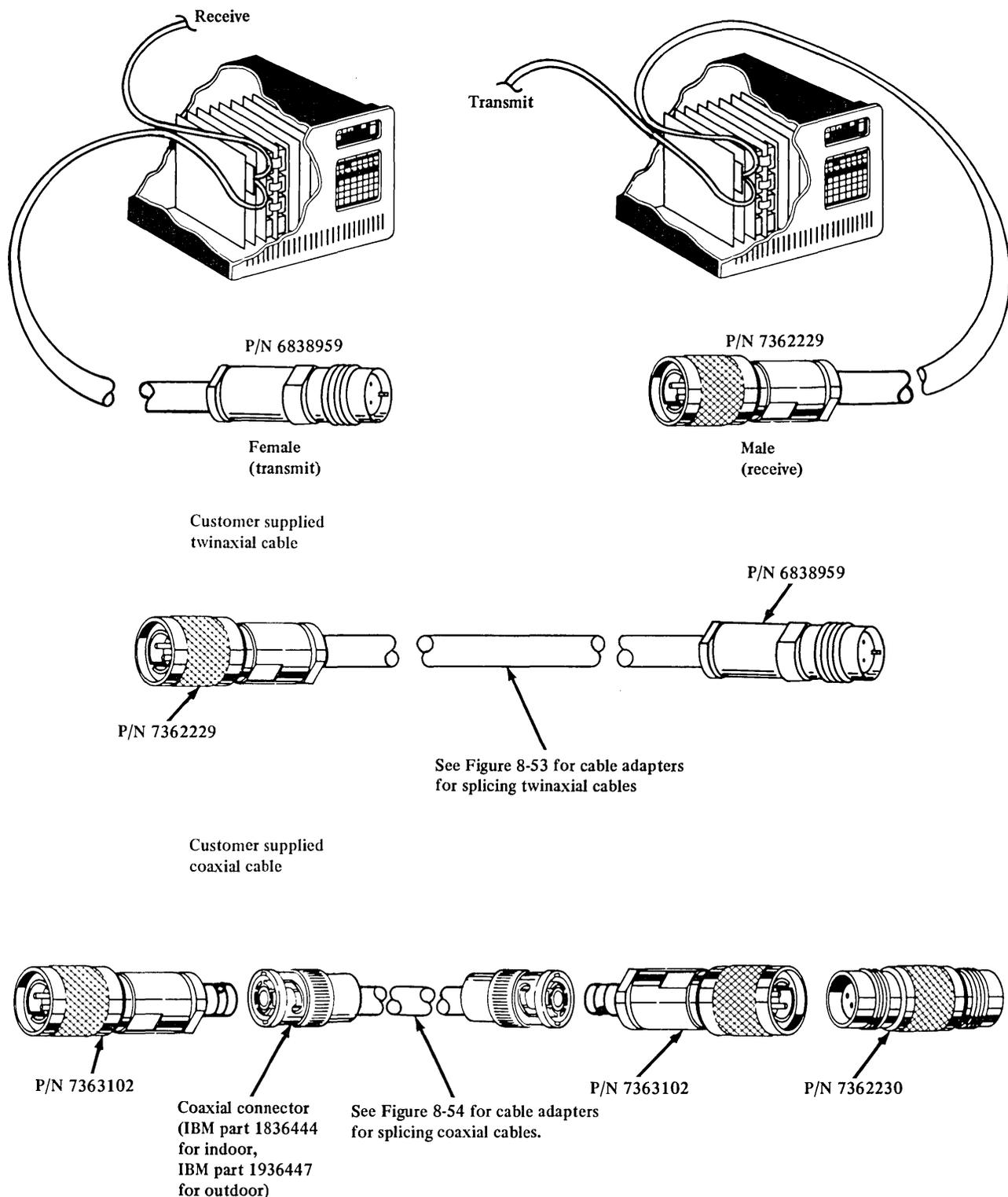
Figure 8-52. Customer supplied cable attachment
