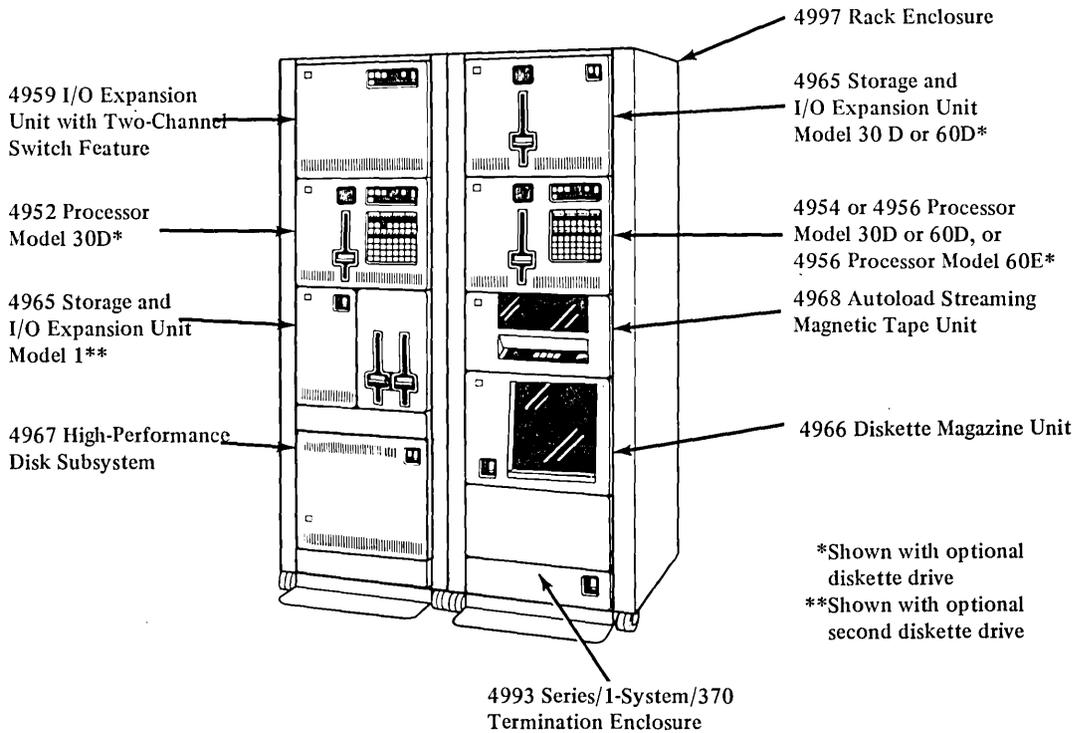
Figure 2-1. (Part 2 of 3) Series/1 machine units
